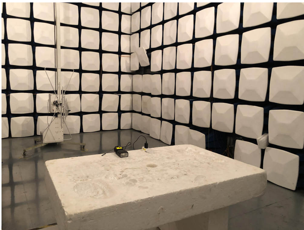
Test Setup Photo(s) of Radiated Emissions Measurement
