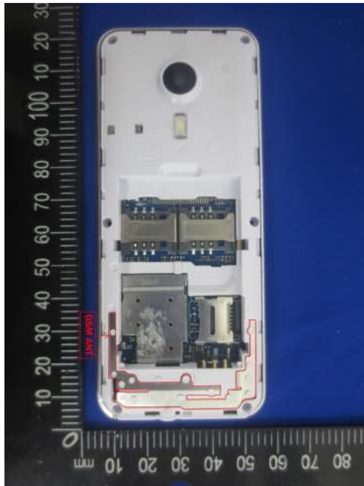
Fig.14.1 EUT Antenna Locations
