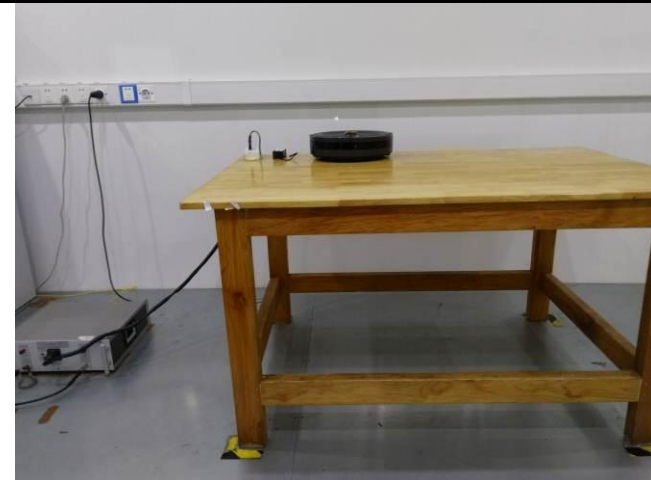
Conducted Emissions Test Setup Front View
