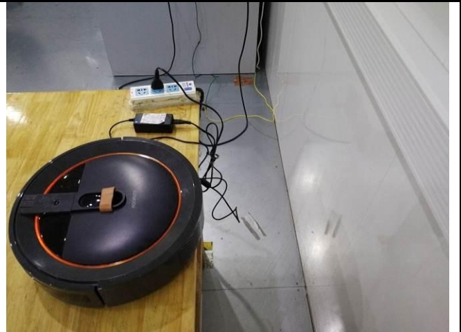
Conducted Emissions Test Setup Side View
