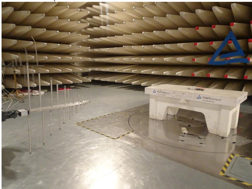
Test setup Frequency Range 200MHz-1GHz Log periodic Antenna(ECG Simulation mode)
