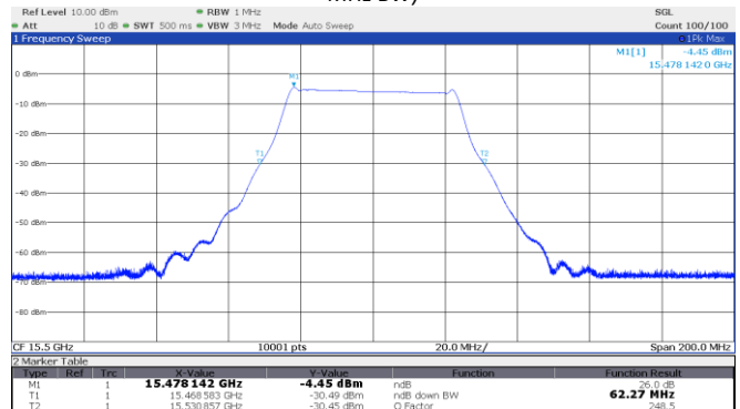
Figure 8.2-12: 26 dB OBW Low channel: 15.50 GHz, shortest pulse (50 MHz BW)
