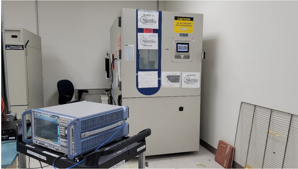
Figure 18 – Test setup: Frequency stability, antenna conducted port.
