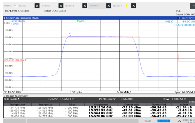
Figure 8.4-5: Emission mask, Middle channel: 15.55 GHz, longest pulse. (25 MHz BW)
