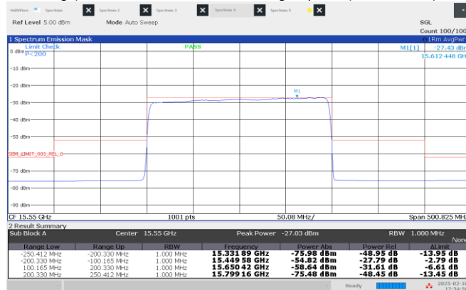
Figure 8.4-23: Emission mask, Middle channel: 15.55 GHz, longest pulse. (200 MHz BW)
