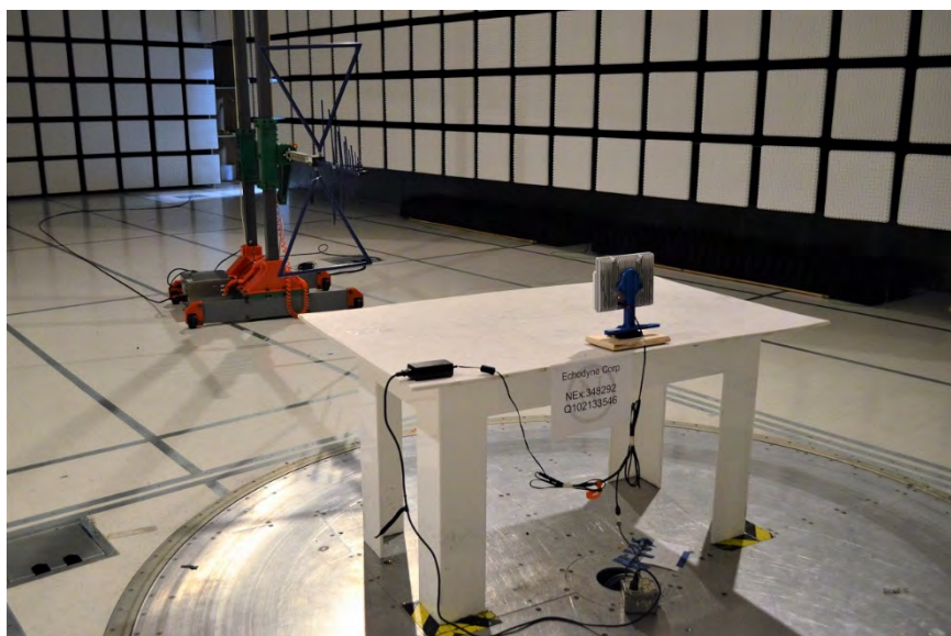
Figure 3.6-2: Radiated Emissions Test Setup – below 1GHz (Back)
