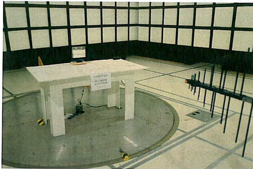
Figure 3.6-1: Radiated Emissions Test Setup – below 1GHz (Front)
