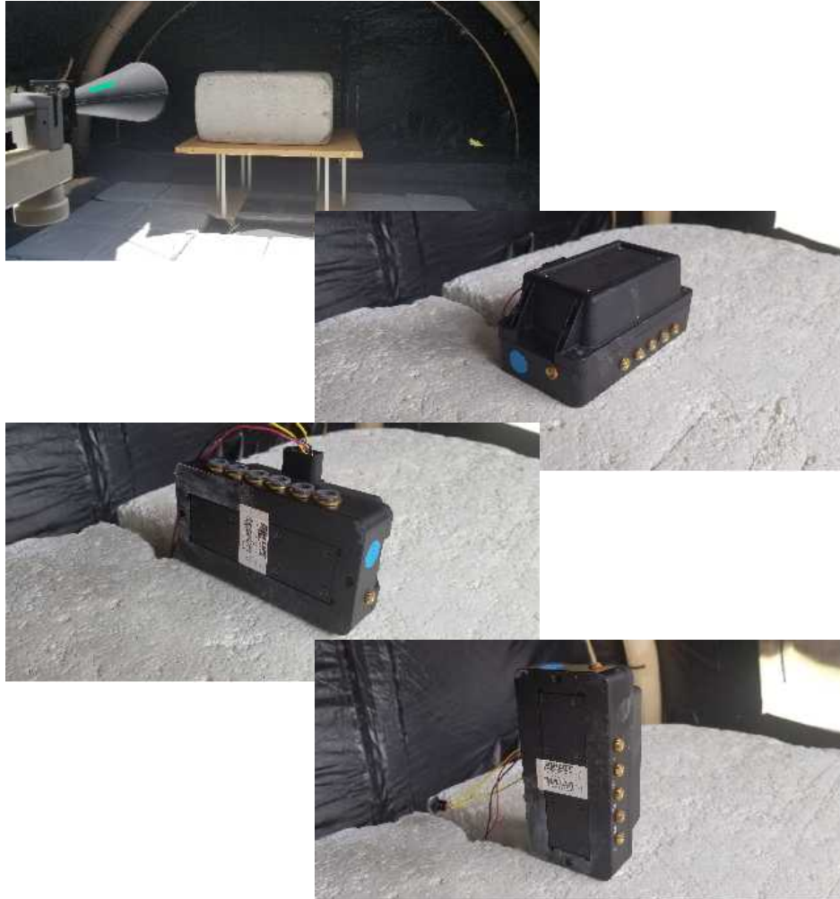
Figure 4: Radiated Emissions Test Setup Photograph(s).
