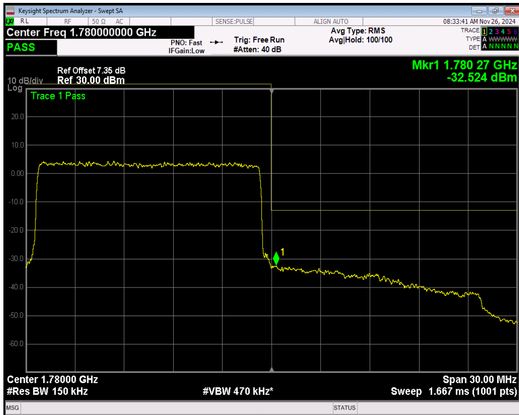
Band66 16QAM BW=15MHz Channel=132597 RB Size=1 Position=#0
