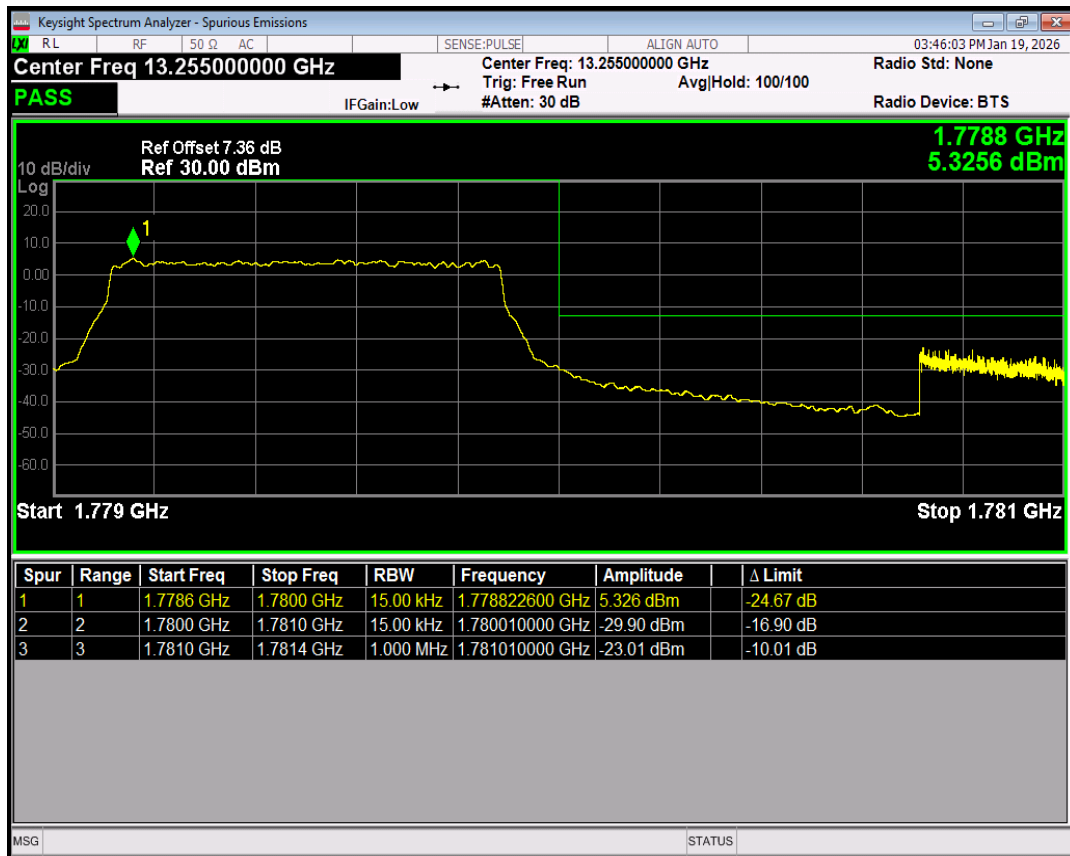
Band66 16QAM BW=1.4MHz Channel=132665 RB Size=1 Position=#0
