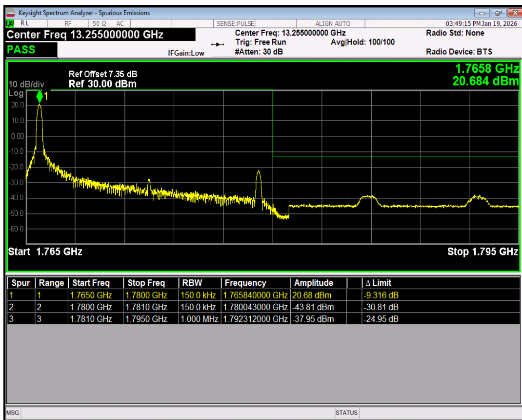
Band66 QPSK BW=15MHz Channel=132597 RB Size=1 Position=#Max
