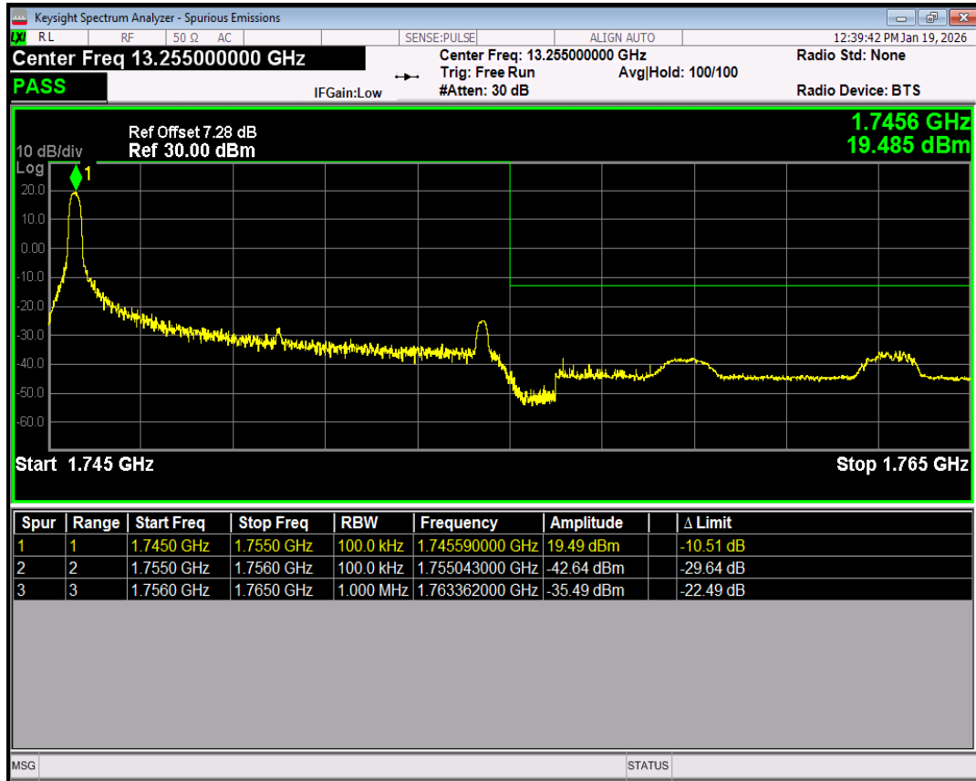
Band4 16QAM BW=10MHz Channel=20350 RB Size=1 Position=#Max
