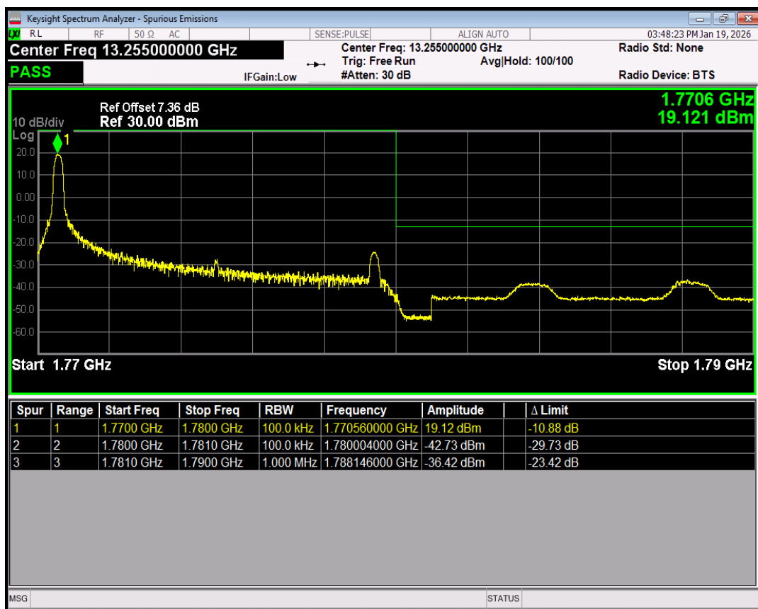
Band66 QPSK BW=10MHz Channel=132622 RB Size=1 Position=#Max
