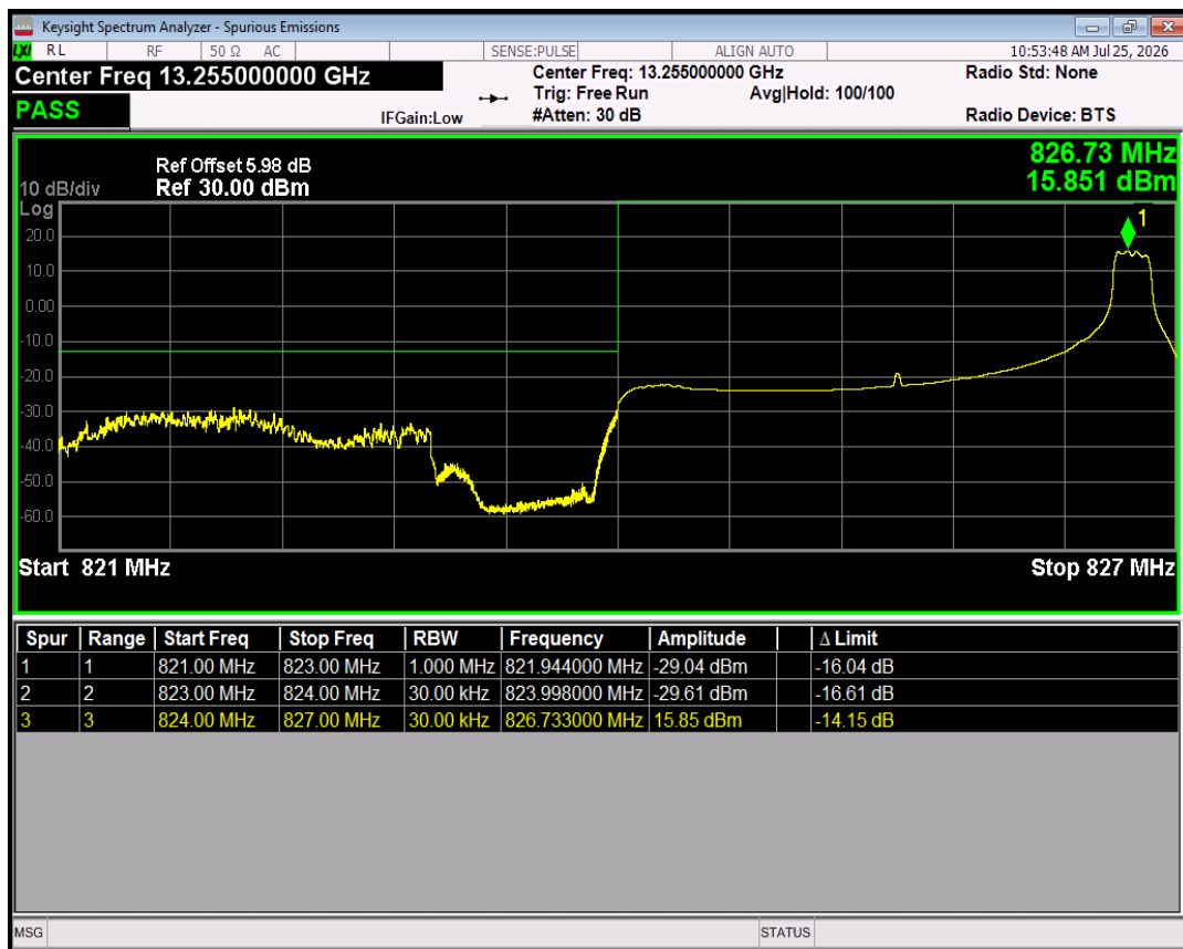
Band5 16QAM BW=3MHz Channel=20415 RB Size=15 Position=#0
