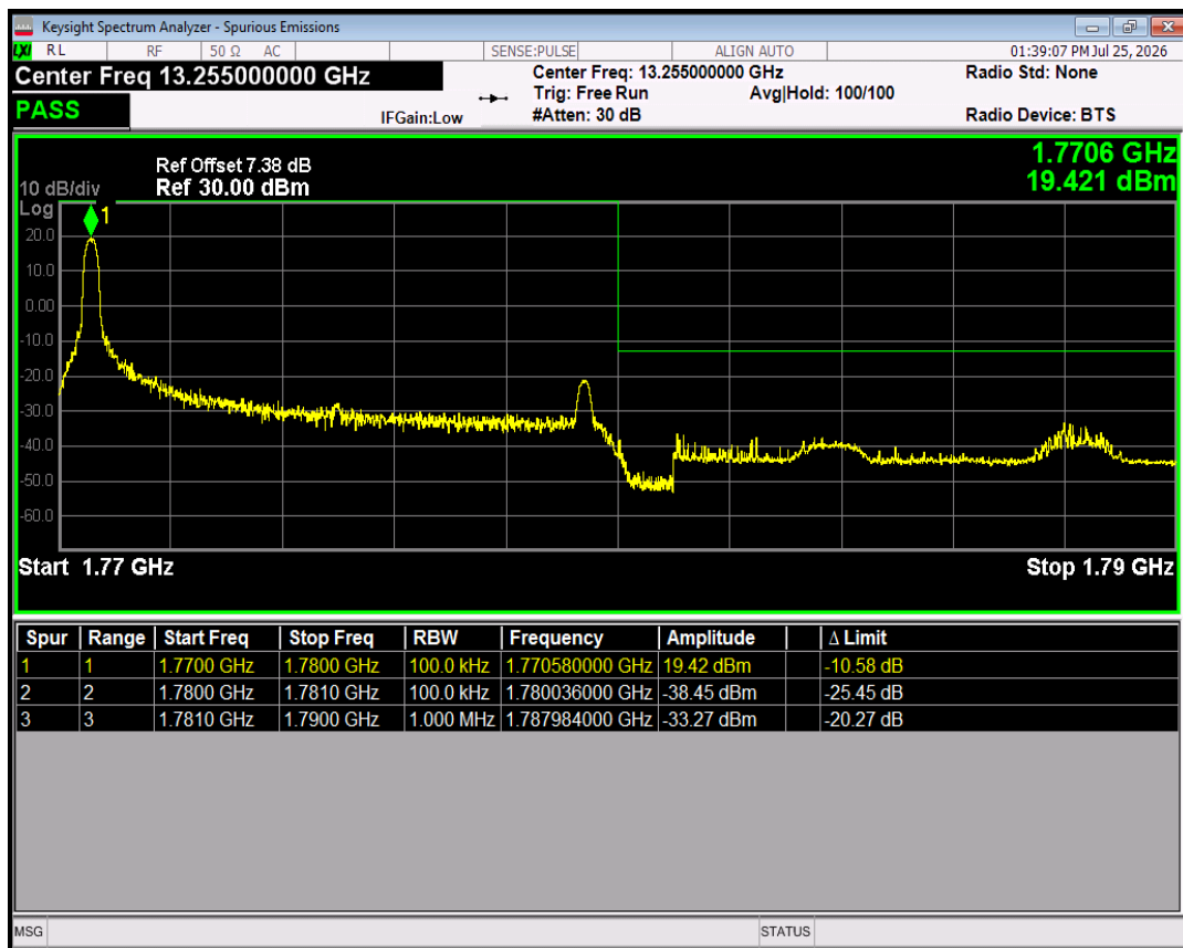
Band66 QPSK BW=10MHz Channel=132622 RB Size=1 Position=#Max
