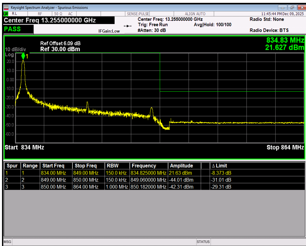
Band26(824-849) QPSK BW=15MHz Channel=26965 RB Size=1 Position=#Max
