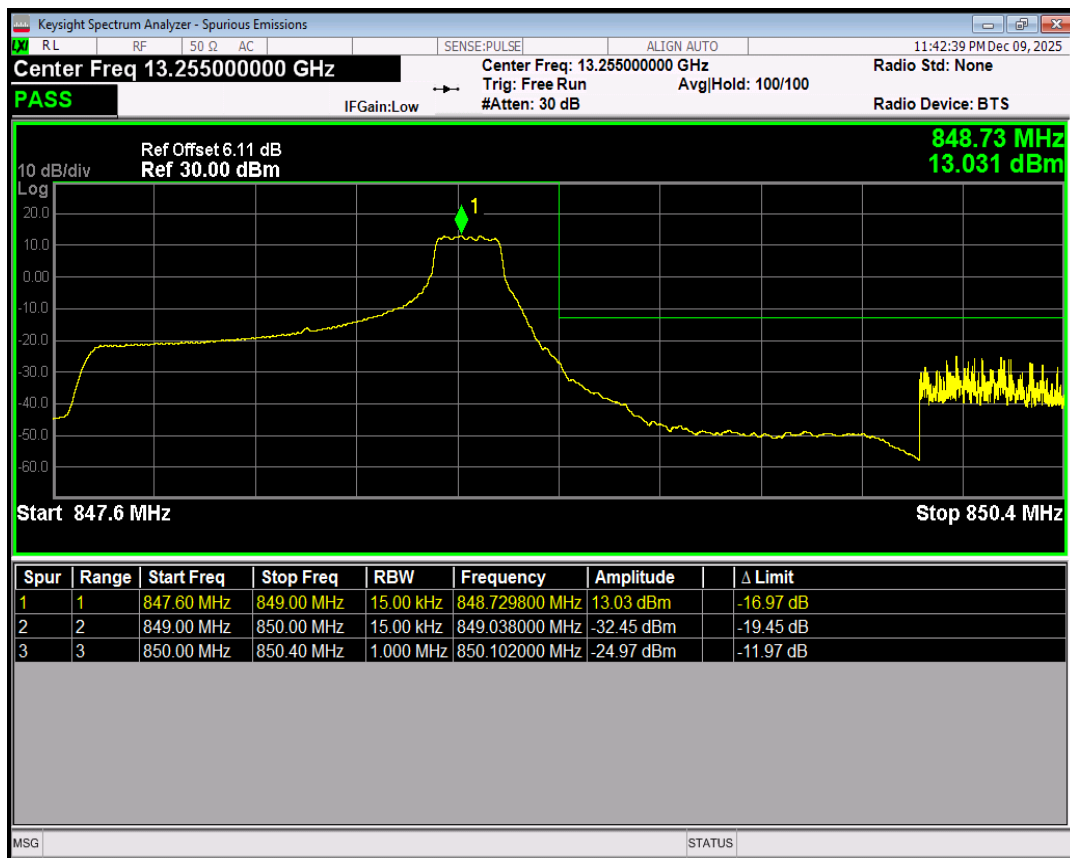
Band26(824-849) 16QAM BW=1.4MHz Channel=27033 RB Size=6 Position=#0
