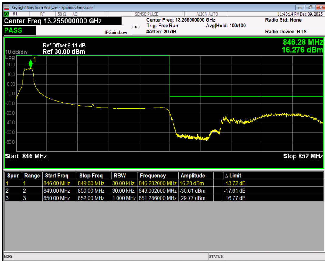
Band26(824-849) QPSK BW=3MHz Channel=27025 RB Size=1 Position=#Max
