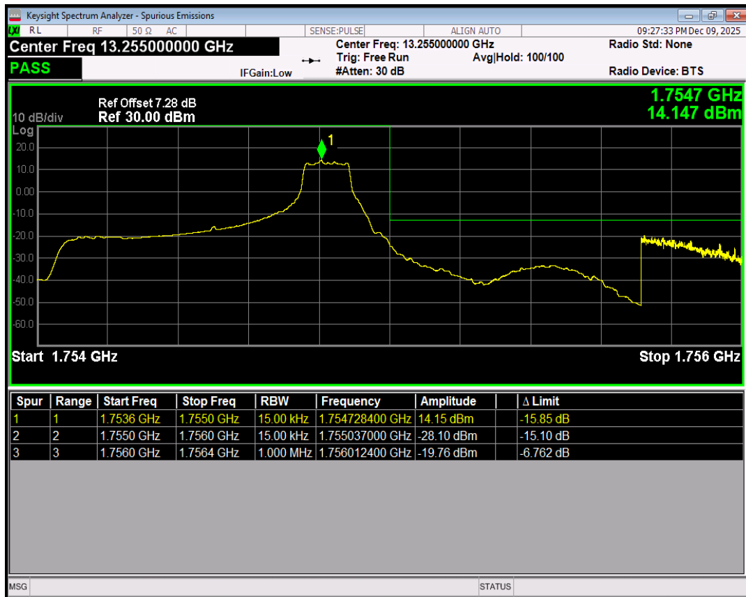
Band4 16QAM BW=1.4MHz Channel=20393 RB Size=6 Position=#0
