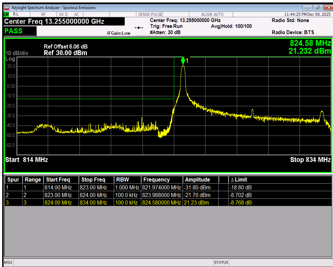
Band26(824-849) QPSK BW=10MHz Channel=26840 RB Size=1 Position=#Max
