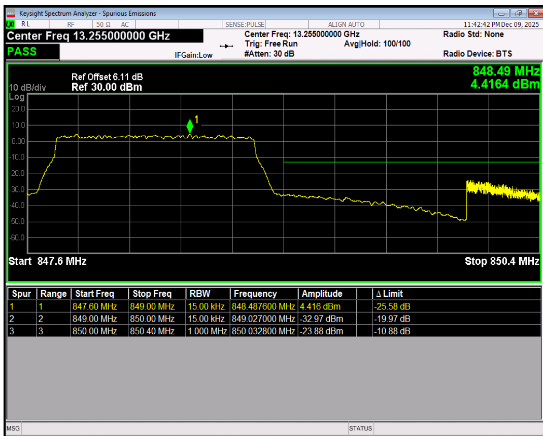
Band26(824-849) QPSK BW=3MHz Channel=26805 RB Size=1 Position=#0
