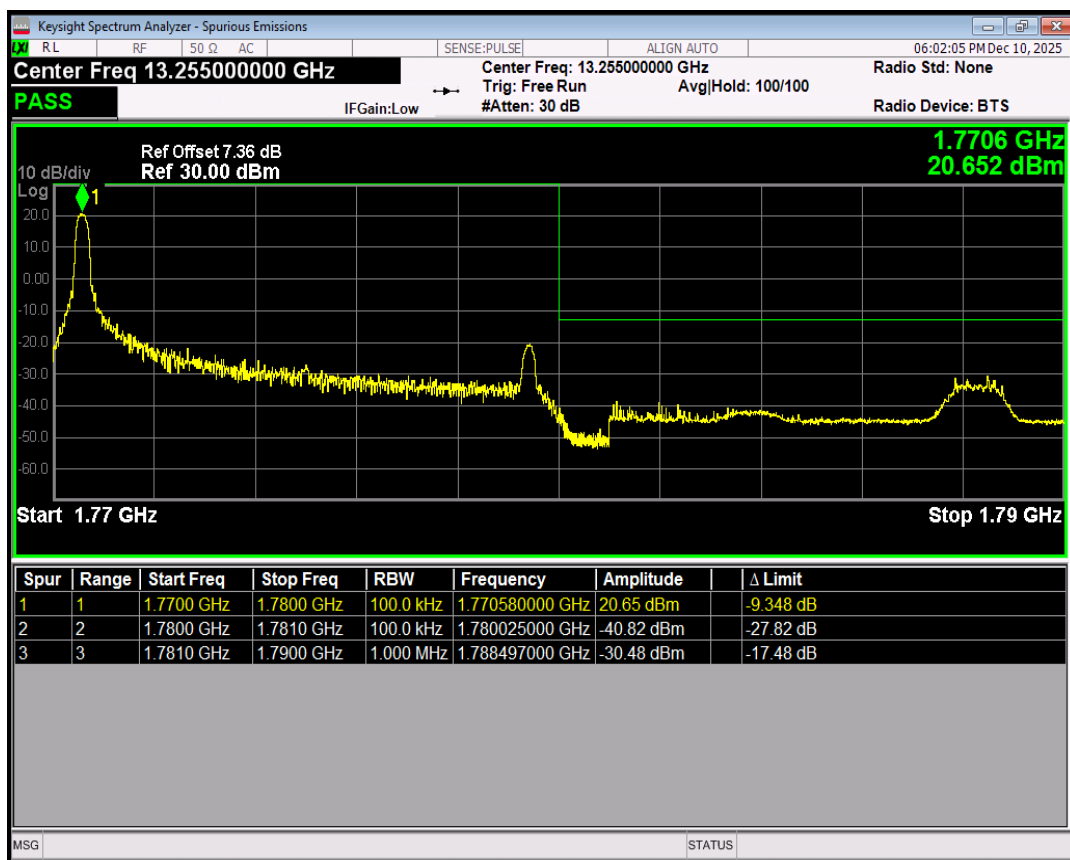
Band66 16QAM BW=10MHz Channel=132622 RB Size=50 Position=#0
