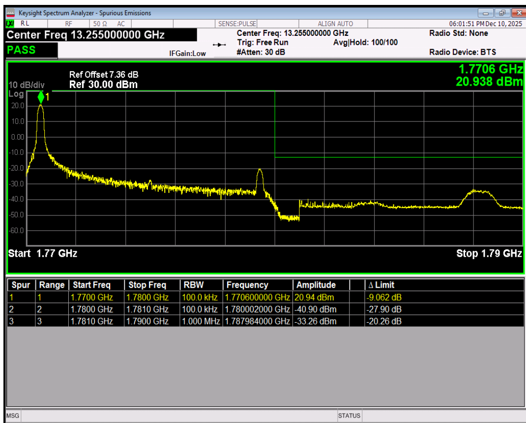
Band66 QPSK BW=10MHz Channel=132622 RB Size=1 Position=#Max
