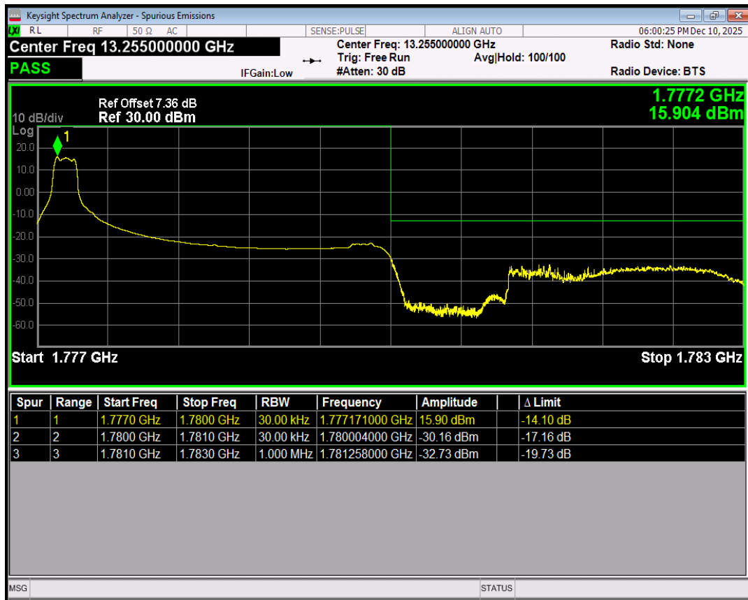
Band66 16QAM BW=3MHz Channel=132657 RB Size=1 Position=#Max
