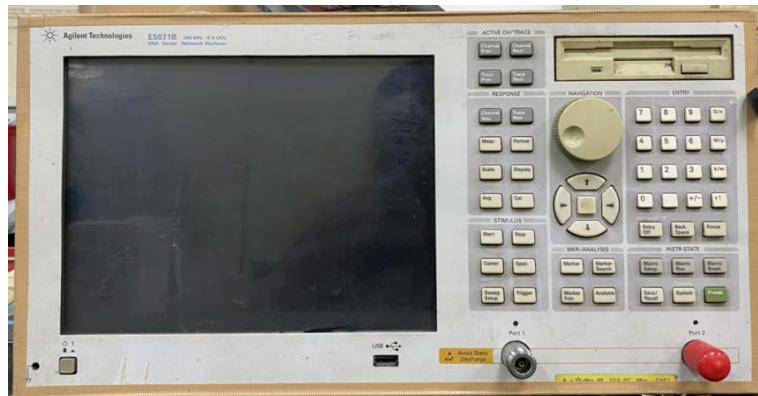
Agilent 5071B (S Parameter (RL/VSWR) Test Equipment)
