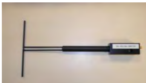
Figure 1 – MVG COMOSAR Validation Dipole
