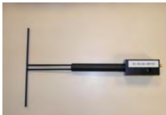
Figure 1 – MVG COMOSAR Validation Dipole
