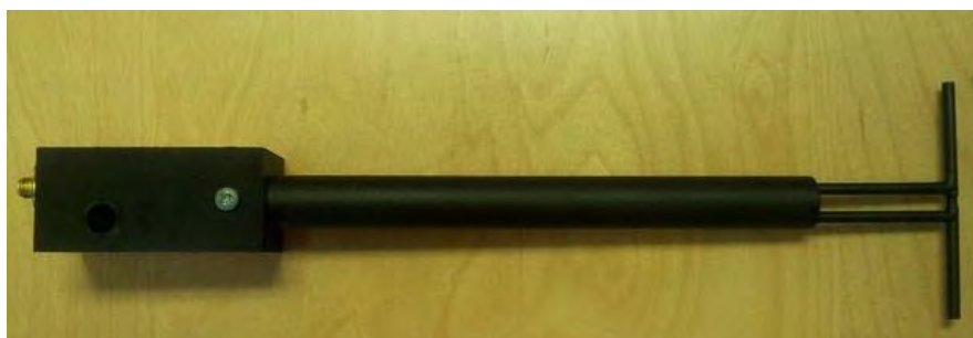
Figure 1 – MVG COMOSAR Validation Dipole
