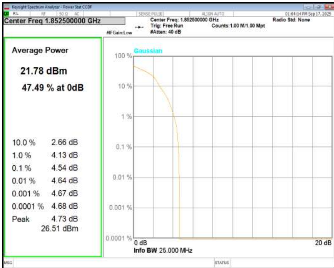
Band2 16QAM BW=5MHz Channel=19175 RB Size=1 Position=#0
