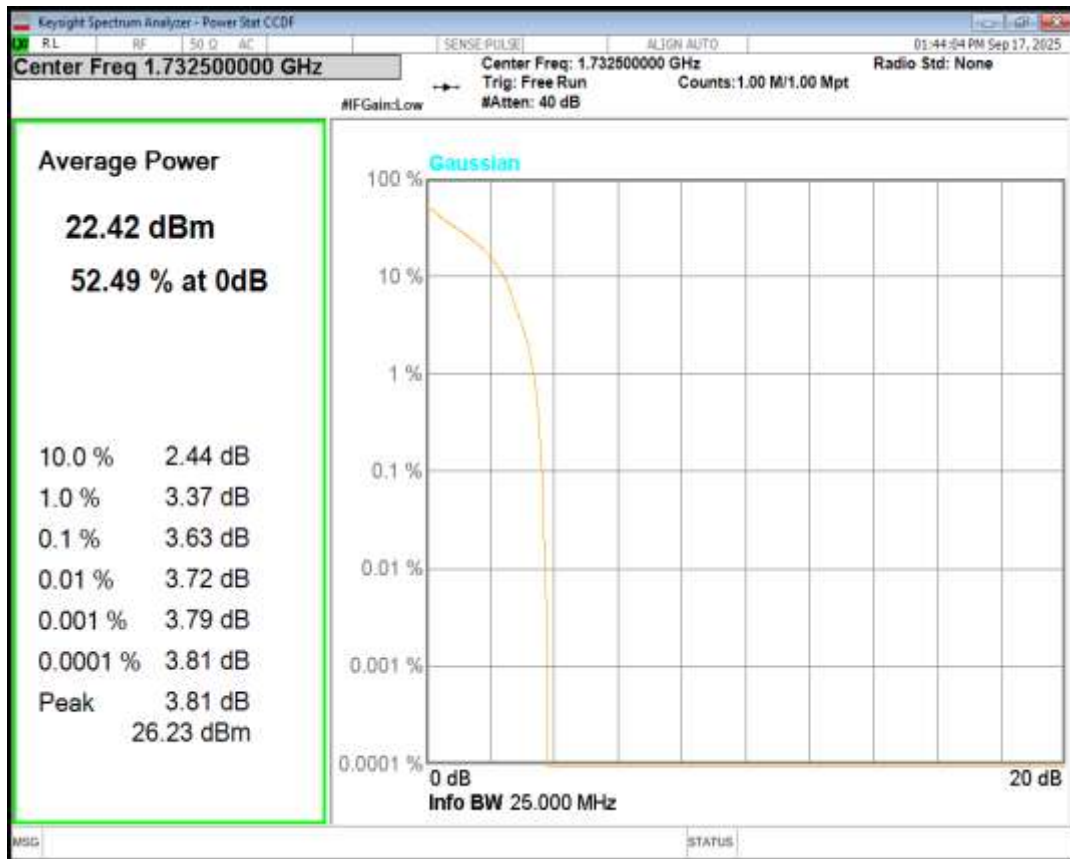
Band4 16QAM BW=5MHz Channel=20375 RB Size=1 Position=#0
