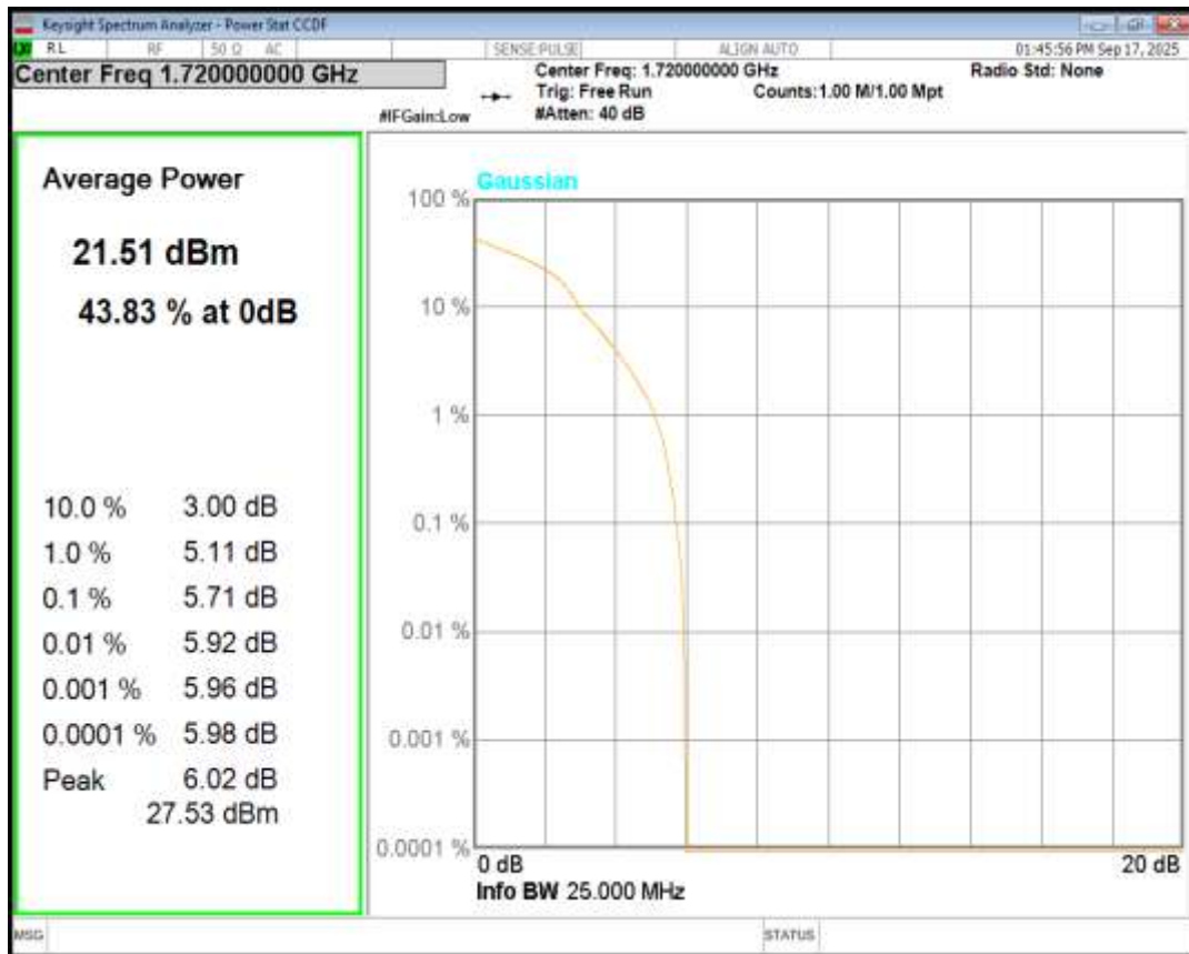
Band4 16QAM BW=20MHz Channel=20175 RB Size=1 Position=#0
