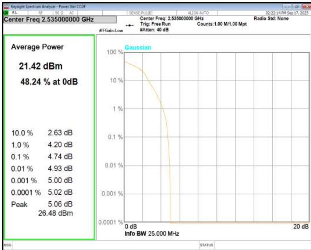
Band7 16QAM BW=10MHz Channel=21400 RB Size=1 Position=#0
