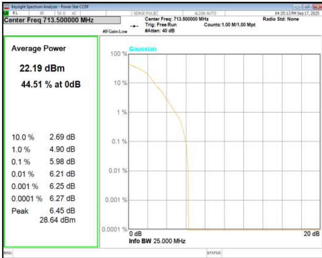
Band12 16QAM BW=3MHz Channel=23165 RB Size=1 Position=#0
