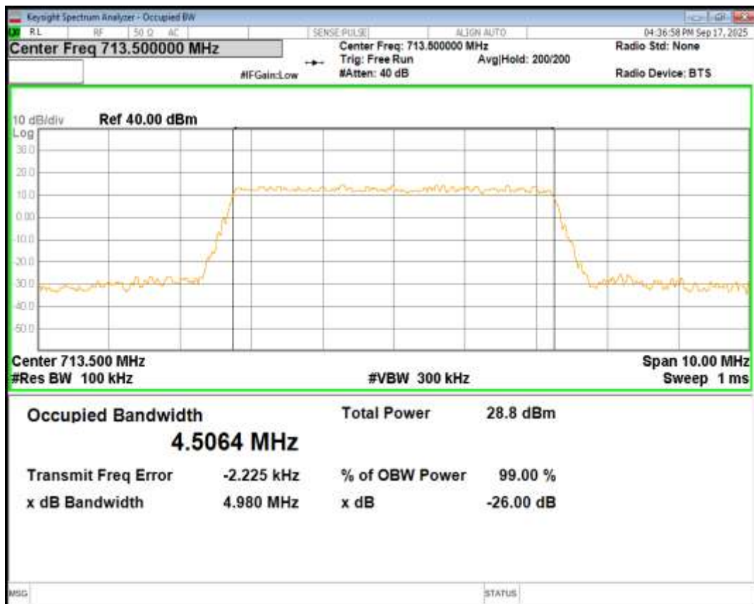
Band12 QPSK BW=1.4MHz Channel=23017 RB Size=6 Position=#0
