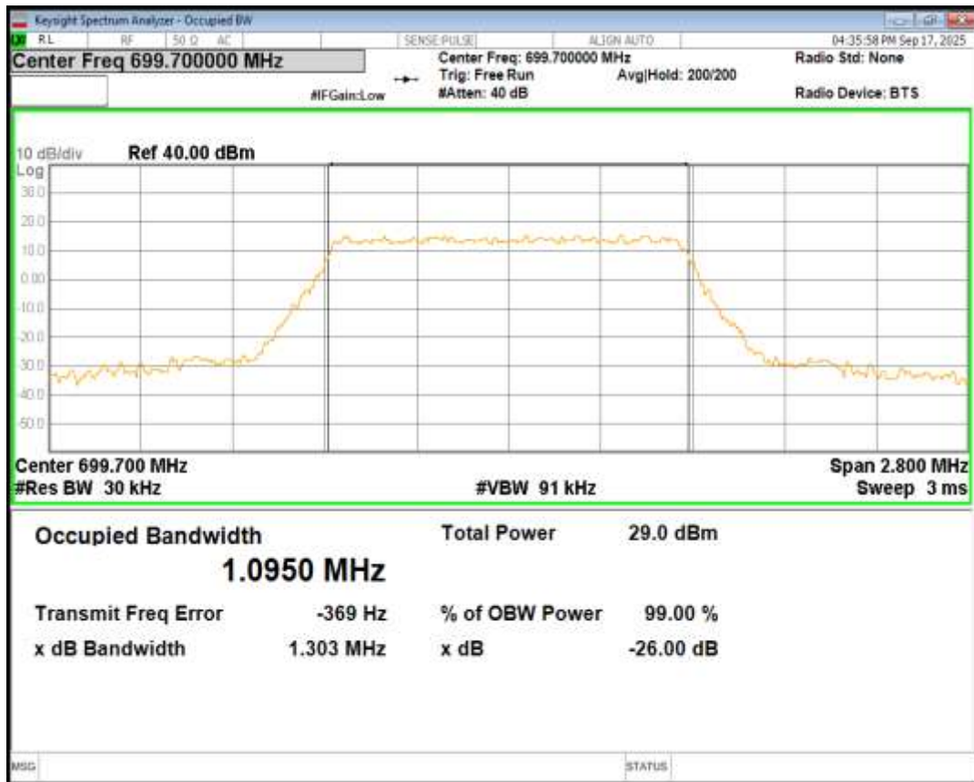
Band12 16QAM BW=1.4MHz Channel=23095 RB Size=6 Position=#0
