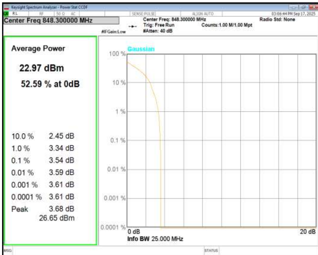
Band5 QPSK BW=10MHz Channel=20450 RB Size=1 Position=#0
