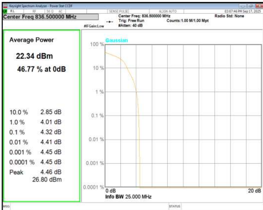
Band5 16QAM BW=10MHz Channel=20600 RB Size=1 Position=#0
