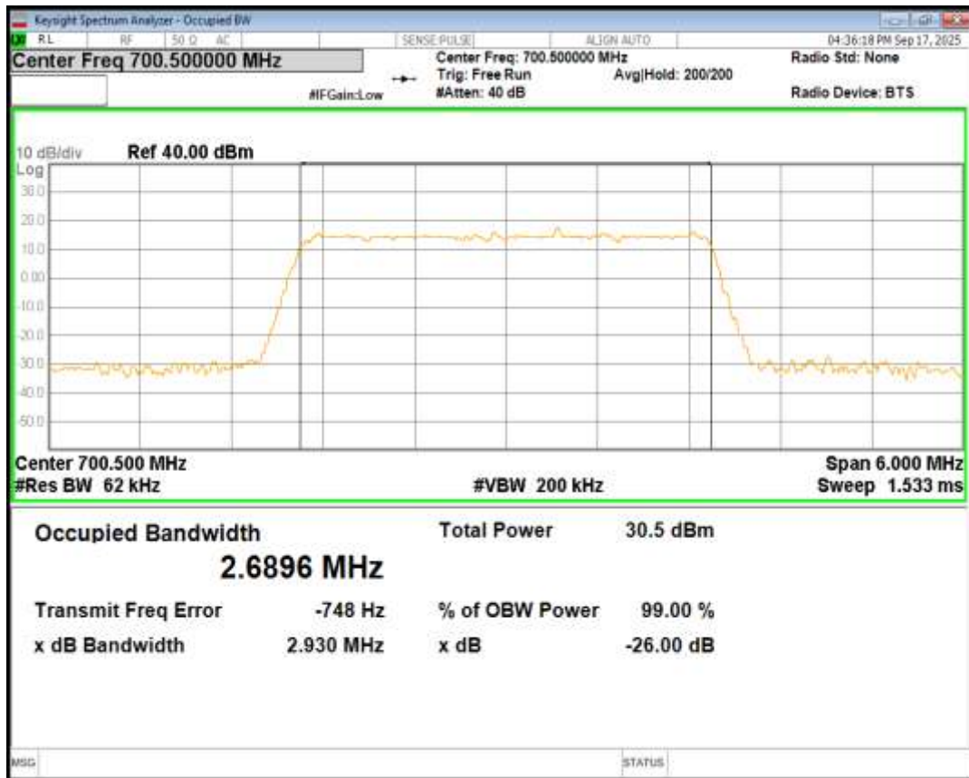
Band12 QPSK BW=3MHz Channel=23095 RB Size=15 Position=#0
