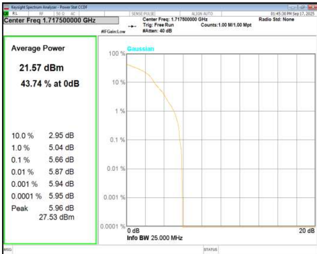
Band4 16QAM BW=15MHz Channel=20325 RB Size=1 Position=#0
