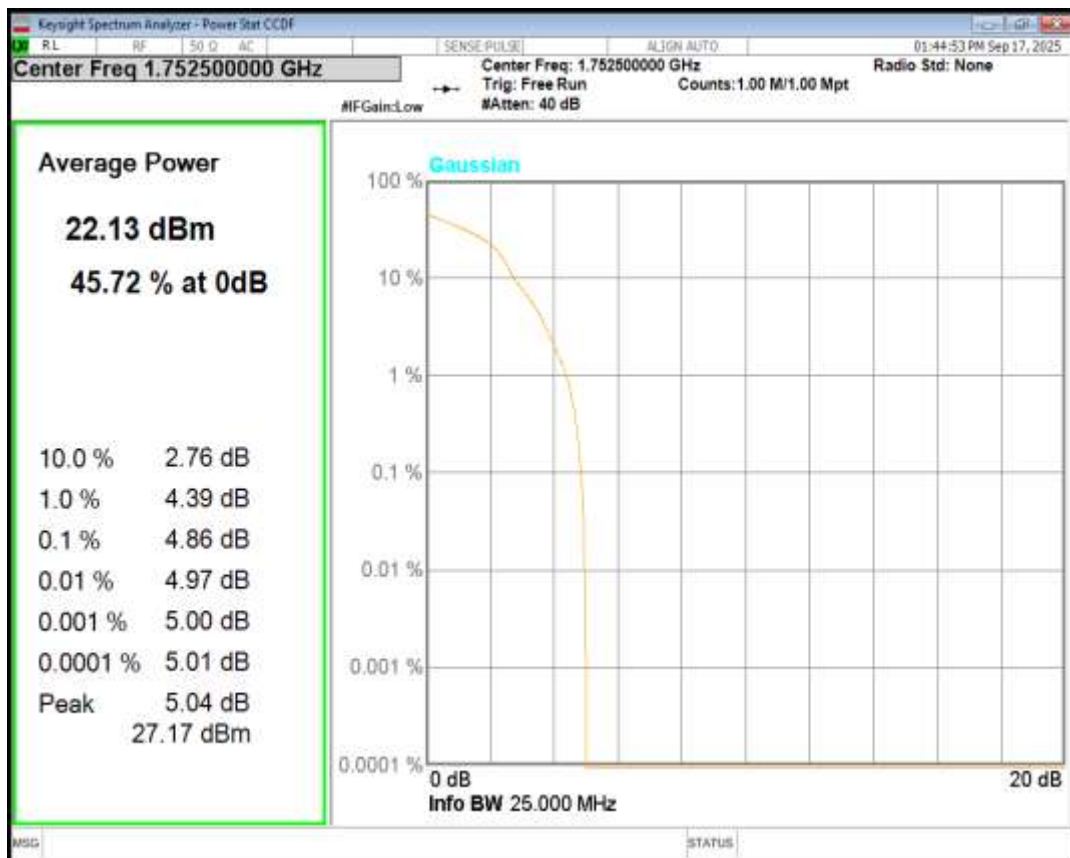
Band4 16QAM BW=5MHz Channel=20175 RB Size=1 Position=#0
