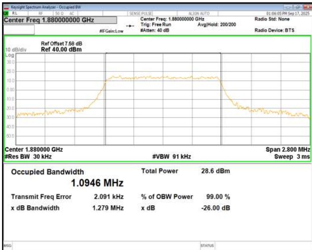
Band2 16QAM BW=1.4MHz Channel=19193 RB Size=6 Position=#0
