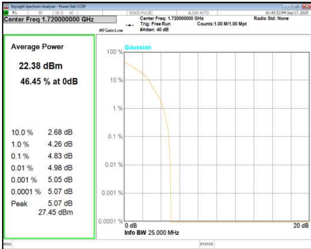
Band4 QPSK BW=15MHz Channel=20175 RB Size=1 Position=#0
