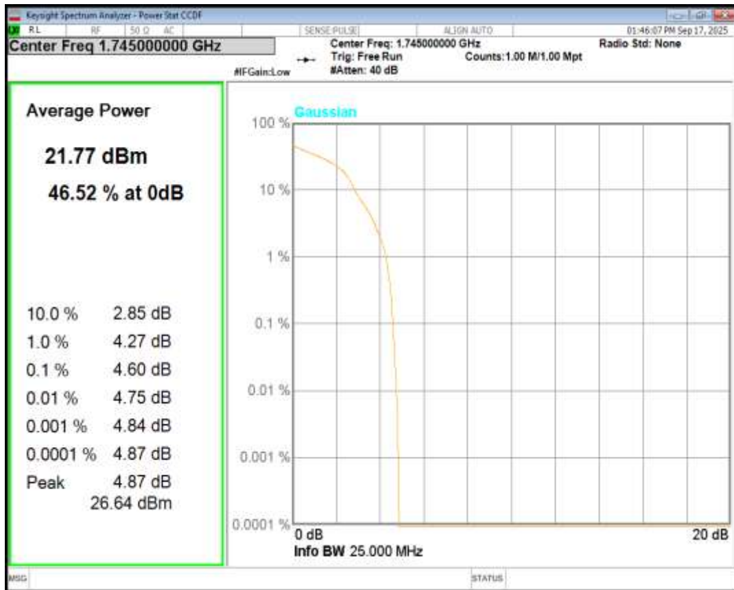
Band4 16QAM BW=3MHz Channel=19965 RB Size=1 Position=#0
