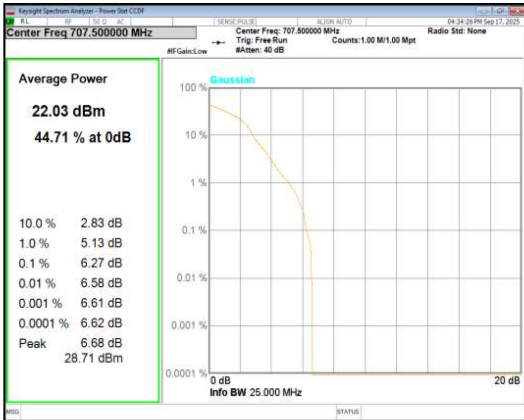
Band12 16QAM BW=1.4MHz Channel=23173 RB Size=1 Position=#0
