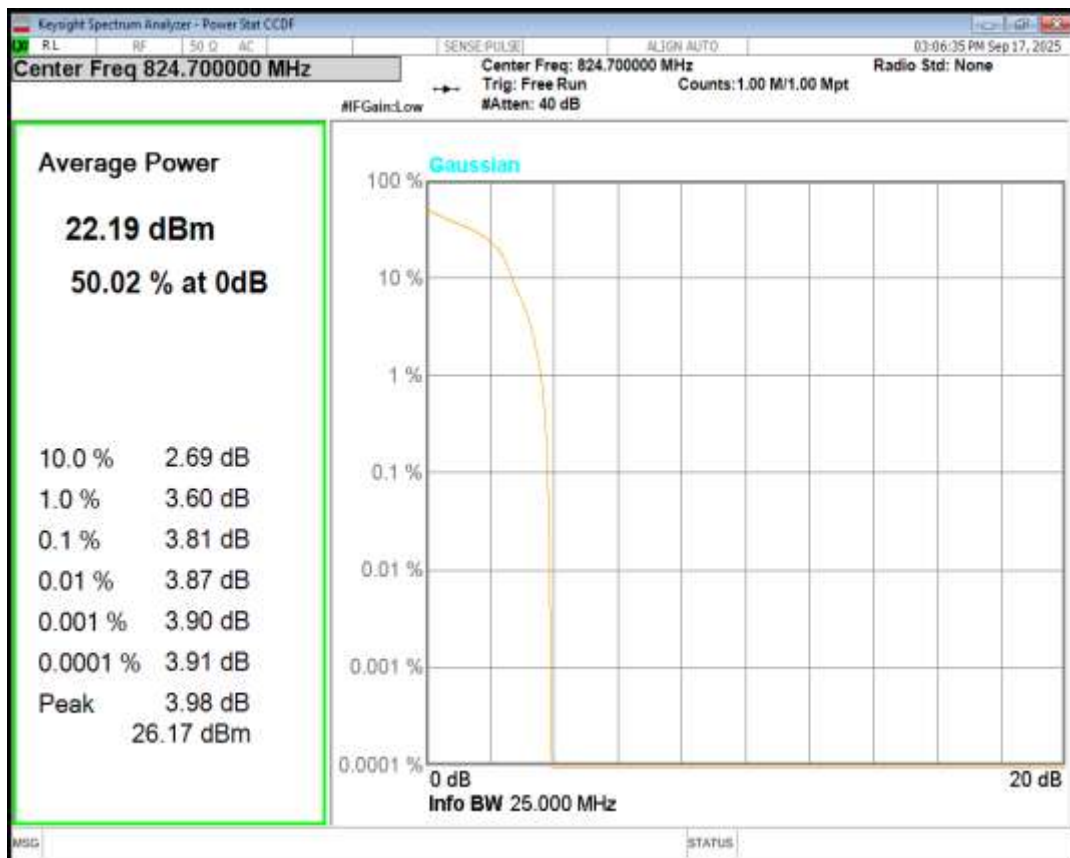
Band5 16QAM BW=1.4MHz Channel=20525 RB Size=1 Position=#0
