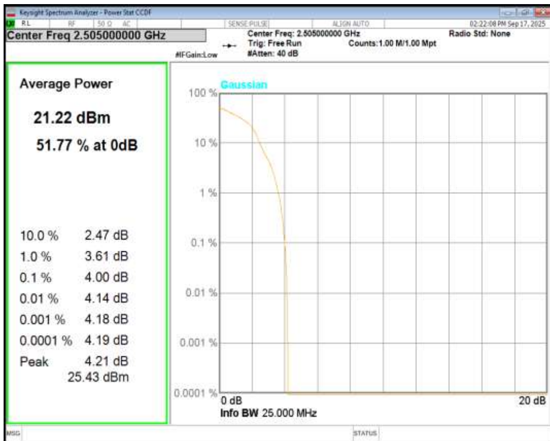
Band7 16QAM BW=10MHz Channel=21100 RB Size=1 Position=#0
