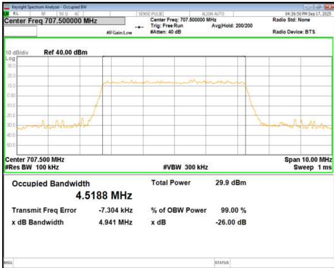
Band12 QPSK BW=5MHz Channel=23155 RB Size=25 Position=#0
