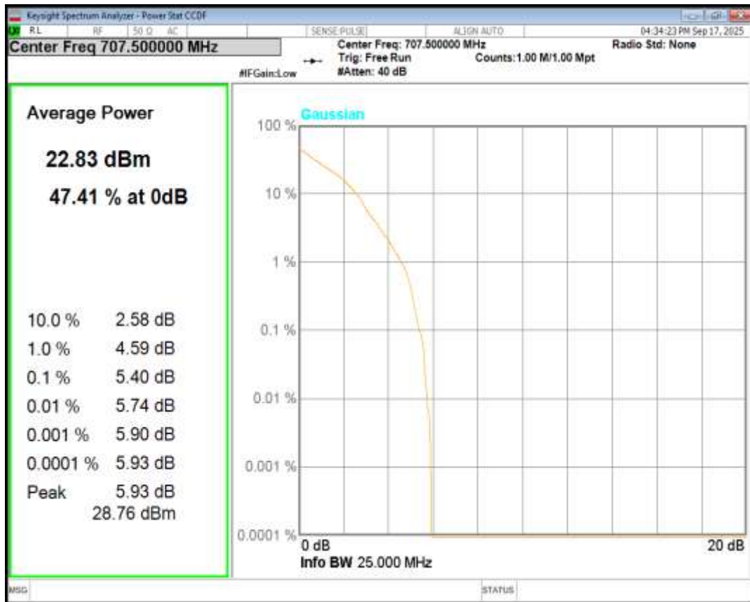
Band12 QPSK BW=1.4MHz Channel=23173 RB Size=1 Position=#0
