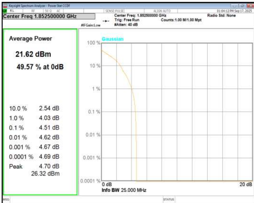
Band2 QPSK BW=5MHz Channel=18900 RB Size=1 Position=#0
