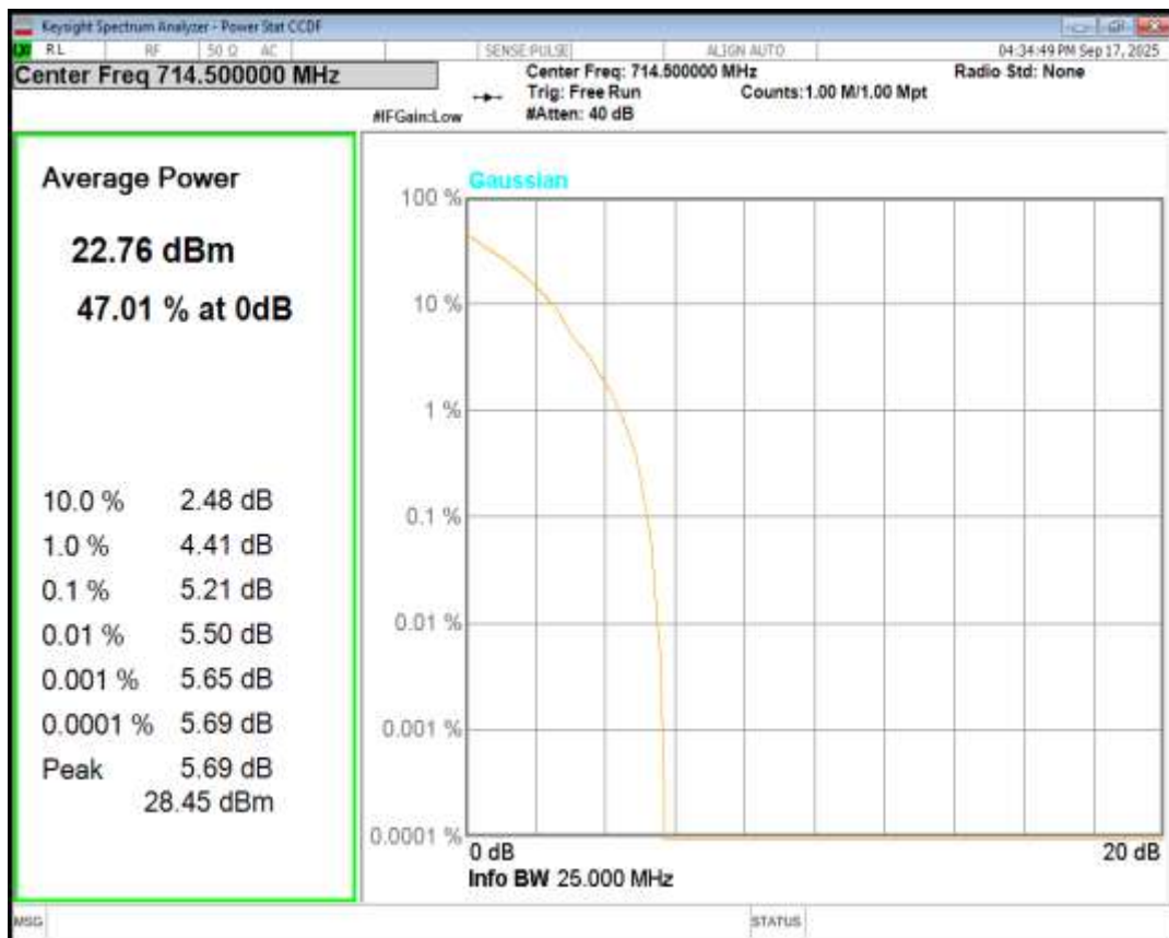
Band12 QPSK BW=5MHz Channel=23035 RB Size=1 Position=#0
