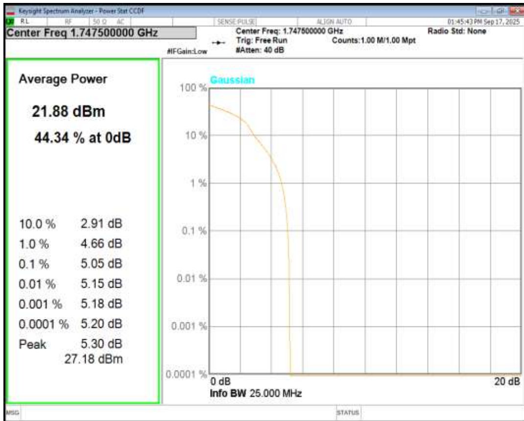
Band4 16QAM BW=15MHz Channel=20175 RB Size=1 Position=#0
