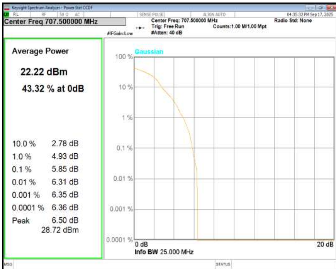
Band12 16QAM BW=10MHz Channel=23130 RB Size=1 Position=#0
