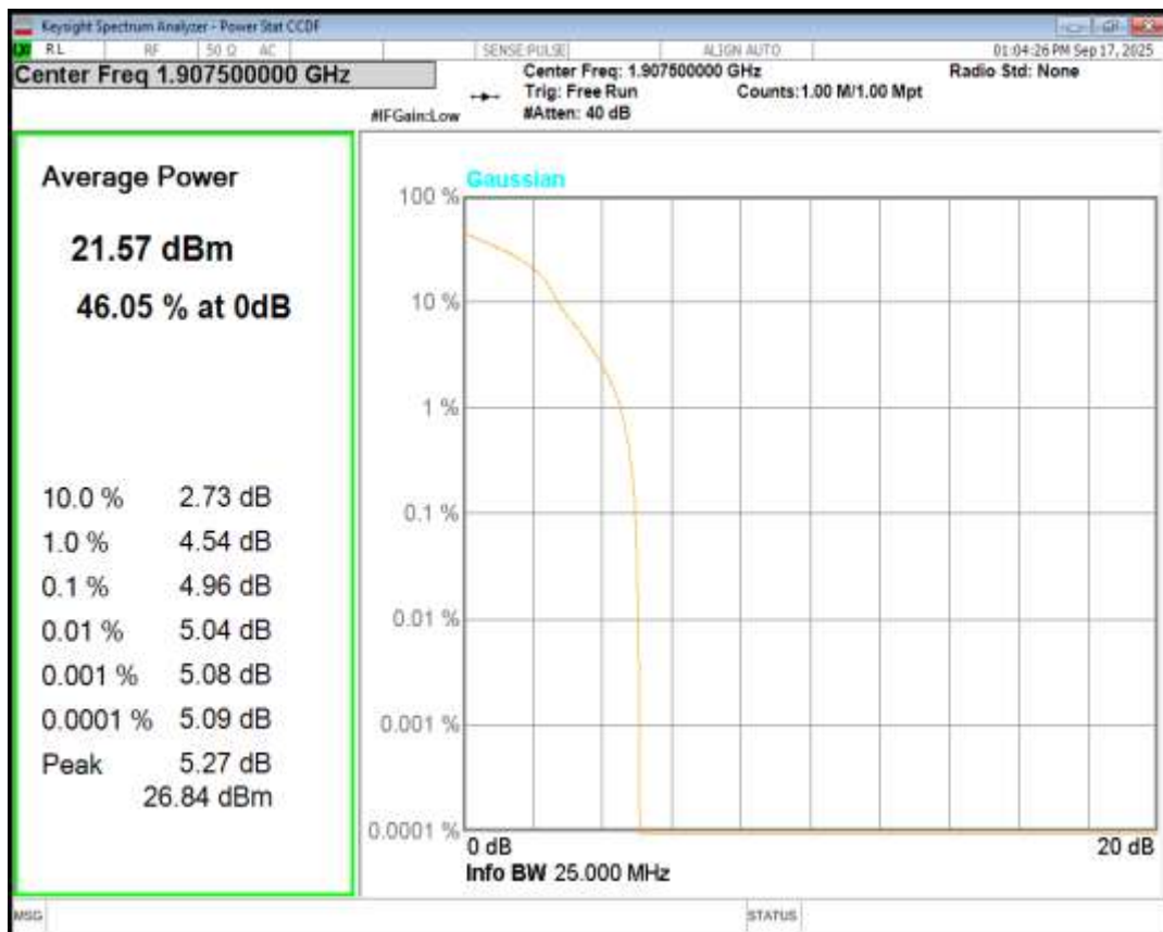
Band2 16QAM BW=5MHz Channel=18900 RB Size=1 Position=#0
