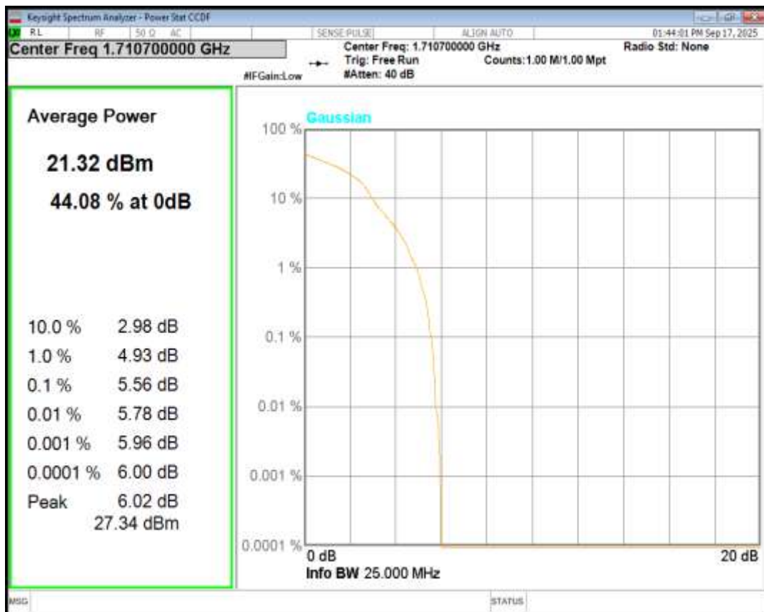
Band4 16QAM BW=1.4MHz Channel=20175 RB Size=1 Position=#0
