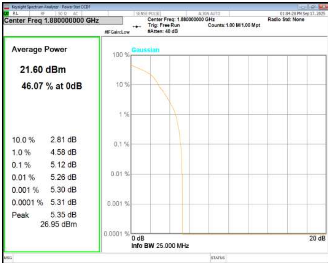
Band2 QPSK BW=1.4MHz Channel=18607 RB Size=1 Position=#0
