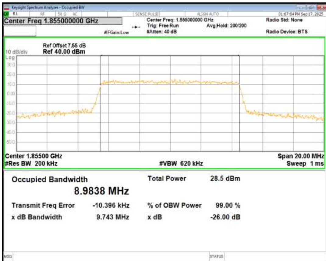
Band2 16QAM BW=10MHz Channel=18900 RB Size=50 Position=#0
