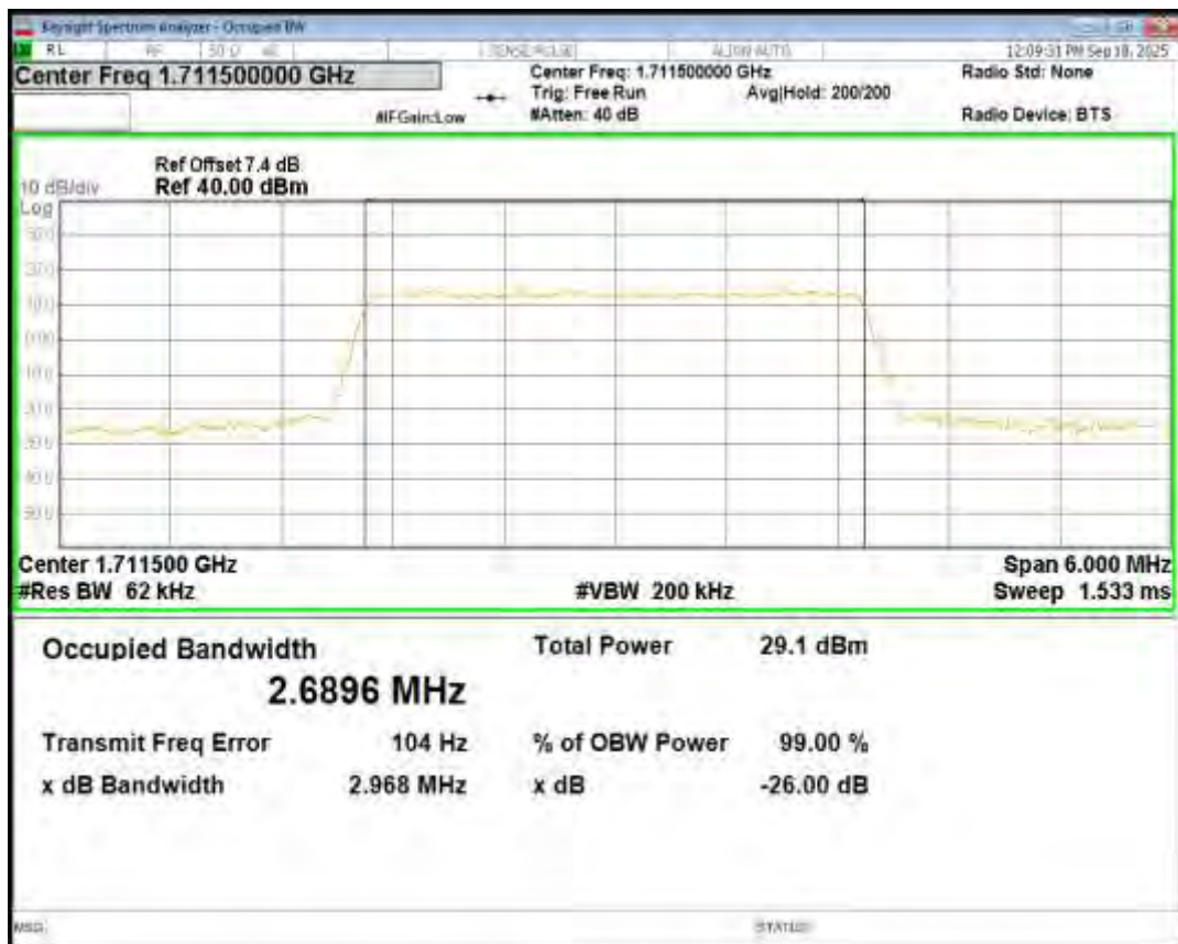
Band4 16QAM BW=3MHz Channel=20175 RB Size=15 Position=#0
