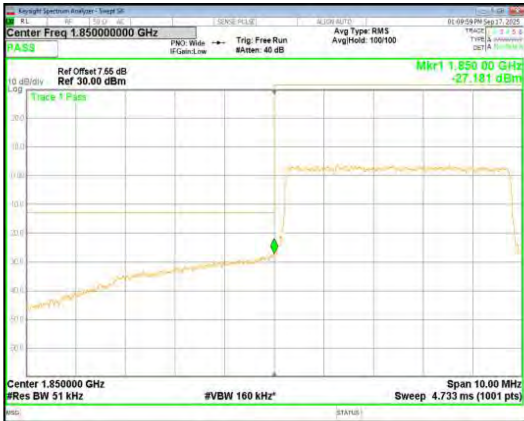
Band2 QPSK BW=5MHz Channel=19175 RB Size=25 Position=#0
