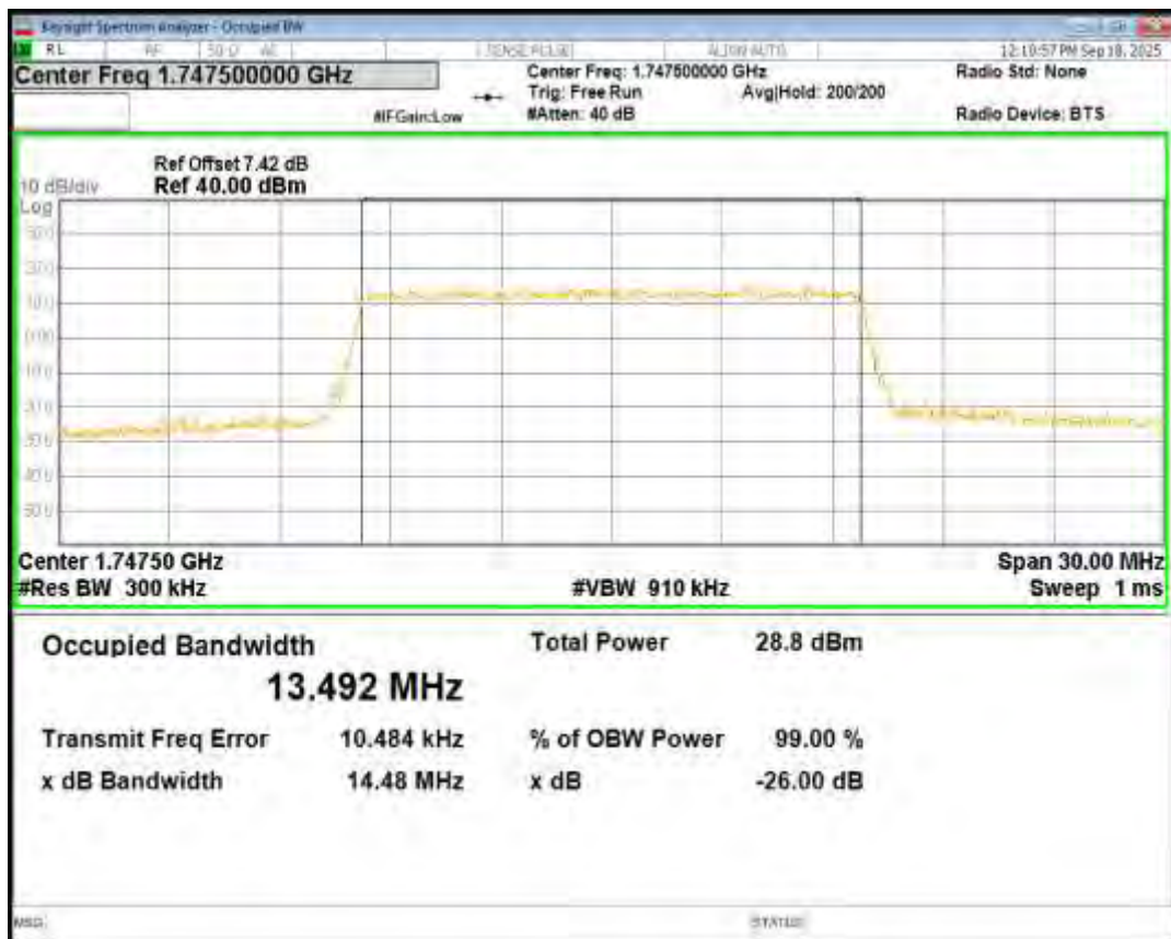
Band4 16QAM BW=20MHz Channel=20050 RB Size=100 Position=#0
