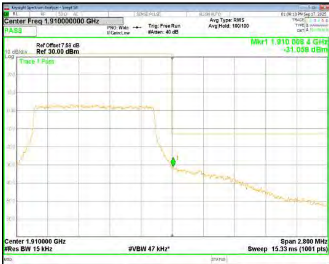
Band2 16QAM BW=10MHz Channel=18650 RB Size=50 Position=#0
