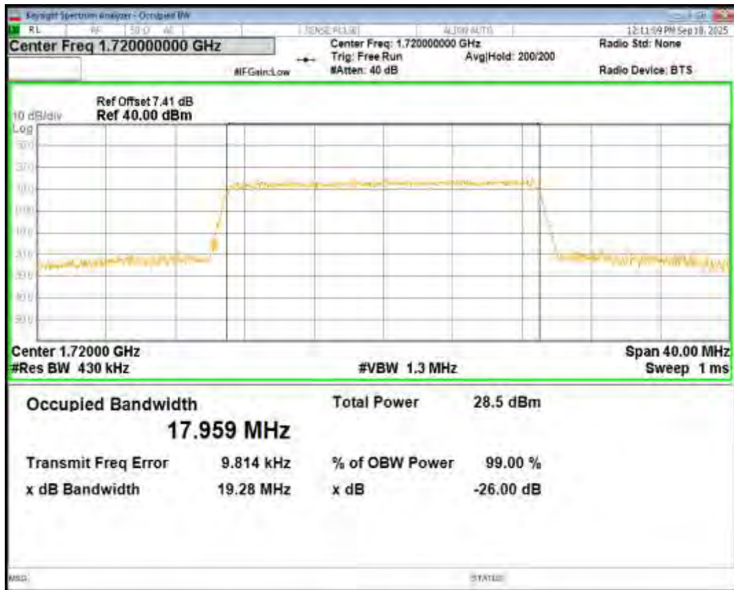
Band4 16QAM BW=20MHz Channel=20175 RB Size=100 Position=#0
