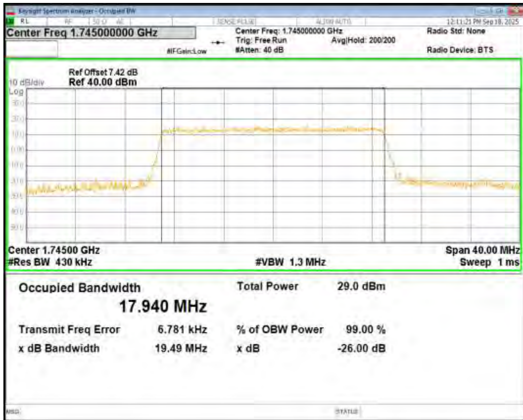
Band4 16QAM BW=3MHz Channel=19965 RB Size=15 Position=#0
