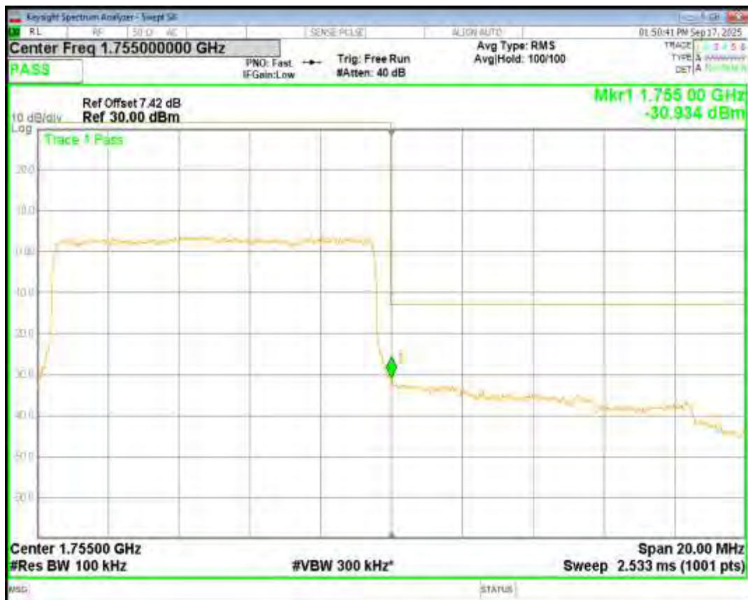
Band4 QPSK BW=15MHz Channel=20025 RB Size=75 Position=#0
