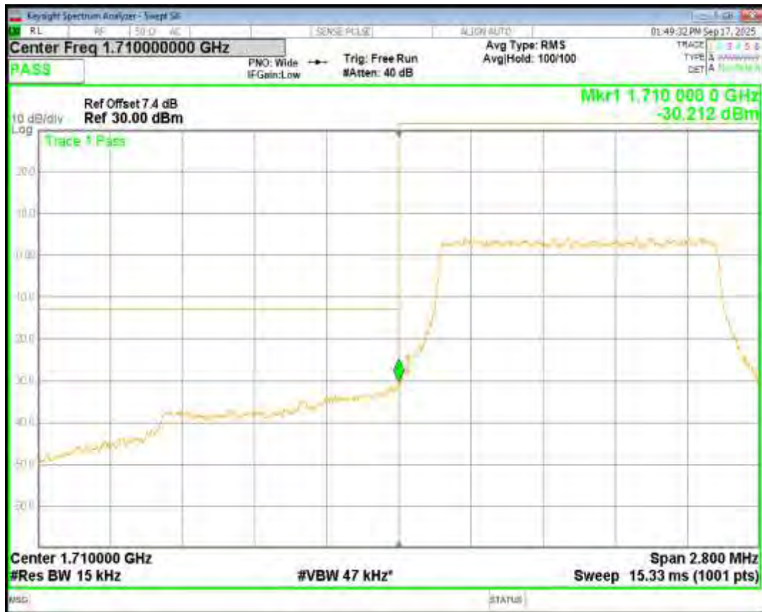
Band4 QPSK BW=1.4MHz Channel=20393 RB Size=6 Position=#0
