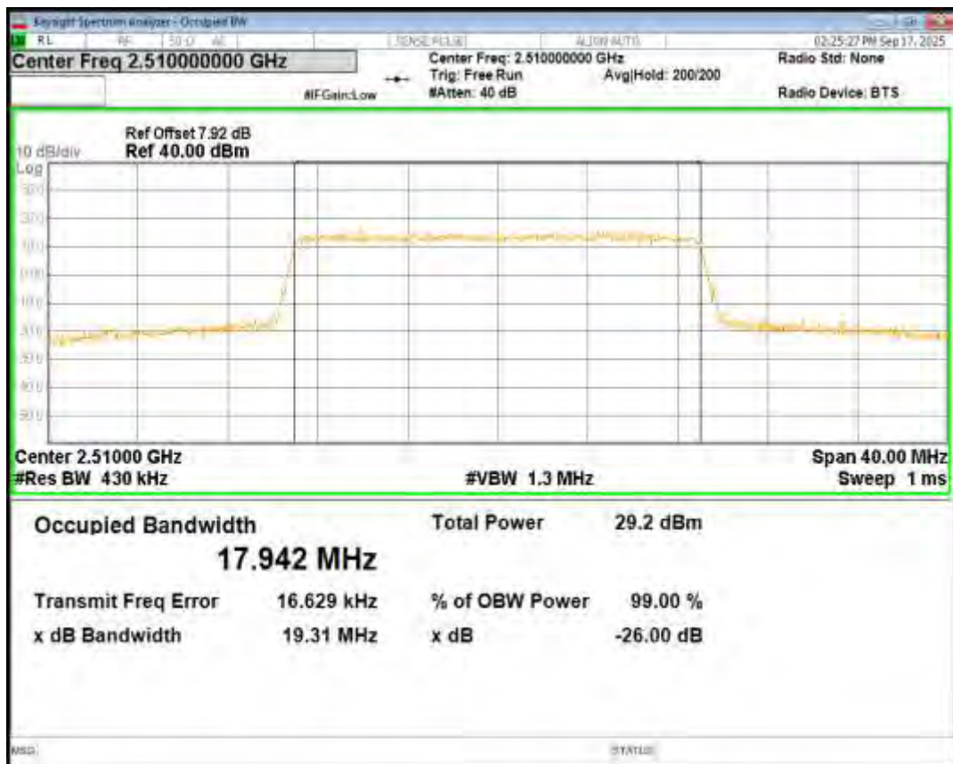
Band7 QPSK BW=20MHz Channel=21100 RB Size=100 Position=#0
