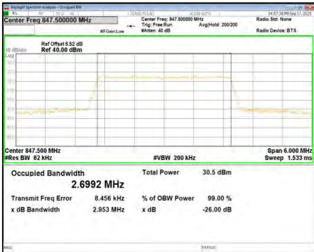
Band5 QPSK BW=5MHz Channel=20425 RB Size=25 Position=#0
