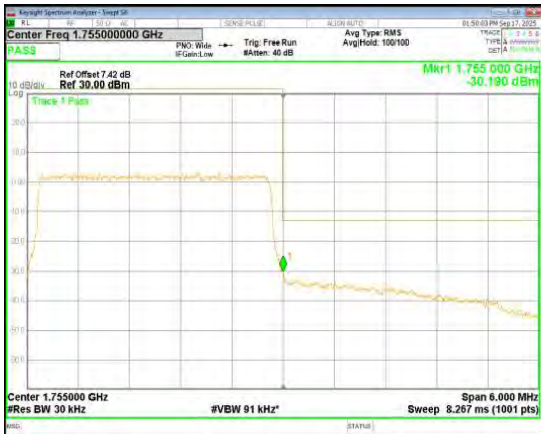
Band4 16QAM BW=5MHz Channel=20375 RB Size=25 Position=#0
