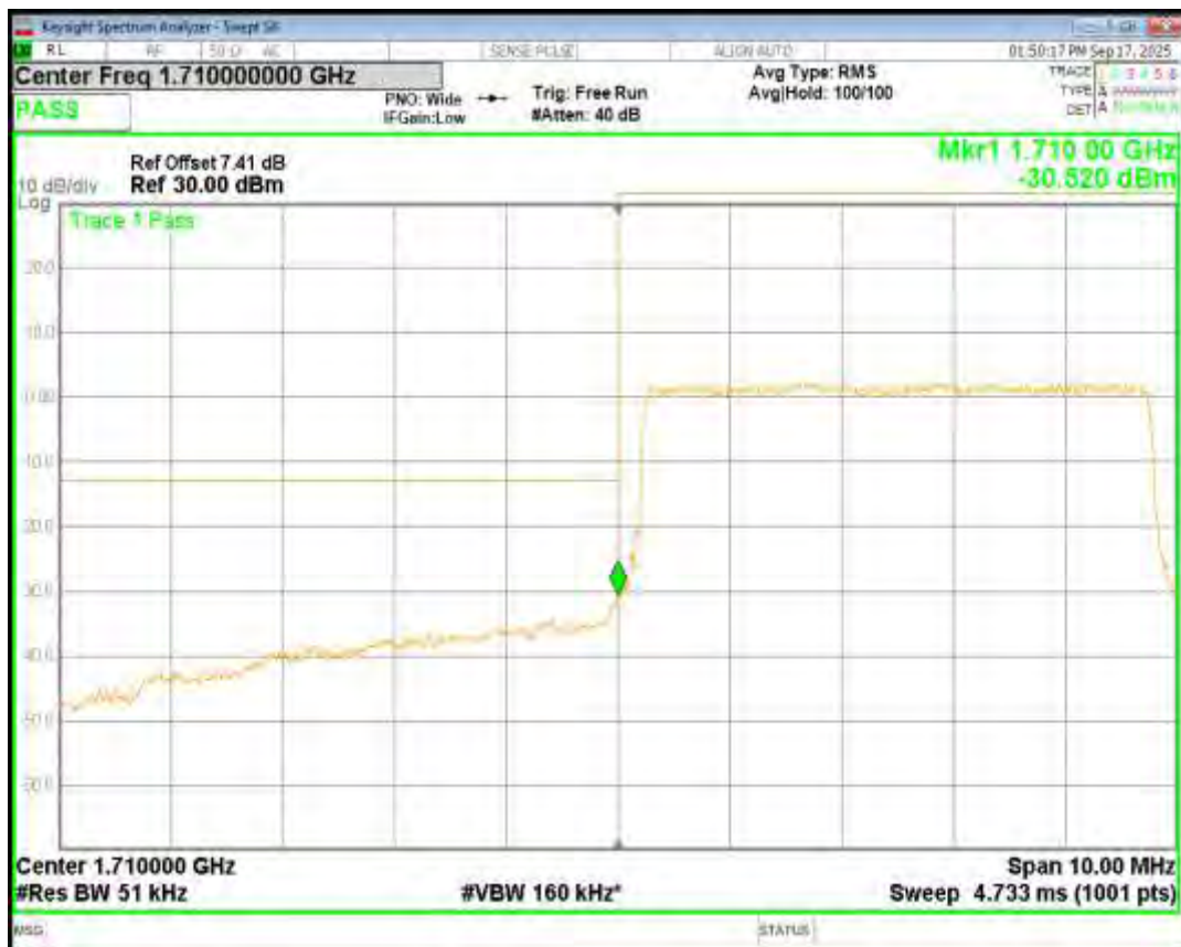
Band4 QPSK BW=1.4MHz Channel=19957 RB Size=6 Position=#0
