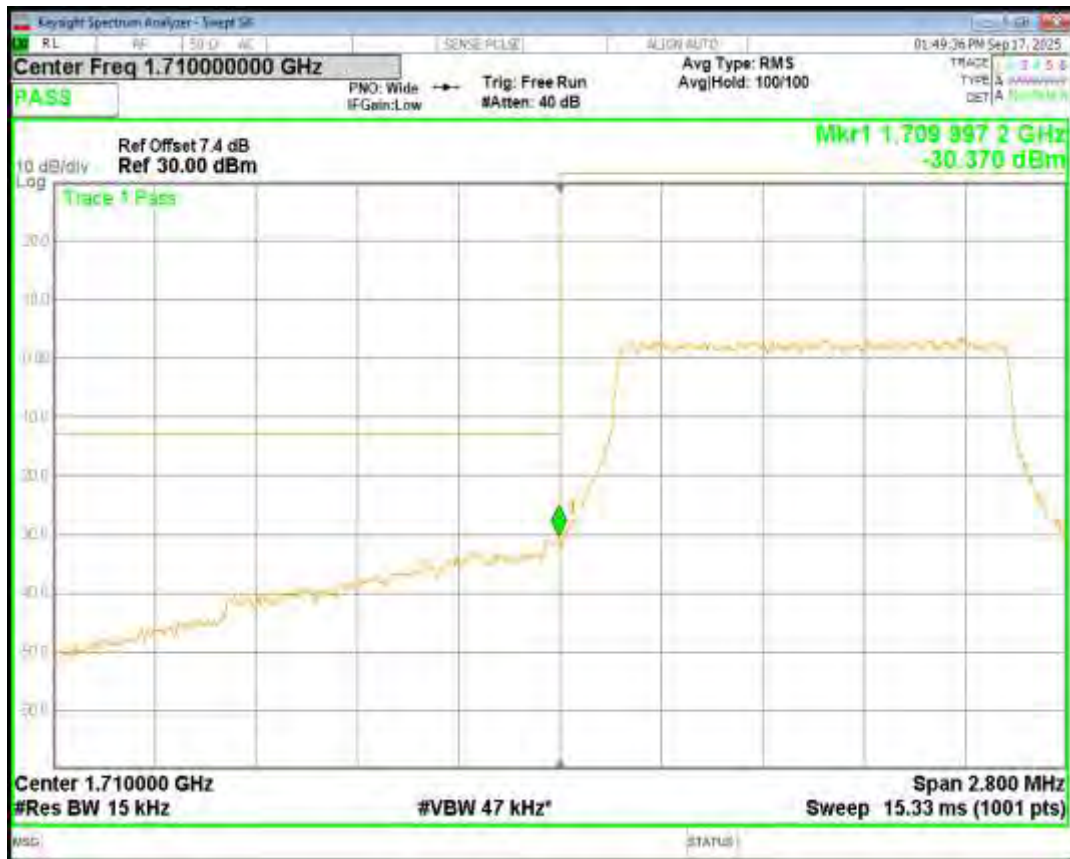
Band4 16QAM BW=1.4MHz Channel=20393 RB Size=6 Position=#0
