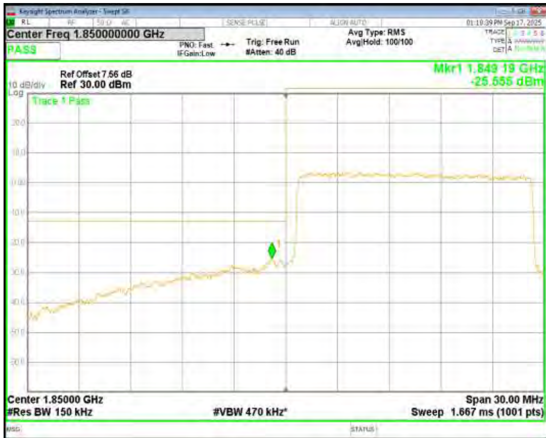
Band2 QPSK BW=15MHz Channel=19125 RB Size=75 Position=#0
