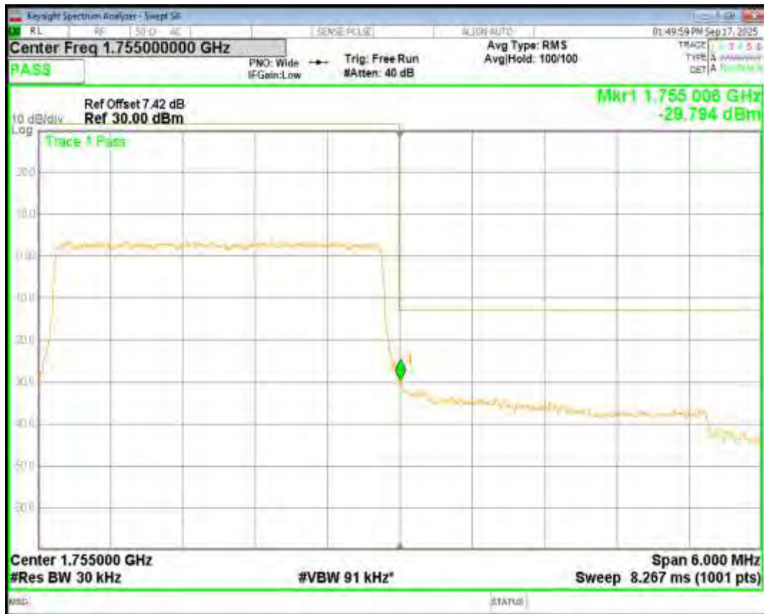
Band4 QPSK BW=5MHz Channel=20375 RB Size=25 Position=#0
