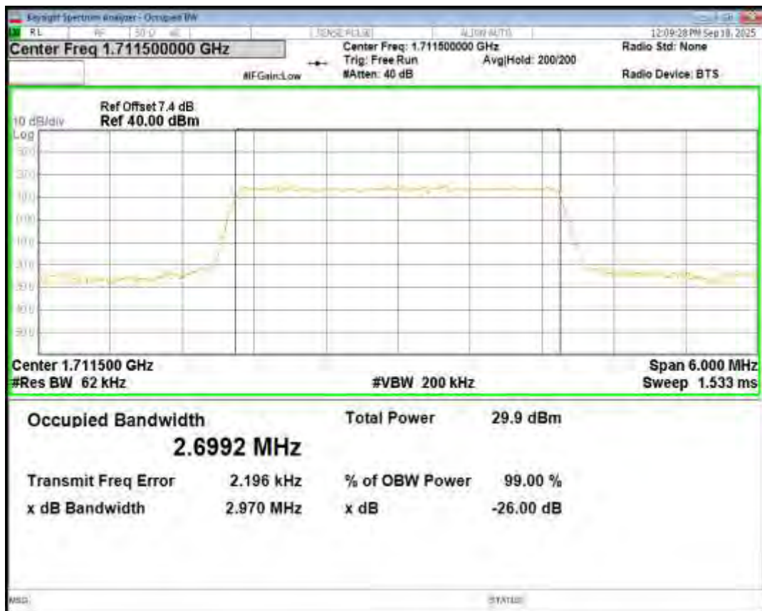
Band4 QPSK BW=3MHz Channel=20175 RB Size=15 Position=#0
