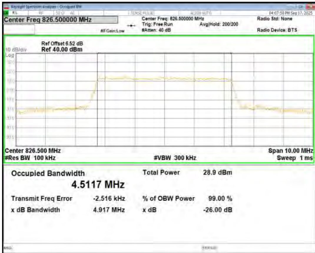
Band5 QPSK BW=1.4MHz Channel=20525 RB Size=6 Position=#0
