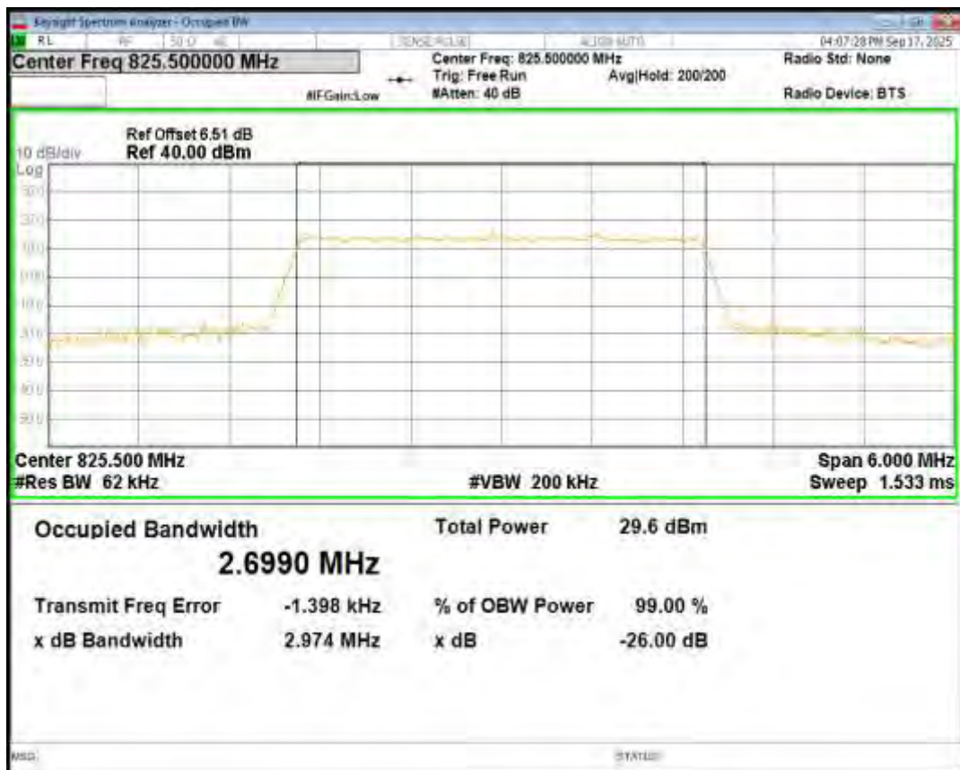
Band5 16QAM BW=3MHz Channel=20525 RB Size=15 Position=#0
