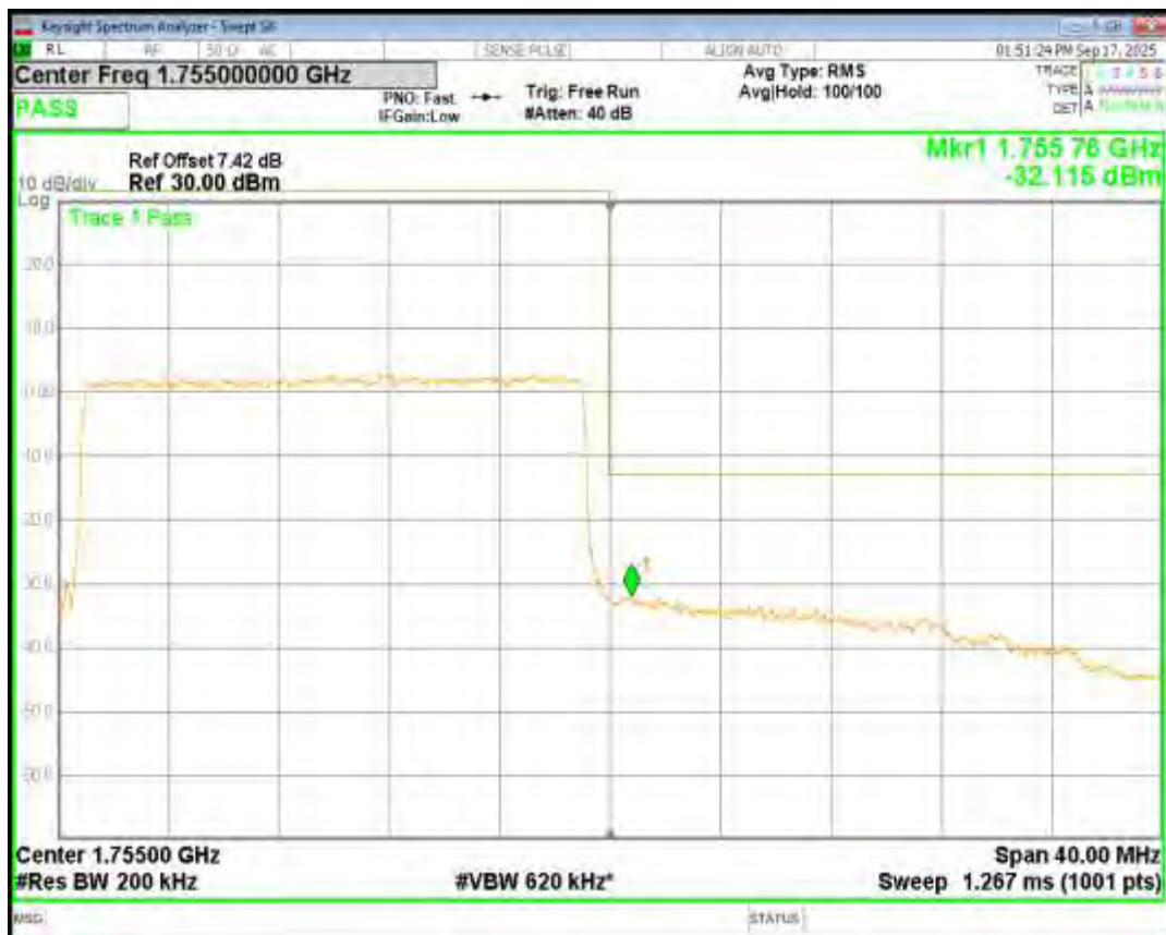
Band4 16QAM BW=3MHz Channel=19965 RB Size=15 Position=#0
