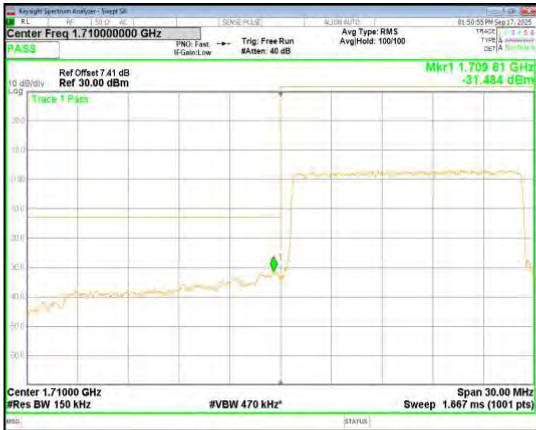
Band4 QPSK BW=15MHz Channel=20325 RB Size=75 Position=#0
