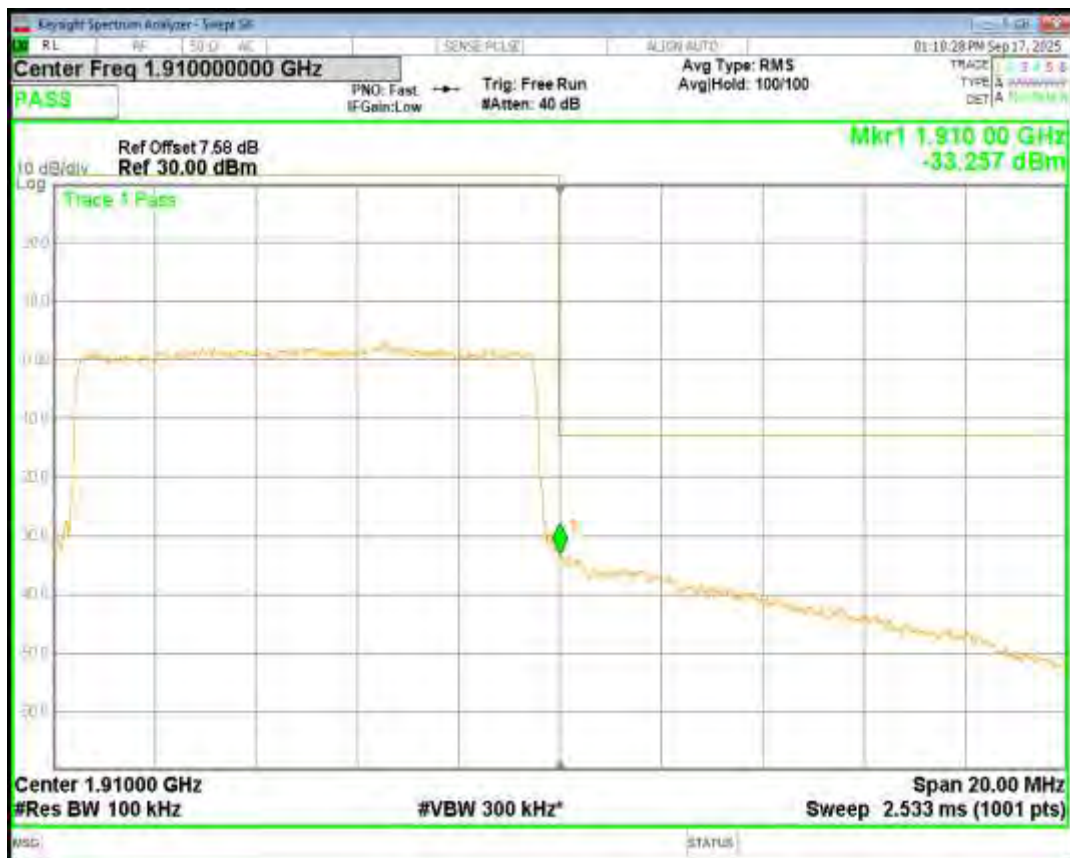
Band2 16QAM BW=15MHz Channel=18675 RB Size=75 Position=#0
