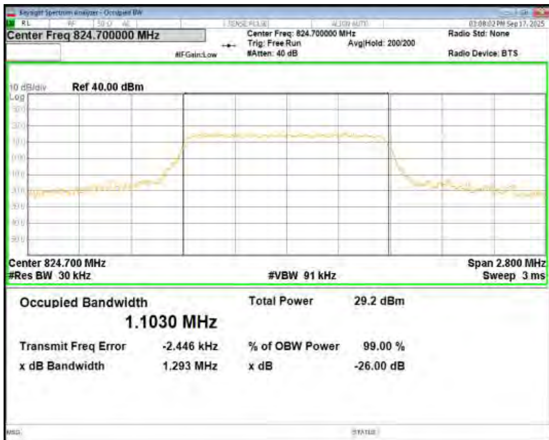
Band5 16QAM BW=1.4MHz Channel=20525 RB Size=6 Position=#0
