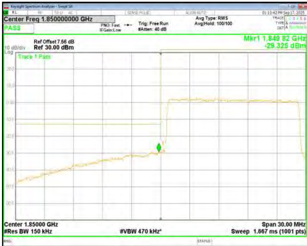
Band2 16QAM BW=15MHz Channel=19125 RB Size=75 Position=#0
