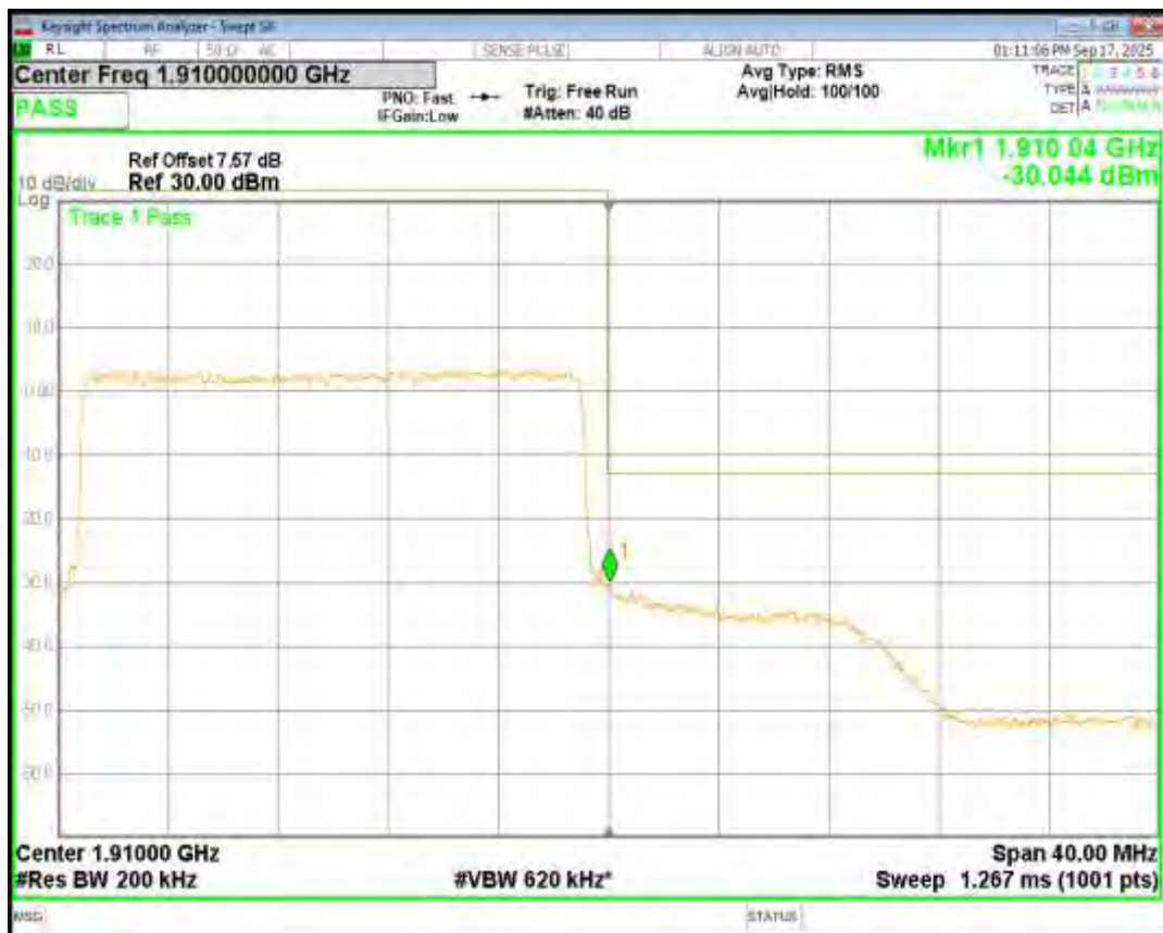
Band2 QPSK BW=3MHz Channel=18615 RB Size=15 Position=#0
