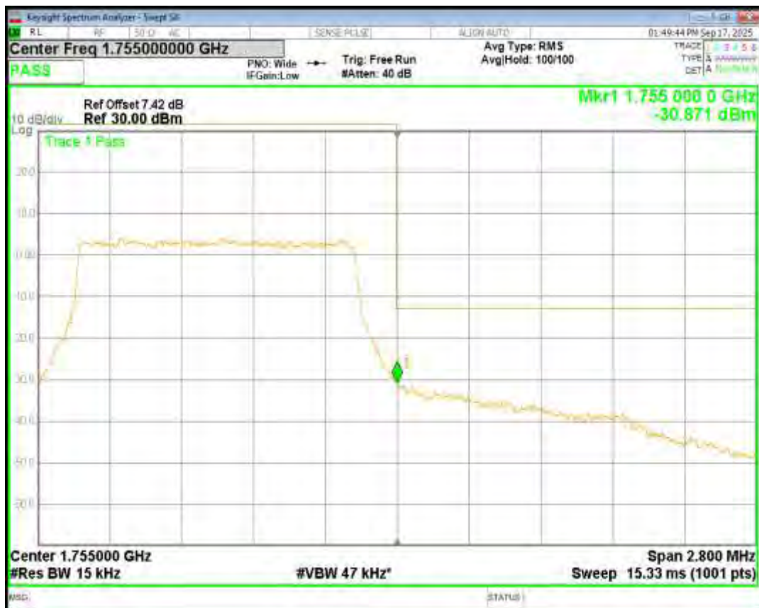
Band4 16QAM BW=10MHz Channel=20000 RB Size=50 Position=#0
