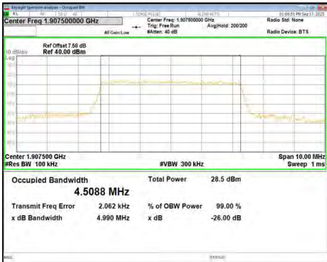
Band2 QPSK BW=10MHz Channel=18650 RB Size=50 Position=#0
