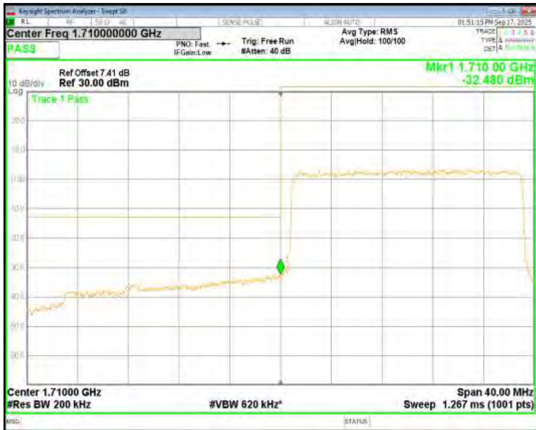
Band4 QPSK BW=20MHz Channel=20300 RB Size=100 Position=#0
