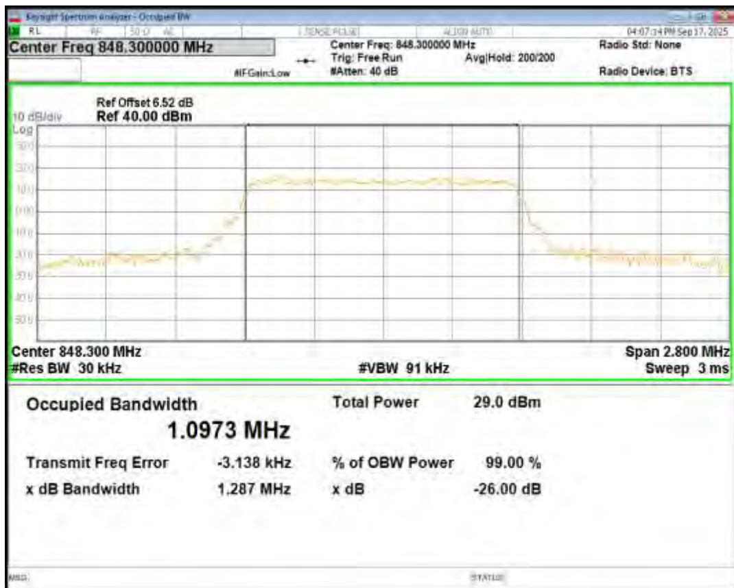
Band5 16QAM BW=10MHz Channel=20450 RB Size=50 Position=#0
