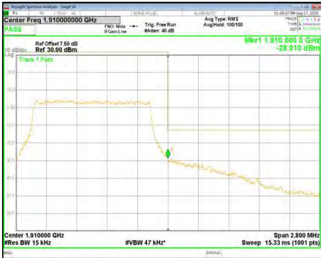
Band2 16QAM BW=5MHz Channel=19175 RB Size=25 Position=#0
