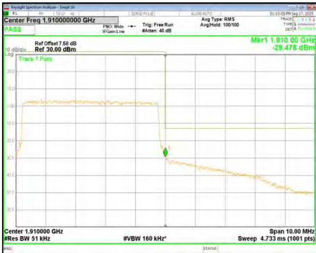
Band4 16QAM BW=1.4MHz Channel=19957 RB Size=6 Position=#0
