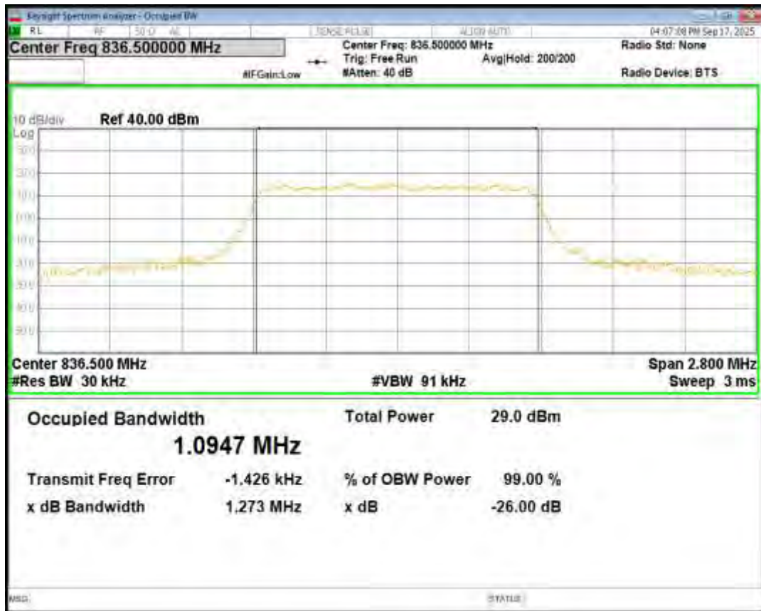
Band5 16QAM BW=1.4MHz Channel=20643 RB Size=6 Position=#0
