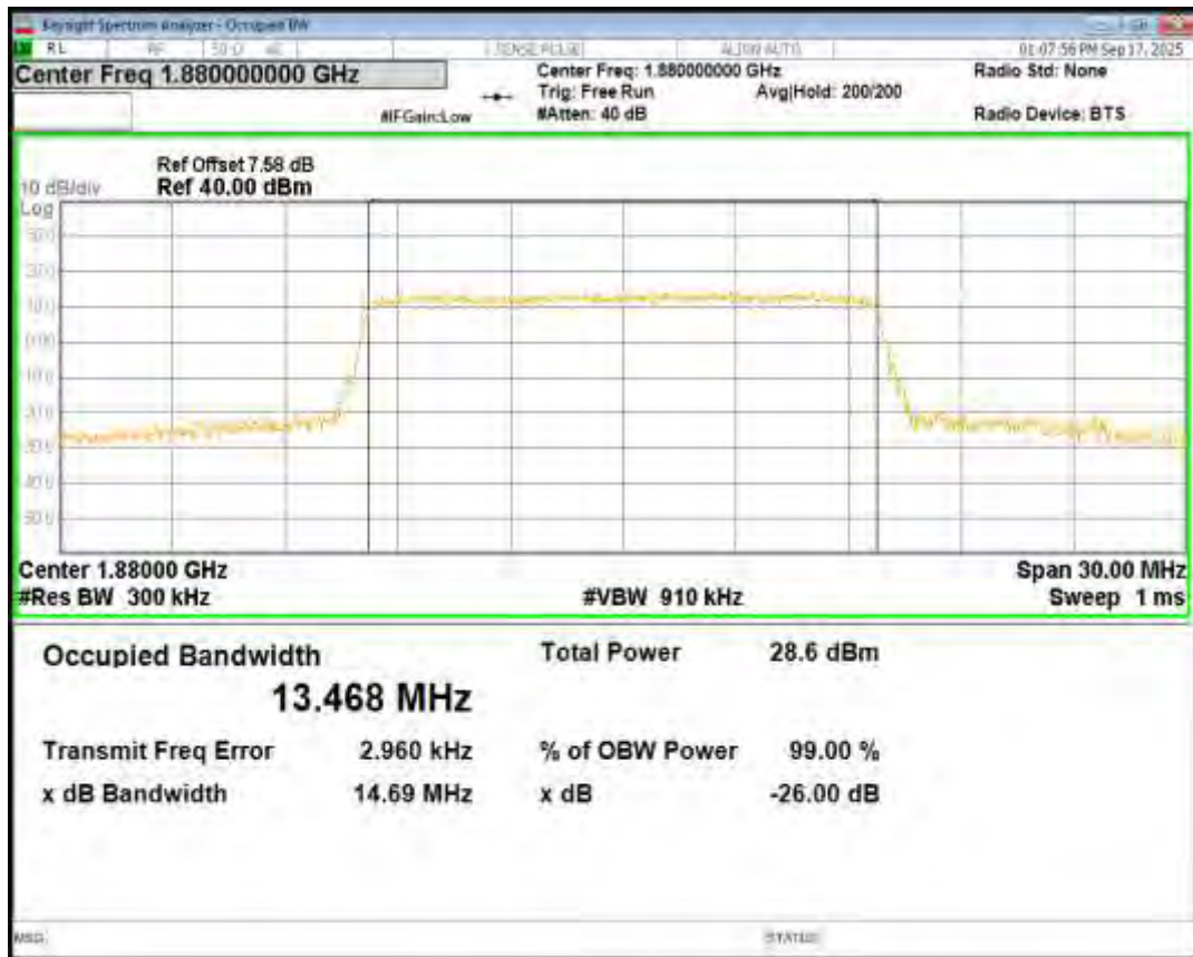
Band2 16QAM BW=20MHz Channel=18900 RB Size=100 Position=#0
