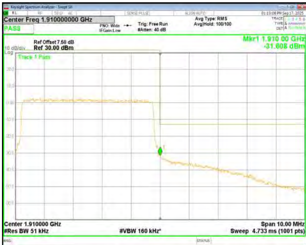
Band2 QPSK BW=1.4MHz Channel=18607 RB Size=6 Position=#0
