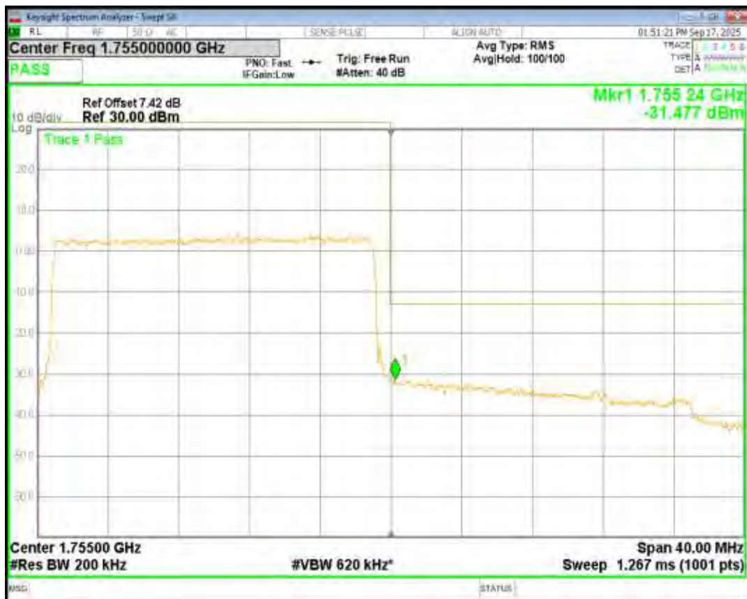
Band4 QPSK BW=3MHz Channel=19965 RB Size=15 Position=#0
