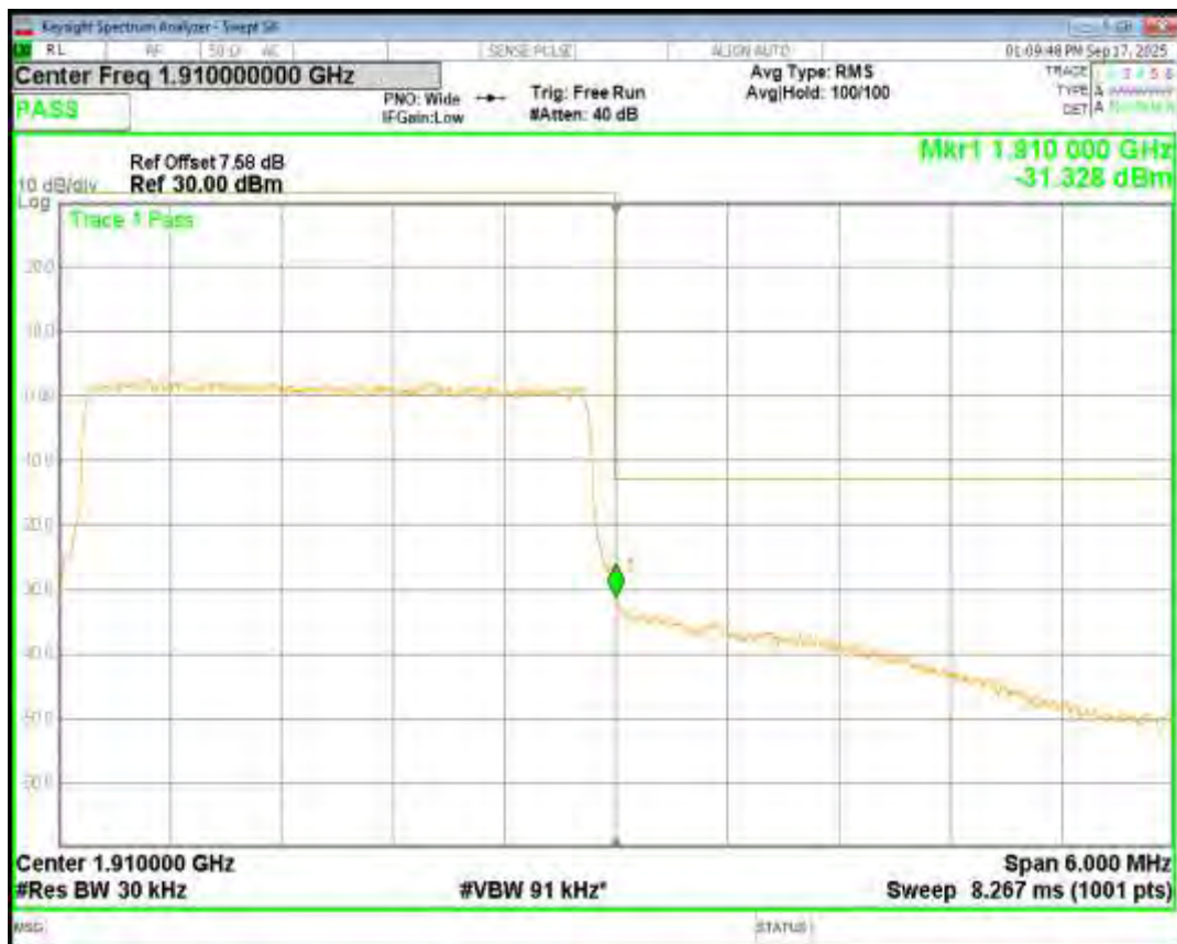
Band2 16QAM BW=5MHz Channel=18625 RB Size=25 Position=#0
