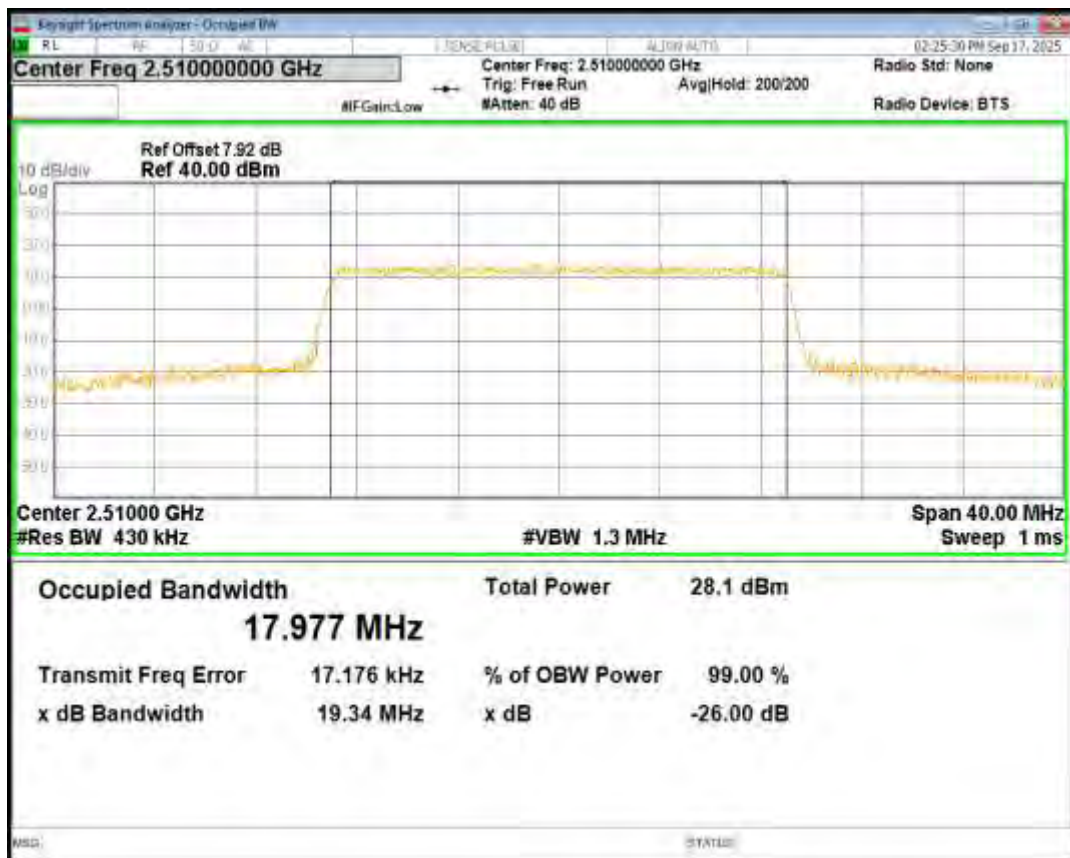
Band7 16QAM BW=20MHz Channel=21100 RB Size=100 Position=#0
