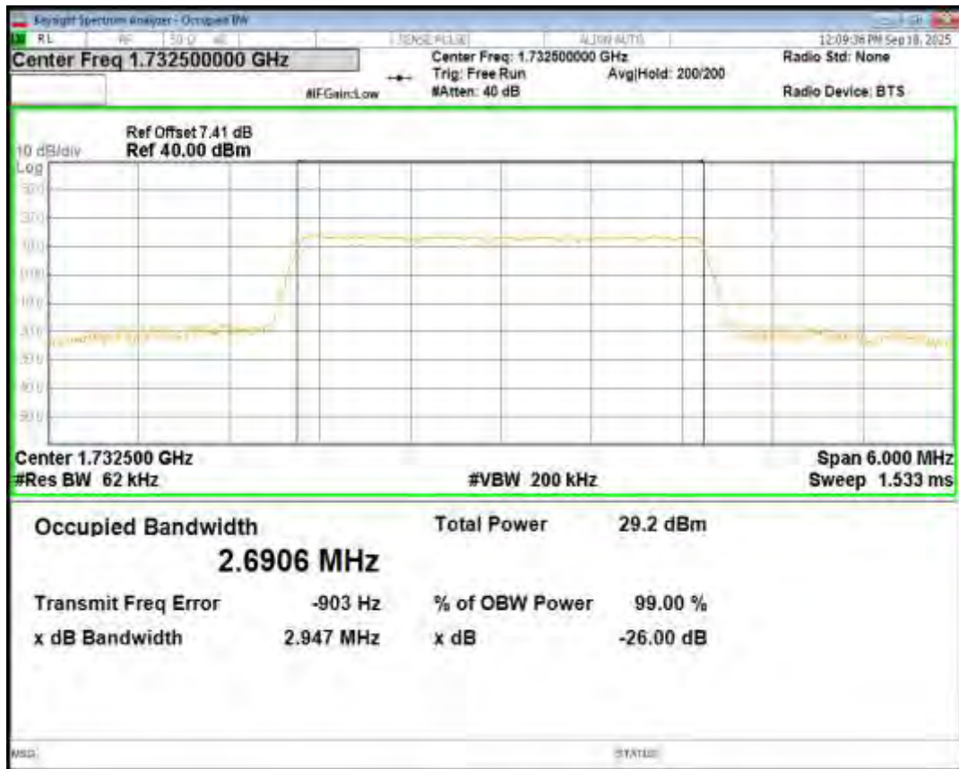
Band4 16QAM BW=3MHz Channel=20385 RB Size=15 Position=#0
