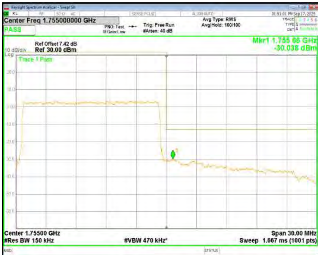
Band4 QPSK BW=20MHz Channel=20050 RB Size=100 Position=#0
