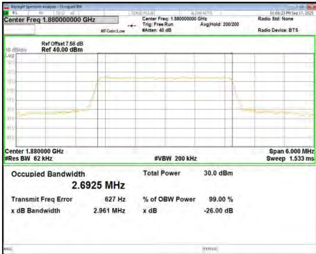
Band2 QPSK BW=3MHz Channel=19185 RB Size=15 Position=#0
