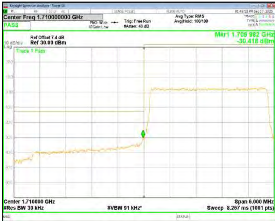
Band4 QPSK BW=5MHz Channel=19975 RB Size=25 Position=#0
