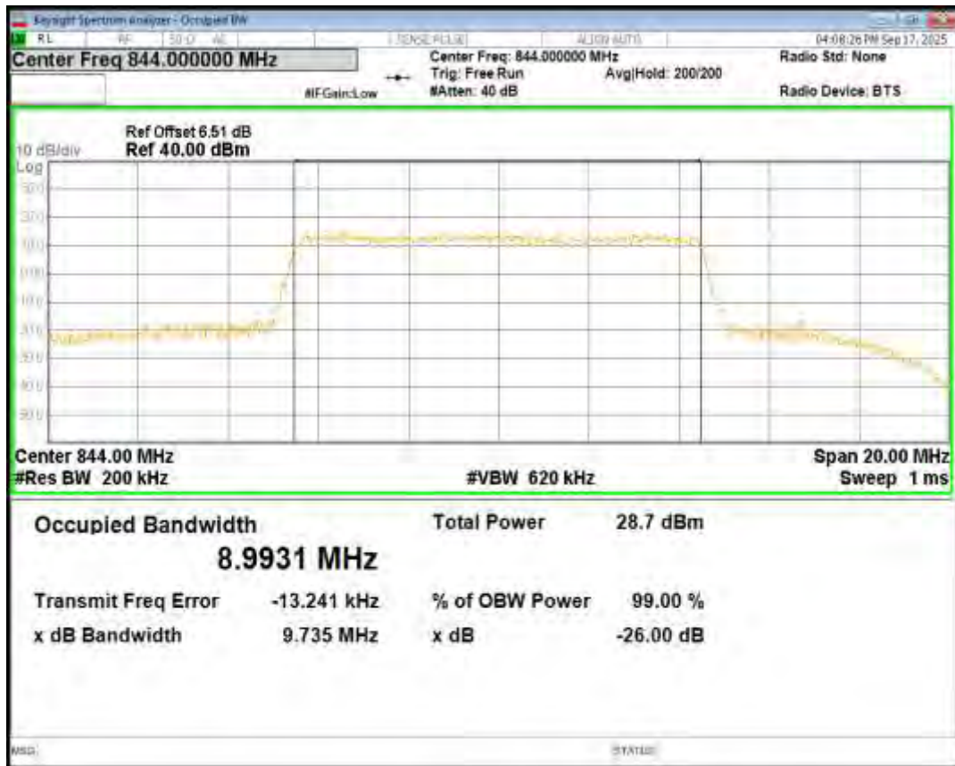
Band5 16QAM BW=3MHz Channel=20415 RB Size=15 Position=#0
