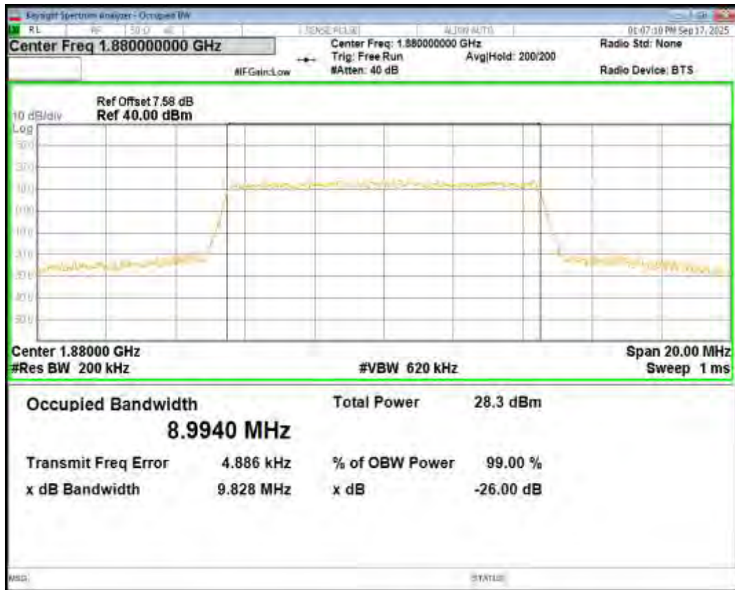
Band2 16QAM BW=10MHz Channel=19150 RB Size=50 Position=#0
