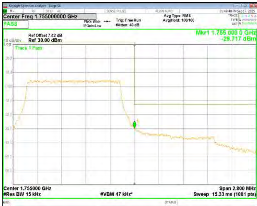
Band4 QPSK BW=10MHz Channel=20000 RB Size=50 Position=#0
