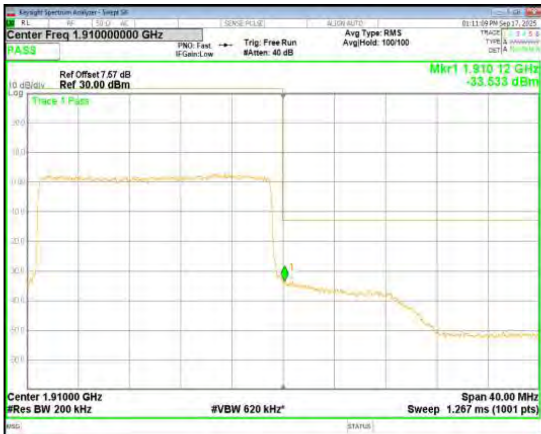
Band2 16QAM BW=3MHz Channel=18615 RB Size=15 Position=#0
