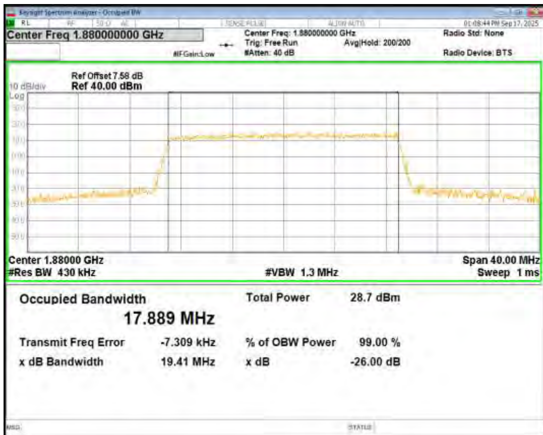
Band2 16QAM BW=3MHz Channel=18900 RB Size=15 Position=#0
