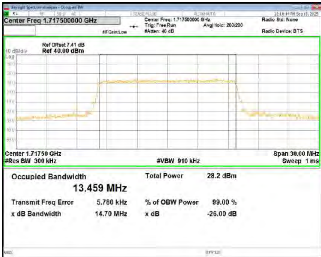
Band4 16QAM BW=15MHz Channel=20175 RB Size=75 Position=#0
