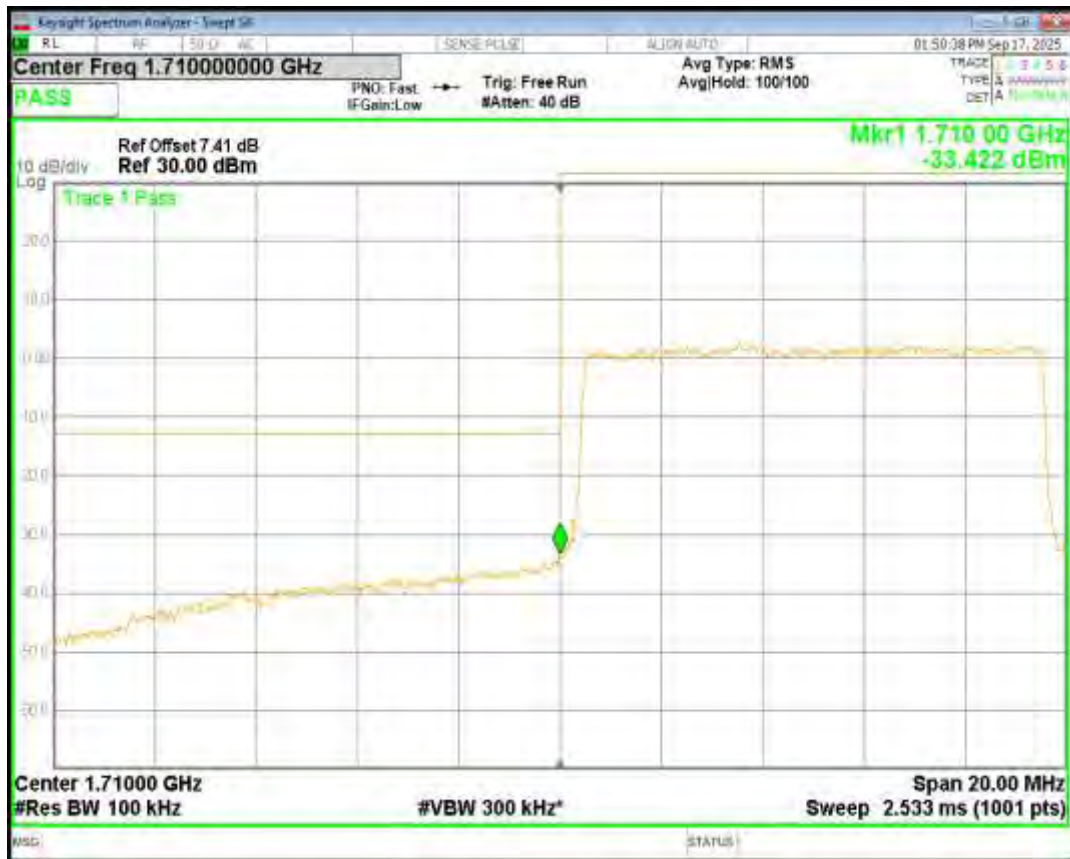
Band4 16QAM BW=10MHz Channel=20350 RB Size=50 Position=#0
