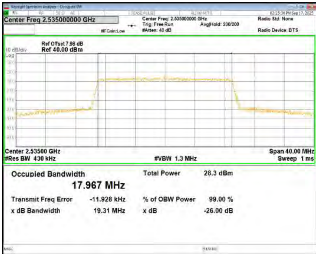
Band7 16QAM BW=20MHz Channel=21350 RB Size=100 Position=#0
