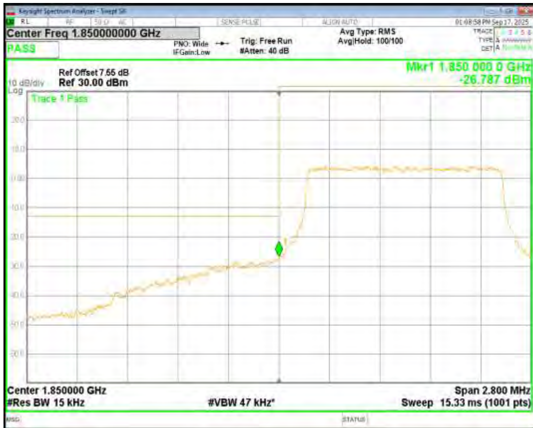
Band2 QPSK BW=10MHz Channel=19150 RB Size=50 Position=#0
