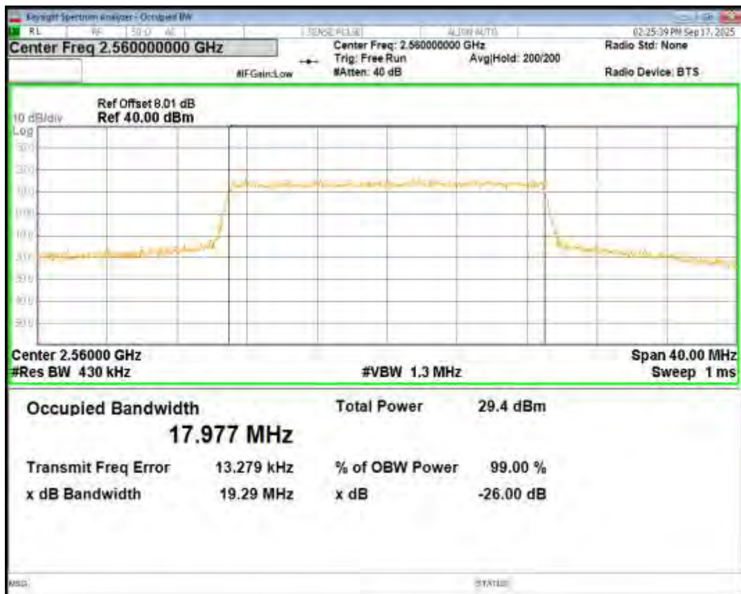
Band7 QPSK BW=5MHz Channel=20775 RB Size=25 Position=#0
