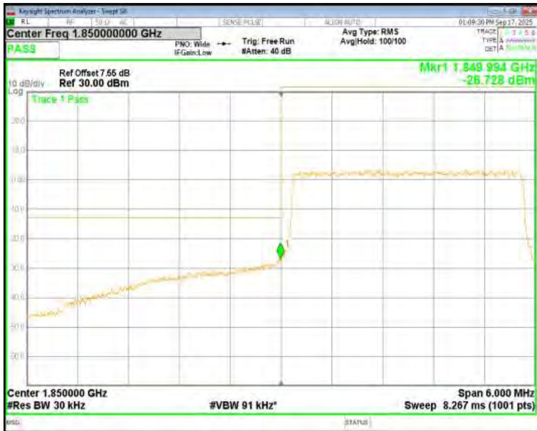
Band2 QPSK BW=3MHz Channel=19185 RB Size=15 Position=#0
