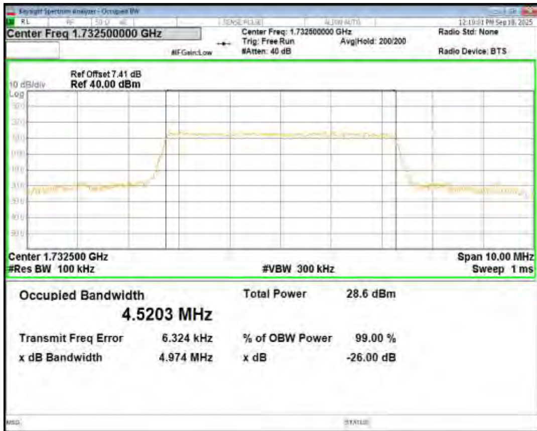
Band4 16QAM BW=5MHz Channel=20375 RB Size=25 Position=#0
