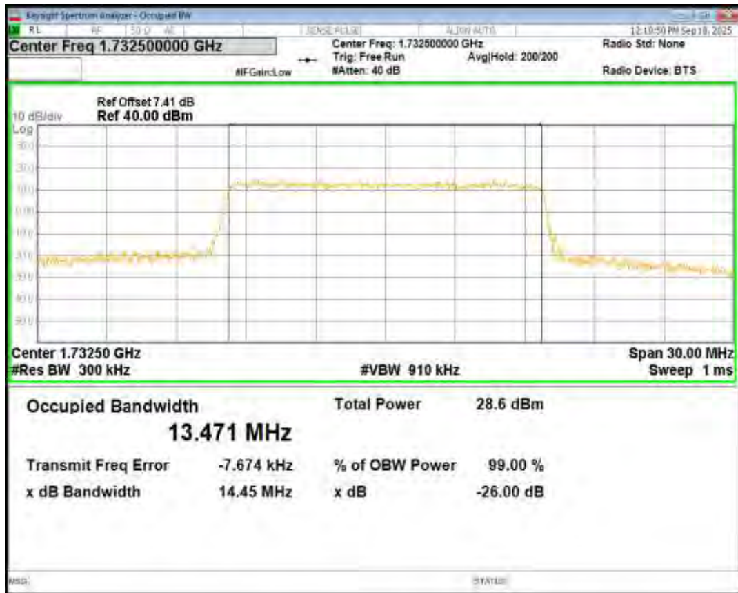
Band4 16QAM BW=15MHz Channel=20325 RB Size=75 Position=#0
