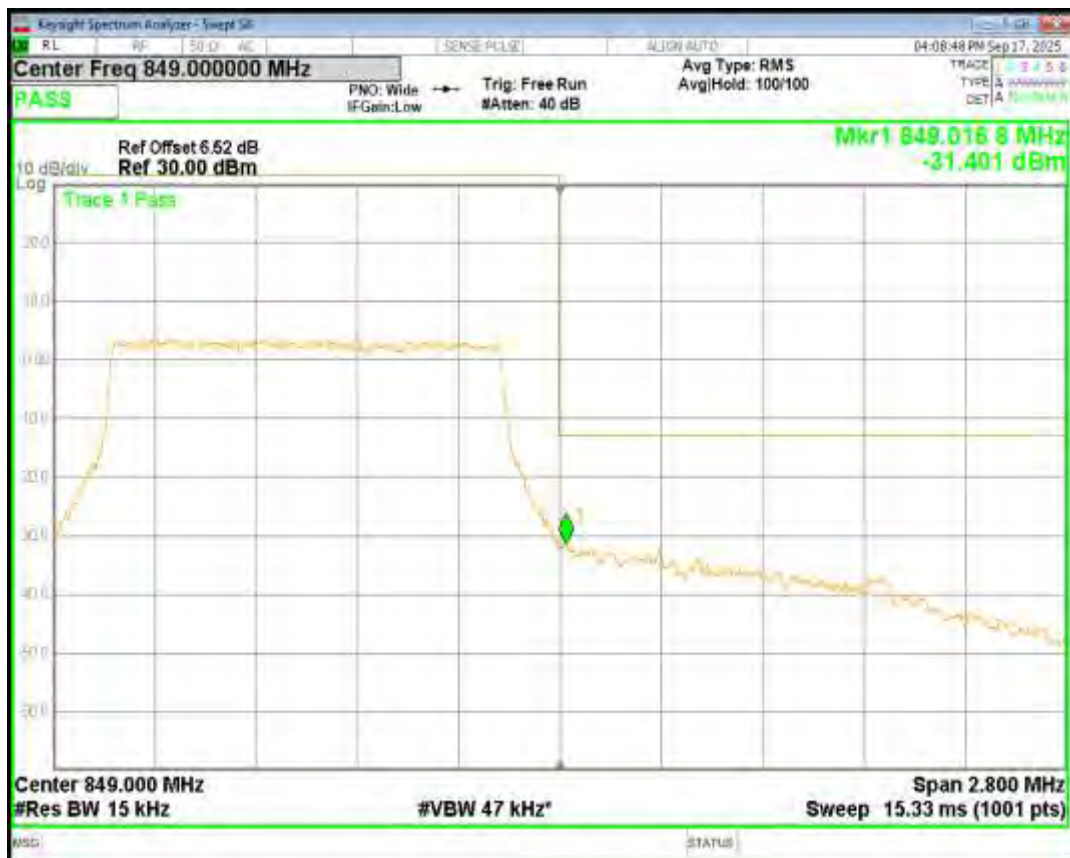
Band5 16QAM BW=10MHz Channel=20450 RB Size=50 Position=#0
