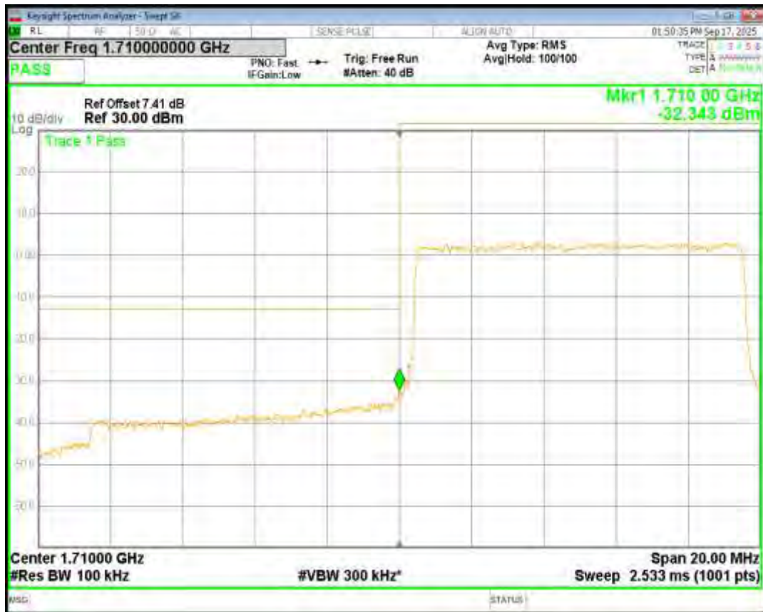
Band4 QPSK BW=10MHz Channel=20350 RB Size=50 Position=#0
