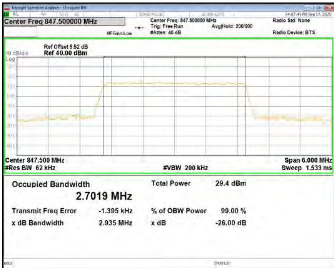
Band5 16QAM BW=5MHz Channel=20425 RB Size=25 Position=#0
