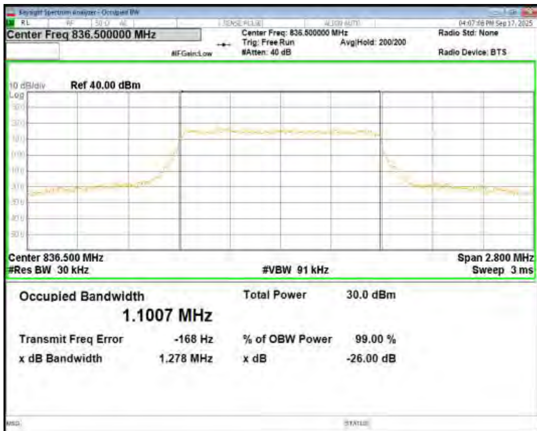
Band5 QPSK BW=1.4MHz Channel=20407 RB Size=6 Position=#0
