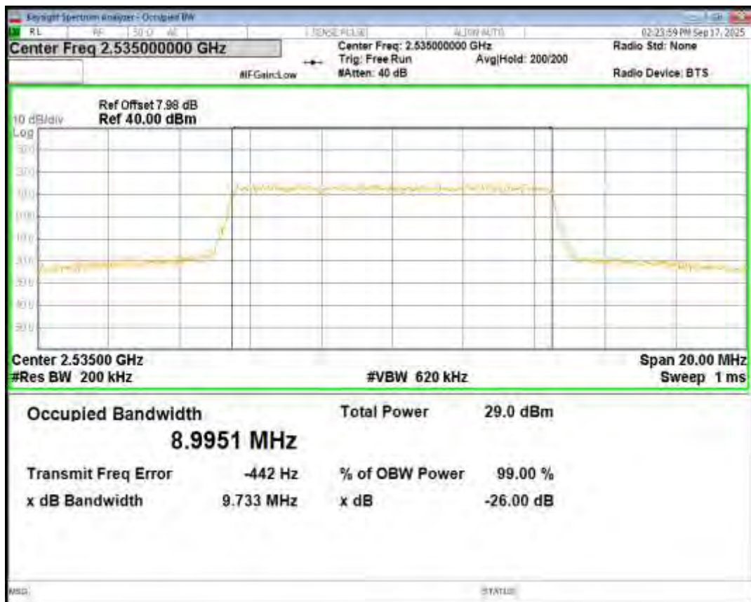
Band7 QPSK BW=10MHz Channel=20800 RB Size=50 Position=#0
