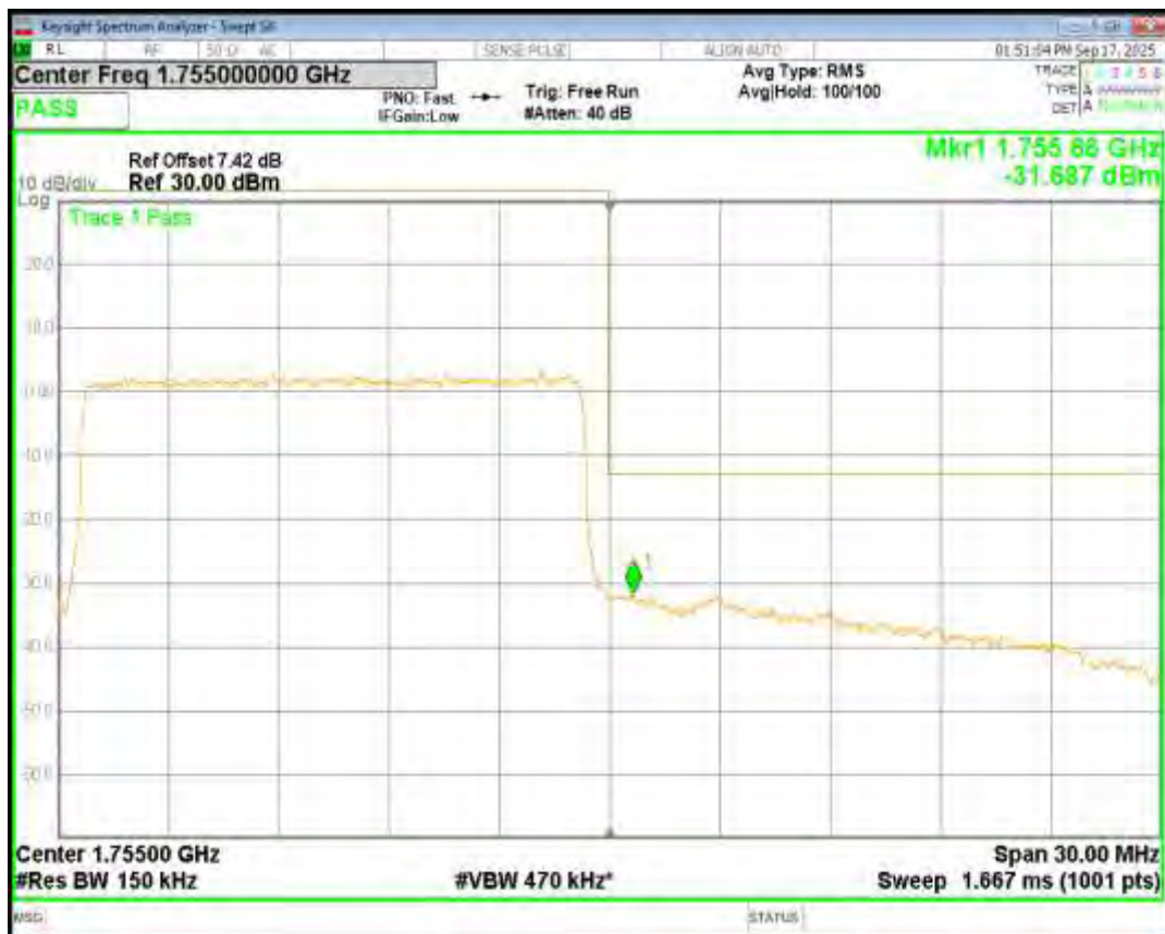
Band4 16QAM BW=20MHz Channel=20050 RB Size=100 Position=#0
