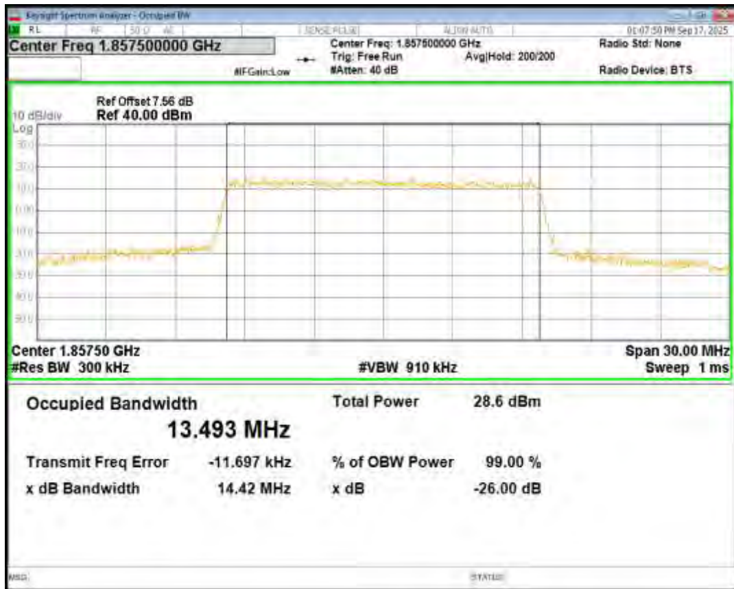
Band2 16QAM BW=3MHz Channel=18615 RB Size=15 Position=#0
