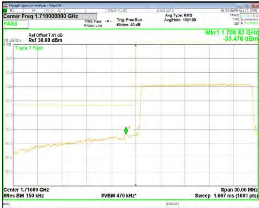
Band4 16QAM BW=15MHz Channel=20325 RB Size=75 Position=#0
