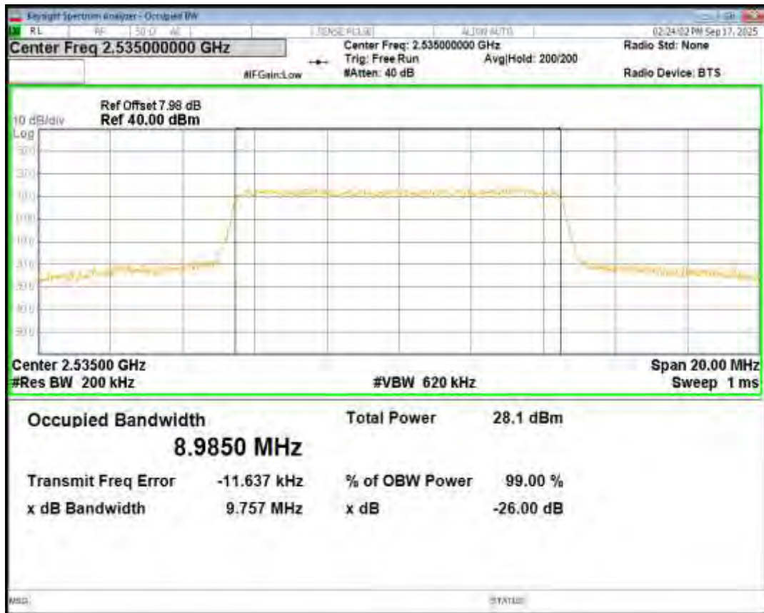
Band7 16QAM BW=10MHz Channel=21400 RB Size=50 Position=#0
