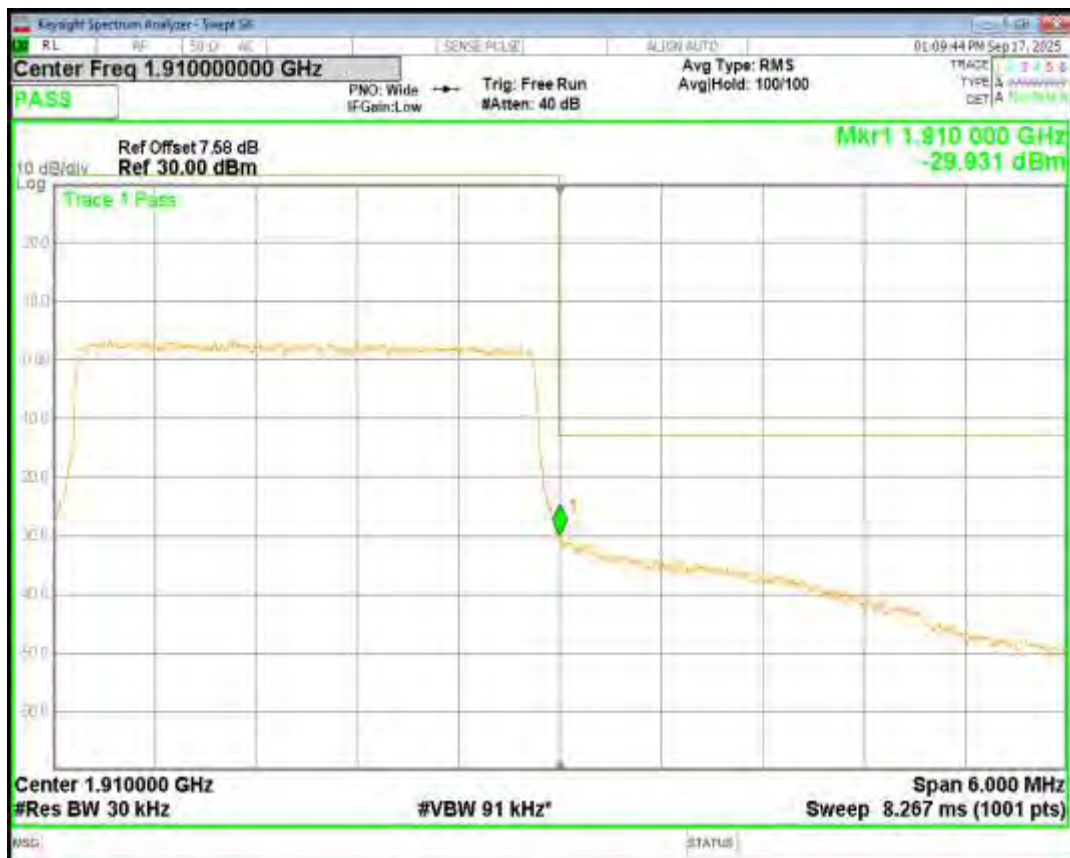
Band2 QPSK BW=5MHz Channel=18625 RB Size=25 Position=#0
