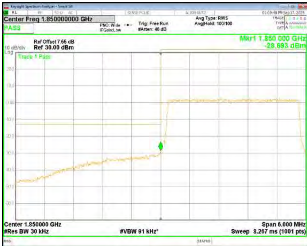
Band2 16QAM BW=3MHz Channel=19185 RB Size=15 Position=#0
