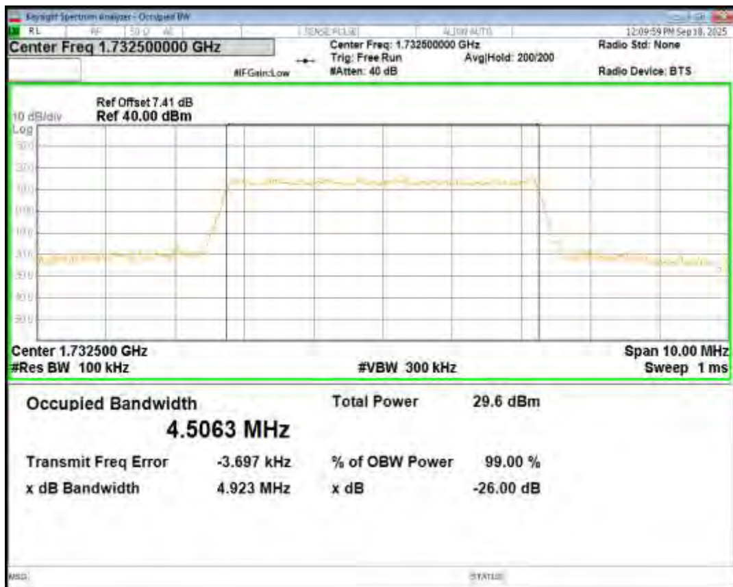
Band4 QPSK BW=5MHz Channel=20375 RB Size=25 Position=#0
