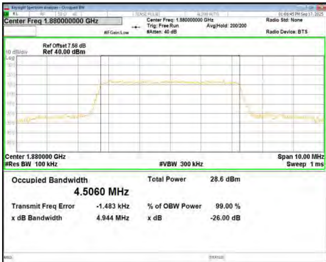
Band2 QPSK BW=1.4MHz Channel=19193 RB Size=6 Position=#0
