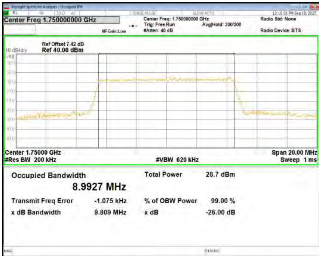
Band4 16QAM BW=15MHz Channel=20025 RB Size=75 Position=#0
