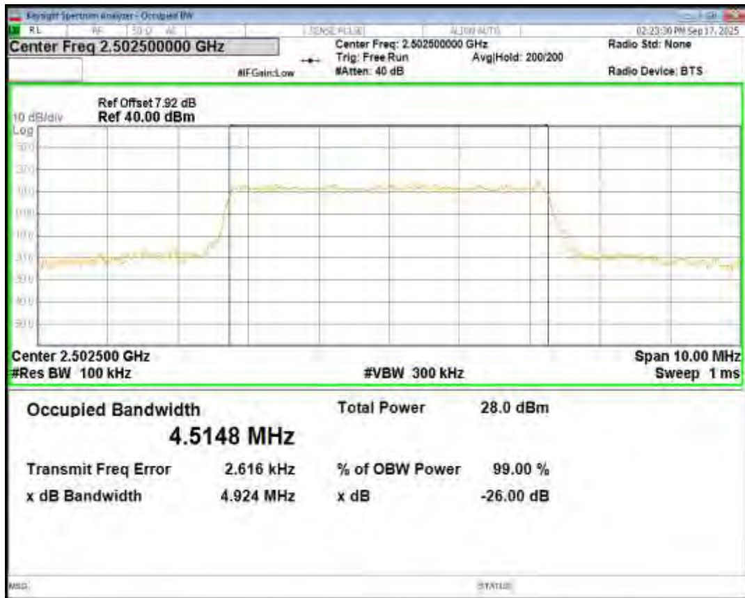
Band7 QPSK BW=10MHz Channel=21100 RB Size=50 Position=#0
