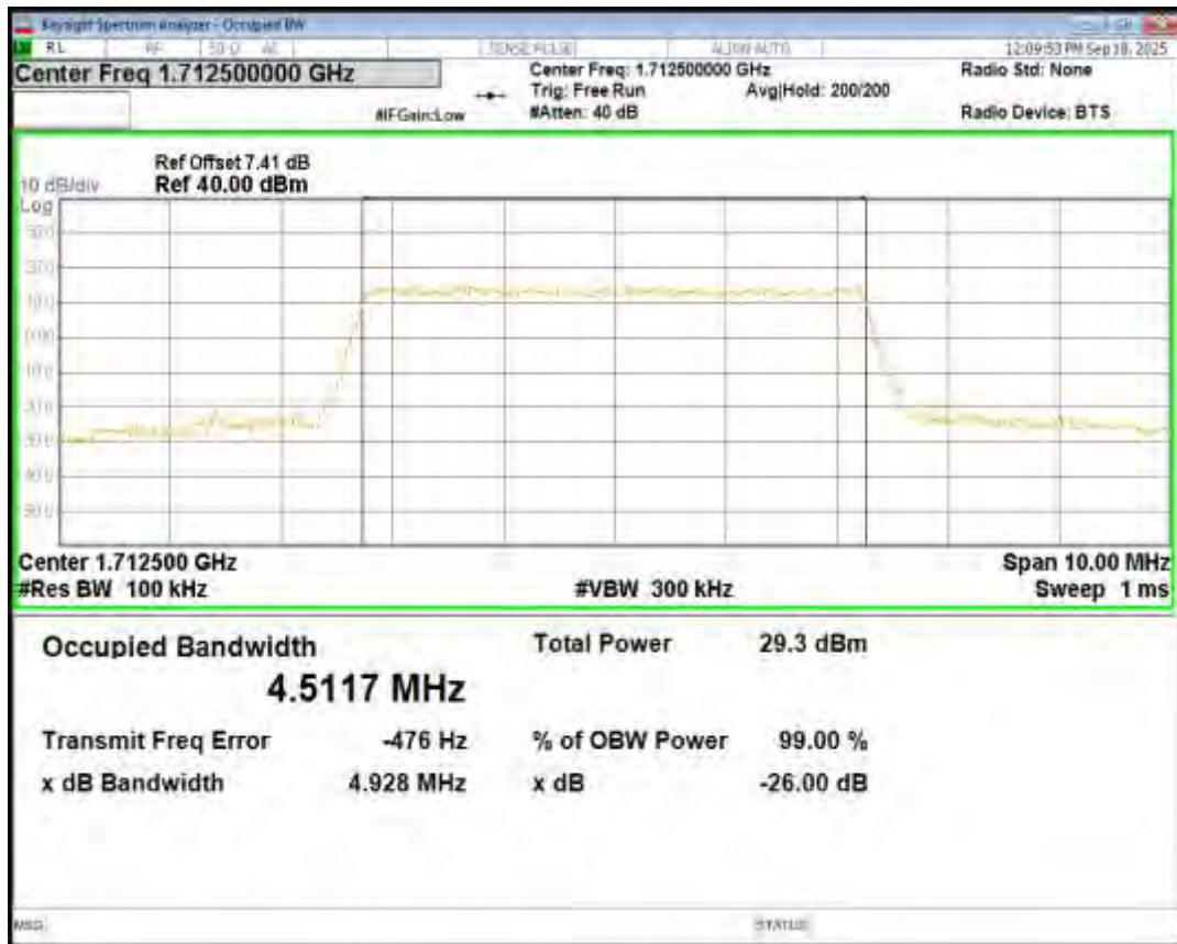
Band4 QPSK BW=5MHz Channel=20175 RB Size=25 Position=#0
