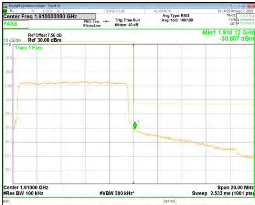
Band2 QPSK BW=15MHz Channel=18675 RB Size=75 Position=#0
