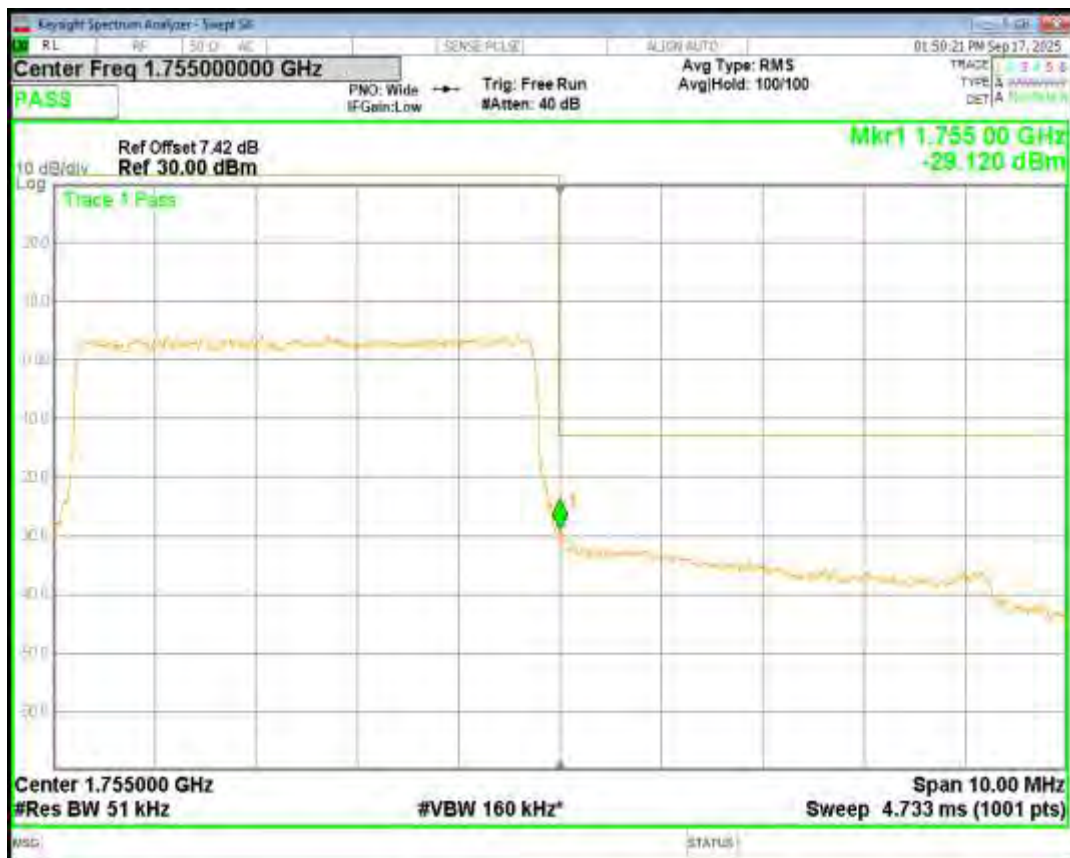
Band5 16QAM BW=1.4MHz Channel=20407 RB Size=6 Position=#0
