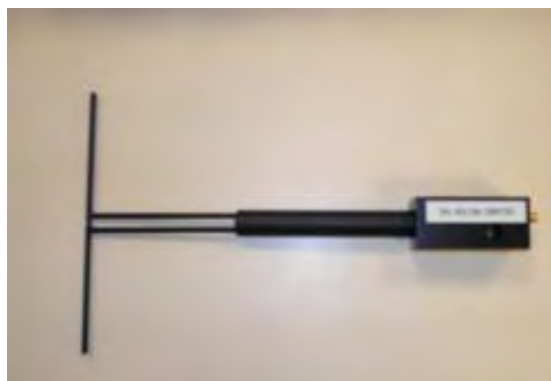
Figure 1 – MVG COMOSAR Validation Dipole
