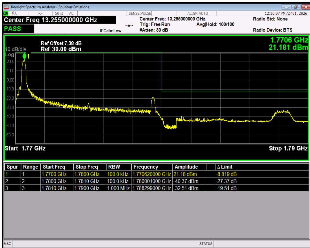
Band66 QPSK BW=10MHz Channel=132622 RB Size=1 Position=#Max
