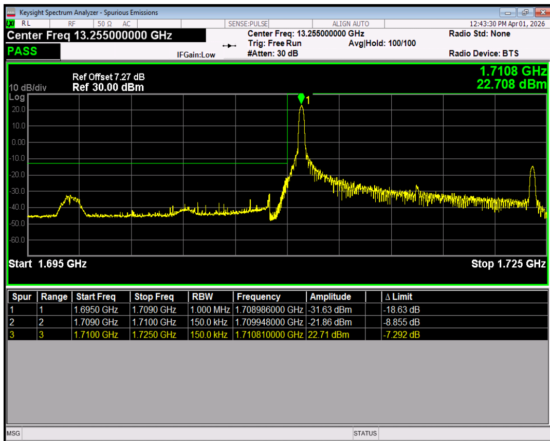
Band66 QPSK BW=15MHz Channel=132047 RB Size=75 Position=#0
