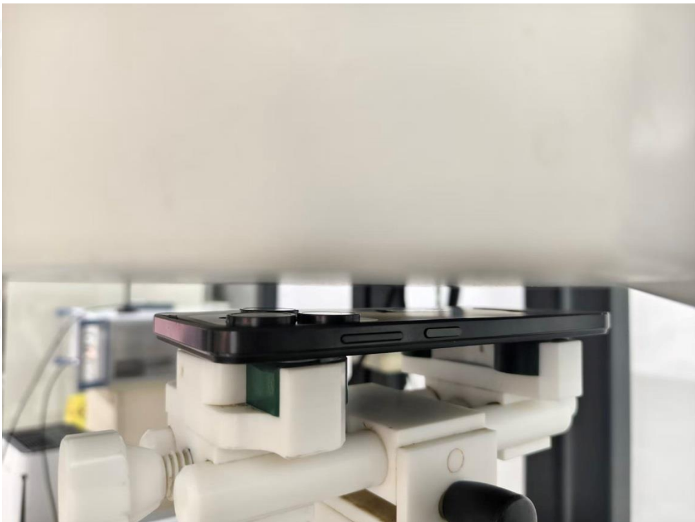
Body Back side(separation distance is 10mm)
