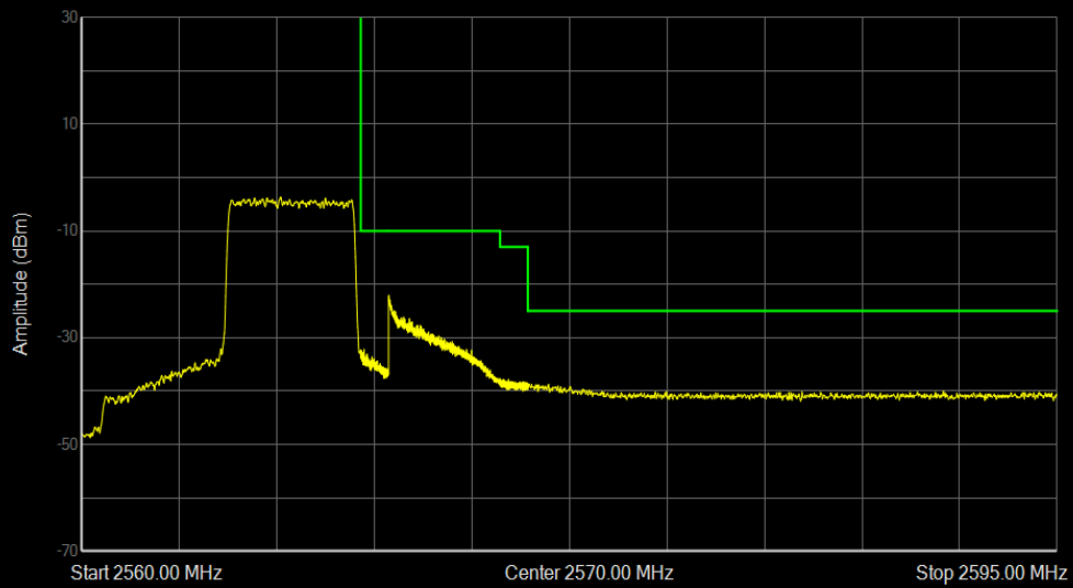
Band7 QPSK BW=5MHz Channel=21425 RB Size=25 Position=#0
