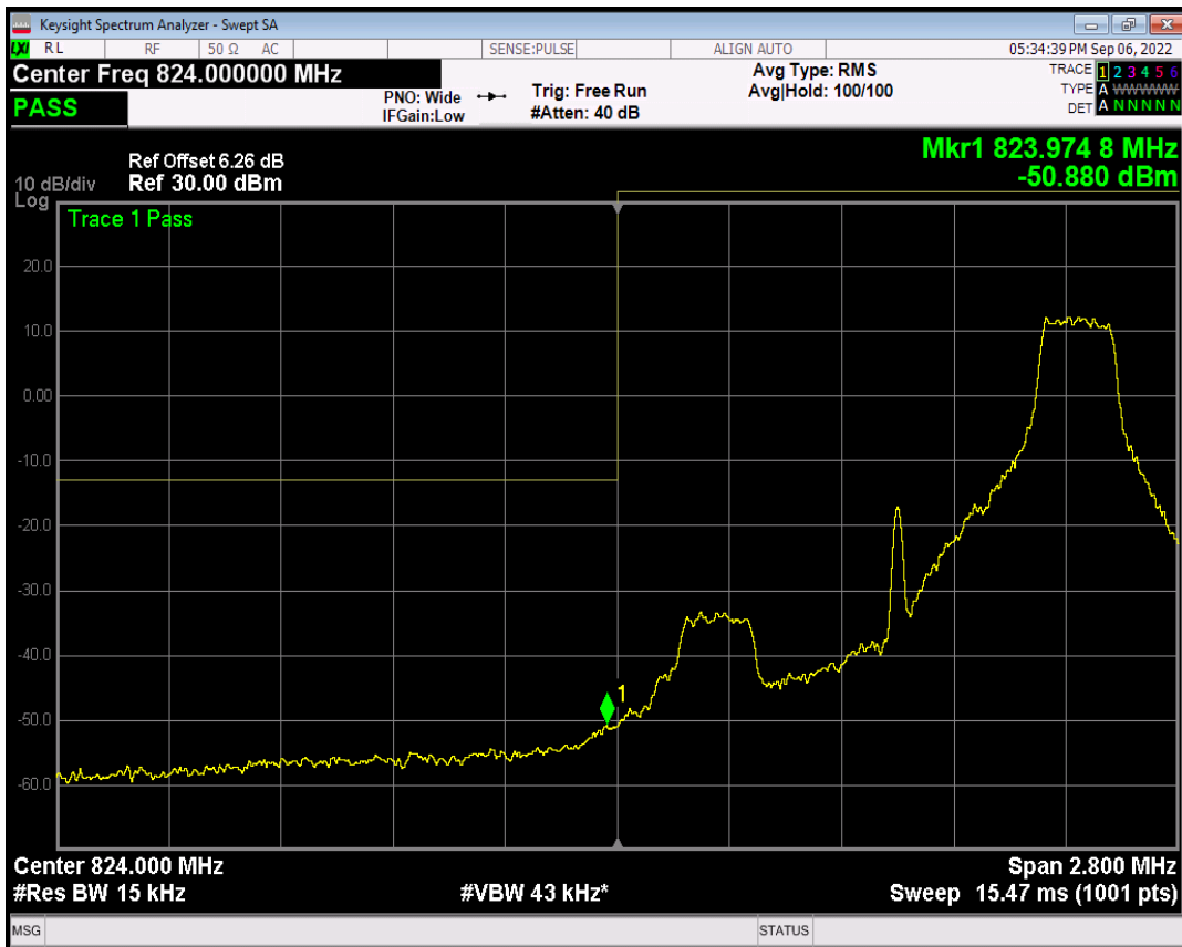
Band5 QAM16 BW=1.4MHz Channel=20407 RB Size=6 Position=#0
