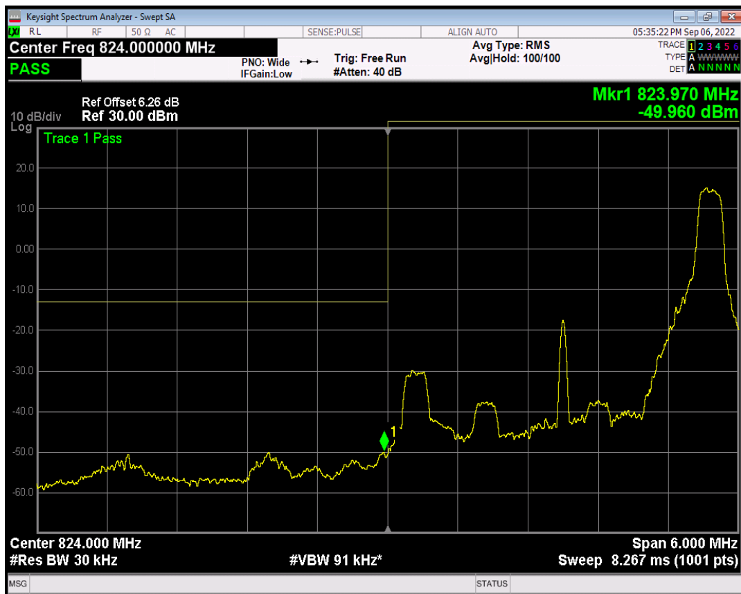
Band5 QAM16 BW=3MHz Channel=20415 RB Size=15 Position=#0
