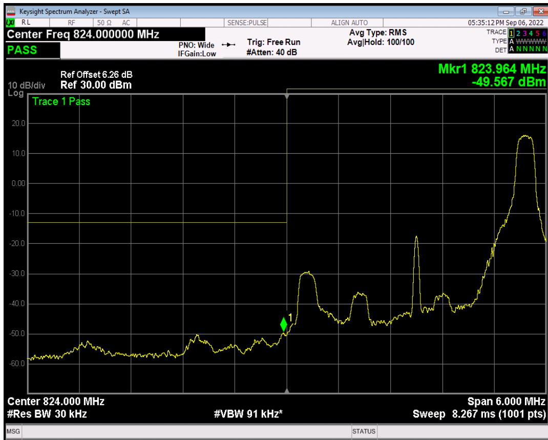
Band5 QPSK BW=3MHz Channel=20415 RB Size=15 Position=#0
