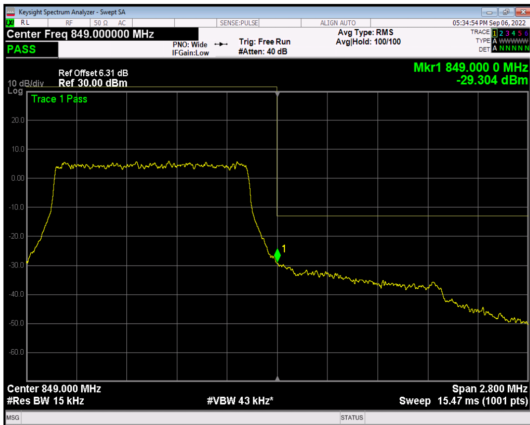
Band5 QAM16 BW=1.4MHz Channel=20643 RB Size=1 Position=#0
