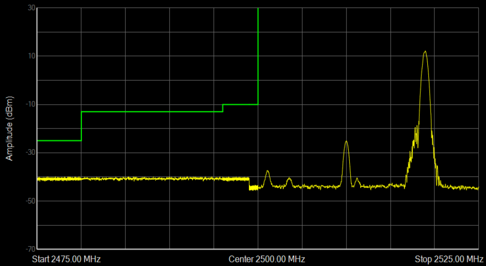
Band7 QPSK BW=20MHz Channel=20850 RB Size=1 Position=#Max
