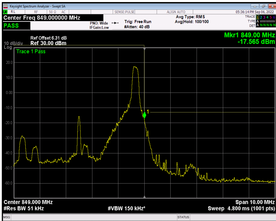
Band5 QAM16 BW=5MHz Channel=20625 RB Size=25 Position=#0
