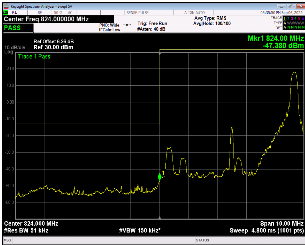
Band5 QPSK BW=5MHz Channel=20425 RB Size=25 Position=#0
