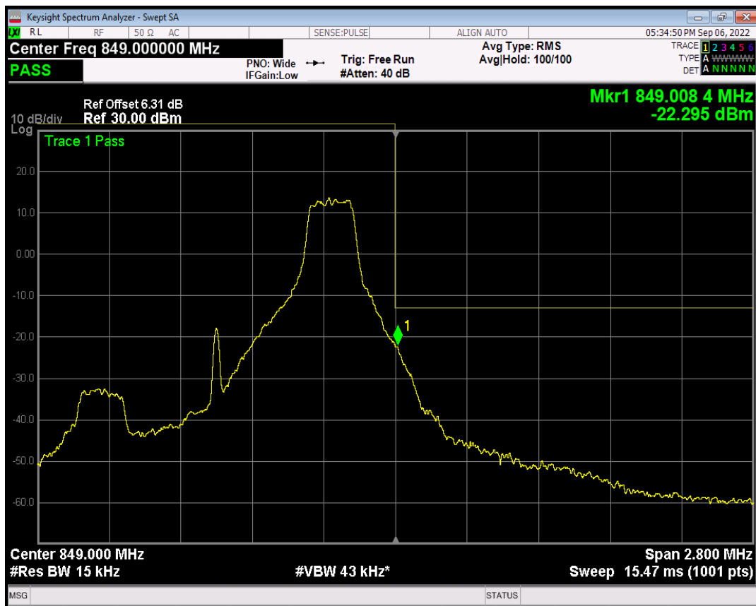
Band5 QPSK BW=1.4MHz Channel=20643 RB Size=1 Position=#0
