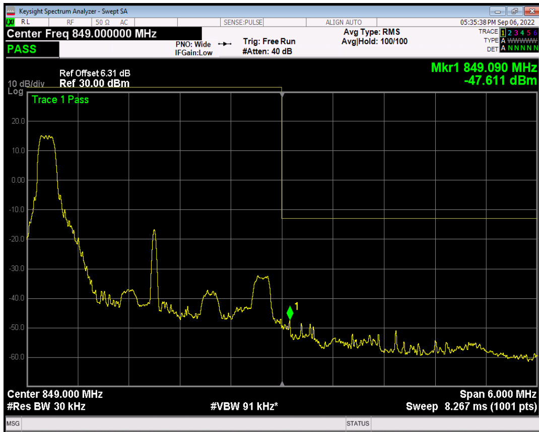
Band5 QAM16 BW=3MHz Channel=20635 RB Size=1 Position=#Max
