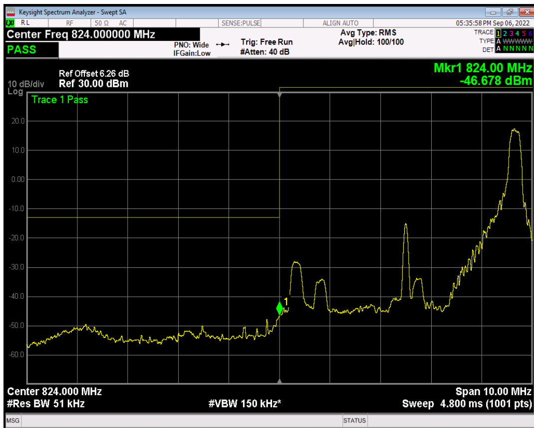
Band5 QAM16 BW=5MHz Channel=20425 RB Size=25 Position=#0
