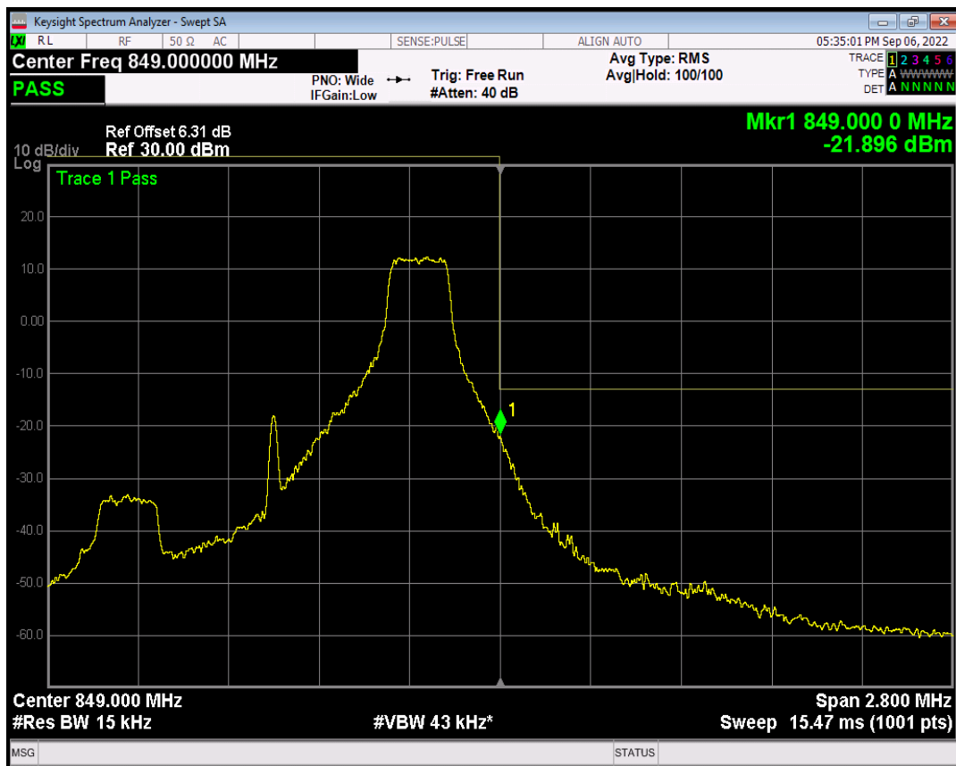
Band5 QAM16 BW=1.4MHz Channel=20643 RB Size=6 Position=#0
