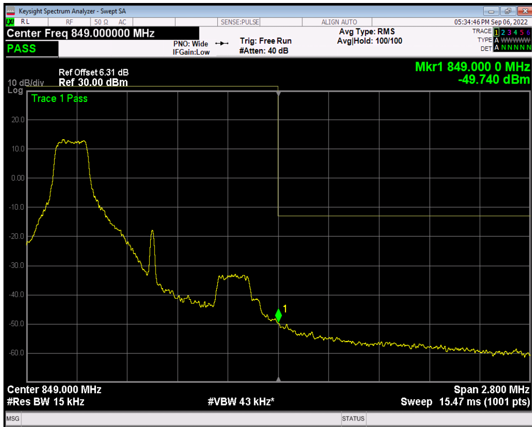
Band5 QPSK BW=1.4MHz Channel=20643 RB Size=6 Position=#0
