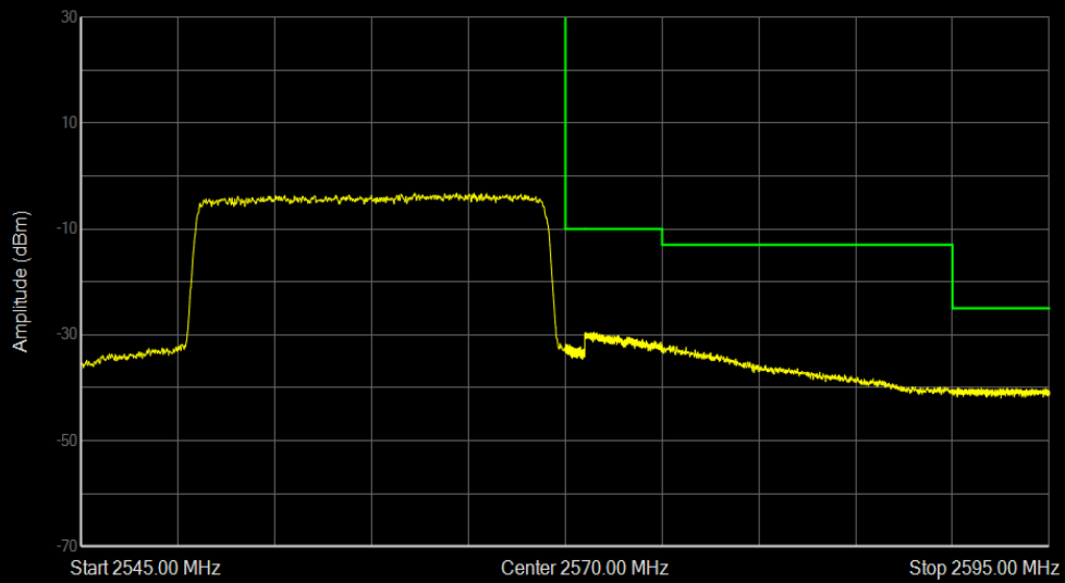
Band7 QPSK BW=20MHz Channel=21350 RB Size=100 Position=#0
