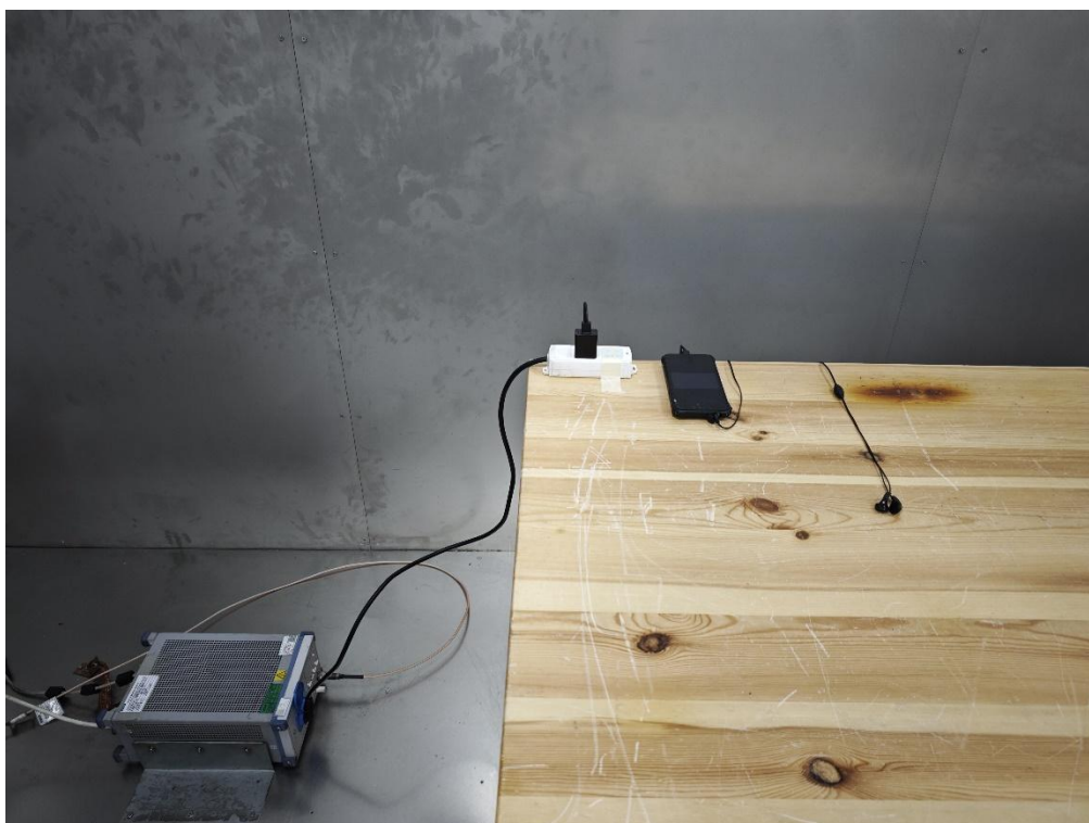
AC Conducted Measurement Photos
