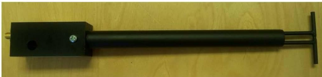
Figure 1 – MVG COMOSAR Validation Dipole
