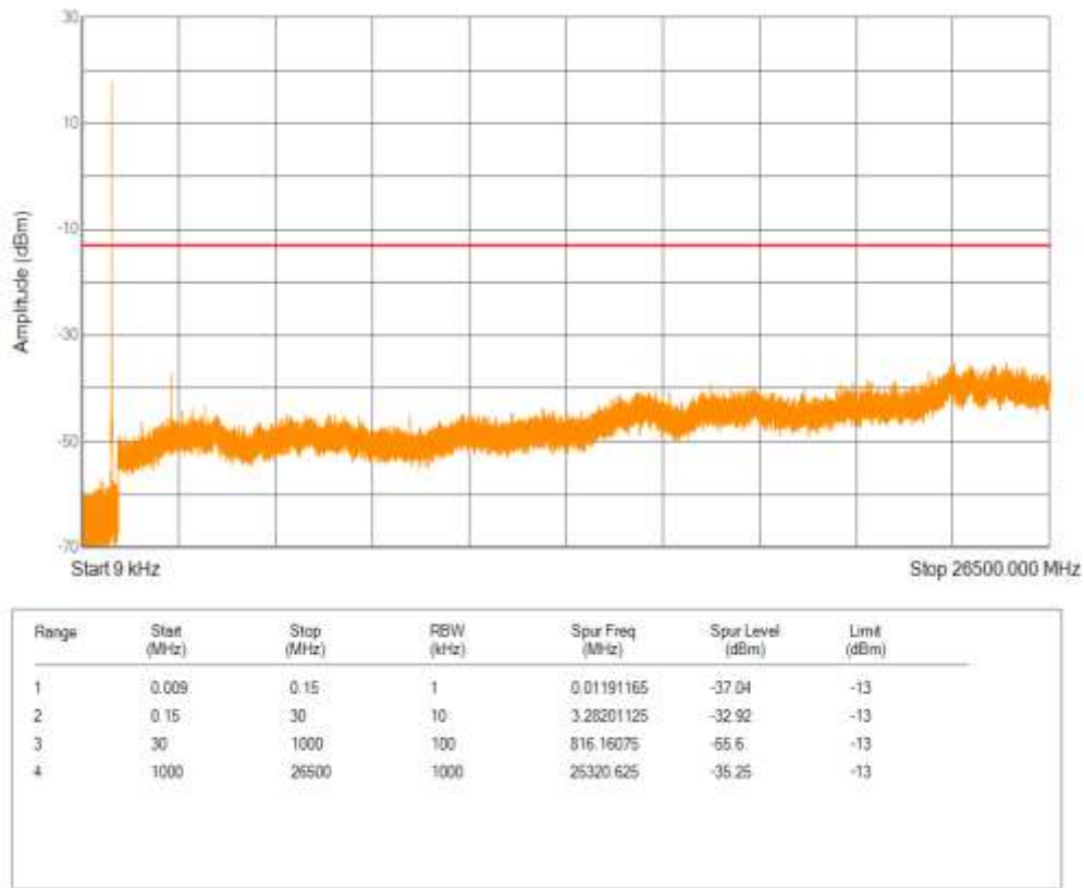
Band5 16QAM BW=1.4MHz Channel=20525 RB Size=6 Position=#0
