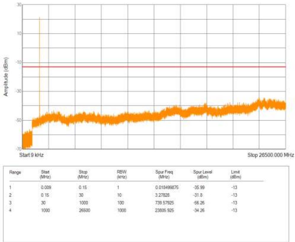
Band4 16QAM BW=5MHz Channel=19975 RB Size=25 Position=#0
