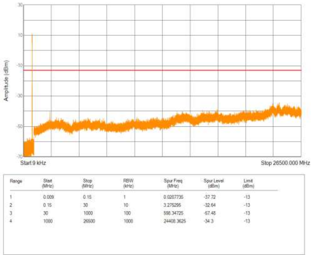
Band5 QPSK BW=1.4MHz Channel=20407 RB Size=6 Position=#0
