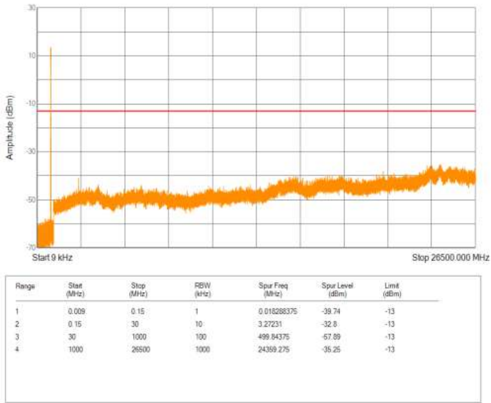
Band5 QPSK BW=3MHz Channel=20635 RB Size=15 Position=#0
