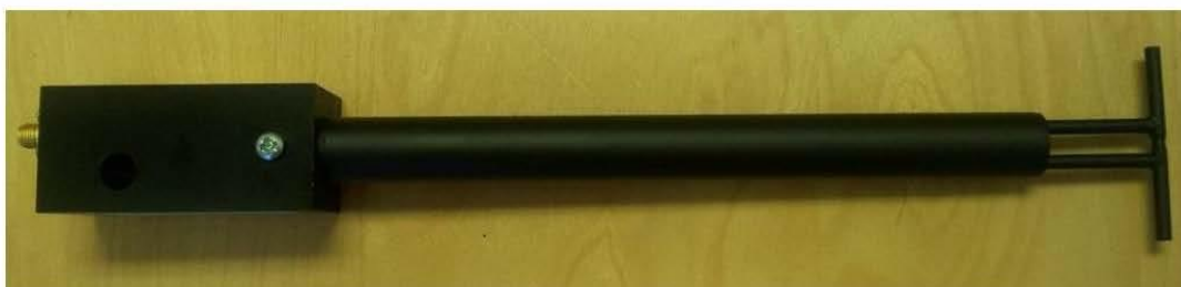
Figure 1 – MVG COMOSAR Validation Dipole
