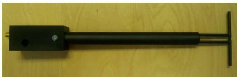
Figure 1 – MVG COMOSAR Validation Dipole
