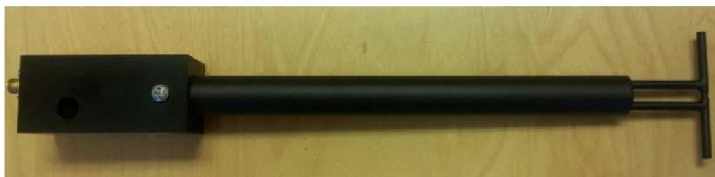
Figure 1 – MVG COMOSAR Validation Dipole
