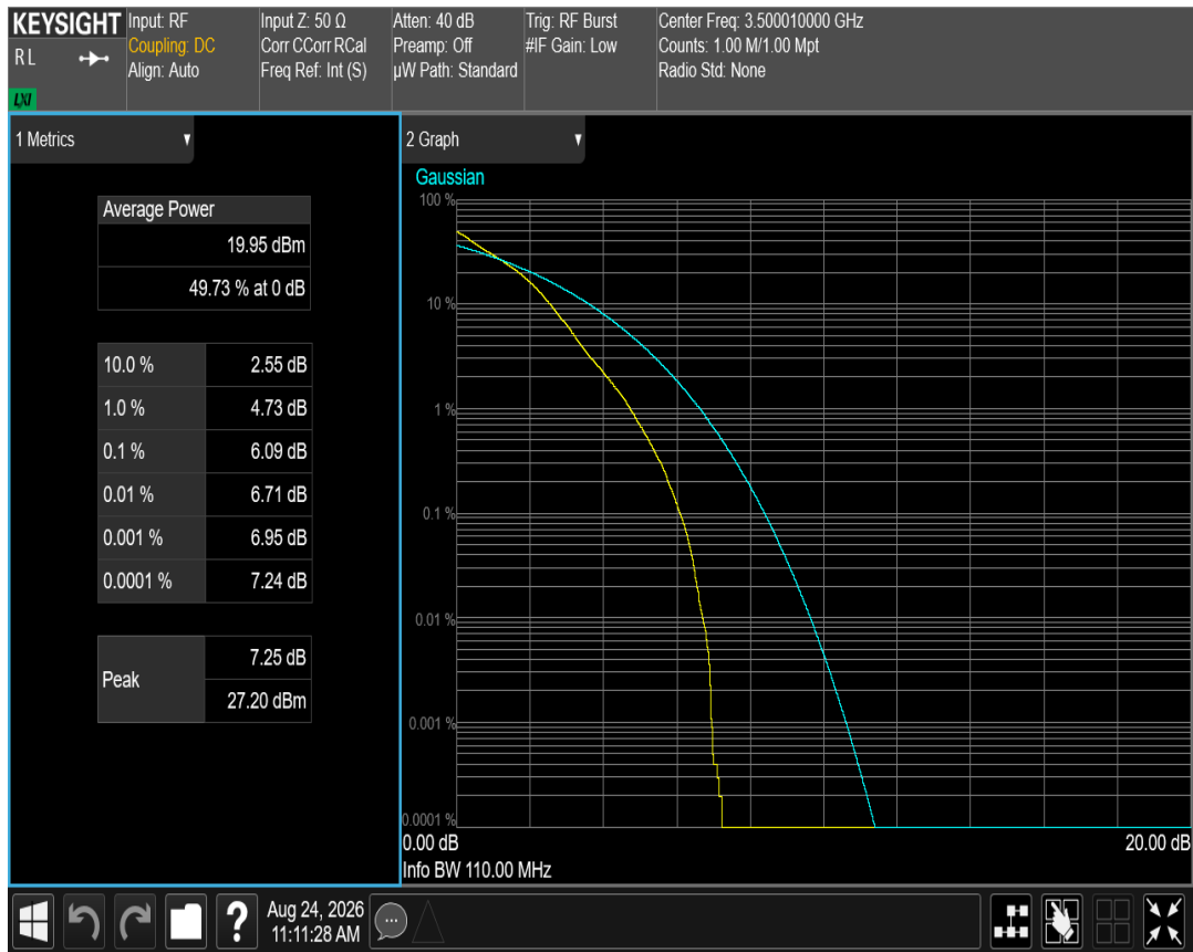
n78(3450-3550) SCS=30kHz DFT_16QAM BW=15MHz Channel=633334 RB=36@0
