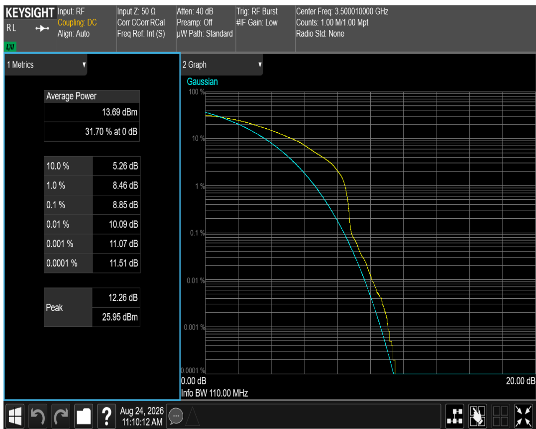
n78(3450-3550) SCS=15kHz DFT_BPSK BW=50MHz Channel=633334 RB=270@0
