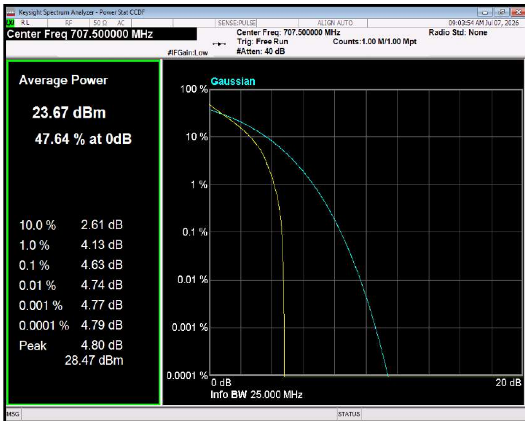
Band12 16QAM BW=5MHz Channel=23095 RB Size=1 Position=#0
