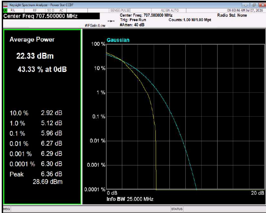
Band12 QPSK BW=3MHz Channel=23095 RB Size=1 Position=#0
