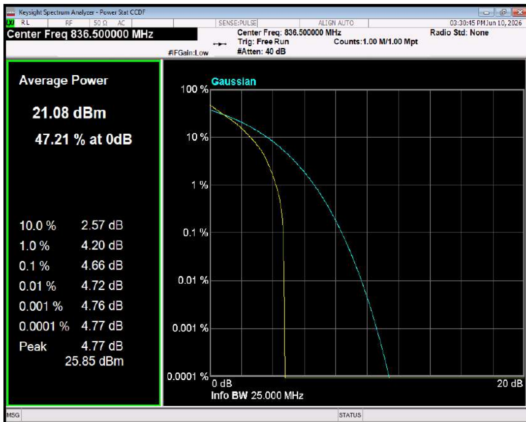
Band5 16QAM BW=5MHz Channel=20525 RB Size=1 Position=#0
