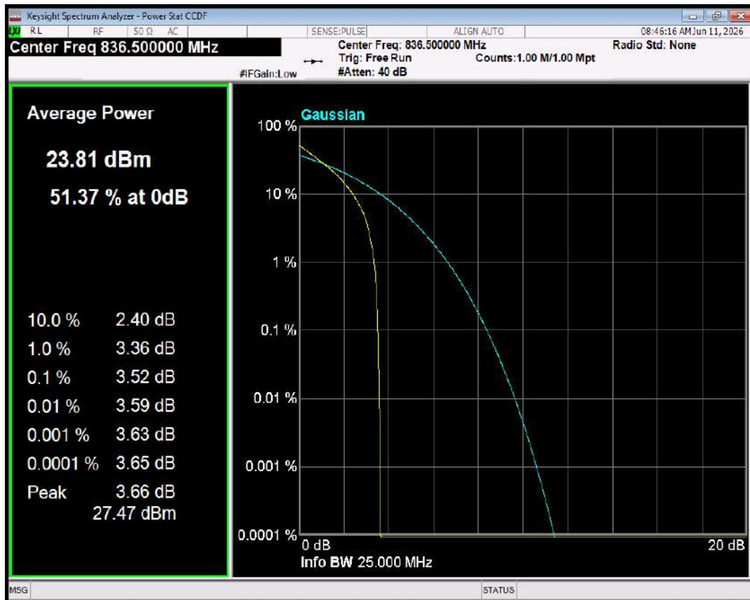
Band26(824-849) 16QAM BW=10MHz Channel=26915 RB Size=1 Position=#0
