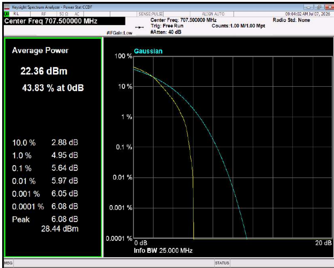
Band17 QPSK BW=5MHz Channel=23790 RB Size=1 Position=#0
