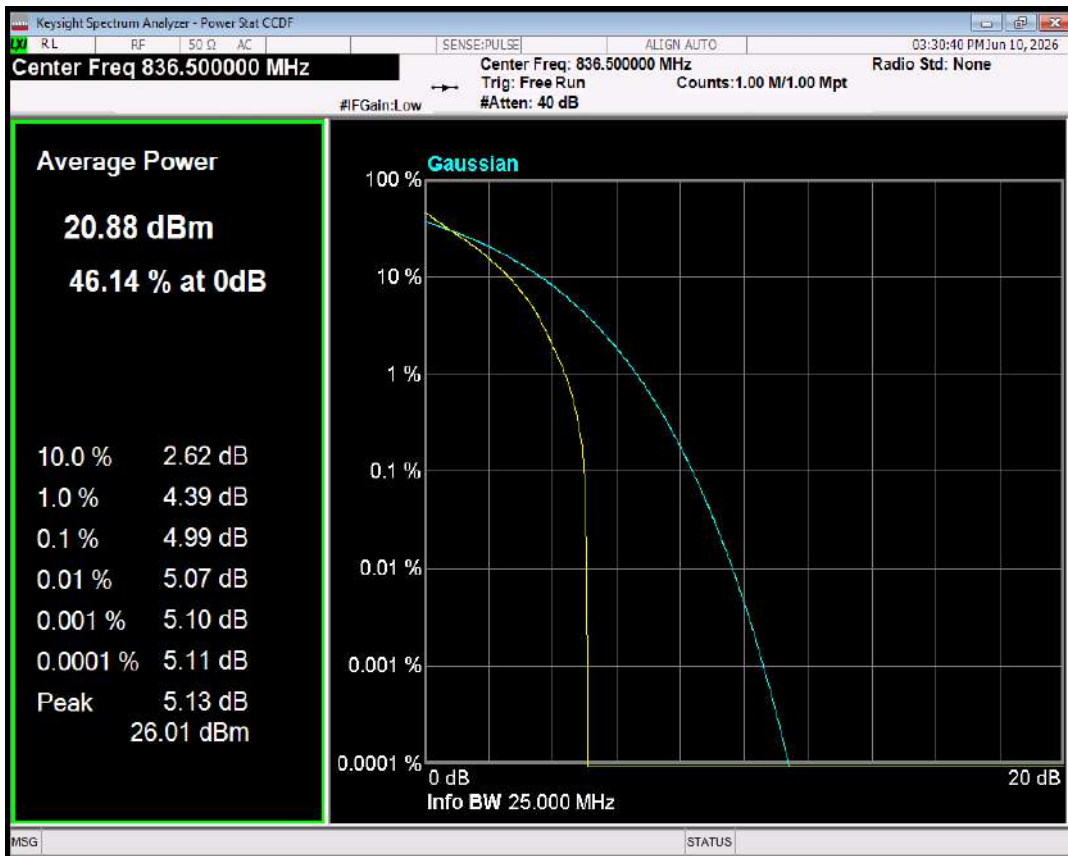
Band5 16QAM BW=3MHz Channel=20525 RB Size=1 Position=#0
