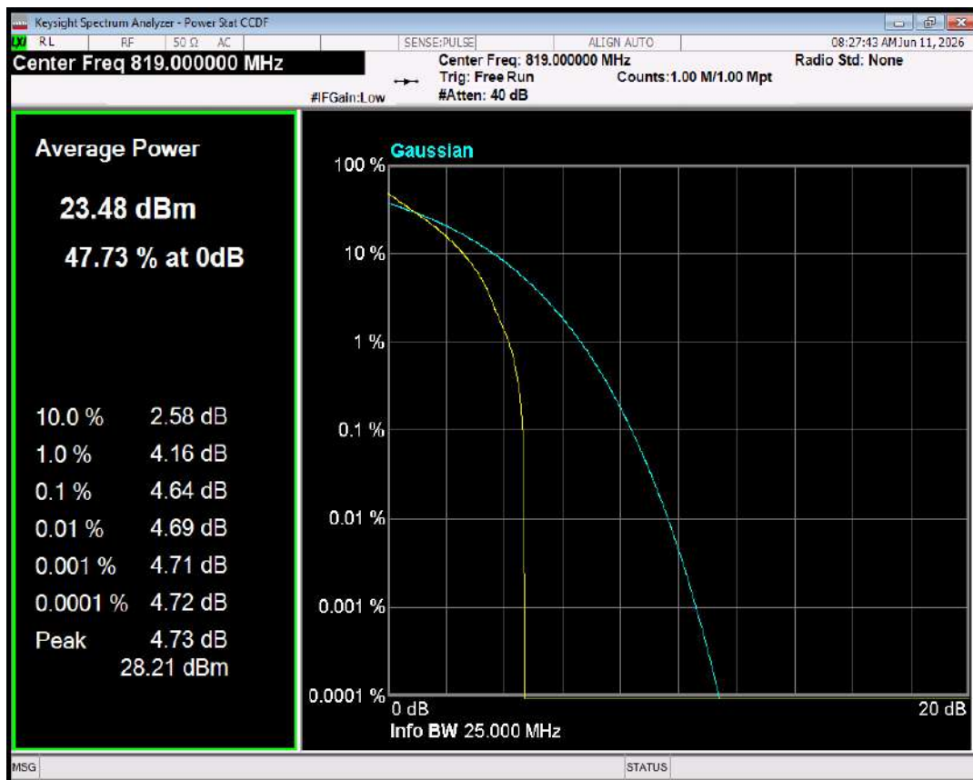
Band26(814-824) 16QAM BW=3MHz Channel=26740 RB Size=1 Position=#0
