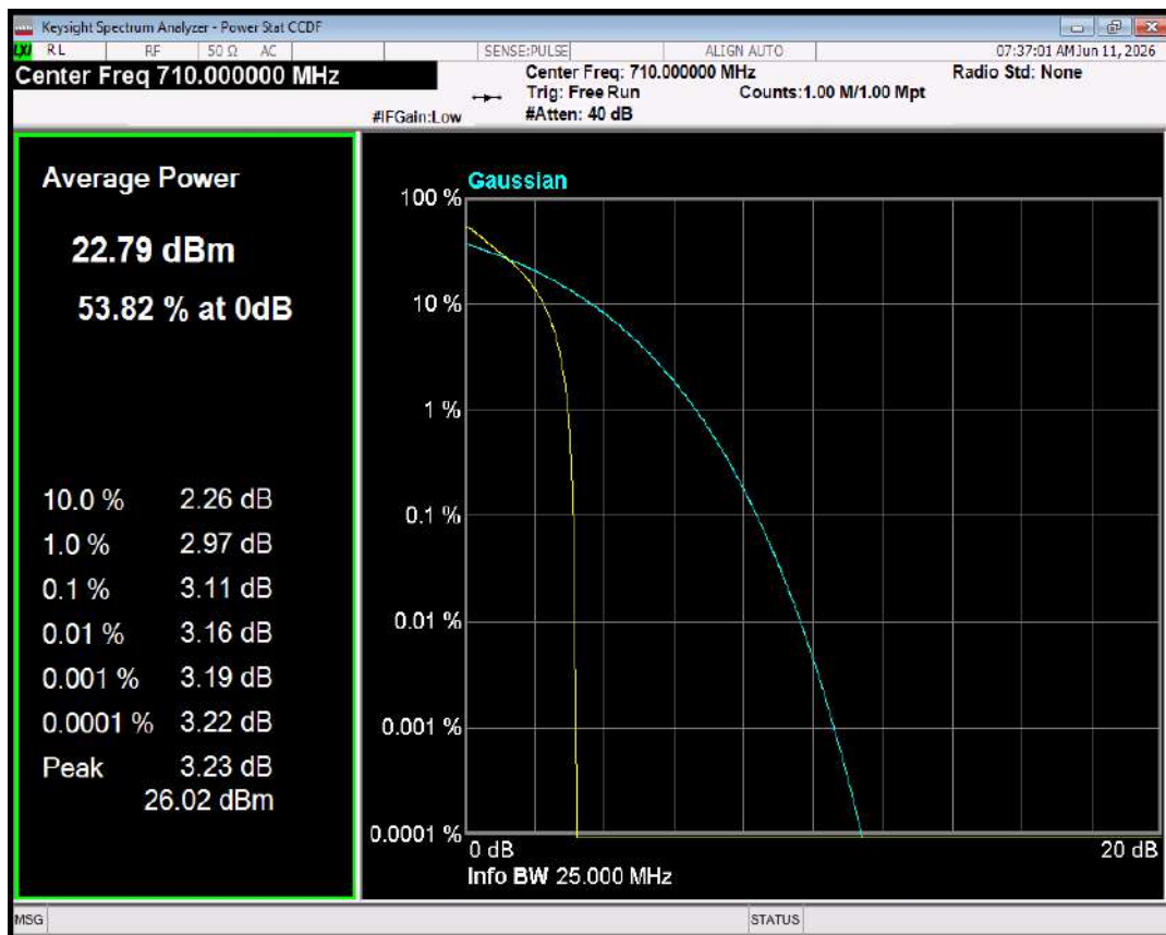
Band17 16QAM BW=5MHz Channel=23790 RB Size=1 Position=#0
