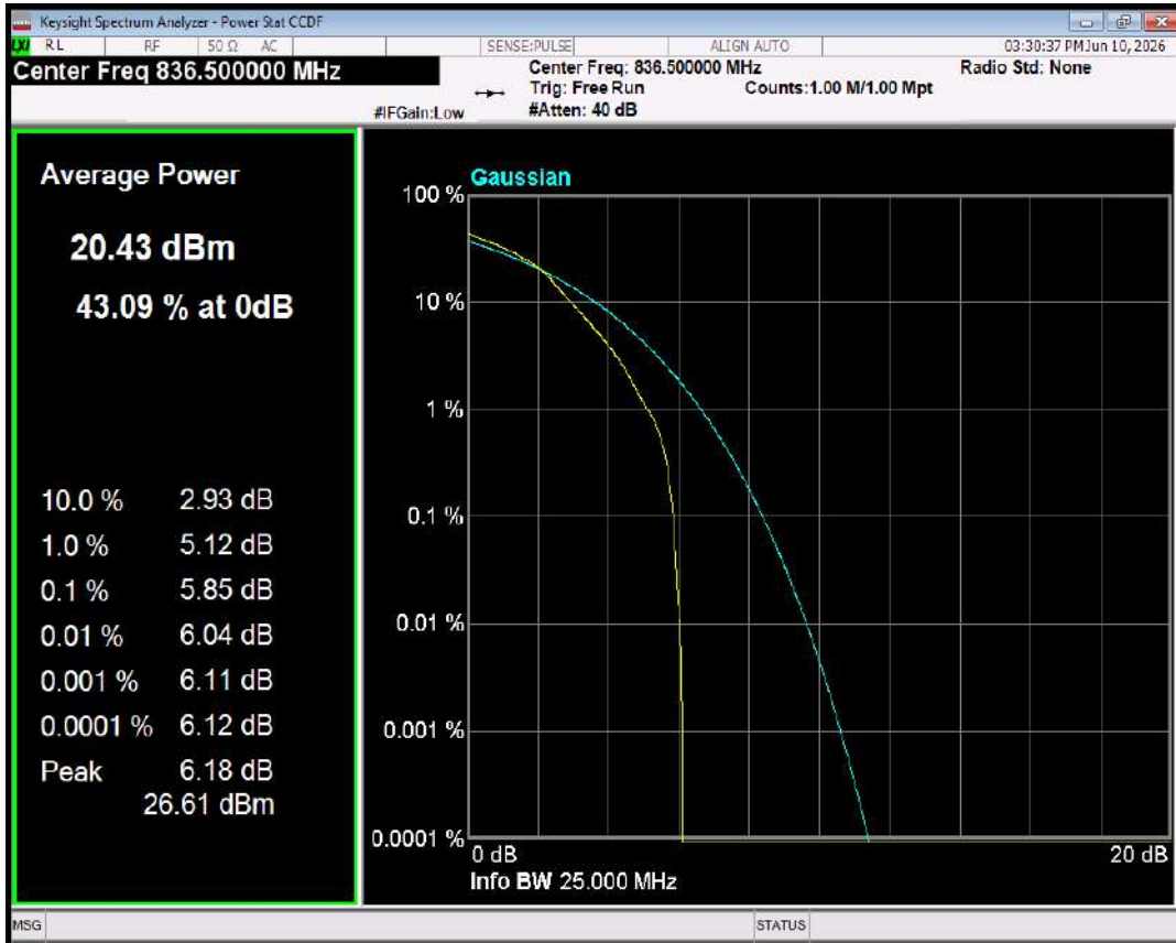
Band5 QPSK BW=3MHz Channel=20525 RB Size=1 Position=#0
