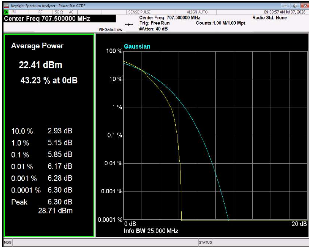
Band12 QPSK BW=10MHz Channel=23095 RB Size=1 Position=#0
