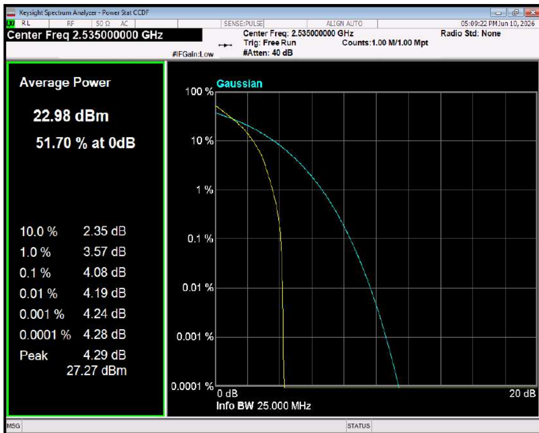
Band7 16QAM BW=10MHz Channel=21100 RB Size=1 Position=#0
