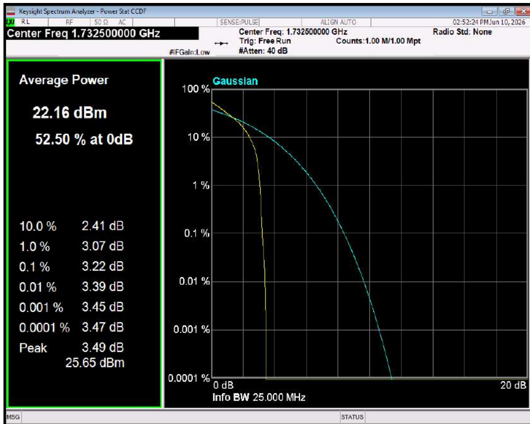
Band4 16QAM BW=3MHz Channel=20175 RB Size=1 Position=#0
