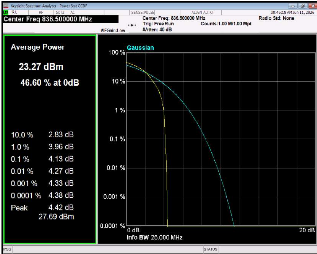
Band26(824-849) QPSK BW=15MHz Channel=26915 RB Size=1 Position=#0
