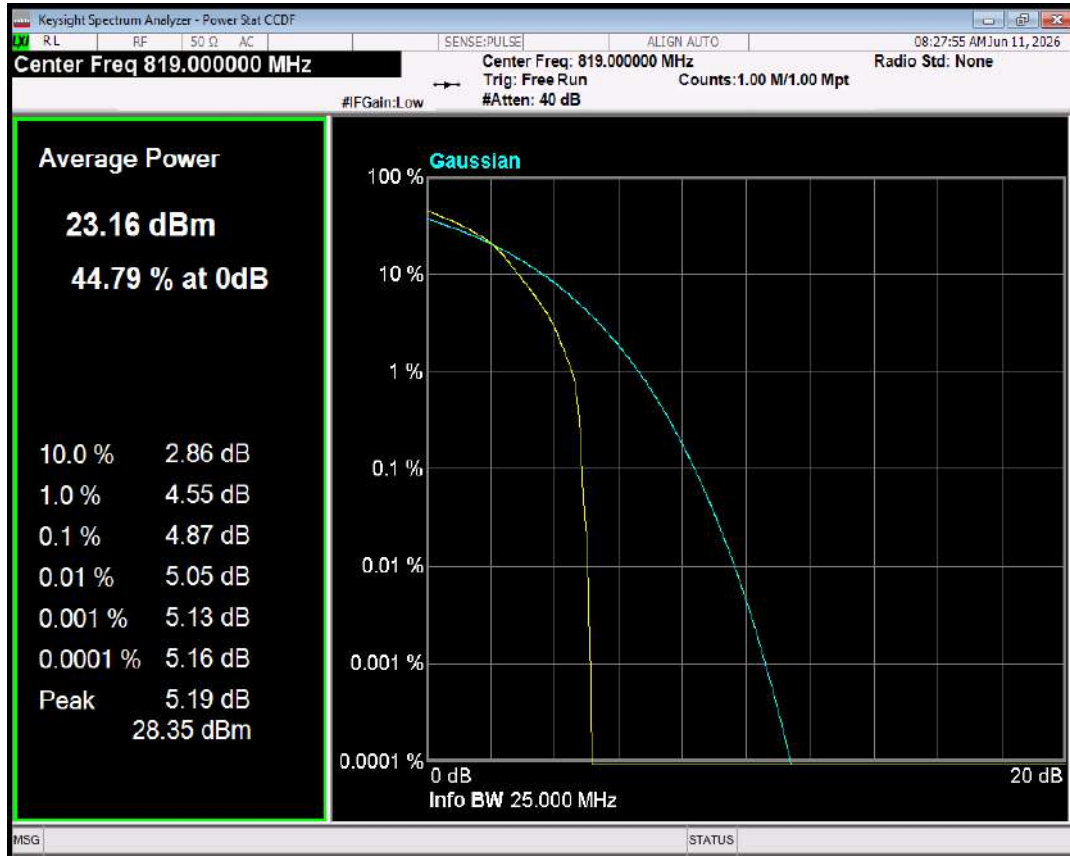
Band26(824-849) QPSK BW=1.4MHz Channel=26915 RB Size=1 Position=#0
