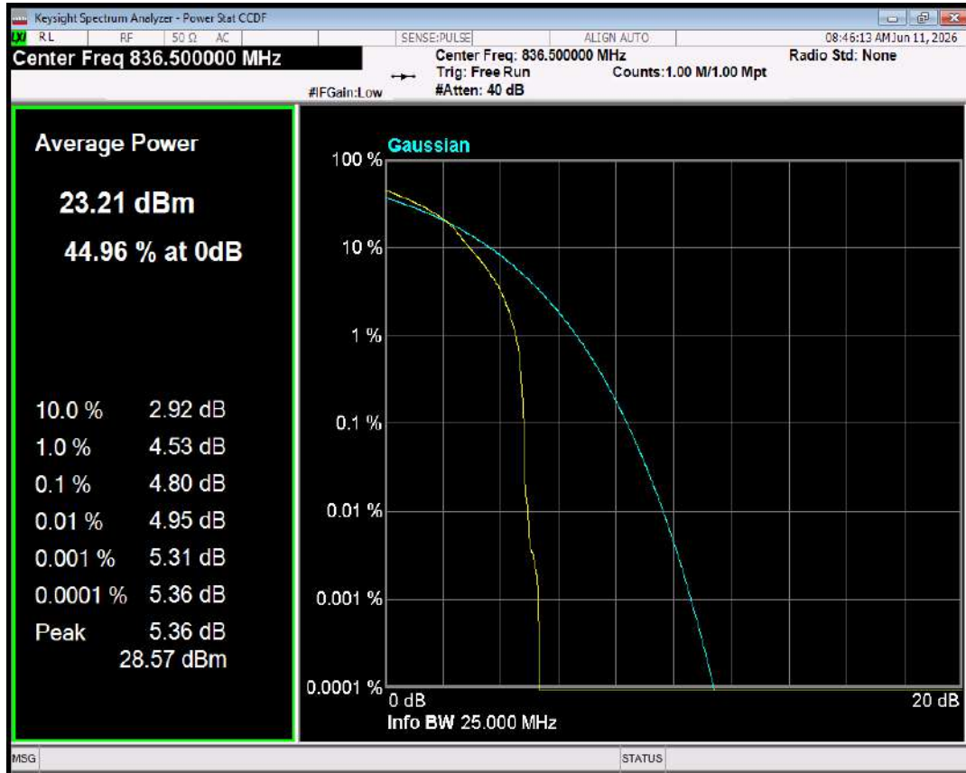
Band26(824-849) QPSK BW=10MHz Channel=26915 RB Size=1 Position=#0
