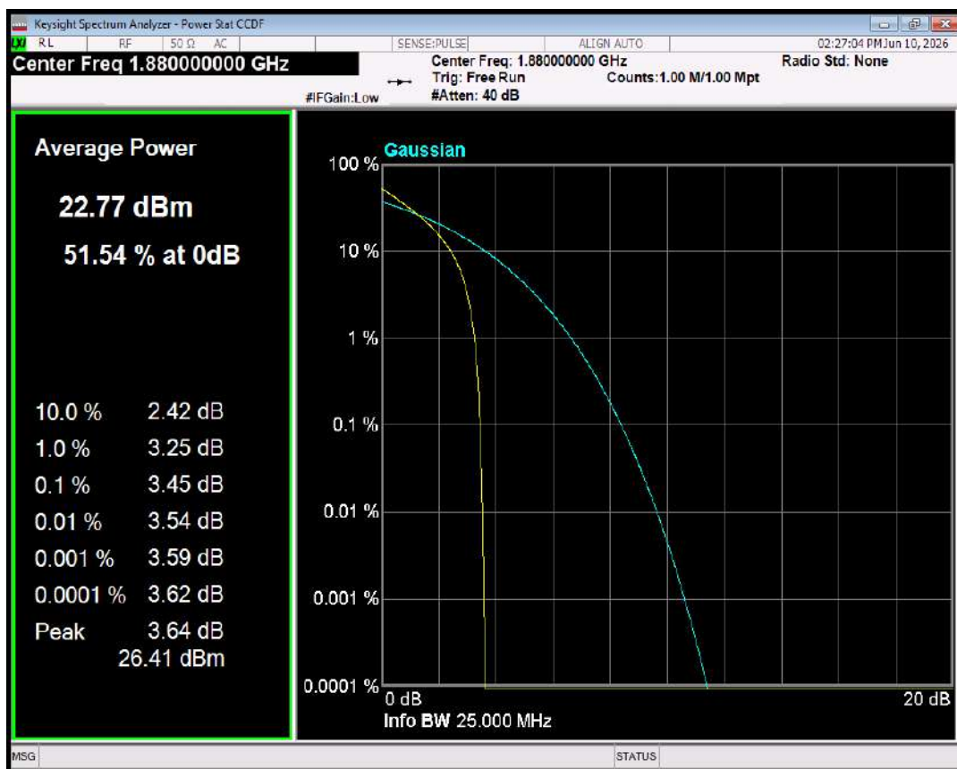
Band2 16QAM BW=15MHz Channel=18900 RB Size=1 Position=#0
