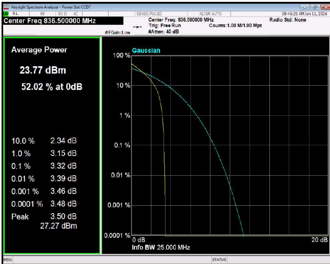
Band26(824-849) 16QAM BW=15MHz Channel=26915 RB Size=1 Position=#0
