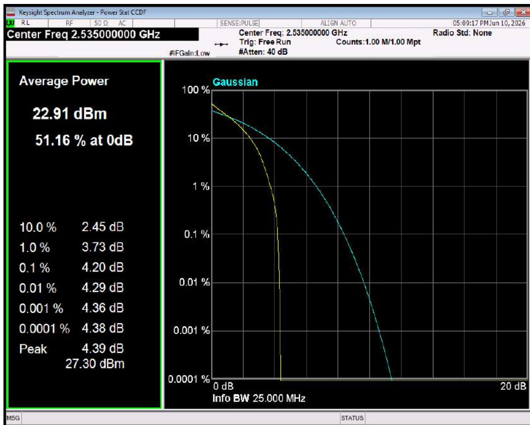
Band7 16QAM BW=5MHz Channel=21100 RB Size=1 Position=#0
