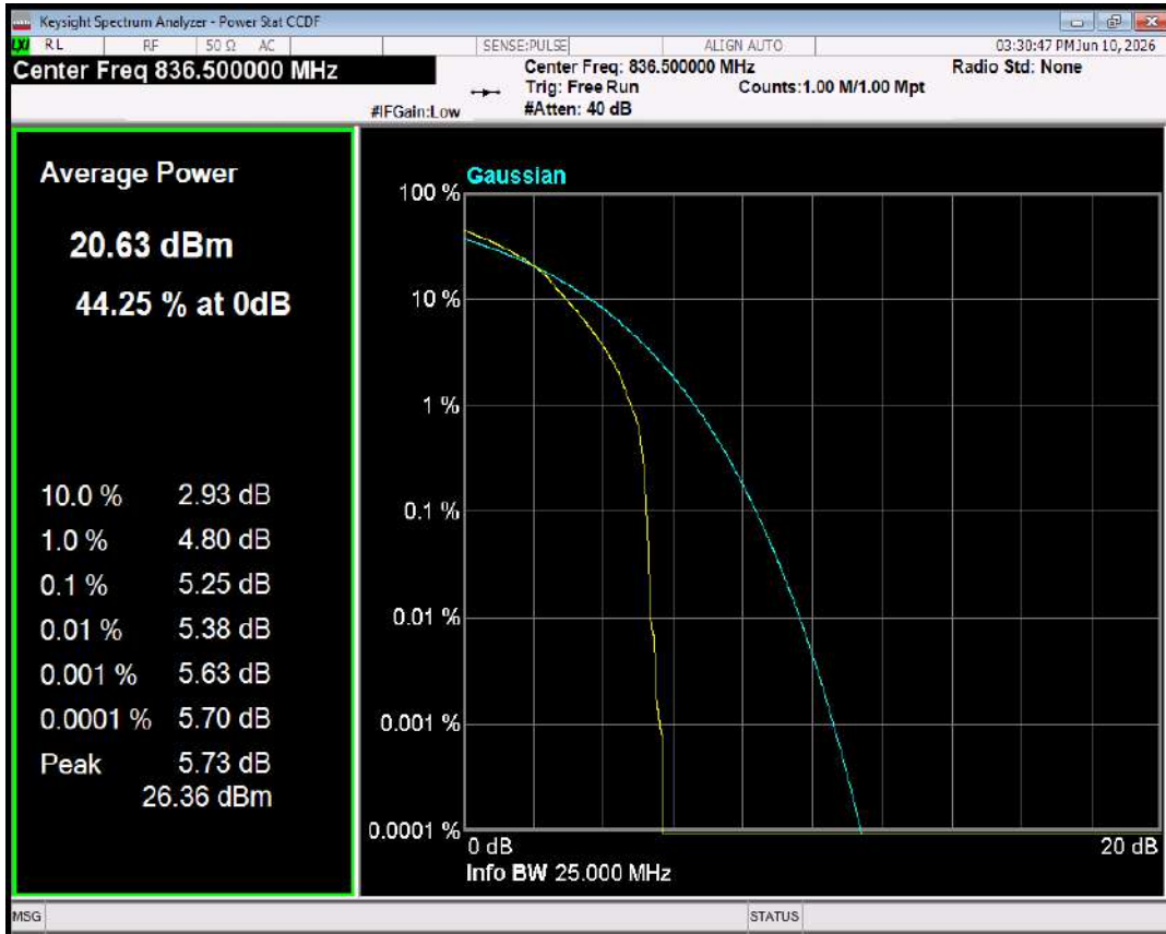
Band5 QPSK BW=10MHz Channel=20525 RB Size=1 Position=#0
