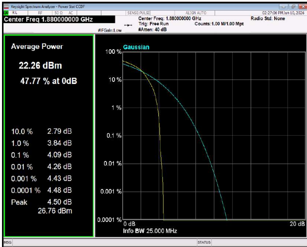
Band2 QPSK BW=20MHz Channel=18900 RB Size=1 Position=#0
