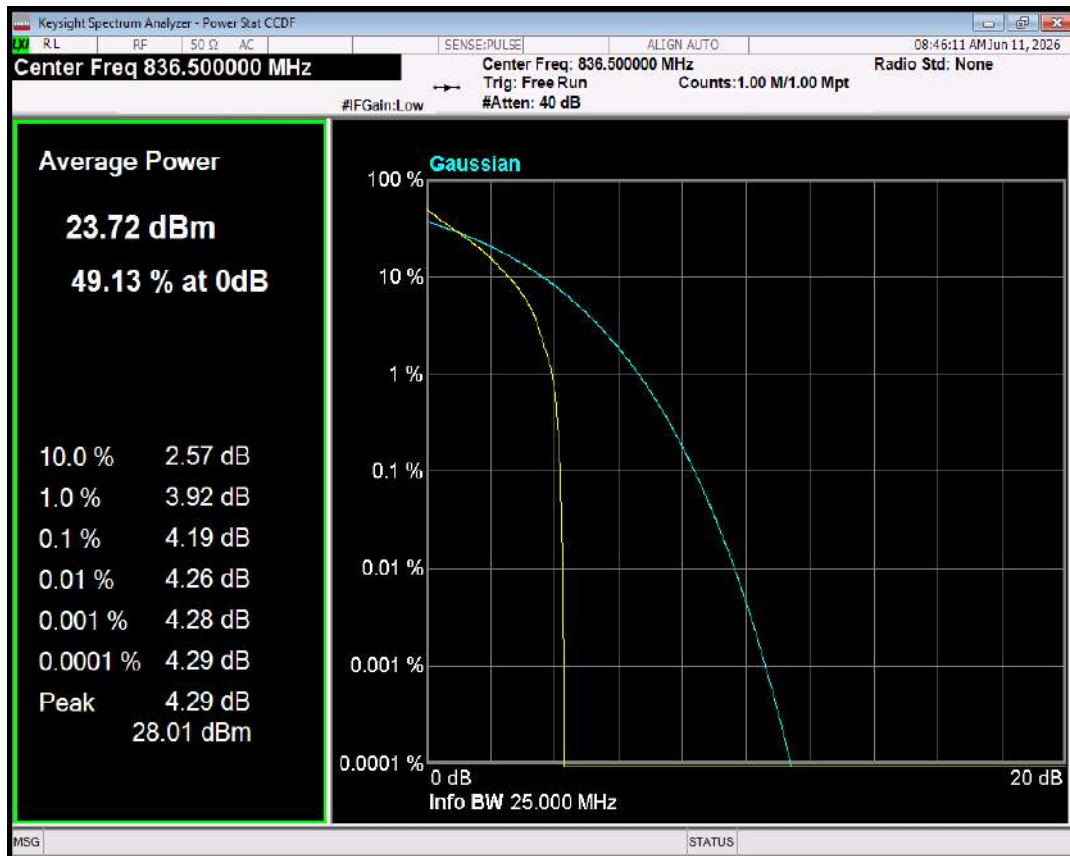
Band26(824-849) 16QAM BW=5MHz Channel=26915 RB Size=1 Position=#0
