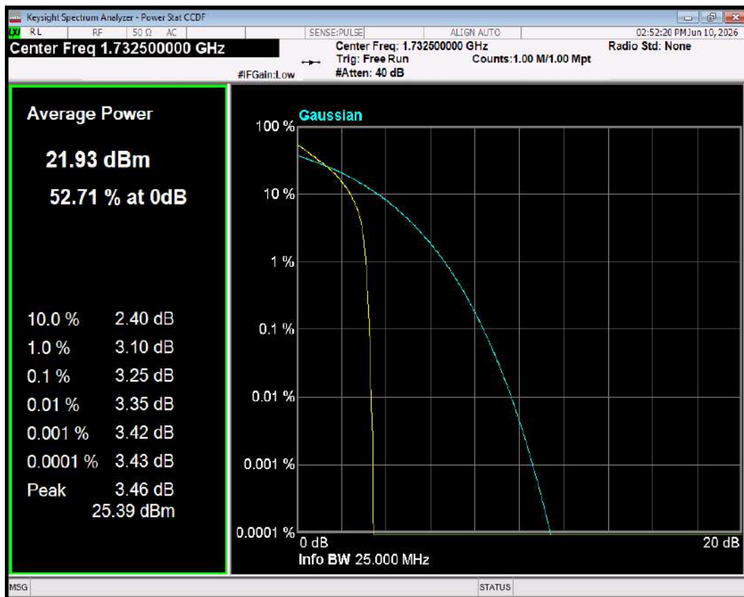
Band4 16QAM BW=1.4MHz Channel=20175 RB Size=1 Position=#0
