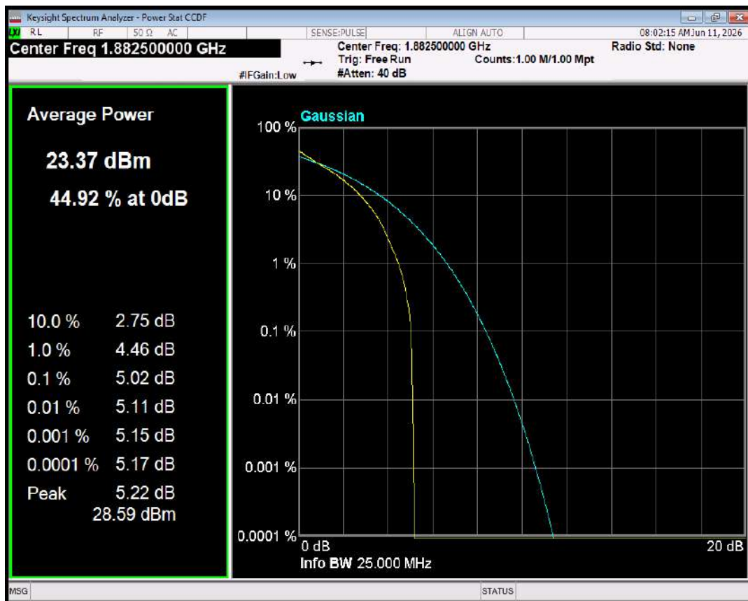
Band25 16QAM BW=3MHz Channel=26365 RB Size=1 Position=#0
