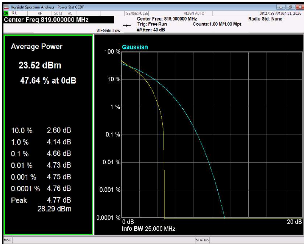
Band26(814-824) 16QAM BW=1.4MHz Channel=26740 RB Size=1 Position=#0
