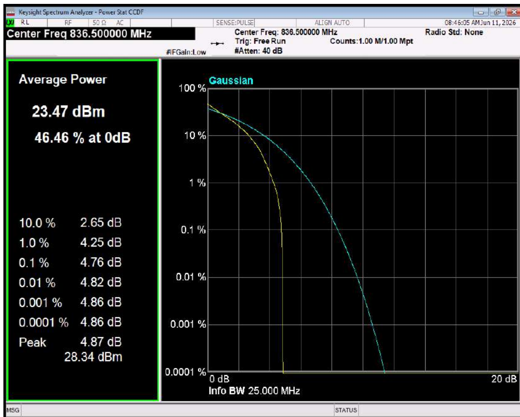
Band26(824-849) 16QAM BW=3MHz Channel=26915 RB Size=1 Position=#0
