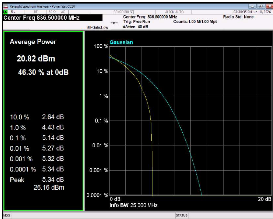
Band5 16QAM BW=1.4MHz Channel=20525 RB Size=1 Position=#0
