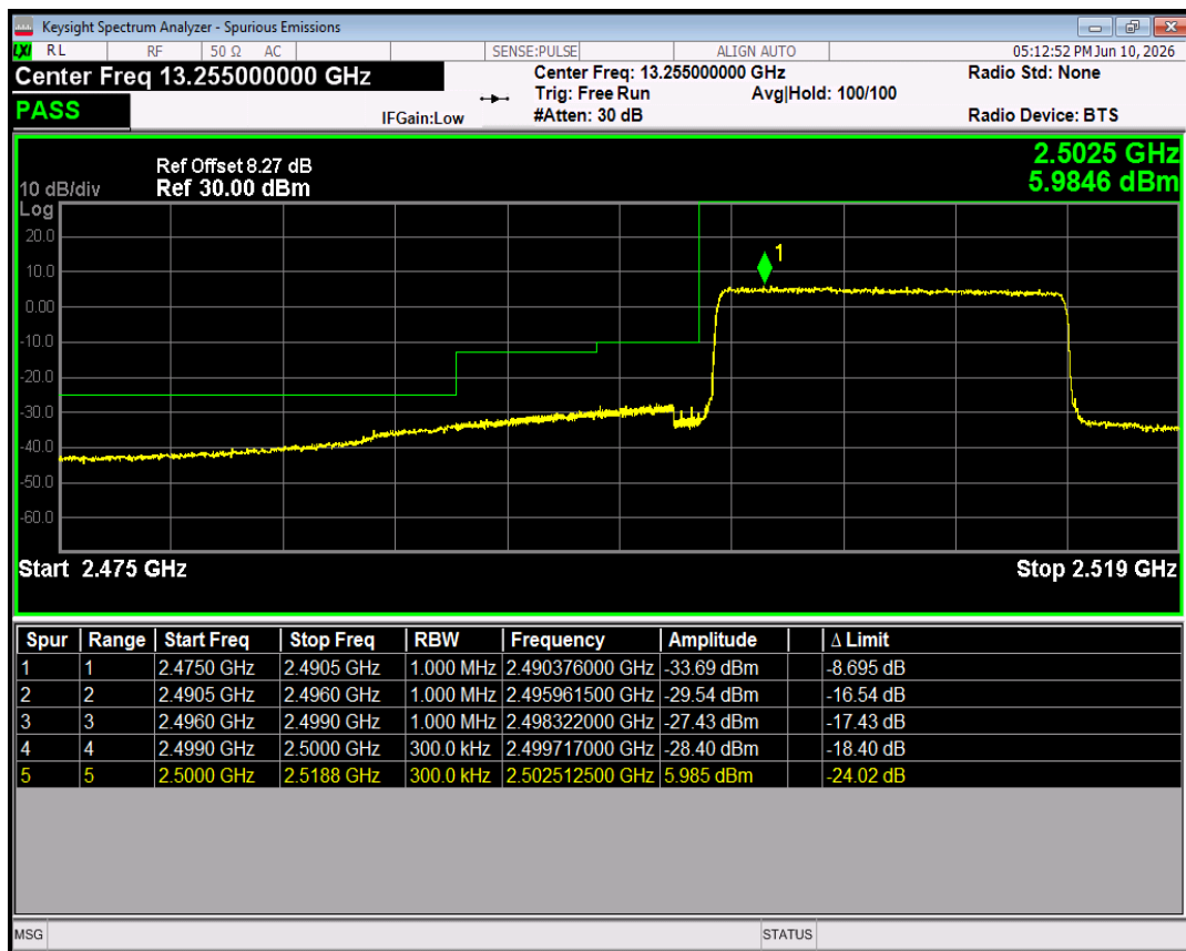
Band7 QPSK BW=15MHz Channel=21375 RB Size=1 Position=#0
