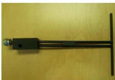
Figure 1 – MVG COMOSAR Validation Dipole
