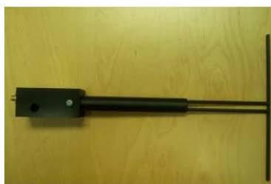
Figure 1 – MVG COMOSAR Validation Dipole
