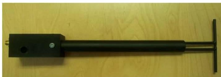
Figure 1 – MVG COMOSAR Validation Dipole
