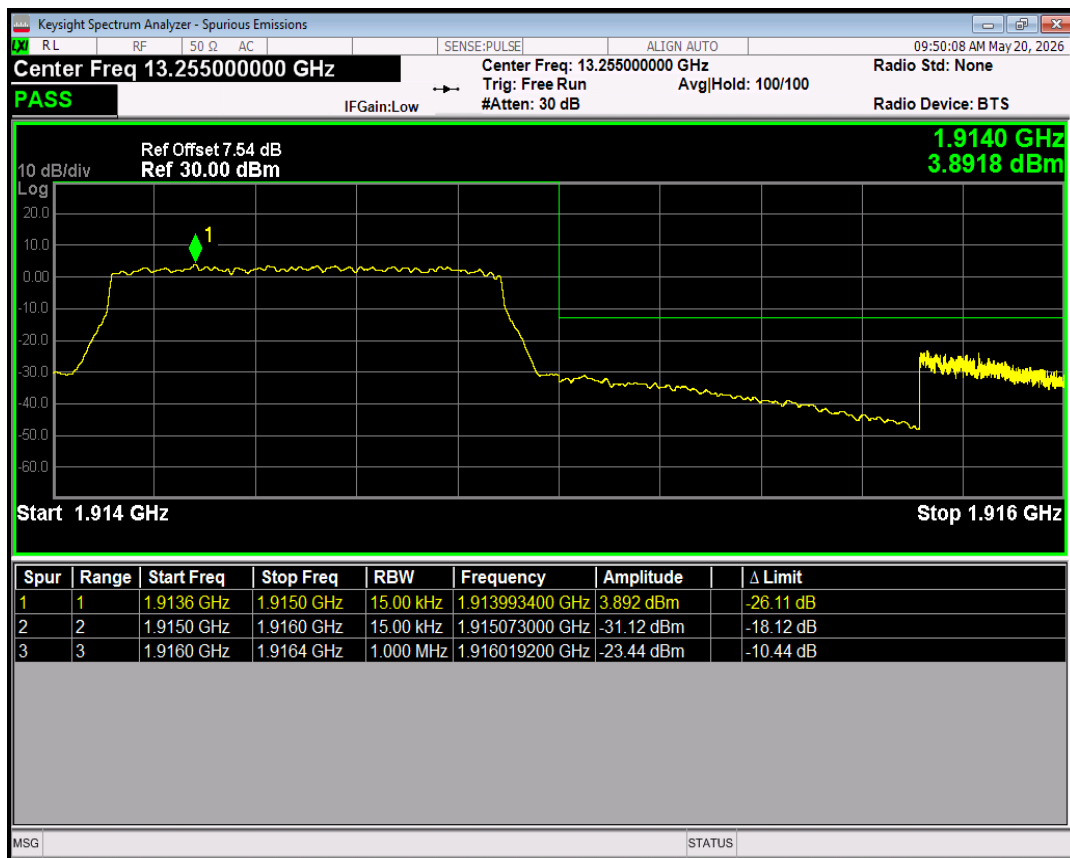
Band25 16QAM BW=1.4MHz Channel=26683 RB Size=1 Position=#Max
