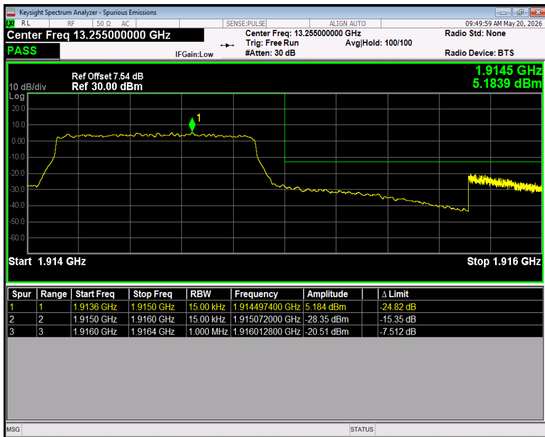
Band25 16QAM BW=1.4MHz Channel=26683 RB Size=1 Position=#0
