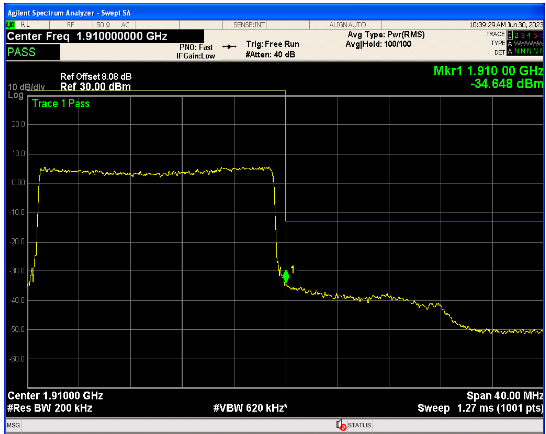
Band2 16QAM BW=20MHz Channel=19100 RB Size=1 Position=#Max
