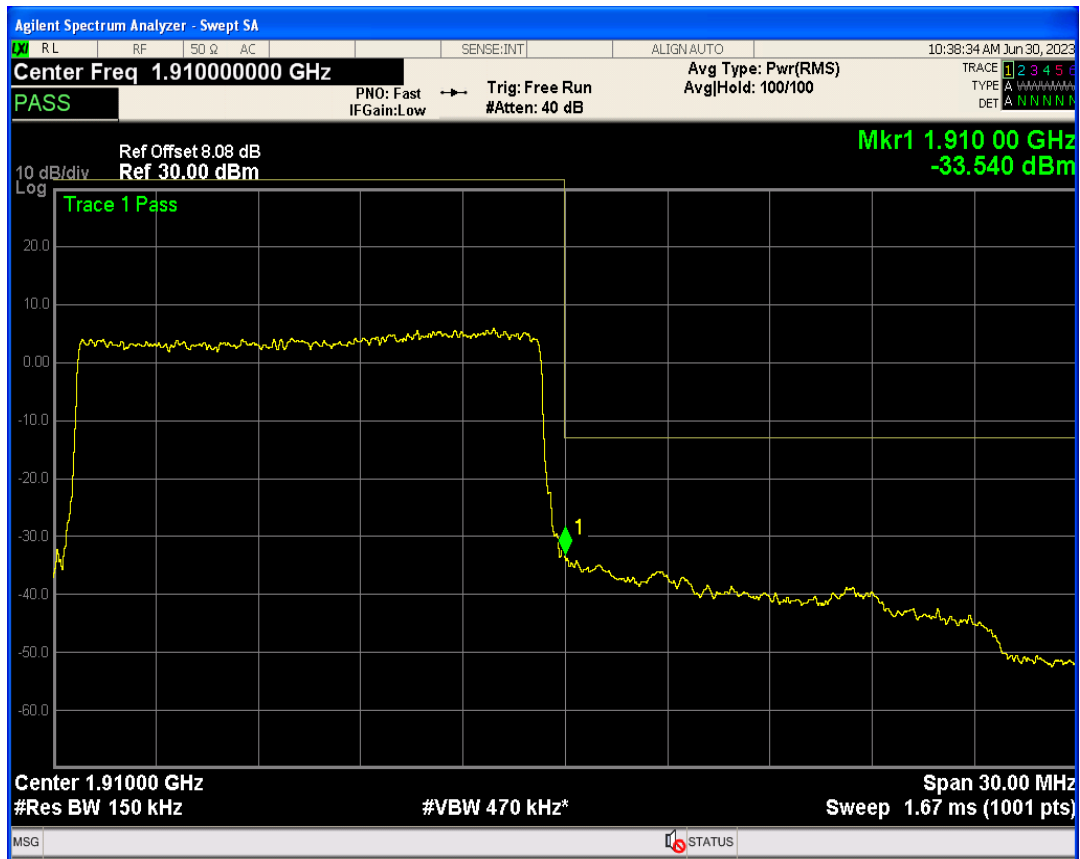
Band2 16QAM BW=15MHz Channel=19125 RB Size=1 Position=#Max
