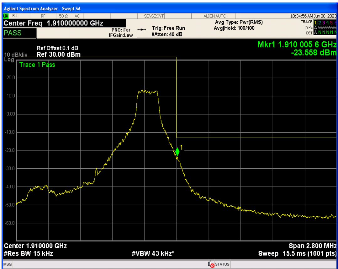
Band2 16QAM BW=1.4MHz Channel=19193 RB Size=6 Position=#0
