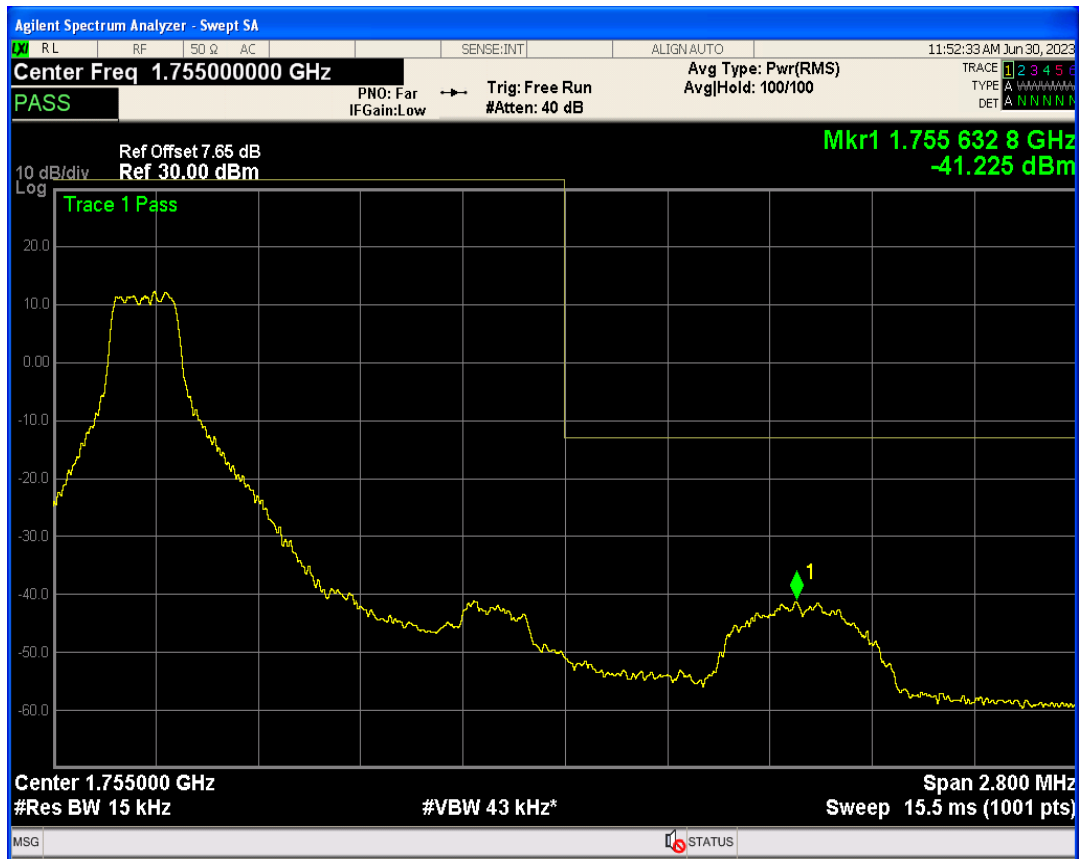
Band4 16QAM BW=1.4MHz Channel=20393 RB Size=1 Position=#Max
