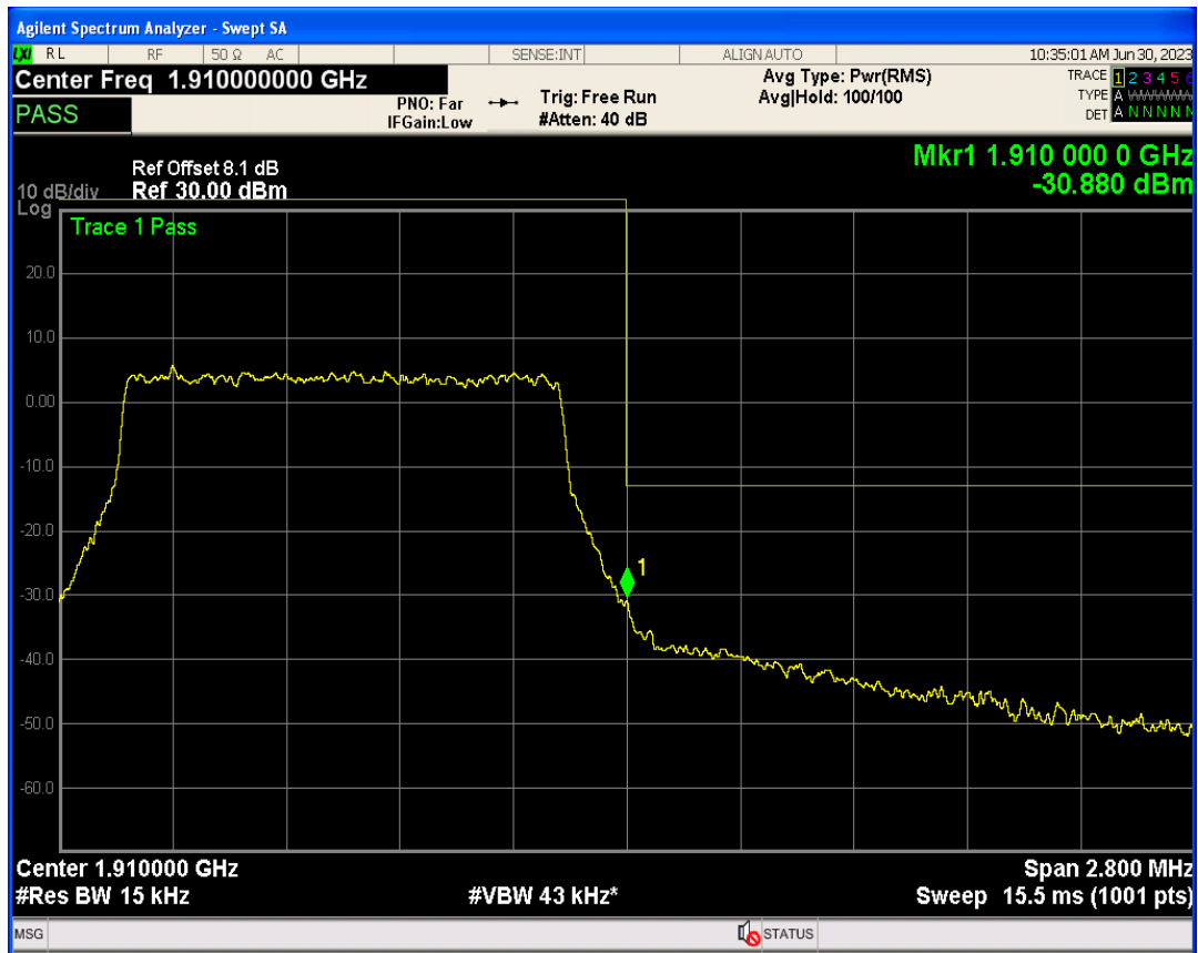
Band2 QPSK BW=3MHz Channel=18615 RB Size=1 Position=#0
