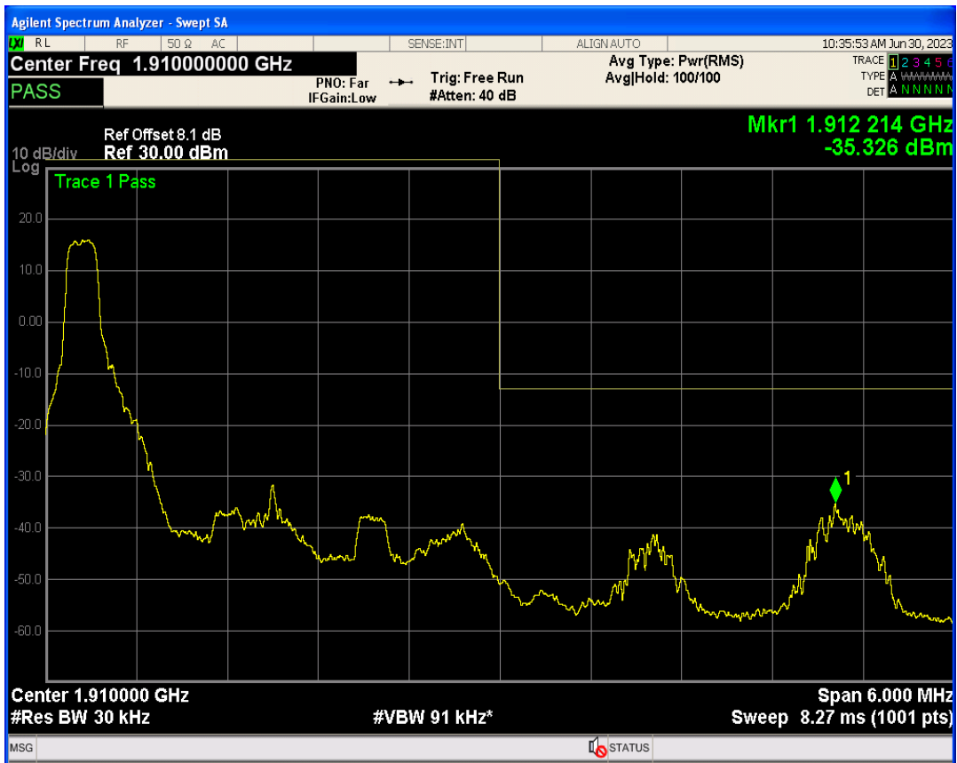
Band2 16QAM BW=3MHz Channel=19185 RB Size=1 Position=#Max
