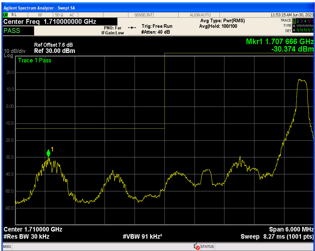
Band4 QPSK BW=3MHz Channel=20385 RB Size=1 Position=#0
