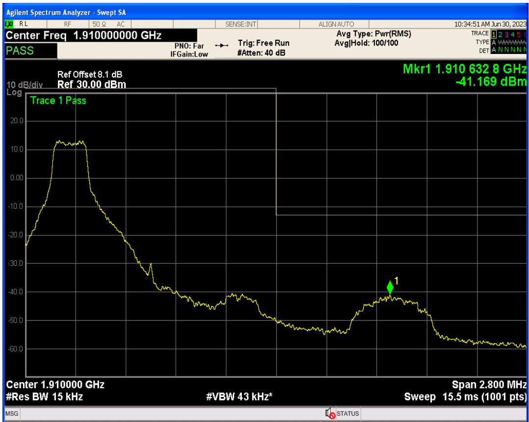
Band2 16QAM BW=1.4MHz Channel=19193 RB Size=1 Position=#Max
