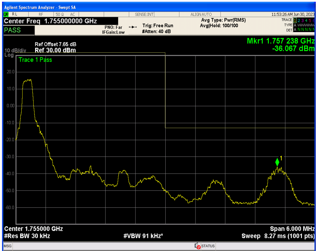
Band4 16QAM BW=3MHz Channel=19965 RB Size=15 Position=#0
