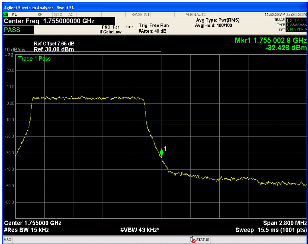
Band4 16QAM BW=1.4MHz Channel=20393 RB Size=1 Position=#0
