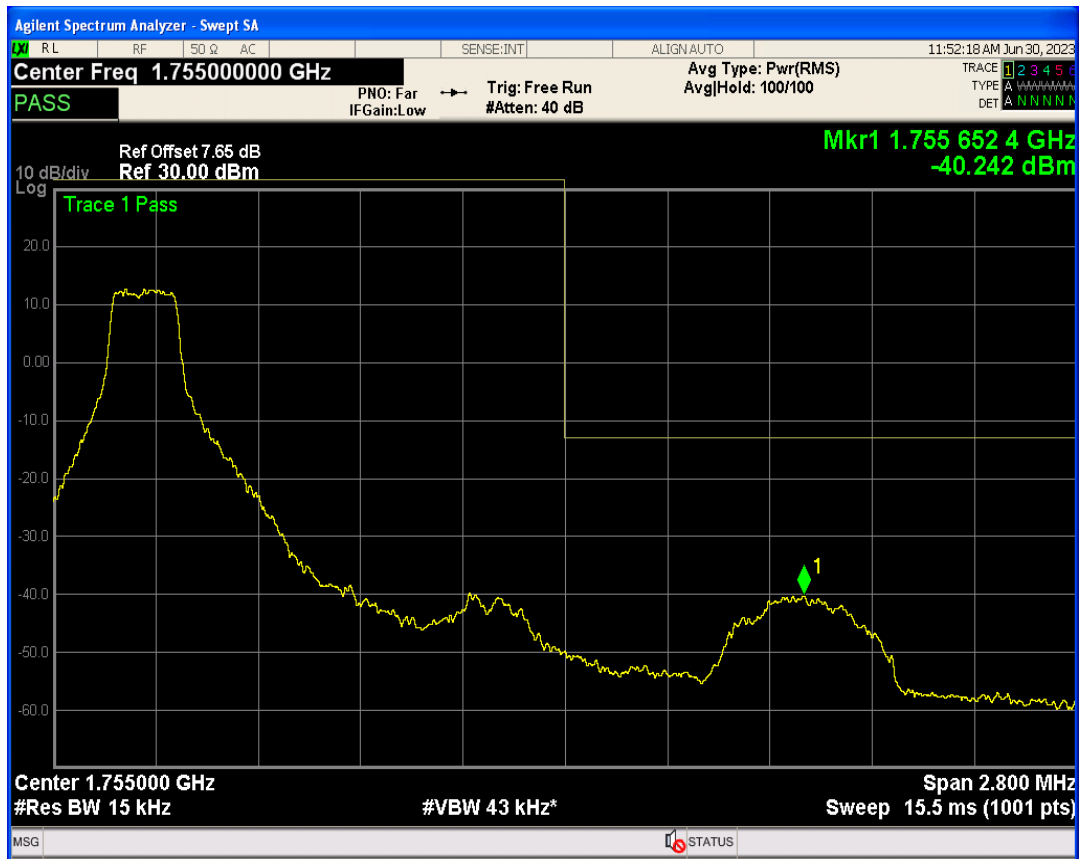
Band4 16QAM BW=1.4MHz Channel=19957 RB Size=6 Position=#0
