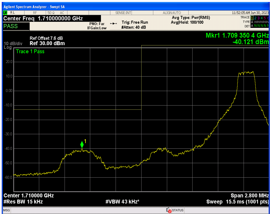
Band4 QPSK BW=1.4MHz Channel=20393 RB Size=1 Position=#0
