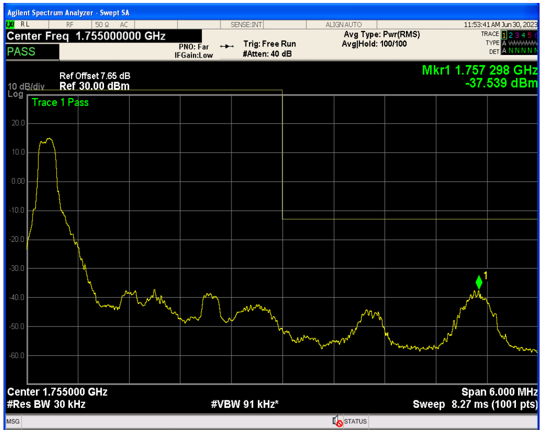
Band4 16QAM BW=3MHz Channel=20385 RB Size=1 Position=#Max
