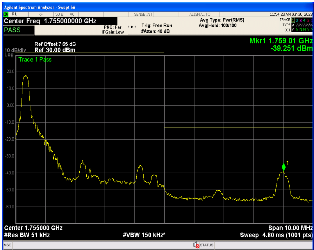
Band4 QPSK BW=5MHz Channel=20375 RB Size=25 Position=#0
