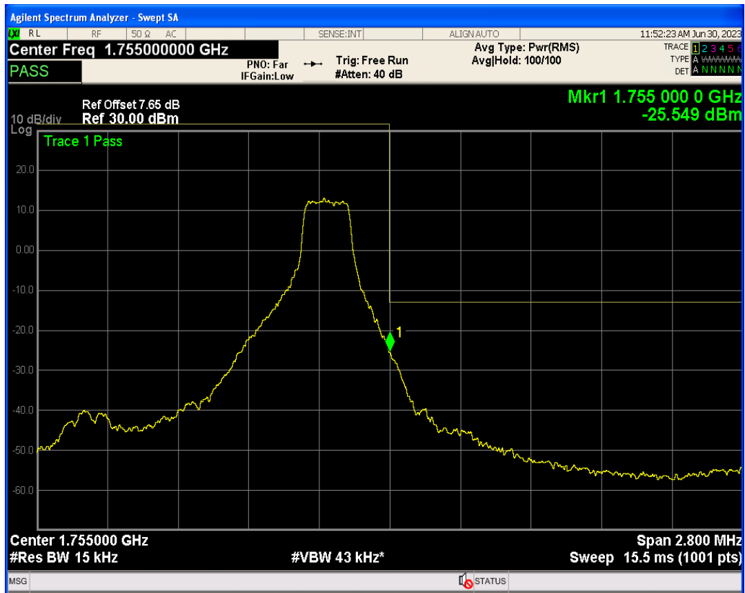
Band4 QPSK BW=1.4MHz Channel=20393 RB Size=6 Position=#0
