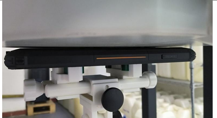
Right Side (Separation distance of 0mm)
