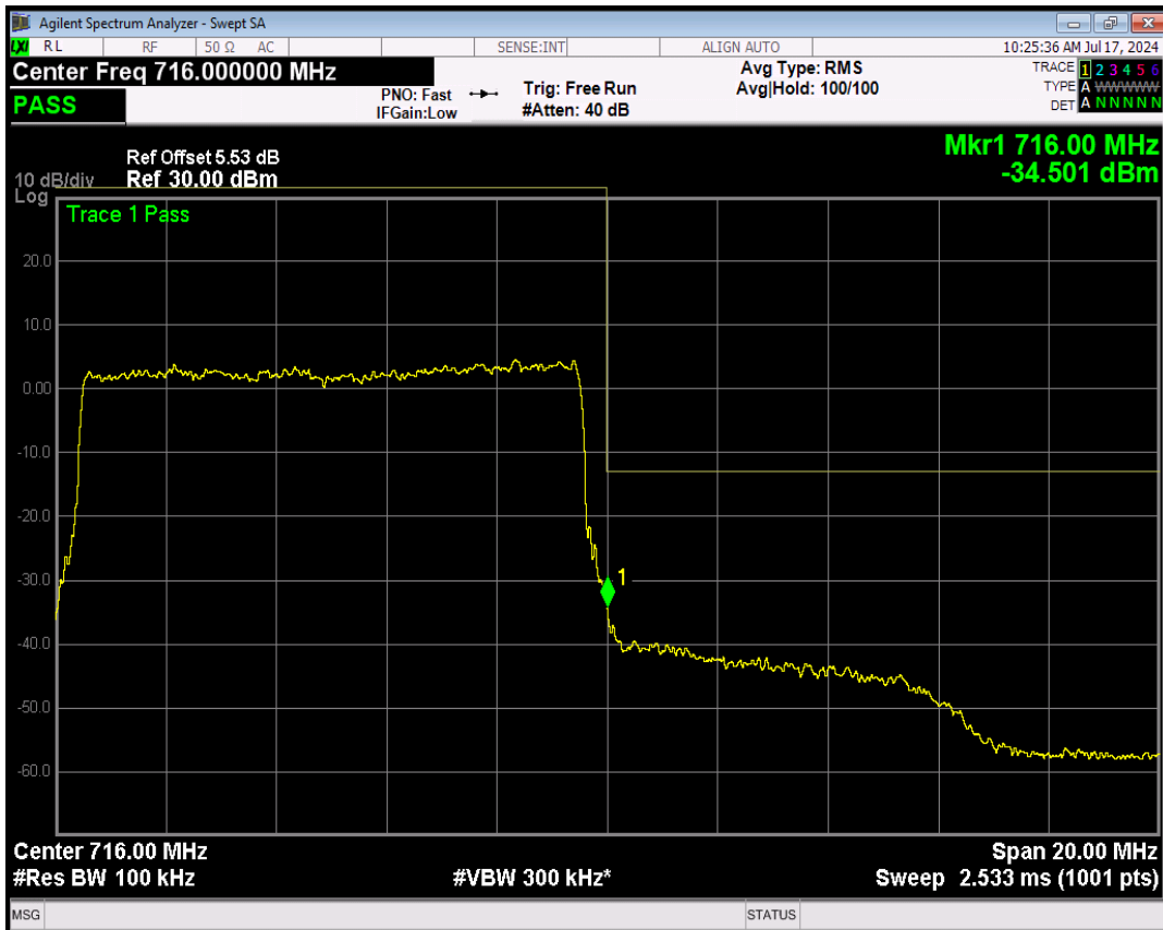
Band17 16QAM BW=10MHz Channel=23800 RB Size=50 Position=#0
