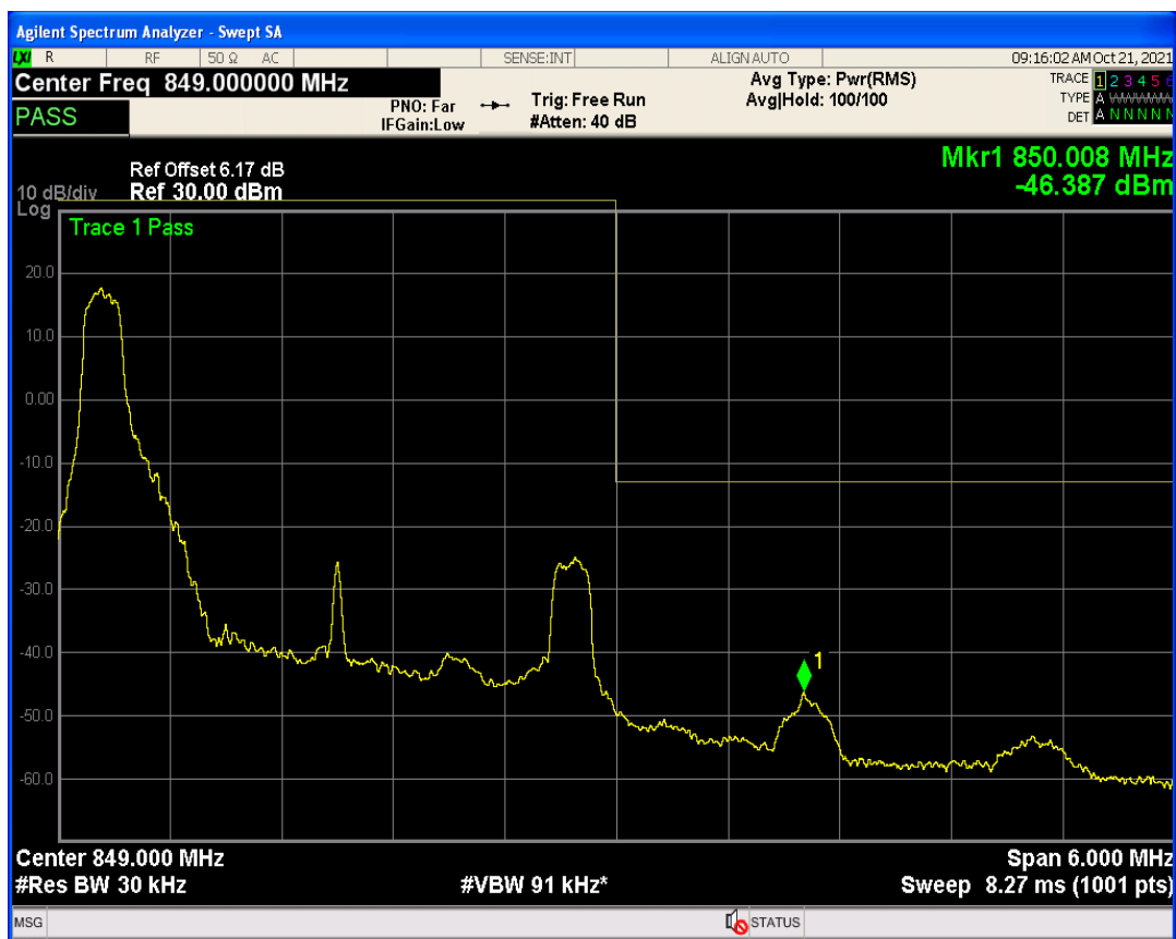
Band5 QPSK BW=3MHz Channel=20635 RB Size=15 Position=#0
