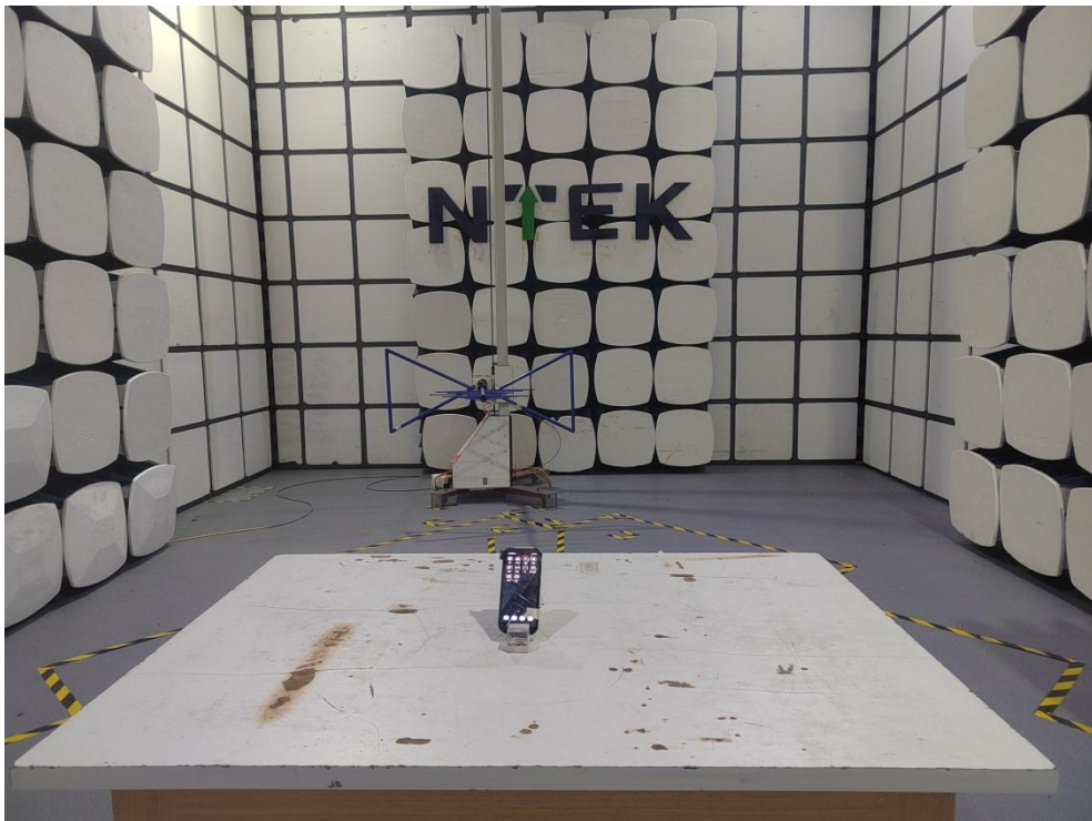
Radiated Measurement Photos(30MHz~1GHz )
