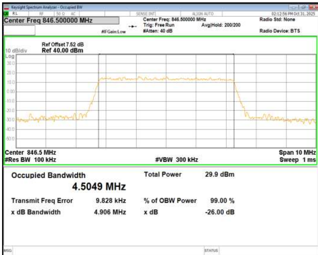
Band26(824-849) QPSK BW=1.4MHz Channel=26915 RB Size=6 Position=#0
