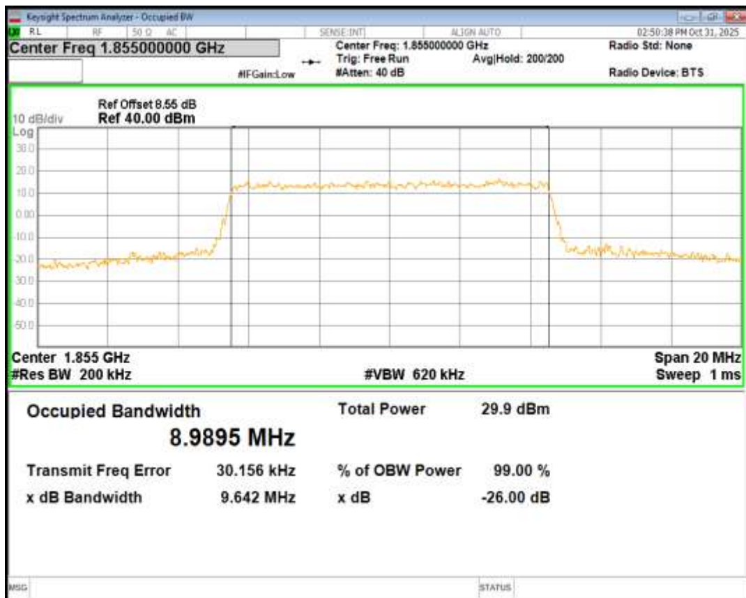
Band2 16QAM BW=10MHz Channel=18900 RB Size=50 Position=#0
