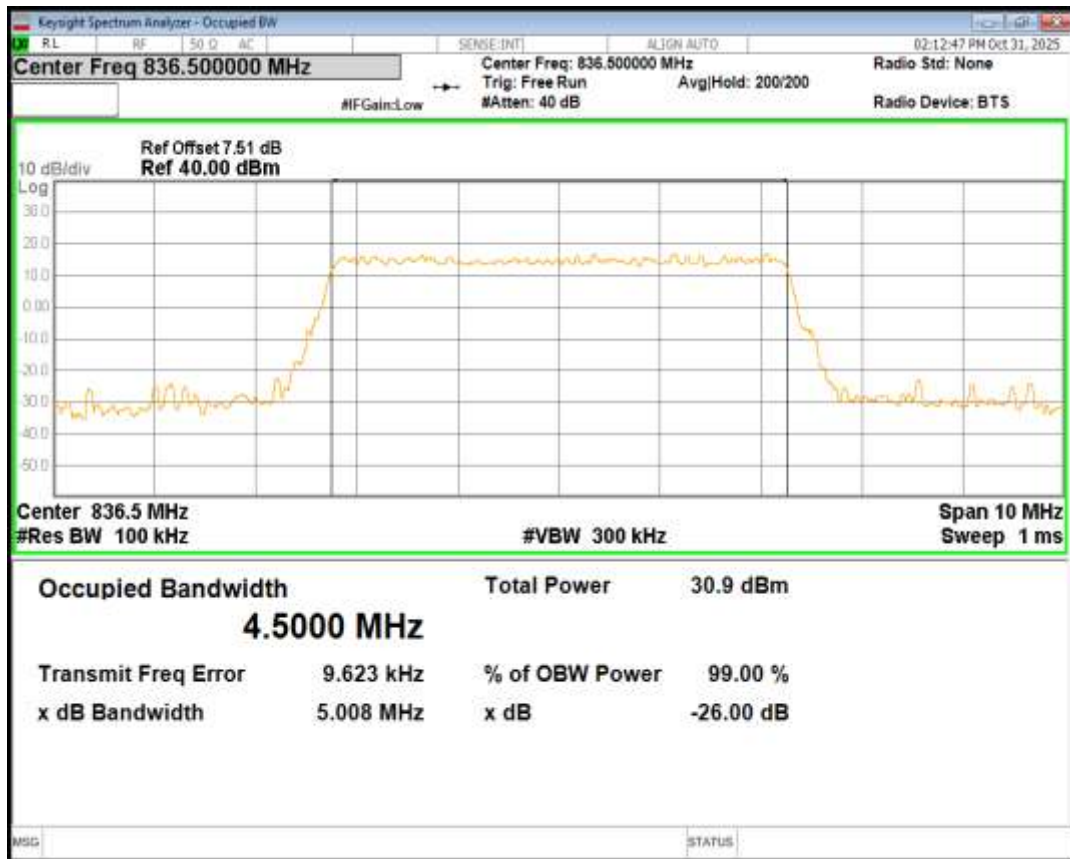
Band26(824-849) QPSK BW=5MHz Channel=27015 RB Size=25 Position=#0
