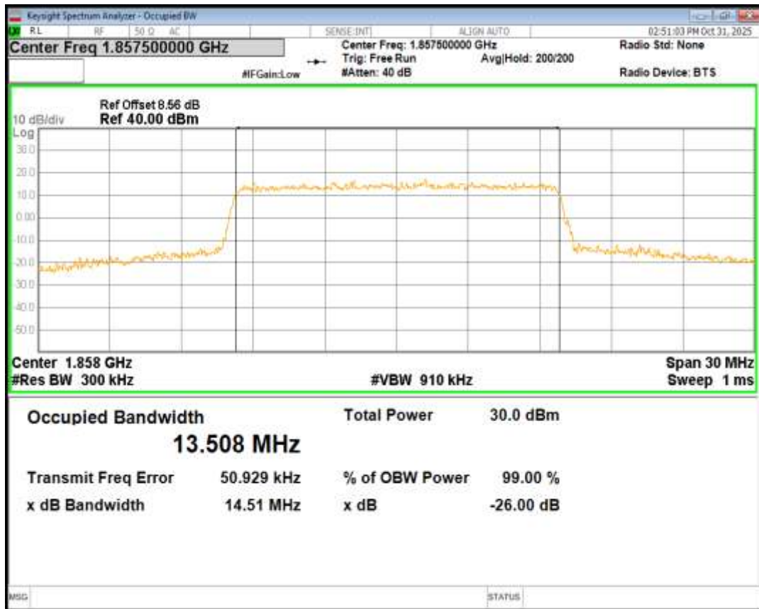
Band2 16QAM BW=15MHz Channel=18900 RB Size=75 Position=#0
