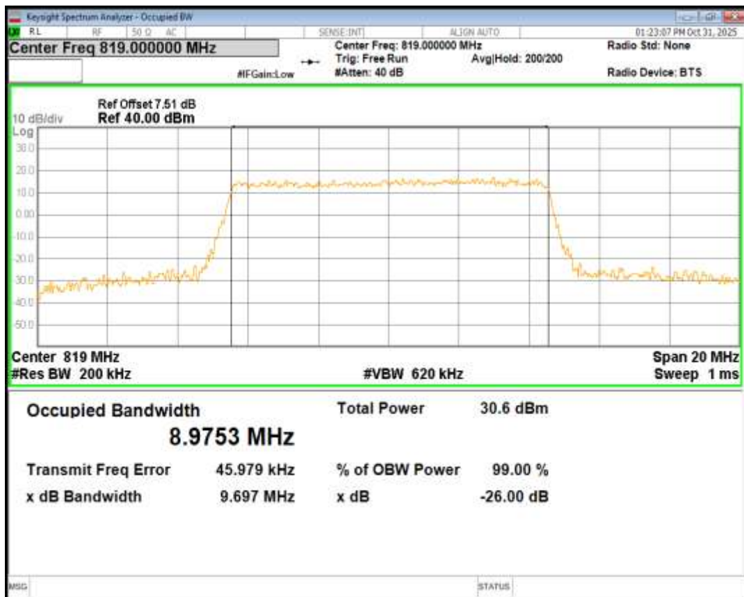
Band26(814-824) QPSK BW=3MHz Channel=26705 RB Size=15 Position=#0
