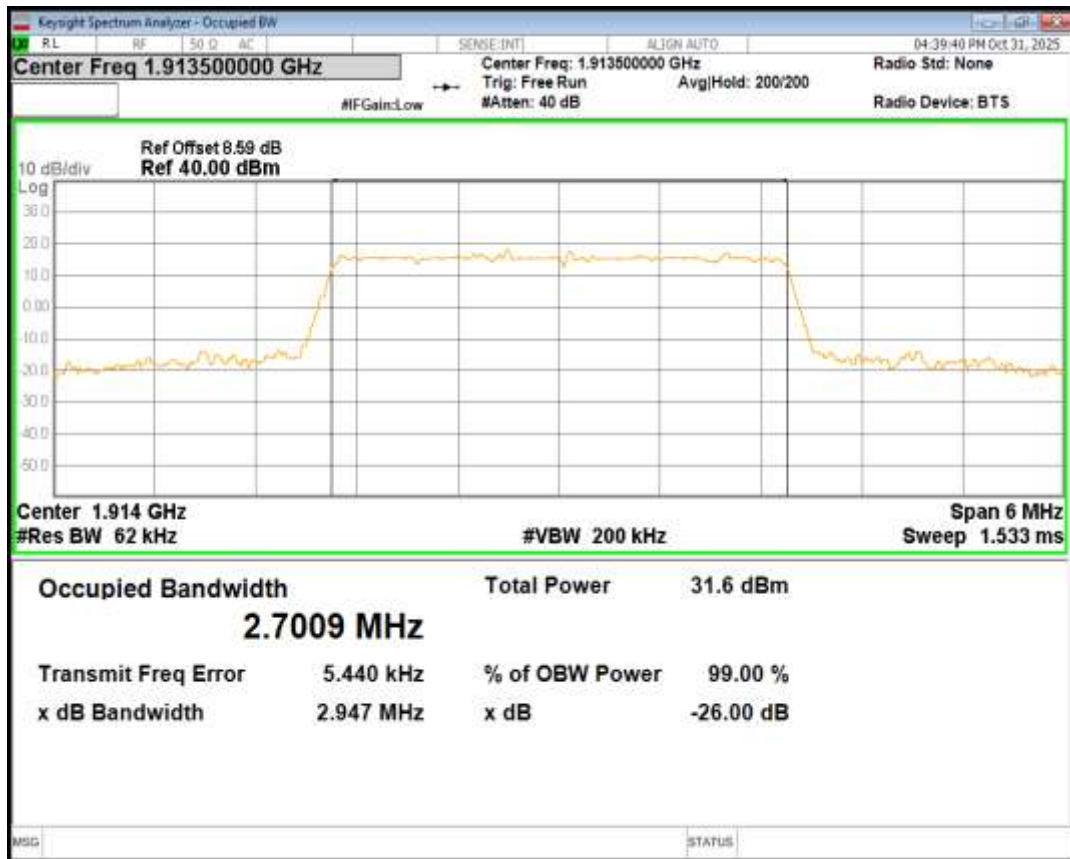
Band25 QPSK BW=5MHz Channel=26065 RB Size=25 Position=#0
