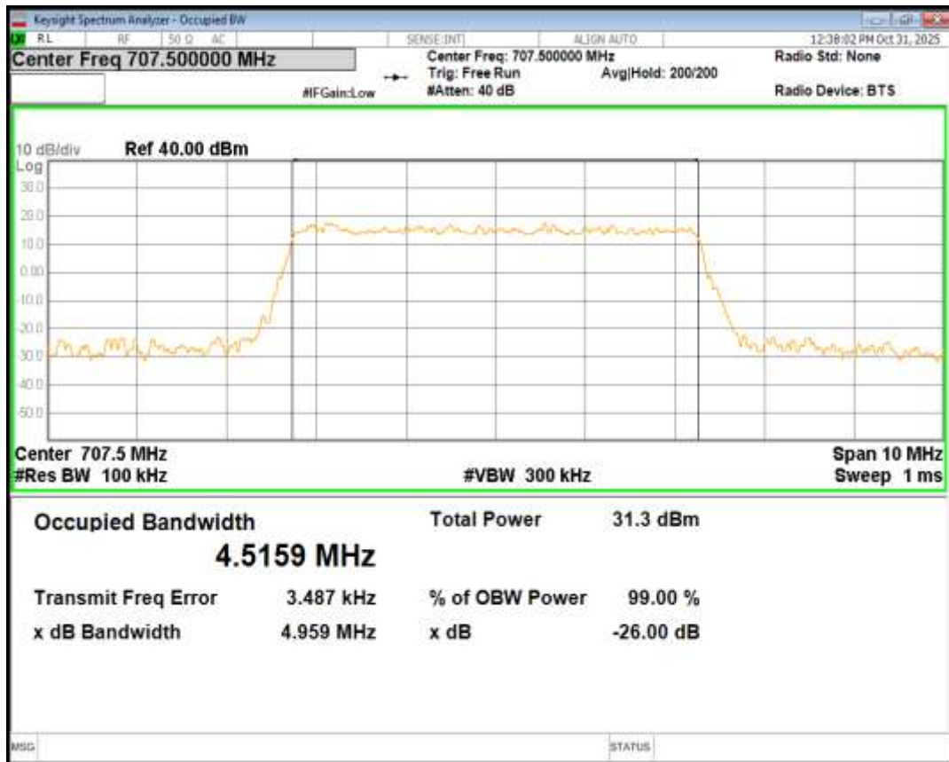
Band12 QPSK BW=5MHz Channel=23155 RB Size=25 Position=#0
