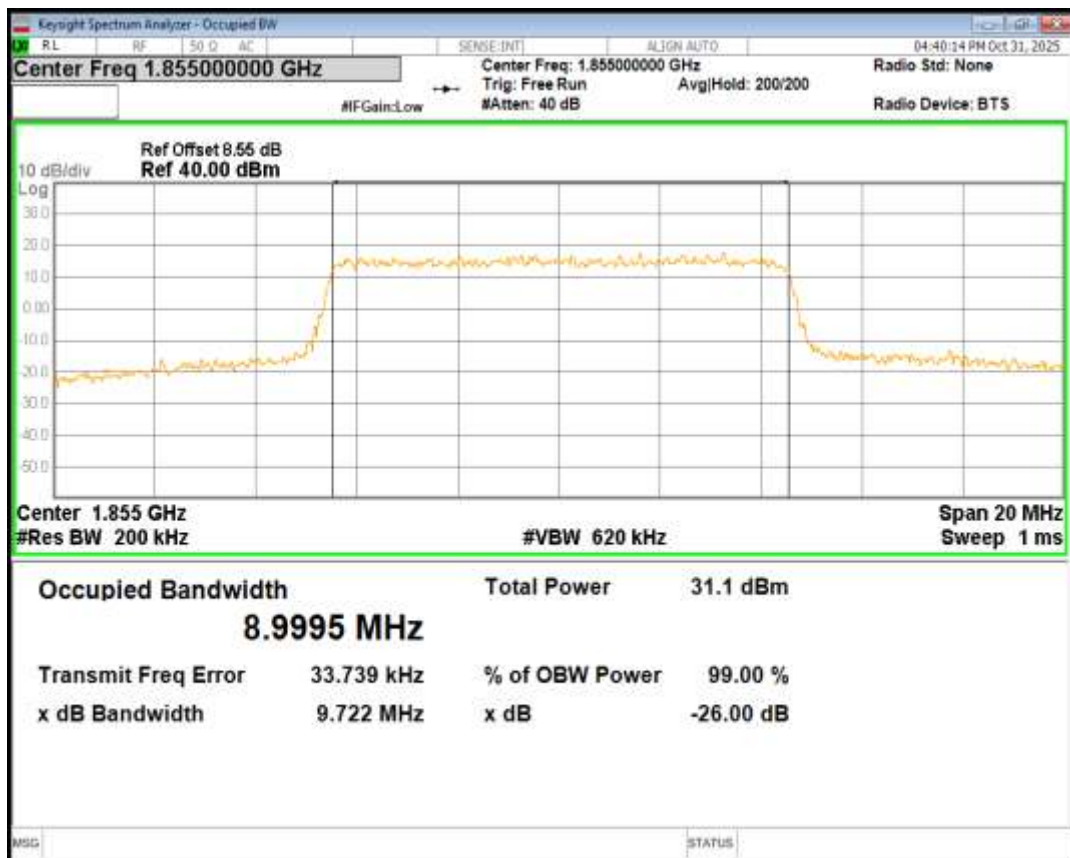
Band25 QPSK BW=10MHz Channel=26365 RB Size=50 Position=#0
