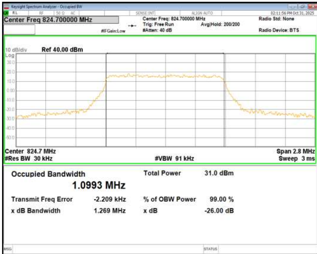
Band26(824-849) 16QAM BW=5MHz Channel=27015 RB Size=25 Position=#0
