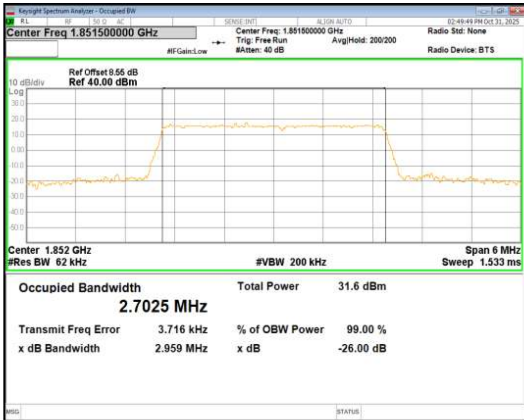
Band2 QPSK BW=3MHz Channel=18900 RB Size=15 Position=#0
