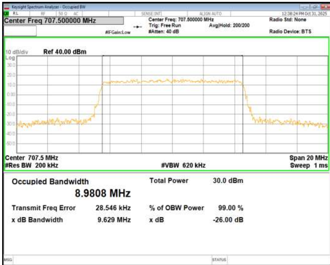
Band12 16QAM BW=10MHz Channel=23130 RB Size=50 Position=#0
