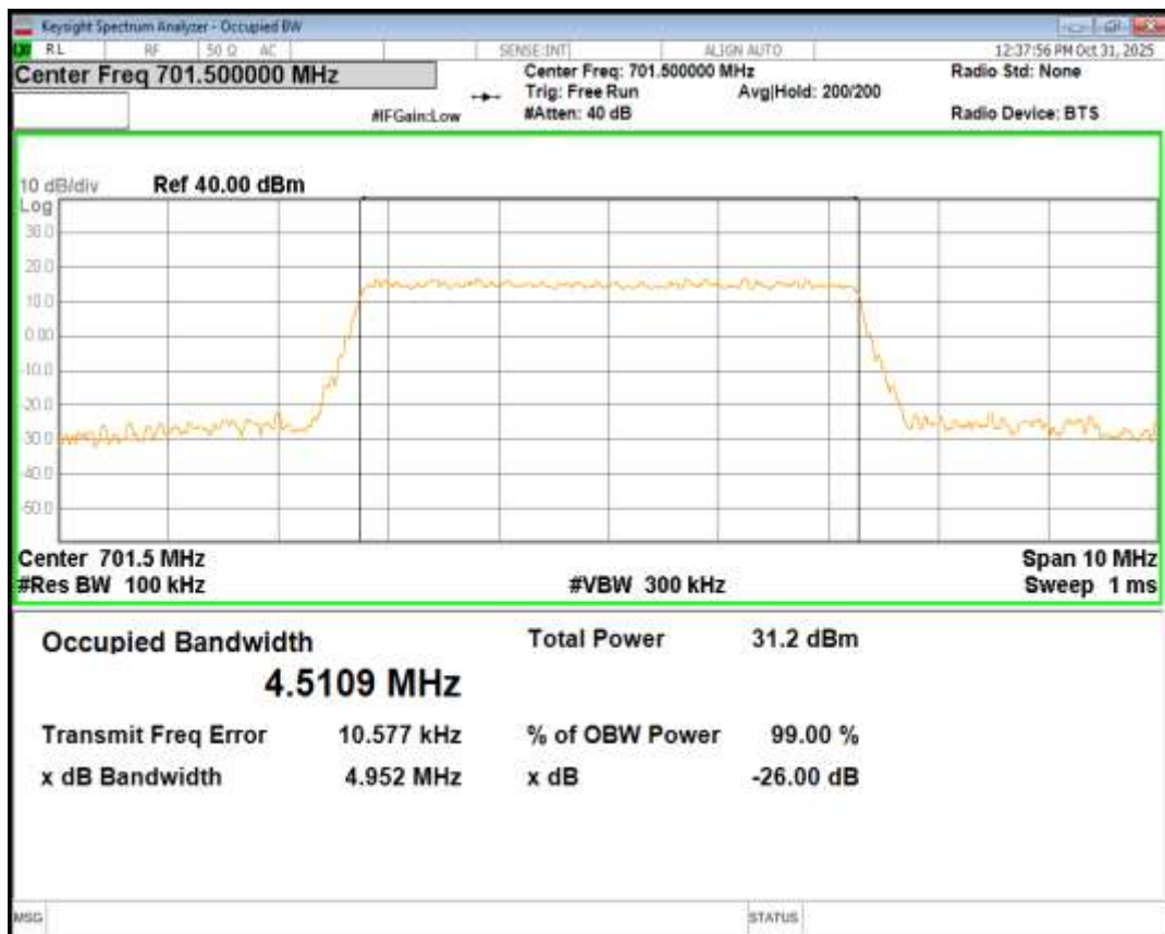
Band12 QPSK BW=5MHz Channel=23095 RB Size=25 Position=#0
