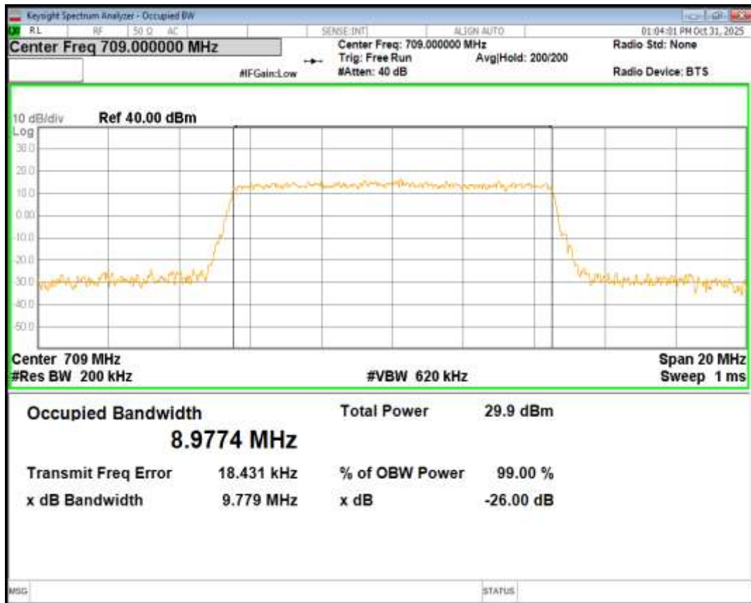
Band17 16QAM BW=10MHz Channel=23790 RB Size=50 Position=#0
