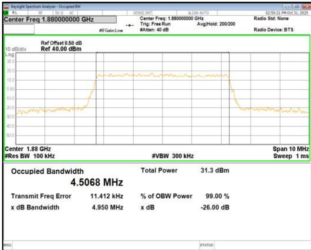
Band2 QPSK BW=5MHz Channel=19175 RB Size=25 Position=#0
