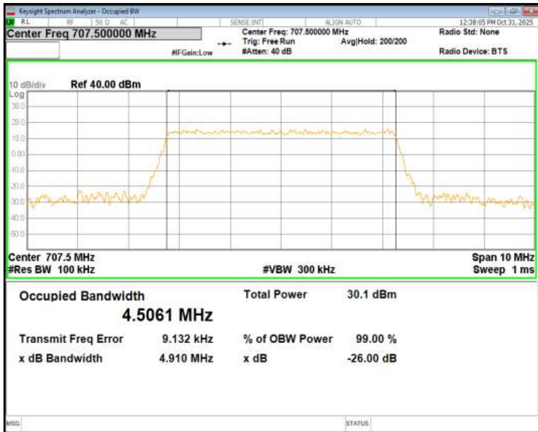
Band12 QPSK BW=1.4MHz Channel=23095 RB Size=6 Position=#0
