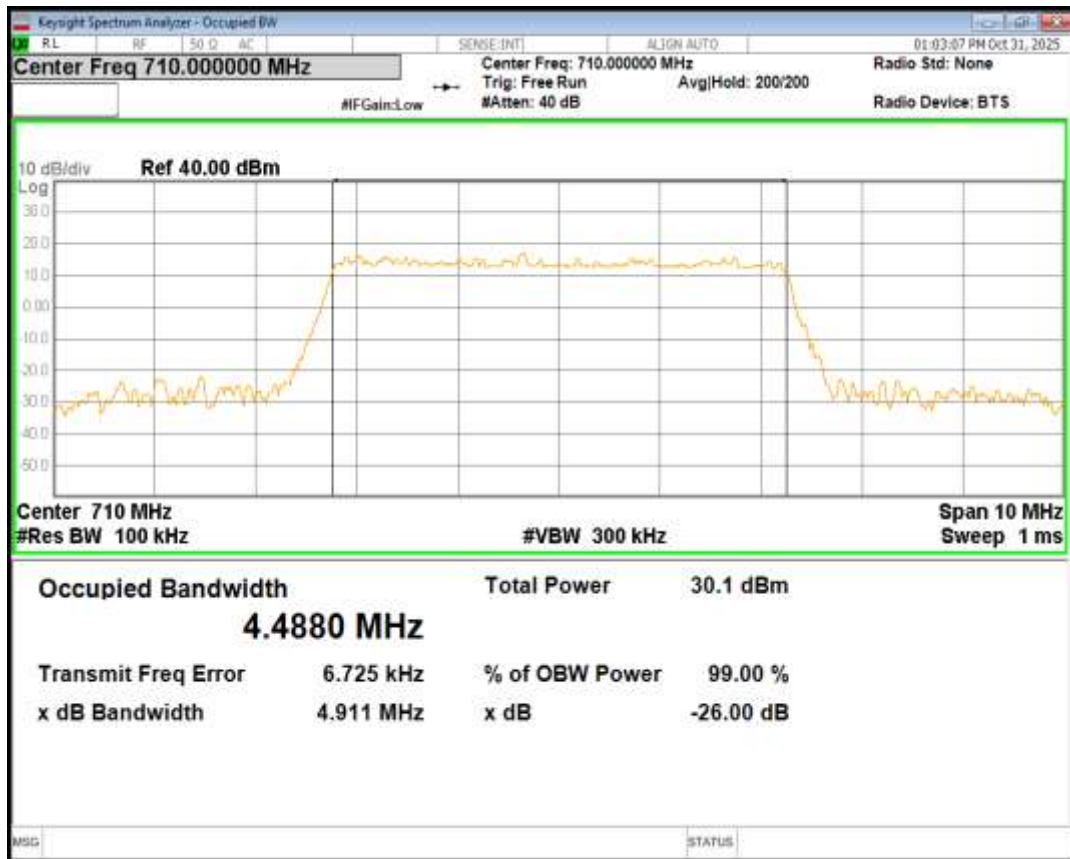
Band17 16QAM BW=5MHz Channel=23825 RB Size=25 Position=#0
