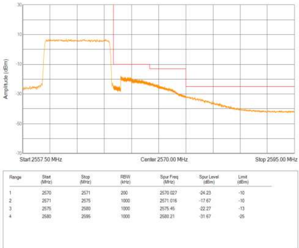
Band7 16QAM BW=15MHz Channel=20825 RB Size=75 Position=#0
