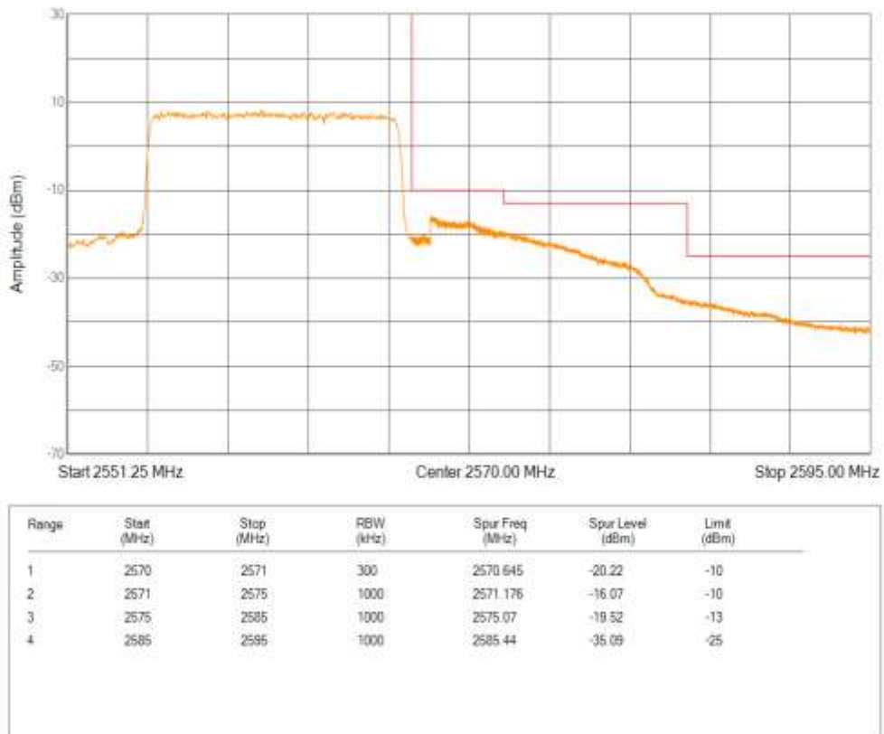
Band7 QPSK BW=20MHz Channel=20850 RB Size=100 Position=#0
