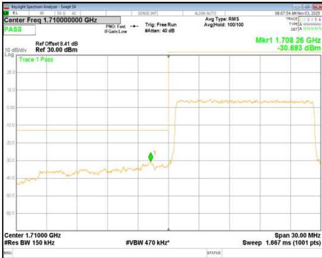
Band66 QPSK BW=15MHz Channel=132597 RB Size=75 Position=#0
