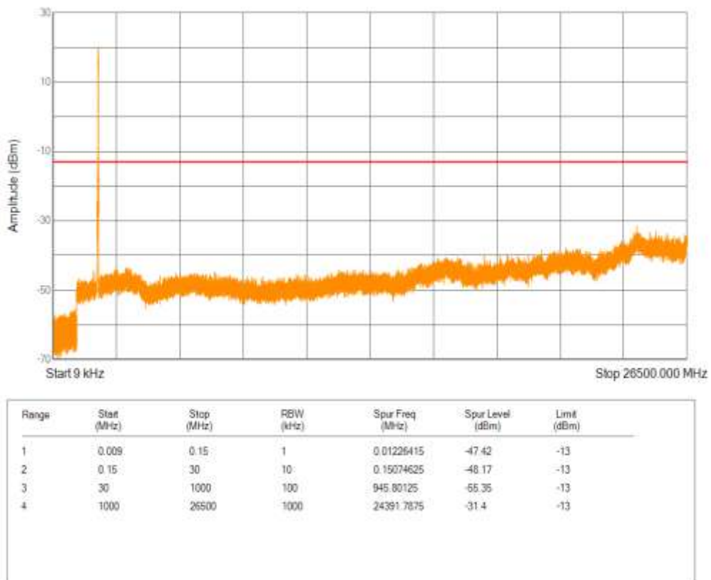
Band2 16QAM BW=3MHz Channel=18615 RB Size=15 Position=#0
