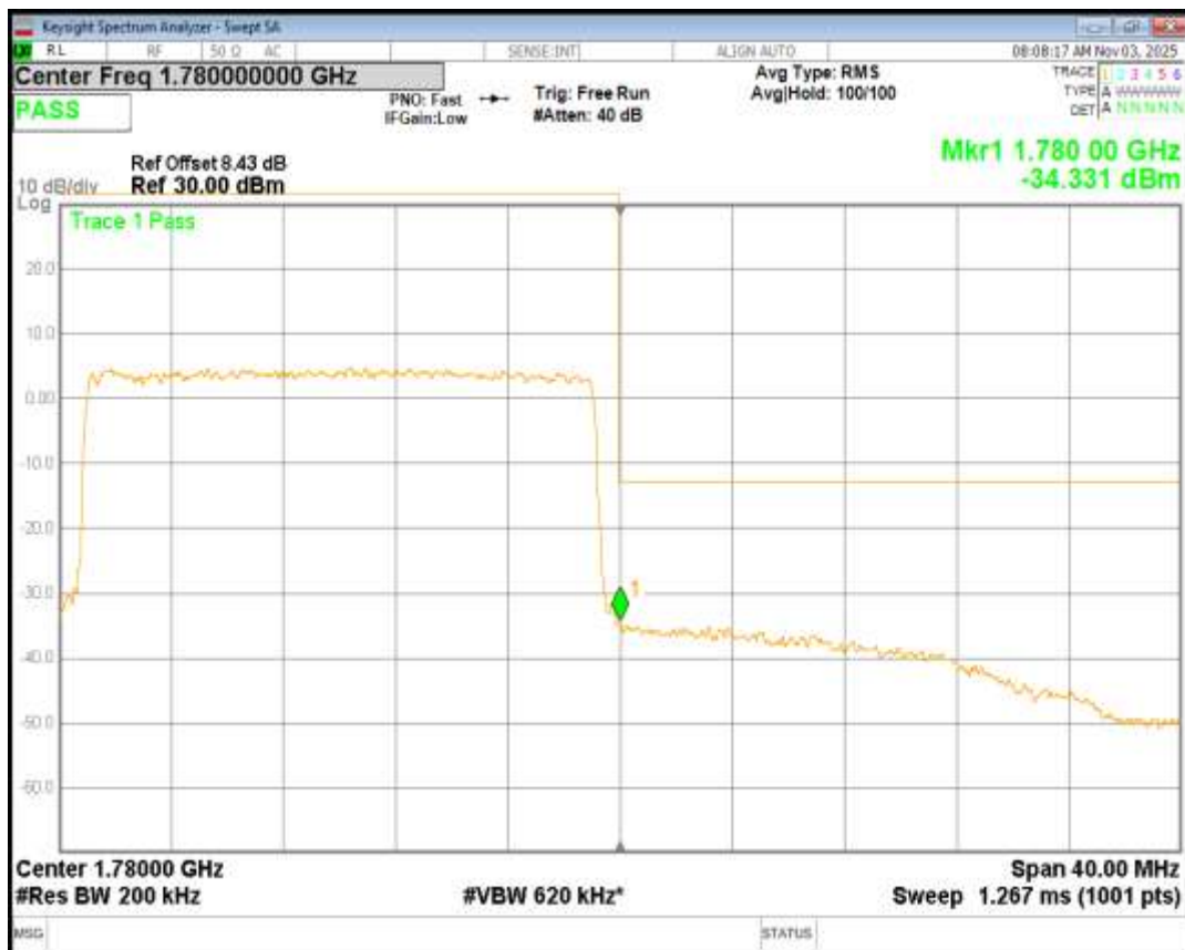
Band66 QPSK BW=3MHz Channel=131987 RB Size=15 Position=#0
