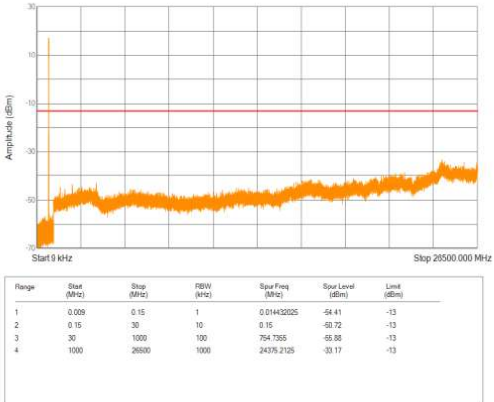
Band12 16QAM BW=5MHz Channel=23035 RB Size=25 Position=#0
