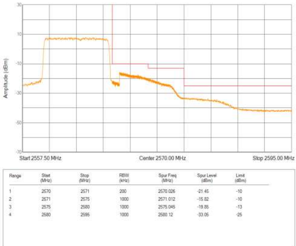
Band7 QPSK BW=15MHz Channel=20825 RB Size=75 Position=#0
