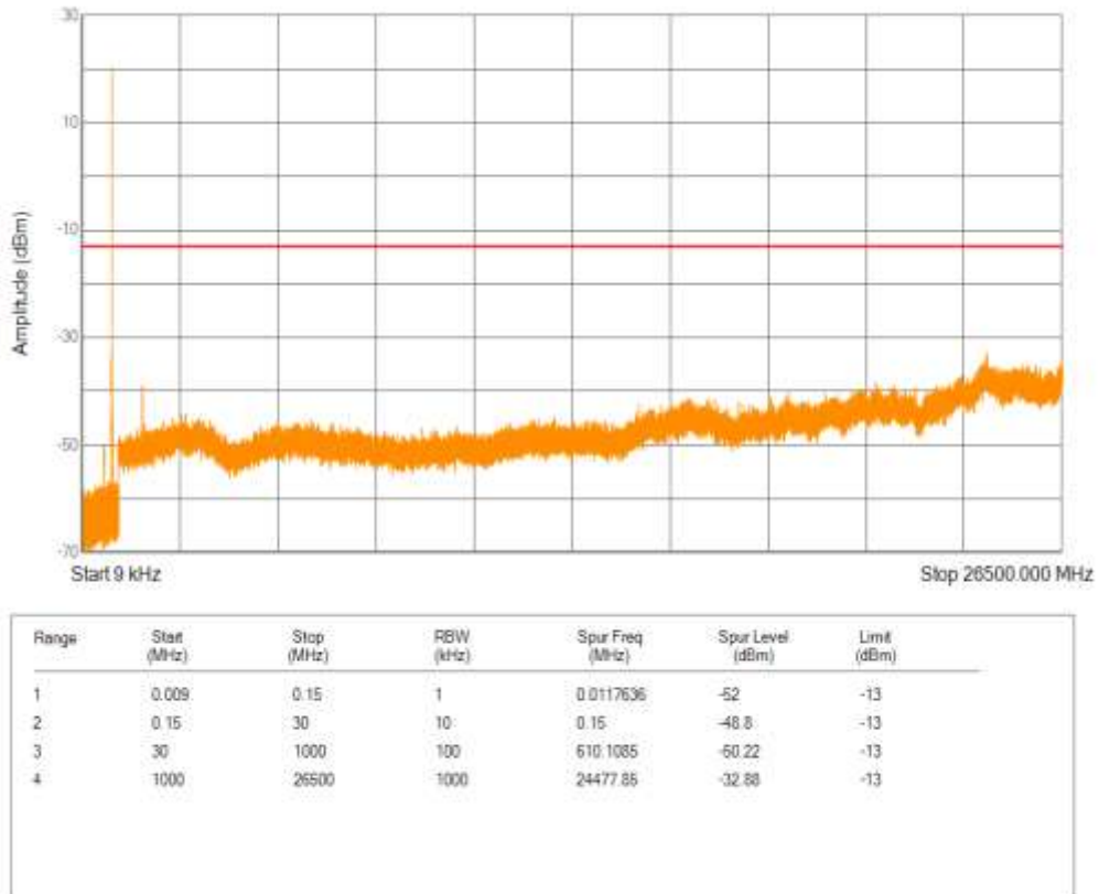
Band26(814-824) 16QAM BW=10MHz Channel=26740 RB Size=50 Position=#0
