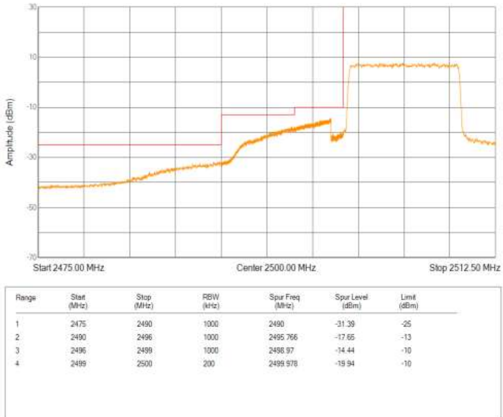
Band7 QPSK BW=10MHz Channel=21400 RB Size=50 Position=#0
