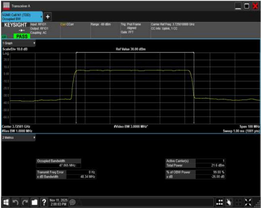
n78(3700-3800) SCS=30kHz DFT QPSK BW=50MHz Channel=651666 RB=128@0
