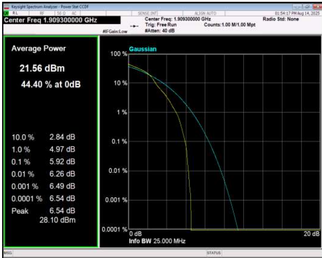
Band2 16QAM BW=10MHz Channel=18650 RB Size=1 Position=#0
