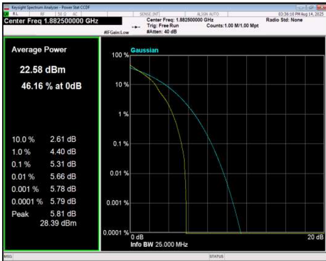
Band25 16QAM BW=5MHz Channel=26665 RB Size=1 Position=#0
