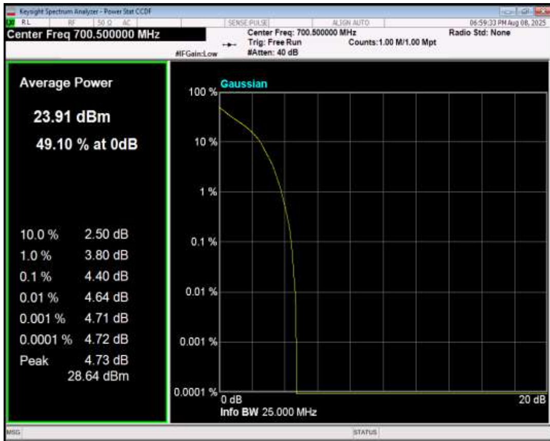
Band12 QPSK BW=3MHz Channel=23095 RB Size=1 Position=#0
