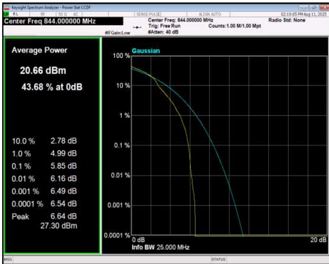
Band26(824-849) 16QAM BW=15MHz Channel=26865 RB Size=1 Position=#0
