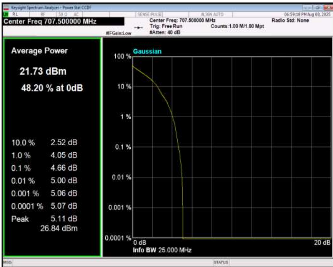
Band12 QPSK BW=10MHz Channel=23095 RB Size=1 Position=#0
