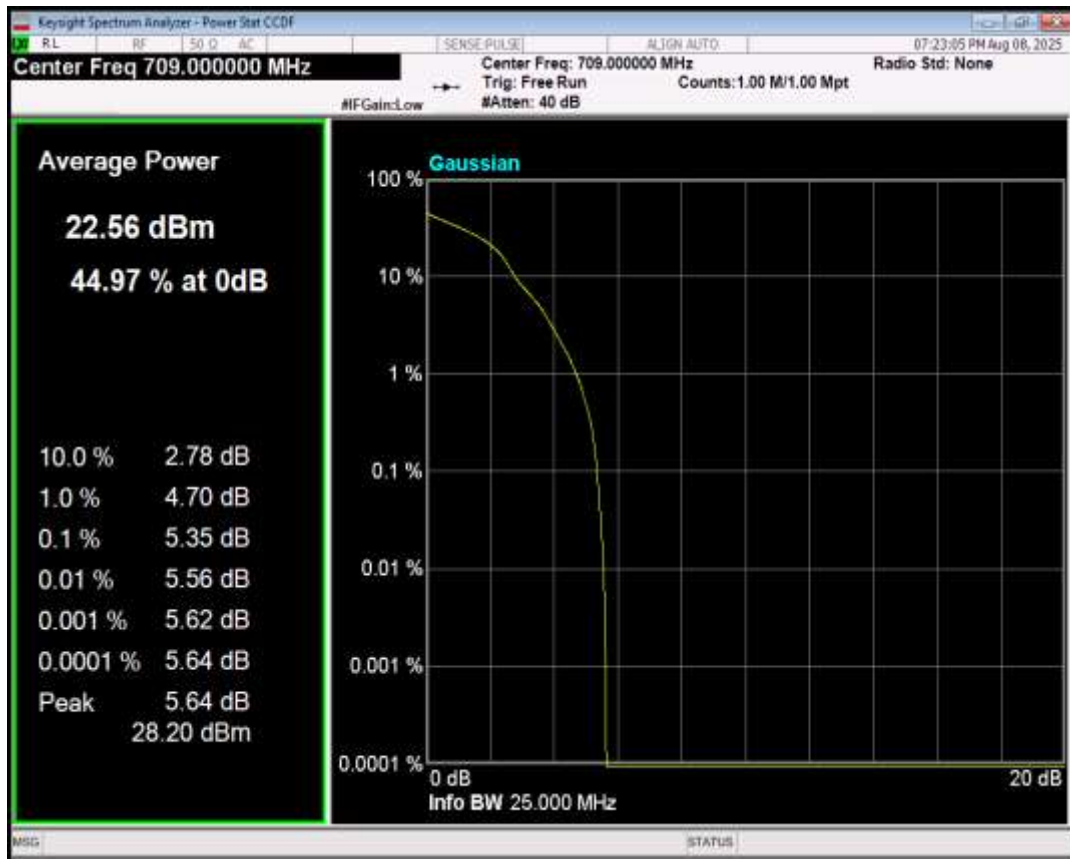
Band17 16QAM BW=10MHz Channel=23790 RB Size=1 Position=#0
