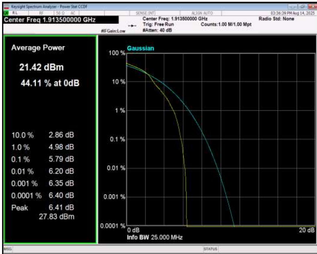
Band25 16QAM BW=5MHz Channel=26065 RB Size=1 Position=#0
