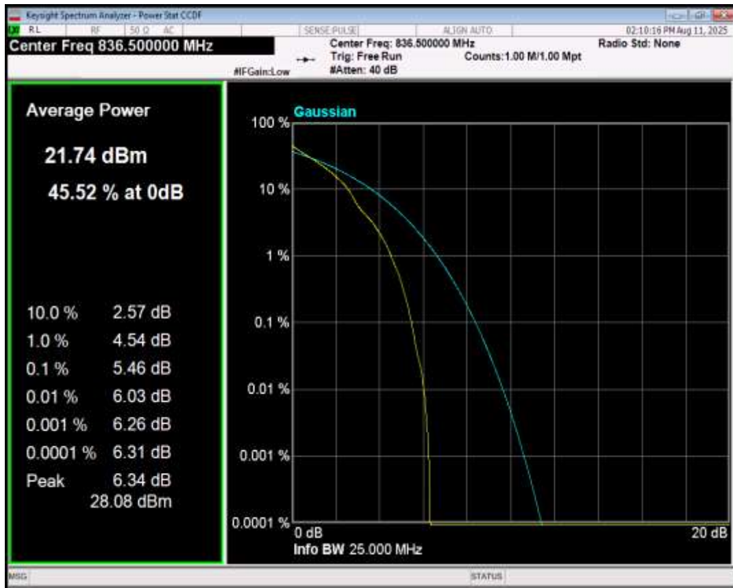
Band26(824-849) QPSK BW=15MHz Channel=26965 RB Size=1 Position=#0
