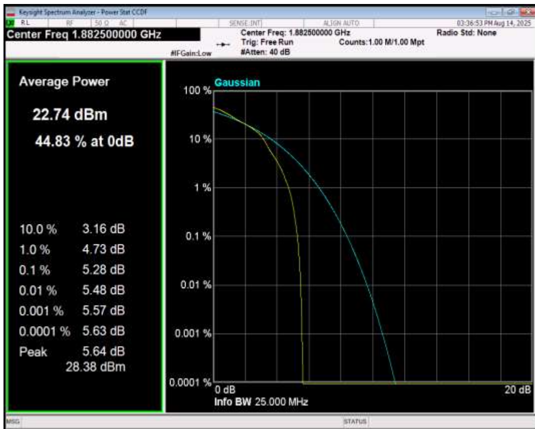
Band25 QPSK BW=1.4MHz Channel=26047 RB Size=1 Position=#0
