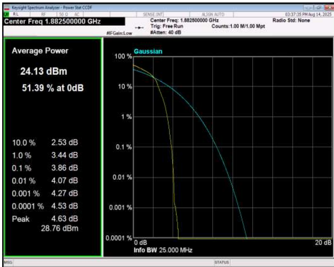
Band25 16QAM BW=15MHz Channel=26115 RB Size=1 Position=#0
