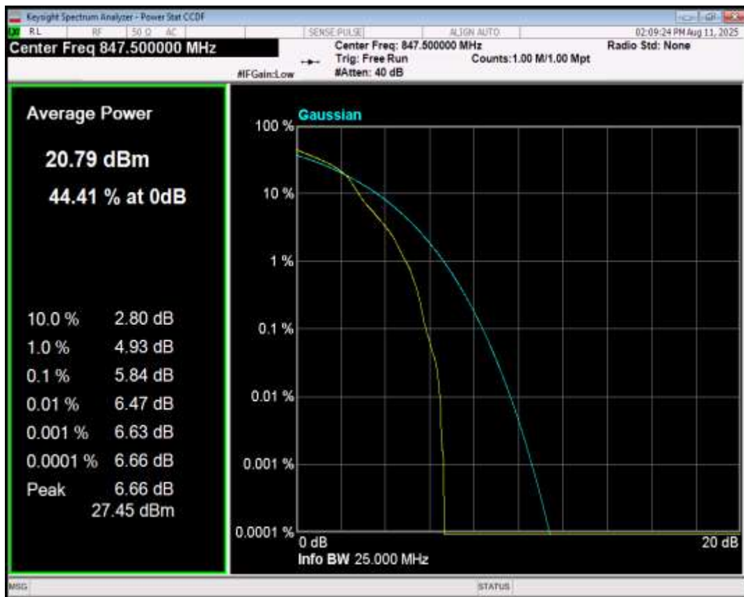
Band26(824-849) 16QAM BW=5MHz Channel=26815 RB Size=1 Position=#0
