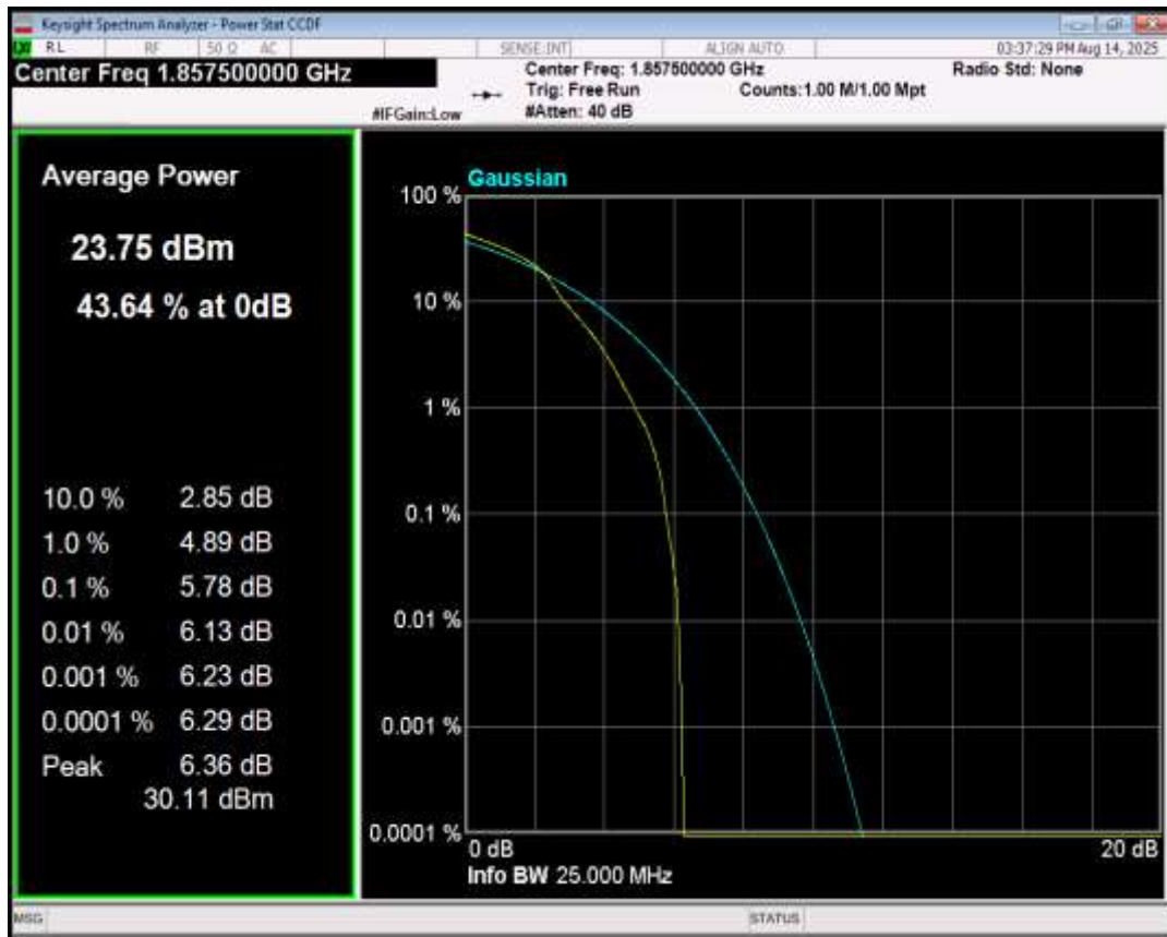
Band25 16QAM BW=20MHz Channel=26590 RB Size=1 Position=#0
