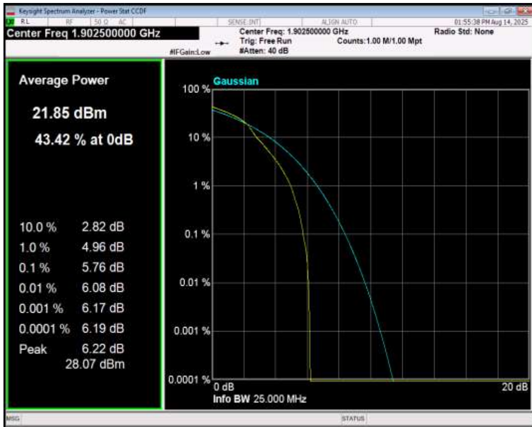
Band2 16QAM BW=20MHz Channel=18700 RB Size=1 Position=#0
