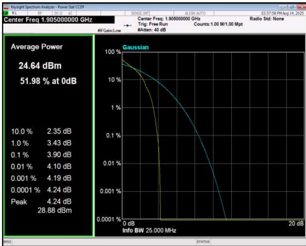
Band25 QPSK BW=3MHz Channel=26055 RB Size=1 Position=#0
