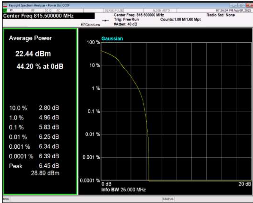
Band26(814-824) 16QAM BW=3MHz Channel=26740 RB Size=1 Position=#0
