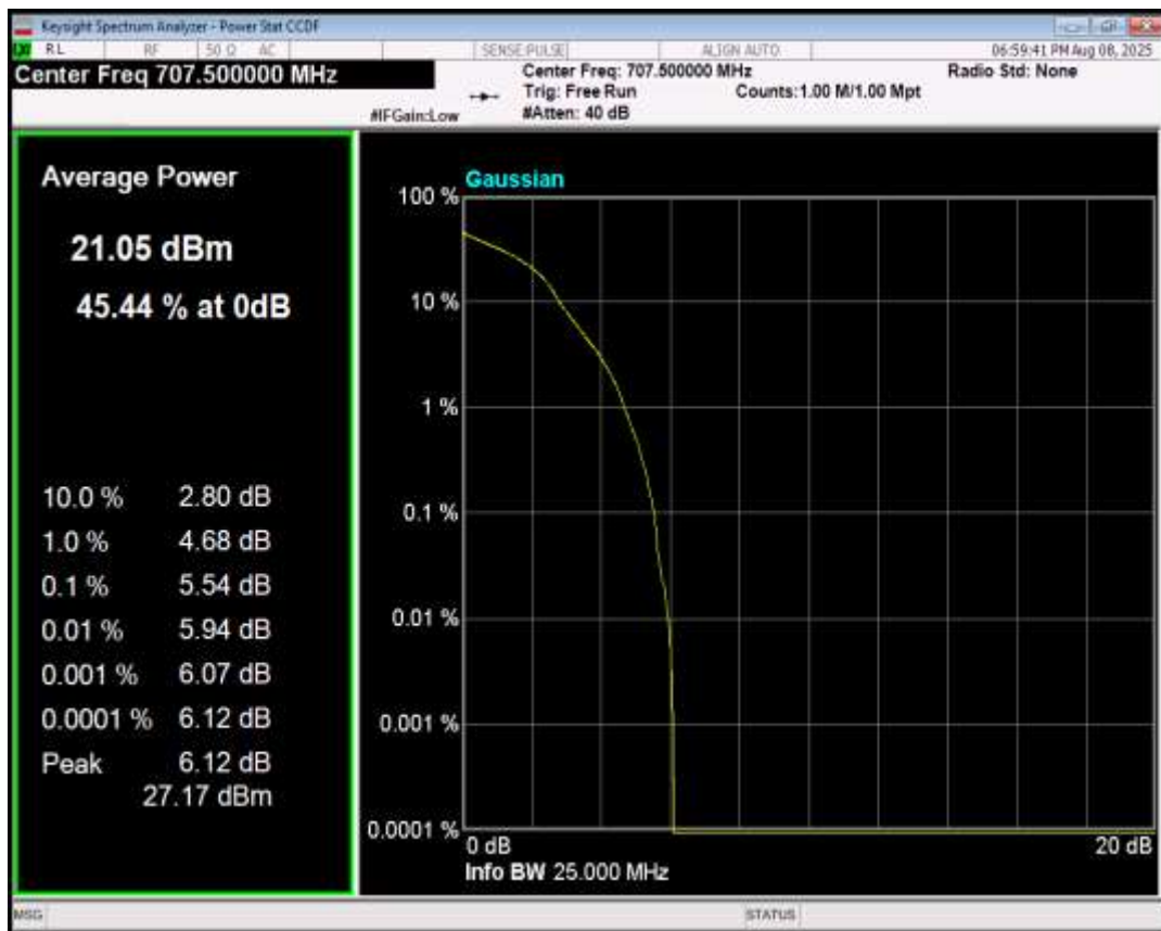
Band12 16QAM BW=3MHz Channel=23165 RB Size=1 Position=#0
