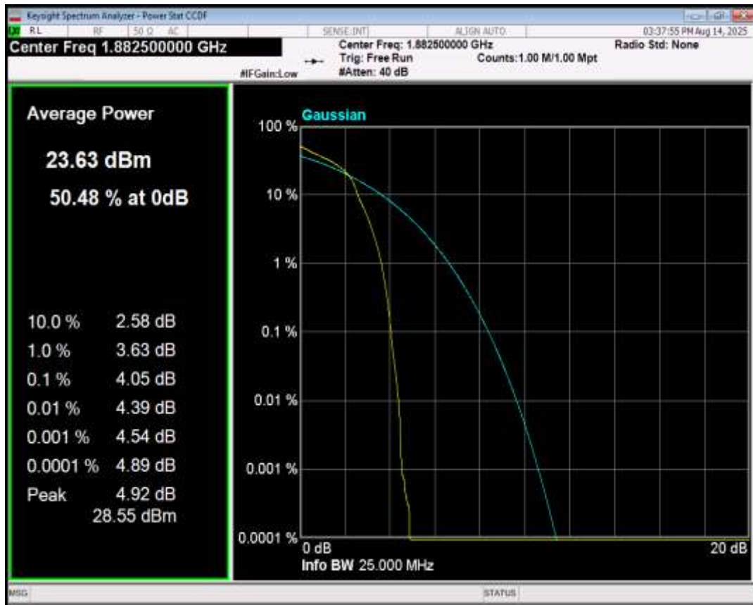
Band25 16QAM BW=20MHz Channel=26140 RB Size=1 Position=#0
