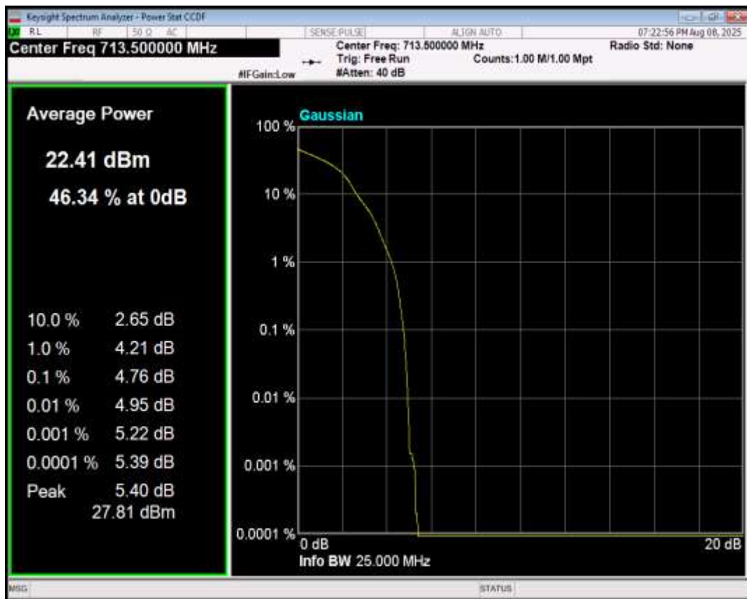
Band17 QPSK BW=10MHz Channel=23780 RB Size=1 Position=#0
