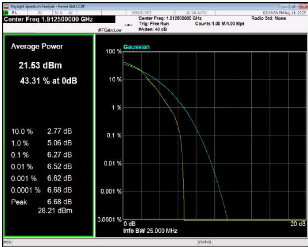
Band25 16QAM BW=5MHz Channel=26365 RB Size=1 Position=#0
