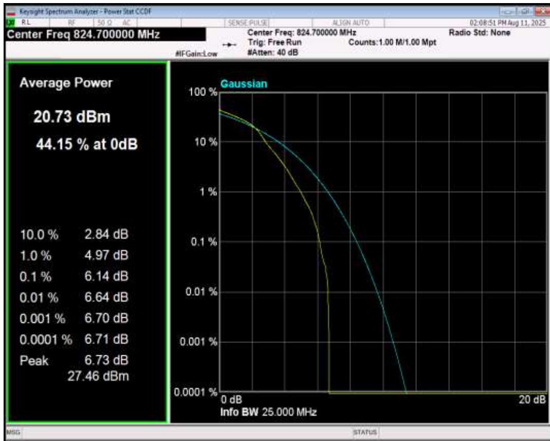
Band26(824-849) 16QAM BW=1.4MHz Channel=26915 RB Size=1 Position=#0
