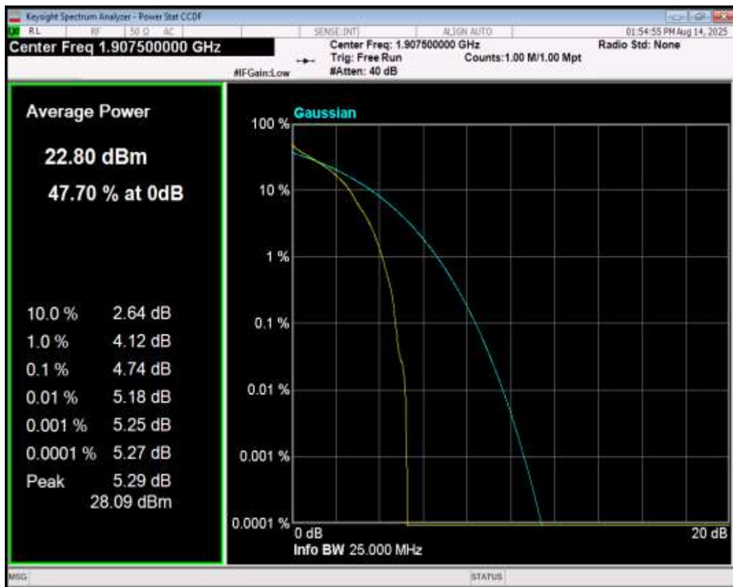
Band25 16QAM BW=1.4MHz Channel=26047 RB Size=1 Position=#0
