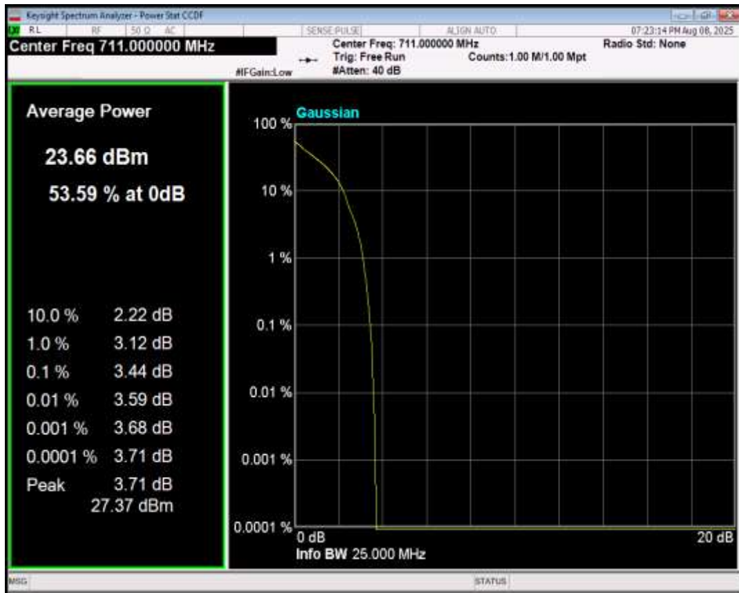
Band17 QPSK BW=5MHz Channel=23755 RB Size=1 Position=#0
