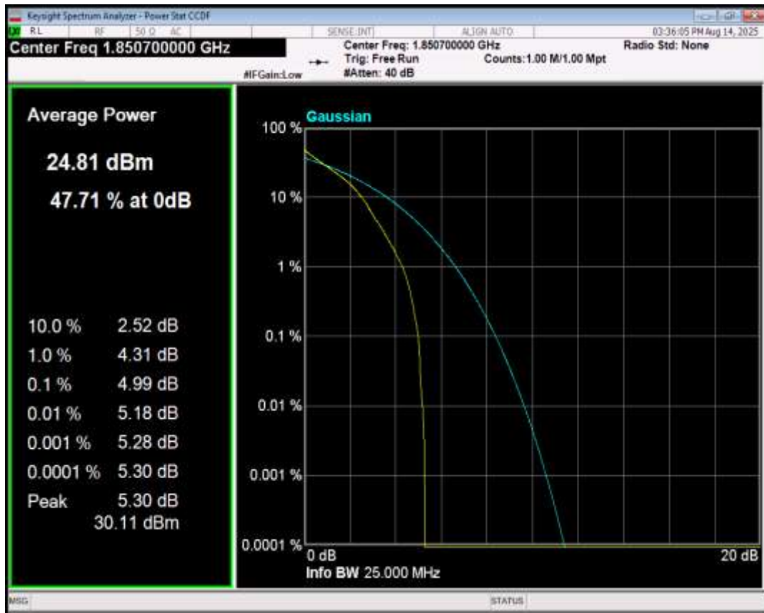
Band25 QPSK BW=10MHz Channel=26090 RB Size=1 Position=#0
