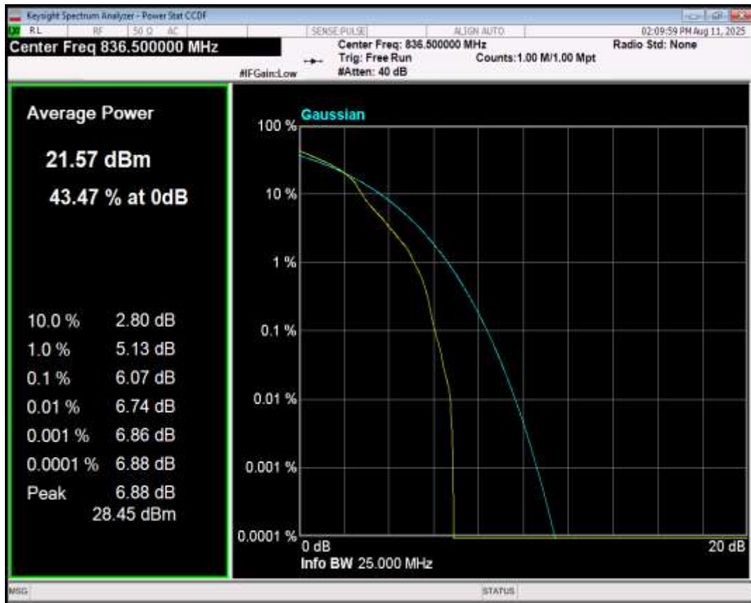
Band26(824-849) 16QAM BW=10MHz Channel=26990 RB Size=1 Position=#0
