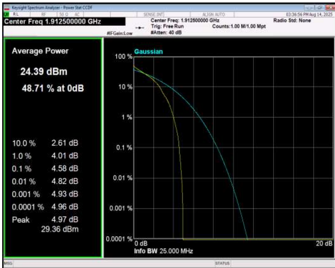
Band26(814-824) 16QAM BW=1.4MHz Channel=26697 RB Size=1 Position=#0
