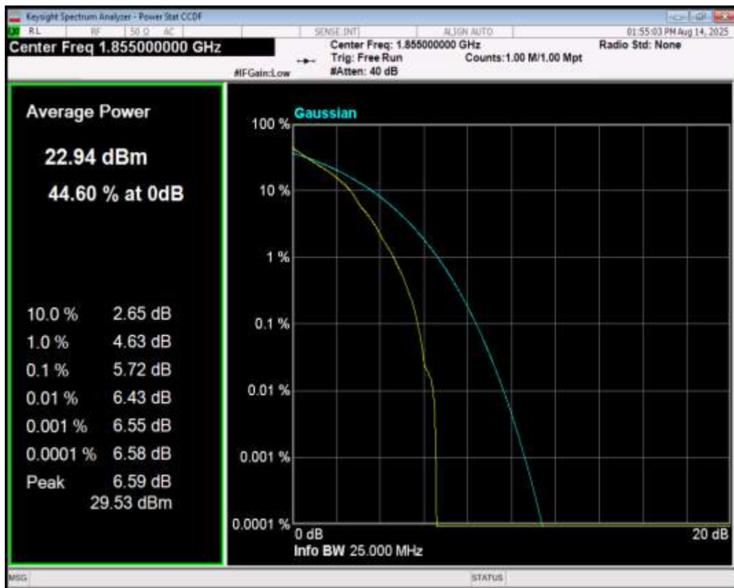
Band2 QPSK BW=10MHz Channel=18900 RB Size=1 Position=#0
