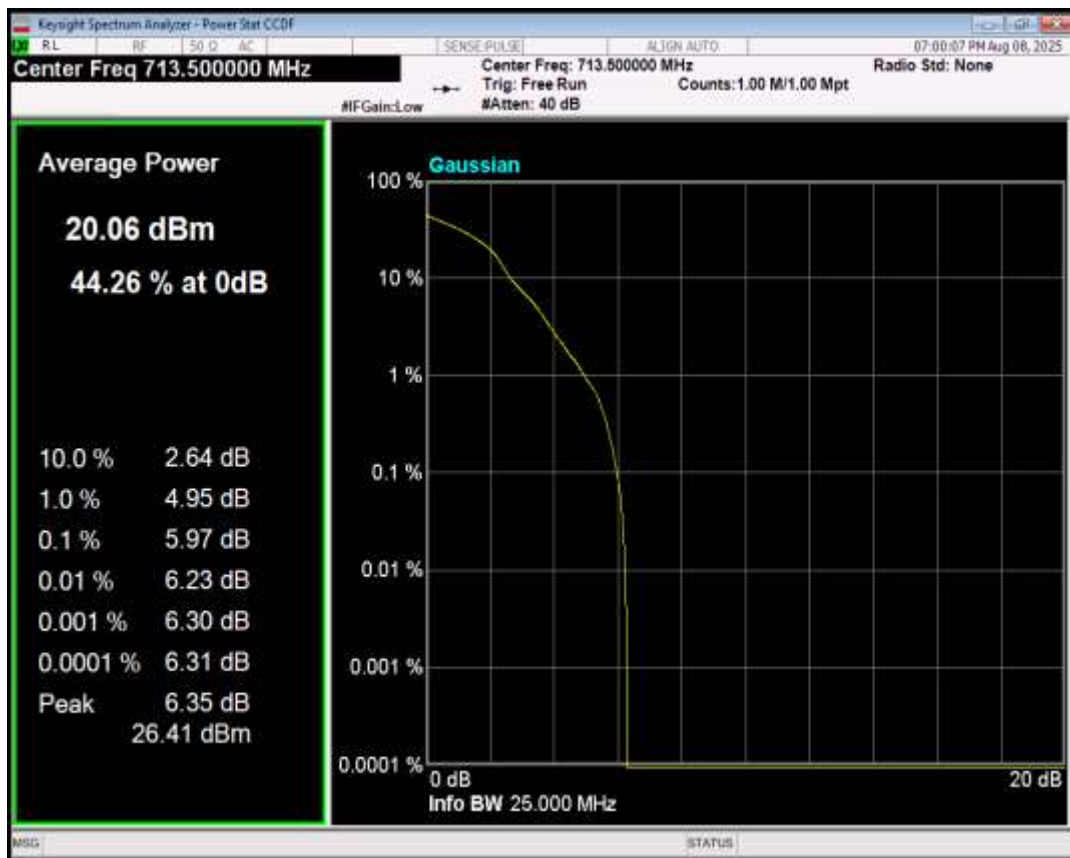
Band12 QPSK BW=1.4MHz Channel=23017 RB Size=1 Position=#0
