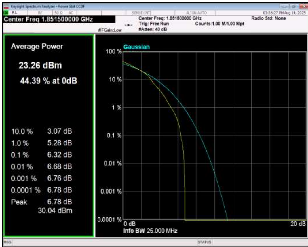
Band25 16QAM BW=3MHz Channel=26365 RB Size=1 Position=#0
