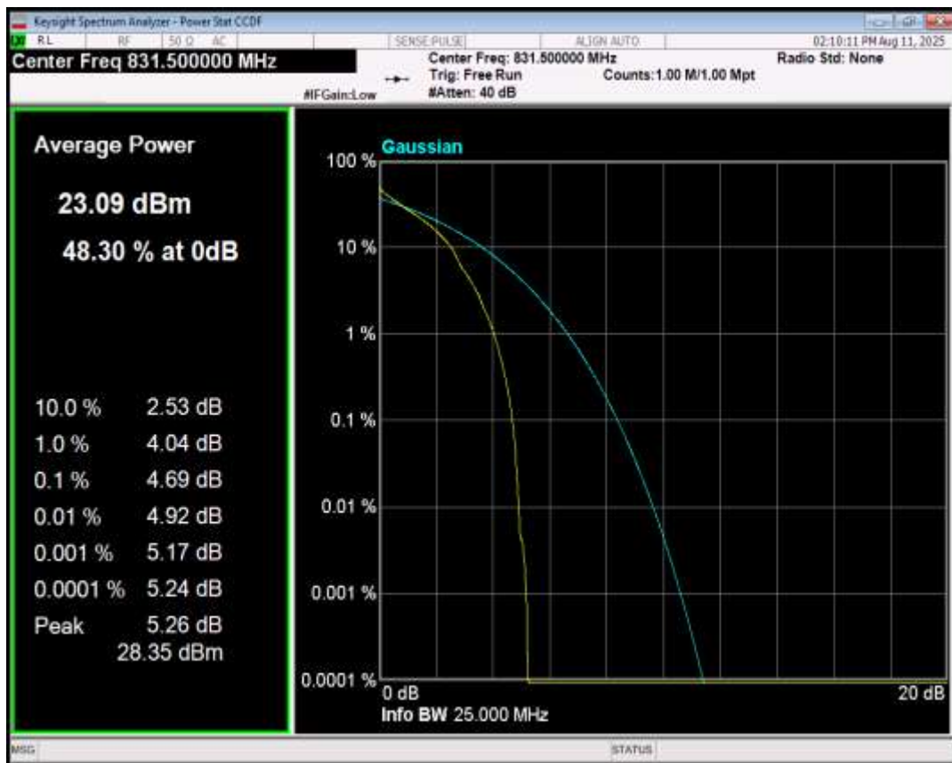
Band26(824-849) QPSK BW=15MHz Channel=26915 RB Size=1 Position=#0
