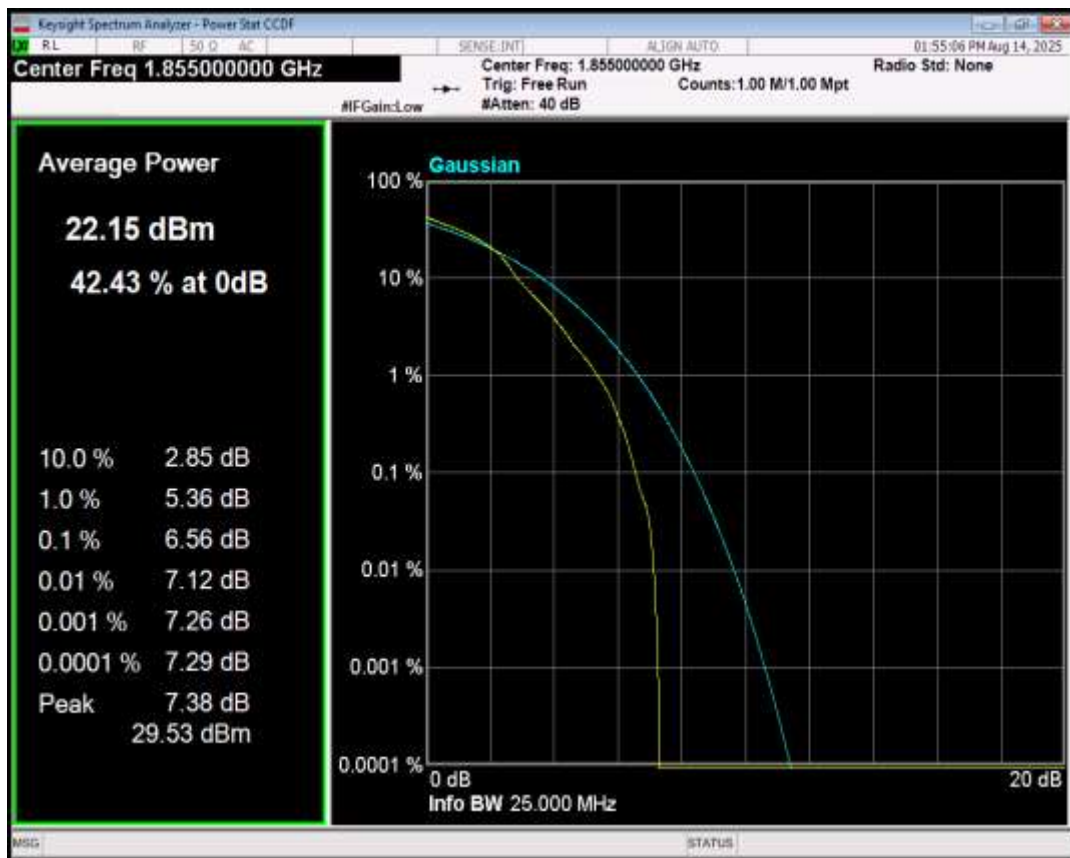
Band2 16QAM BW=10MHz Channel=18900 RB Size=1 Position=#0
