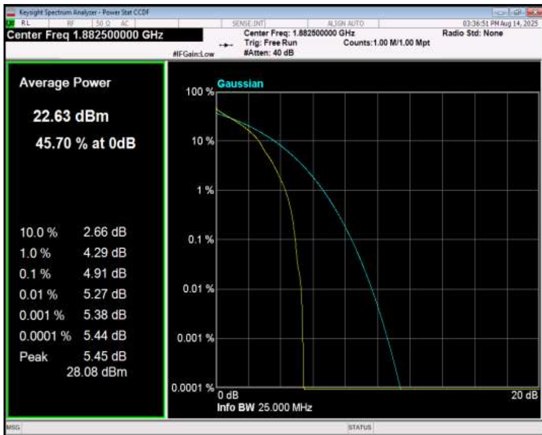
Band25 QPSK BW=5MHz Channel=26065 RB Size=1 Position=#0
