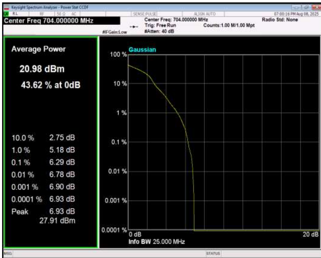
Band12 16QAM BW=10MHz Channel=23095 RB Size=1 Position=#0
