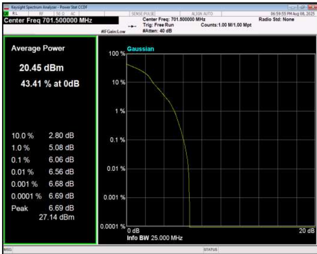
Band12 16QAM BW=5MHz Channel=23095 RB Size=1 Position=#0
