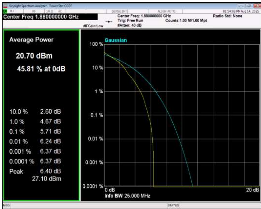
Band2 QPSK BW=1.4MHz Channel=19193 RB Size=1 Position=#0
