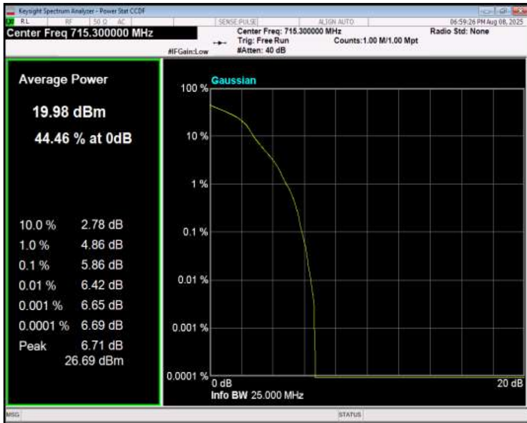
Band12 16QAM BW=10MHz Channel=23060 RB Size=1 Position=#0
