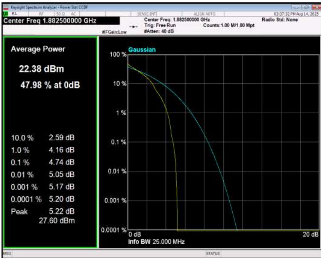
Band25 QPSK BW=20MHz Channel=26140 RB Size=1 Position=#0
