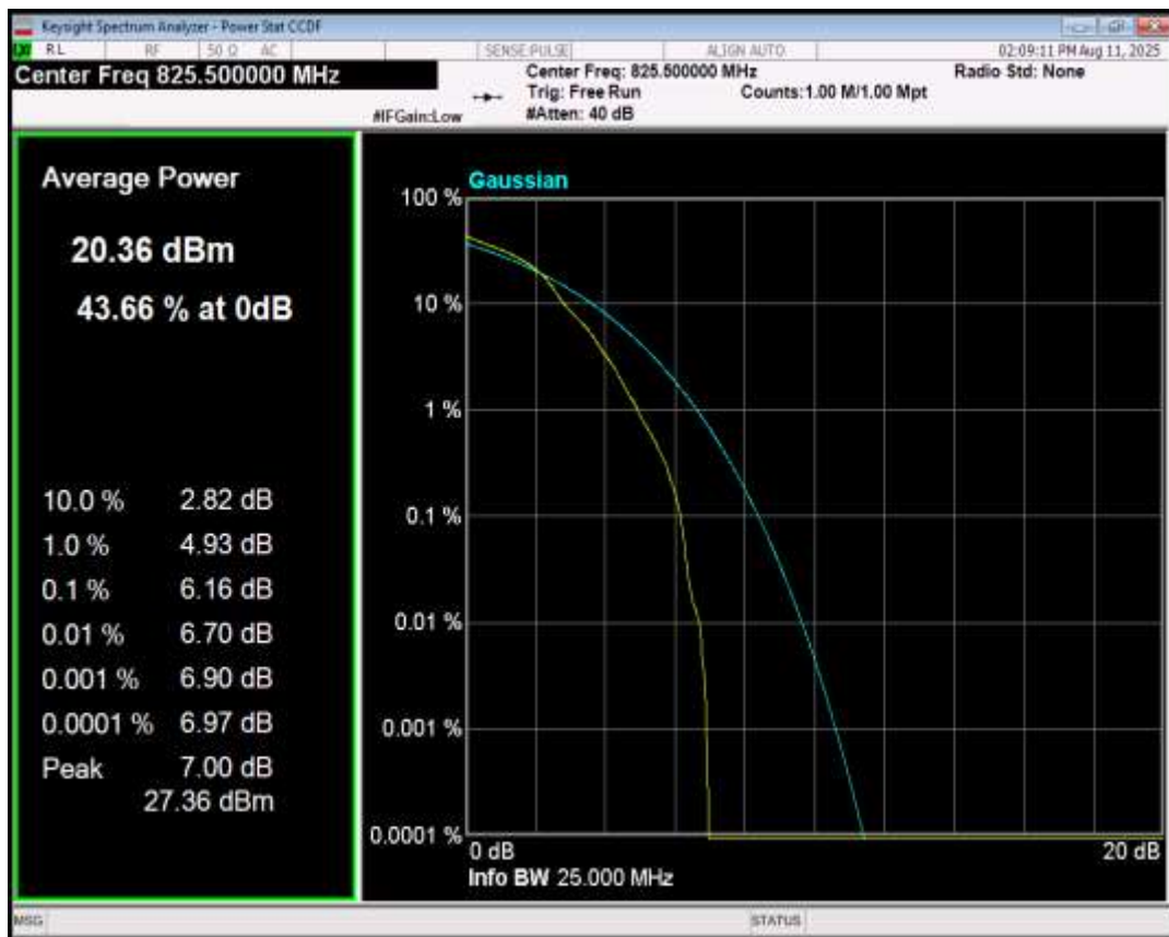
Band26(824-849) 16QAM BW=3MHz Channel=26915 RB Size=1 Position=#0
