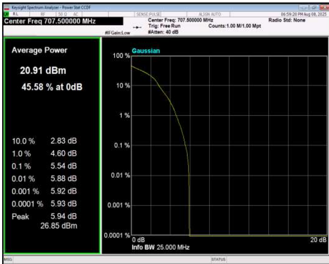
Band12 16QAM BW=1.4MHz Channel=23173 RB Size=1 Position=#0
