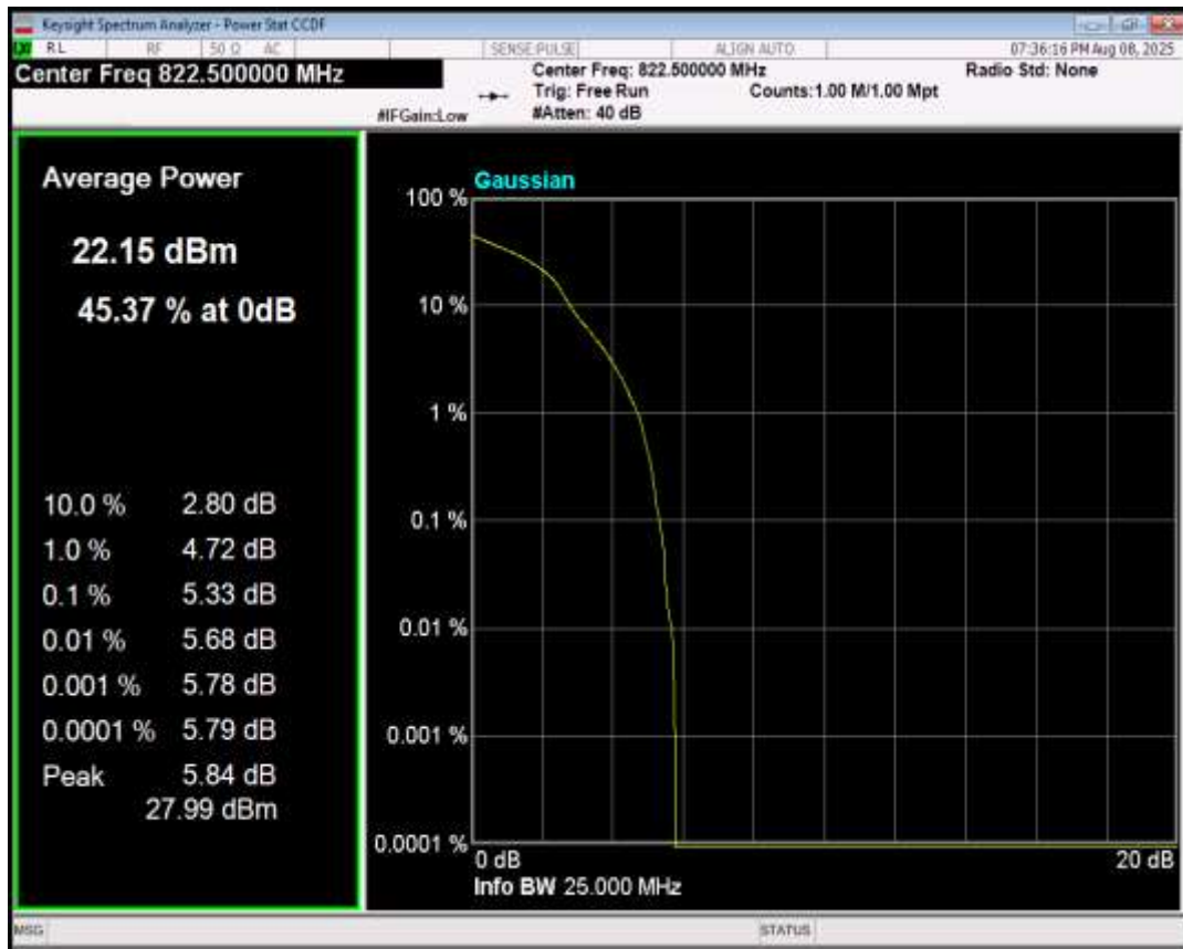
Band26(814-824) 16QAM BW=5MHz Channel=26740 RB Size=1 Position=#0
