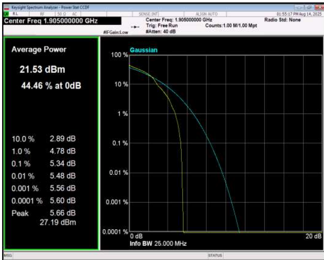
Band2 16QAM BW=15MHz Channel=18675 RB Size=1 Position=#0
