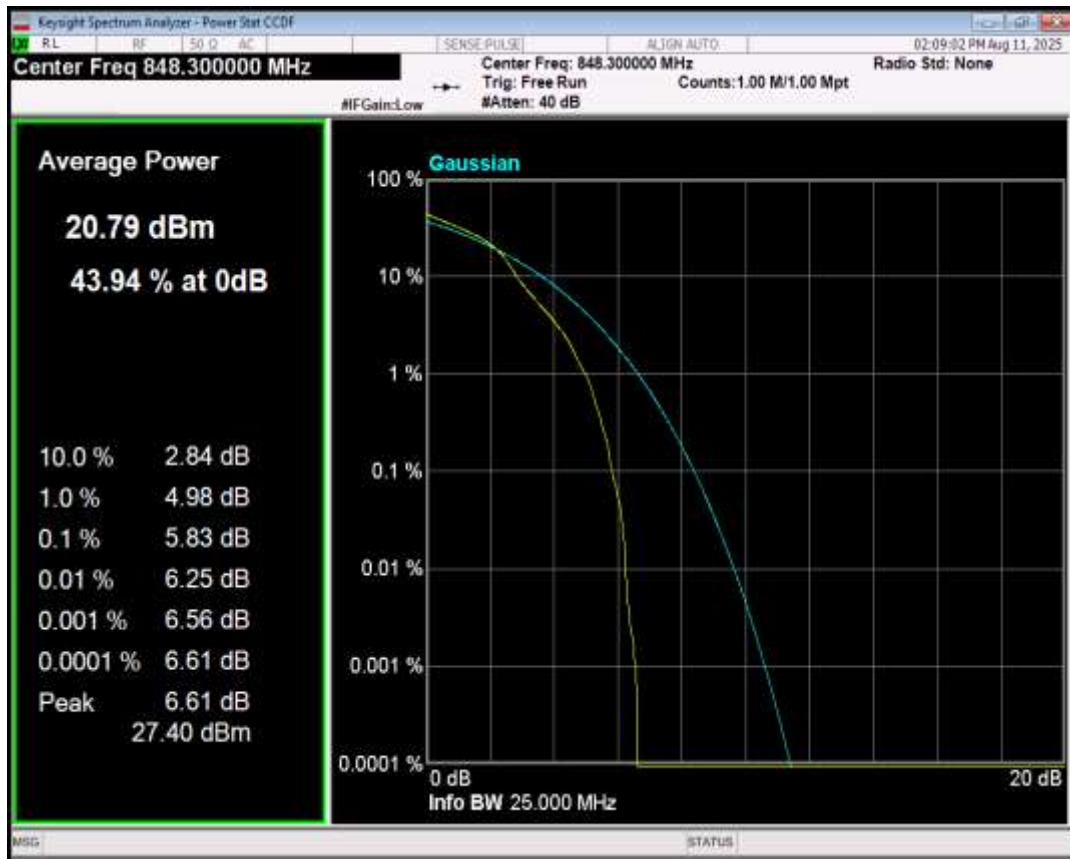
Band26(824-849) 16QAM BW=10MHz Channel=26840 RB Size=1 Position=#0
