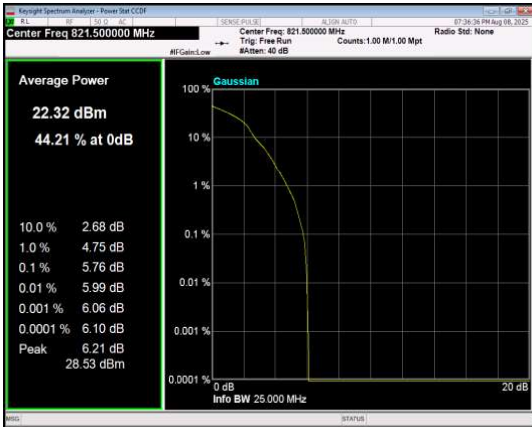
Band26(814-824) 16QAM BW=5MHz Channel=26715 RB Size=1 Position=#0
