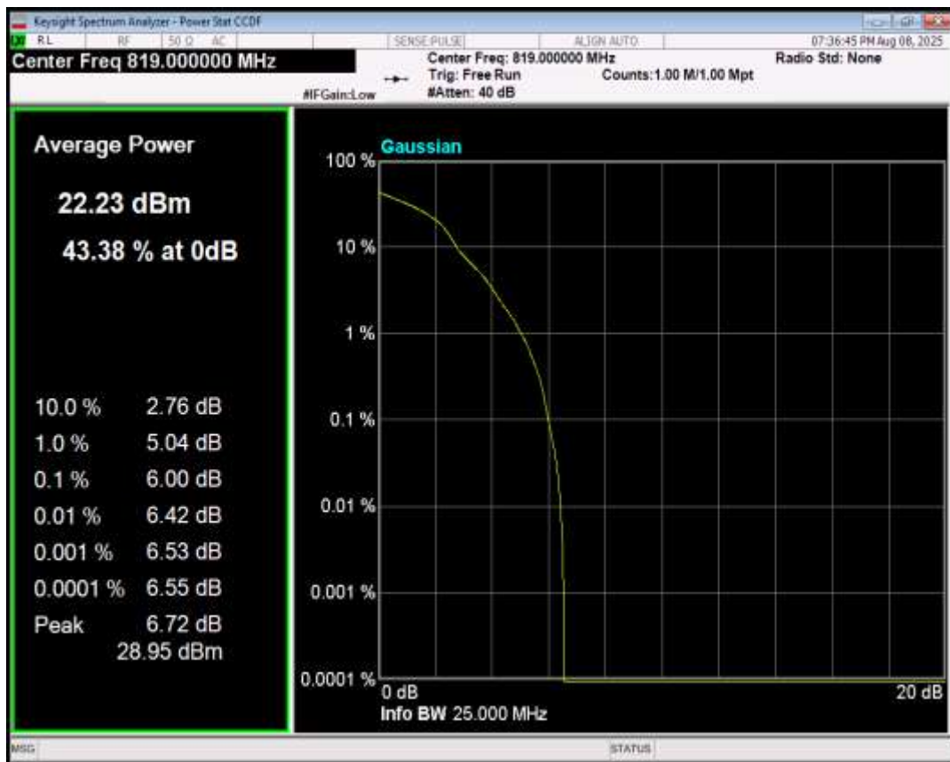
Band26(814-824) 16QAM BW=3MHz Channel=26705 RB Size=1 Position=#0
