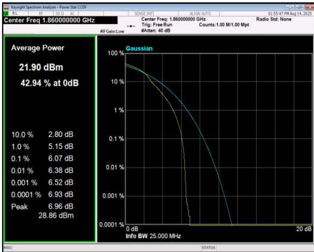
Band2 16QAM BW=20MHz Channel=18900 RB Size=1 Position=#0
