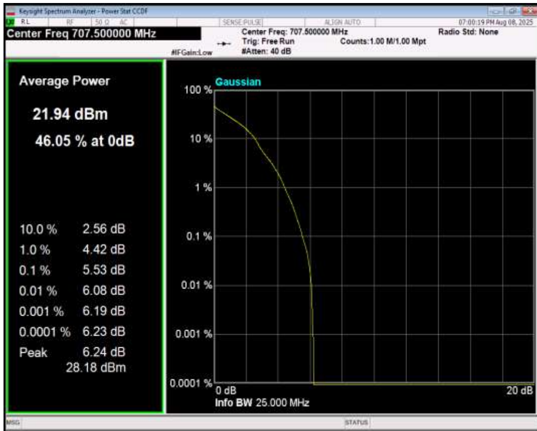
Band12 QPSK BW=10MHz Channel=23130 RB Size=1 Position=#0
