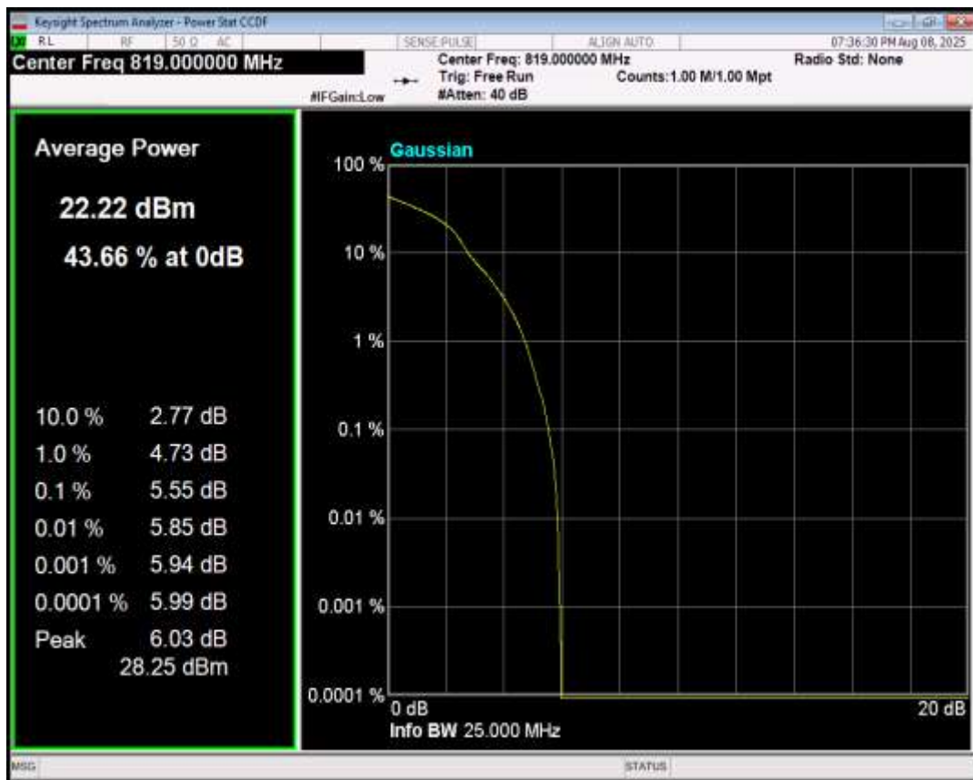
Band26(814-824) 16QAM BW=5MHz Channel=26765 RB Size=1 Position=#0
