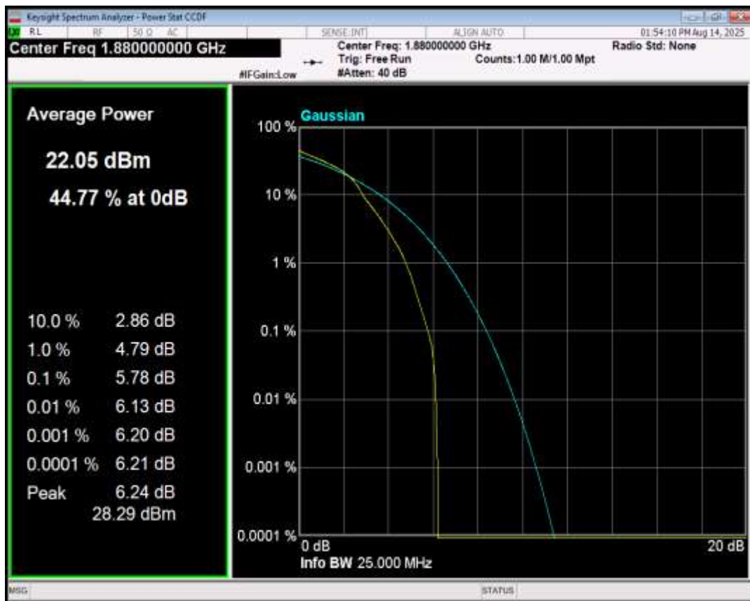
Band2 16QAM BW=1.4MHz Channel=19193 RB Size=1 Position=#0
