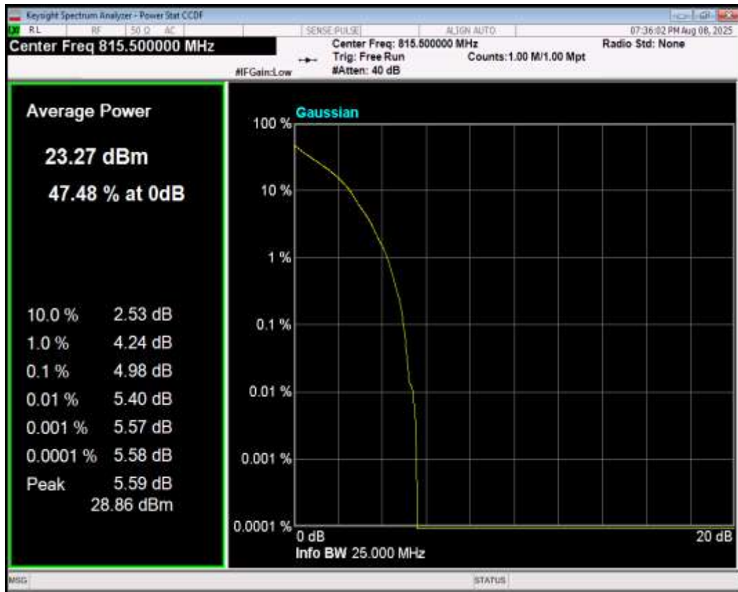
Band26(814-824) QPSK BW=3MHz Channel=26740 RB Size=1 Position=#0
