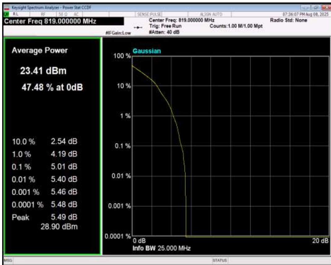
Band26(814-824) QPSK BW=3MHz Channel=26775 RB Size=1 Position=#0
