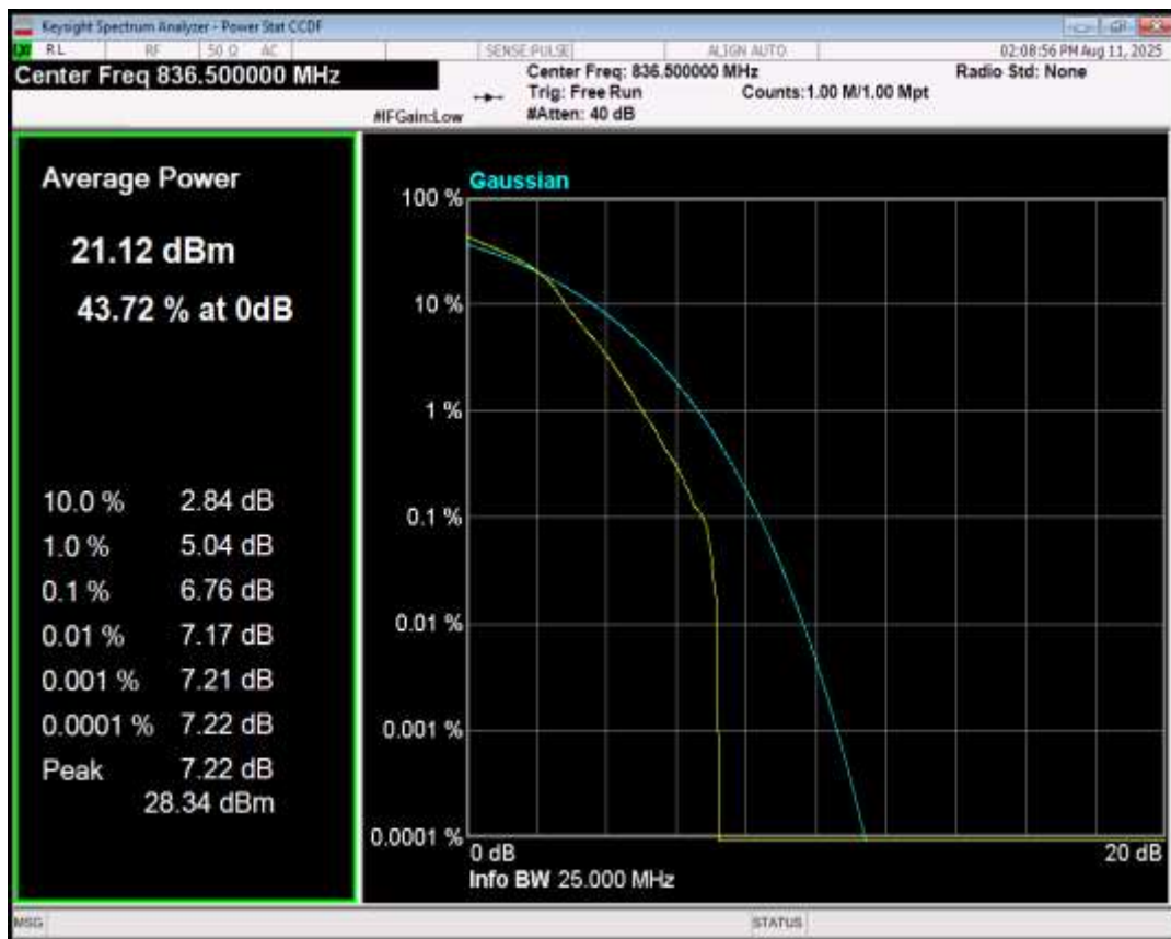
Band26(824-849) 16QAM BW=1.4MHz Channel=27033 RB Size=1 Position=#0
