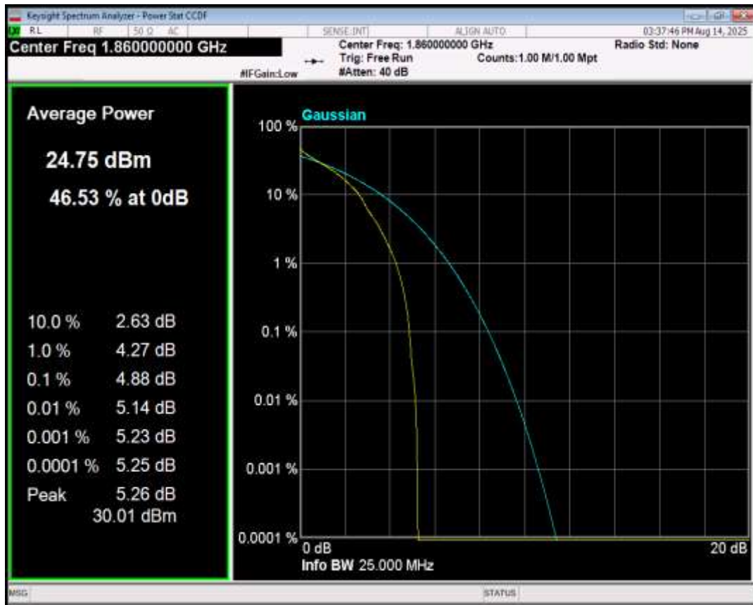
Band25 QPSK BW=15MHz Channel=26615 RB Size=1 Position=#0
