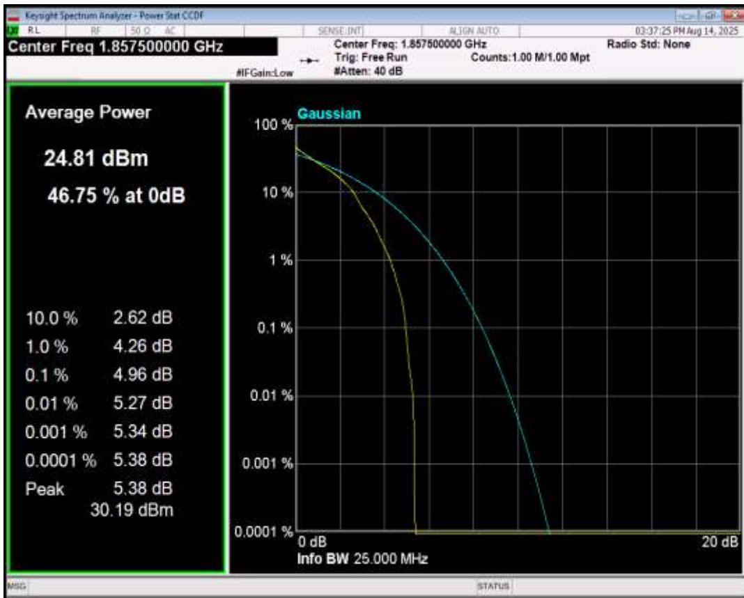
Band25 QPSK BW=15MHz Channel=26365 RB Size=1 Position=#0
