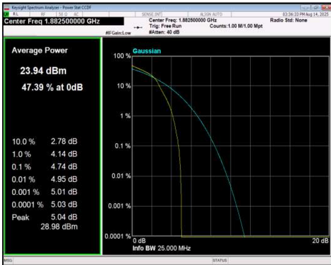
Band25 16QAM BW=3MHz Channel=26675 RB Size=1 Position=#0
