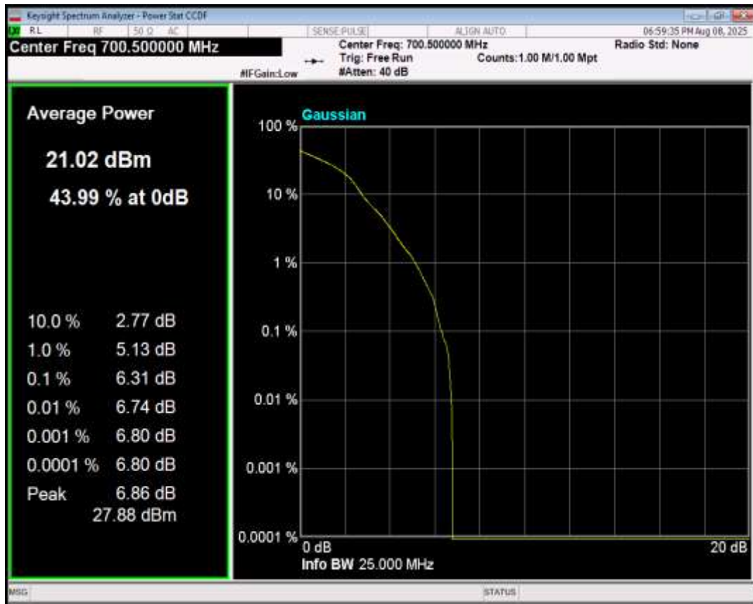
Band12 16QAM BW=3MHz Channel=23095 RB Size=1 Position=#0
