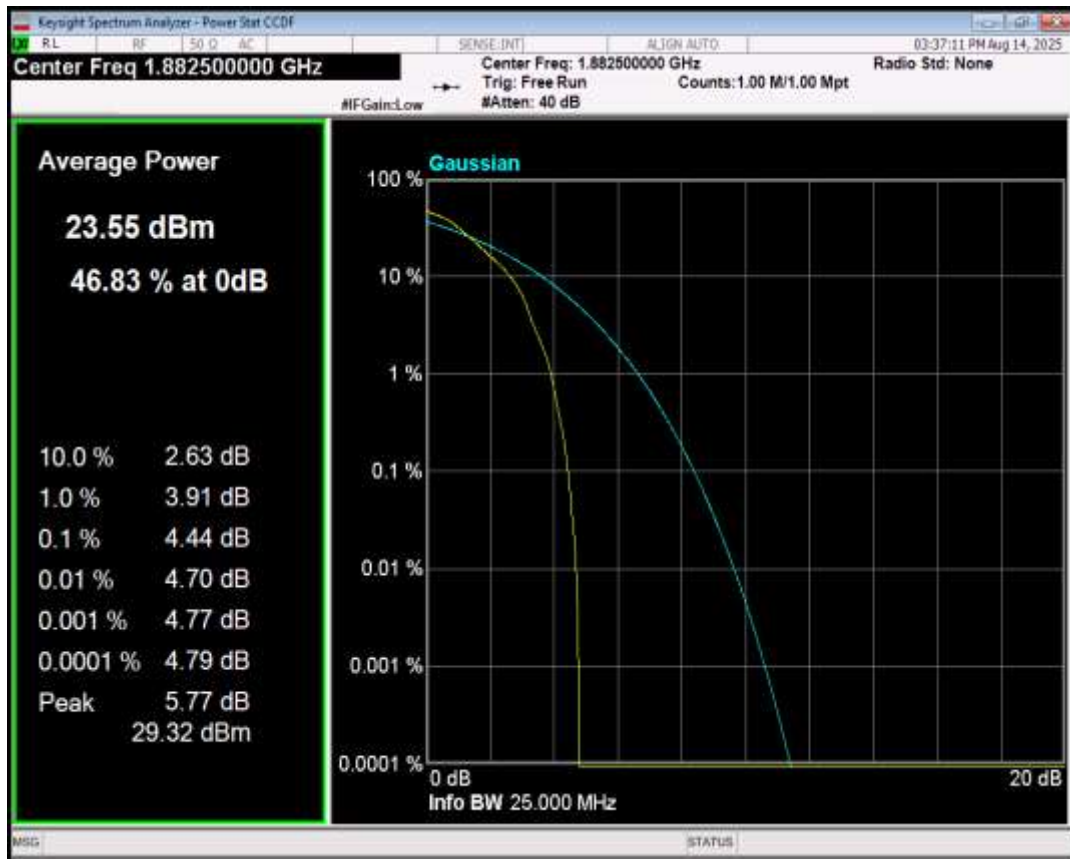
Band25 QPSK BW=10MHz Channel=26640 RB Size=1 Position=#0
