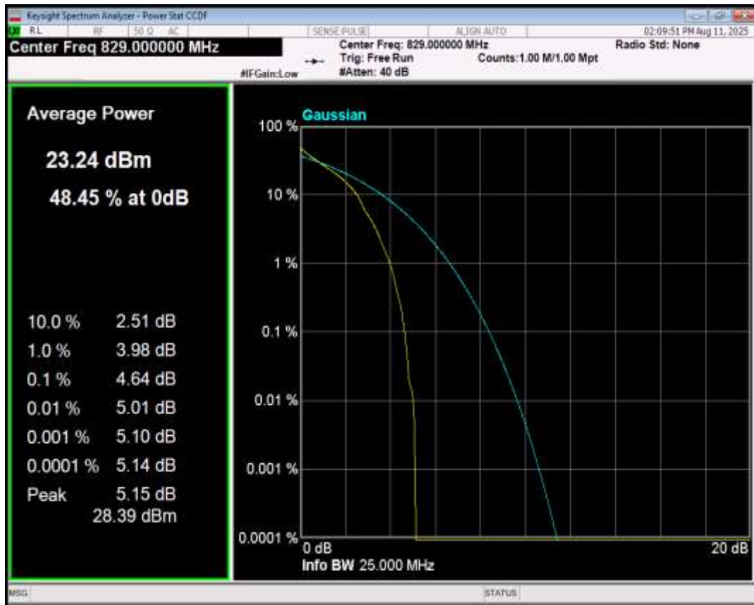
Band26(824-849) QPSK BW=10MHz Channel=26915 RB Size=1 Position=#0
