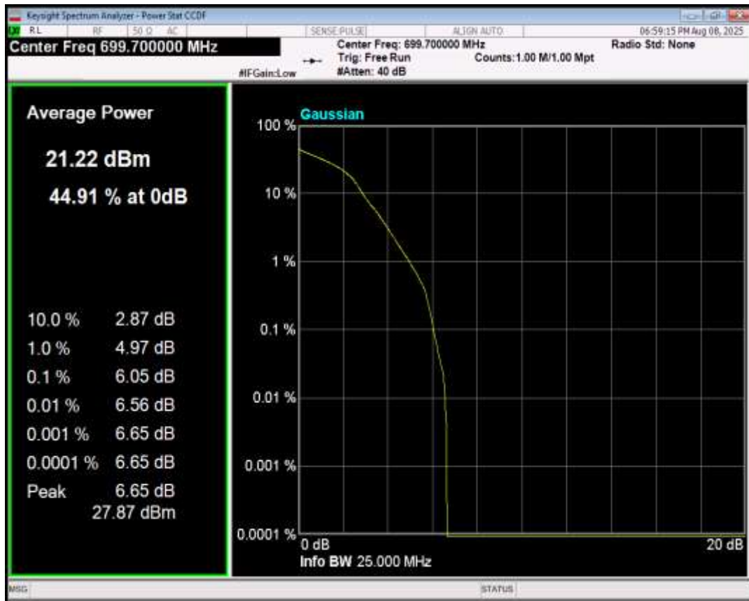
Band12 16QAM BW=1.4MHz Channel=23095 RB Size=1 Position=#0
