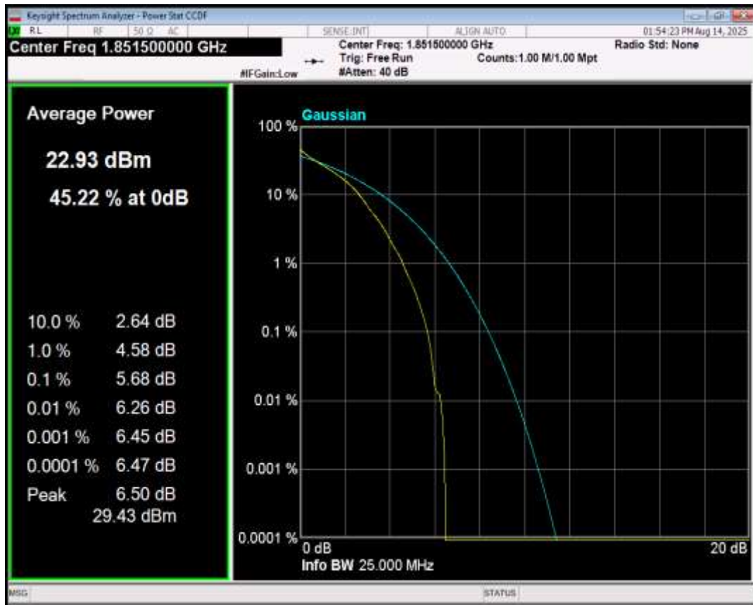
Band2 QPSK BW=3MHz Channel=18900 RB Size=1 Position=#0
