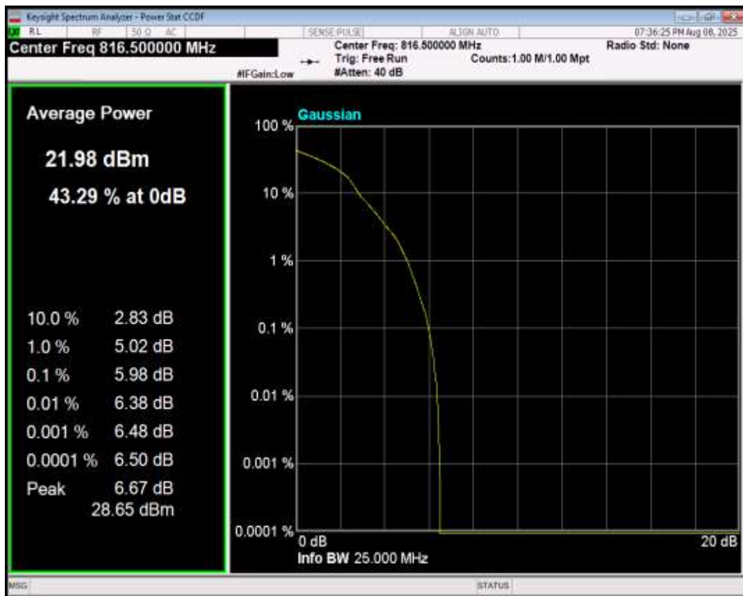
Band26(814-824) QPSK BW=1.4MHz Channel=26697 RB Size=1 Position=#0
