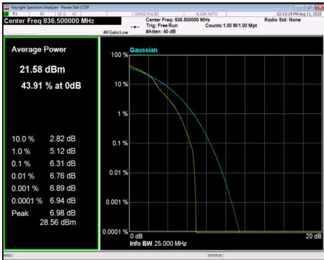
Band26(824-849) 16QAM BW=15MHz Channel=26965 RB Size=1 Position=#0
