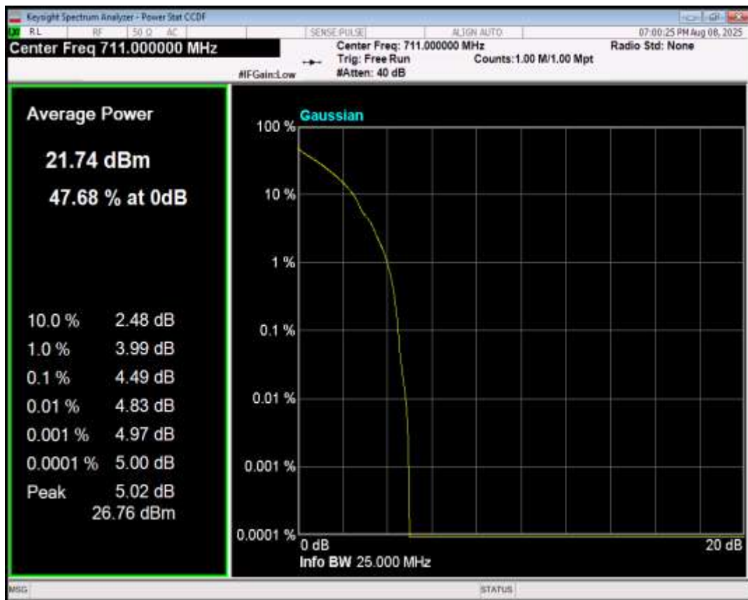
Band12 QPSK BW=3MHz Channel=23025 RB Size=1 Position=#0
