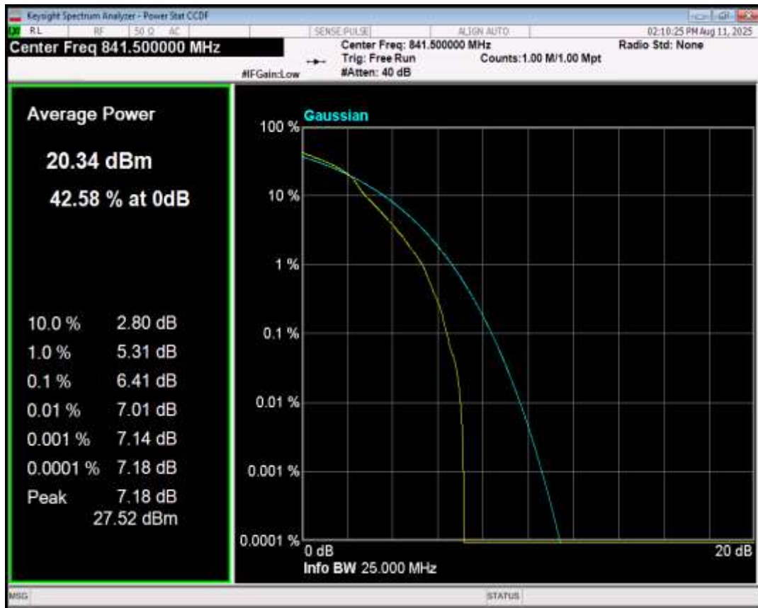
Band26(824-849) 16QAM BW=3MHz Channel=26805 RB Size=1 Position=#0
