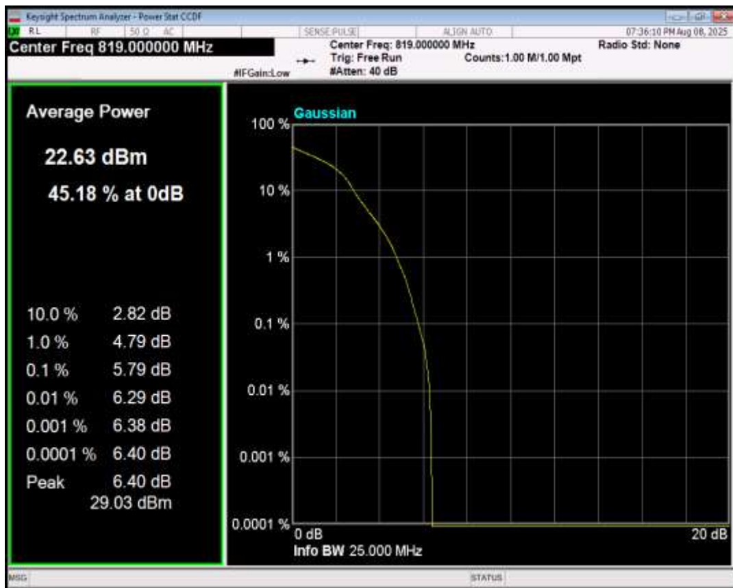
Band26(814-824) 16QAM BW=3MHz Channel=26775 RB Size=1 Position=#0
