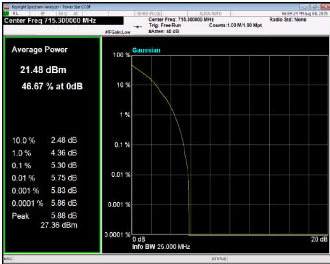
Band12 16QAM BW=5MHz Channel=23155 RB Size=1 Position=#0
