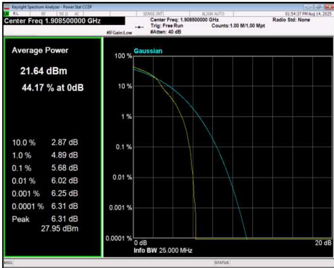
Band2 16QAM BW=5MHz Channel=18625 RB Size=1 Position=#0
