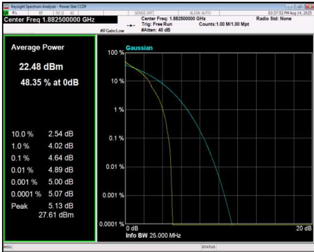
Band25 QPSK BW=20MHz Channel=26590 RB Size=1 Position=#0
