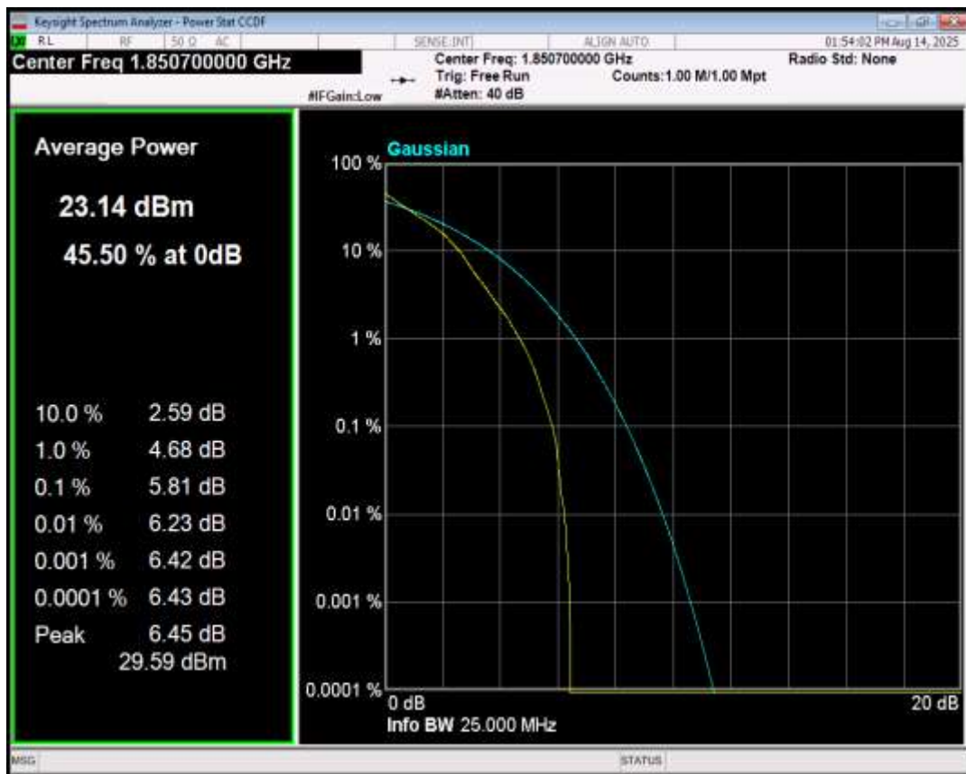
Band2 16QAM BW=5MHz Channel=18900 RB Size=1 Position=#0
