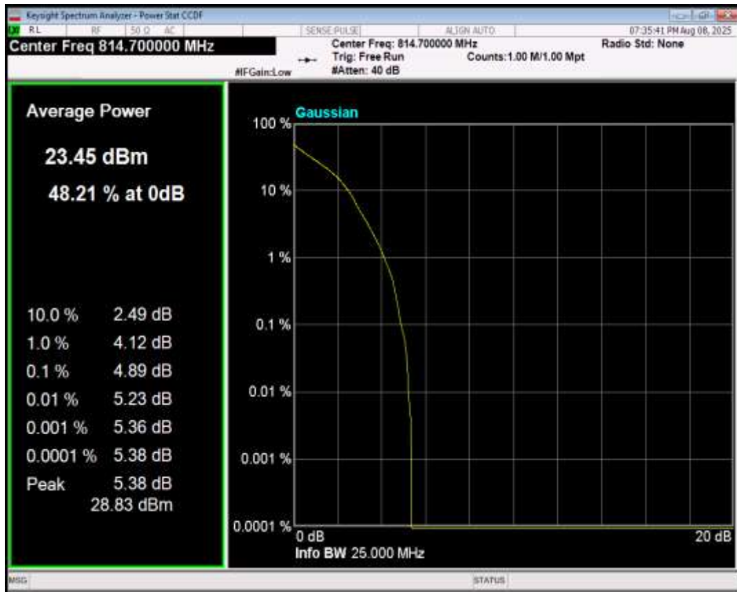
Band26(814-824) QPSK BW=1.4MHz Channel=26740 RB Size=1 Position=#0
