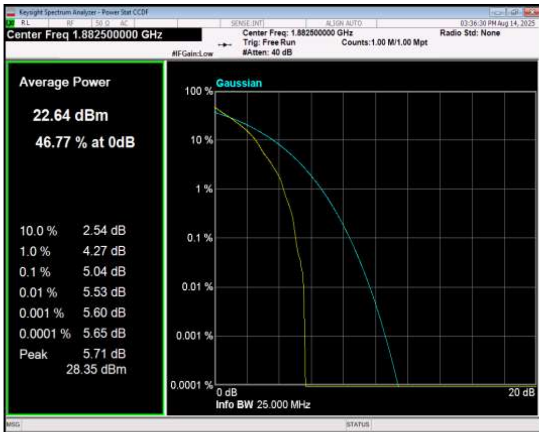
Band25 QPSK BW=3MHz Channel=26675 RB Size=1 Position=#0
