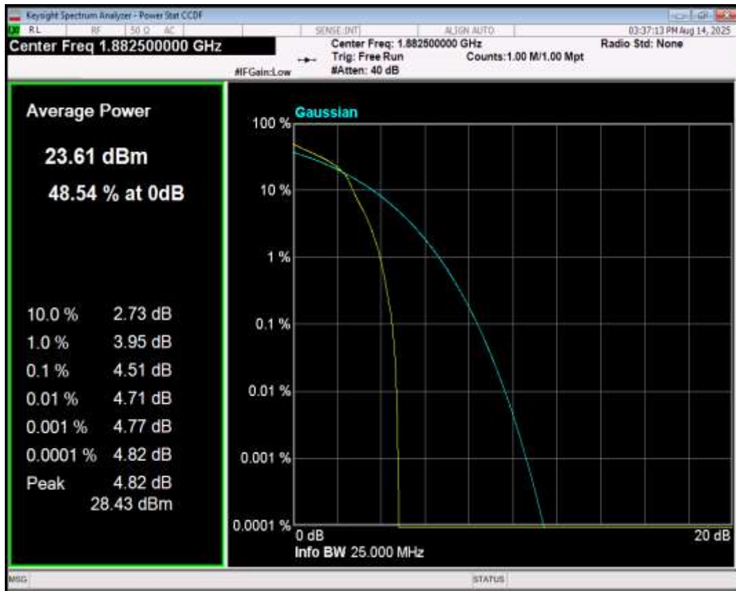
Band25 16QAM BW=10MHz Channel=26640 RB Size=1 Position=#0
