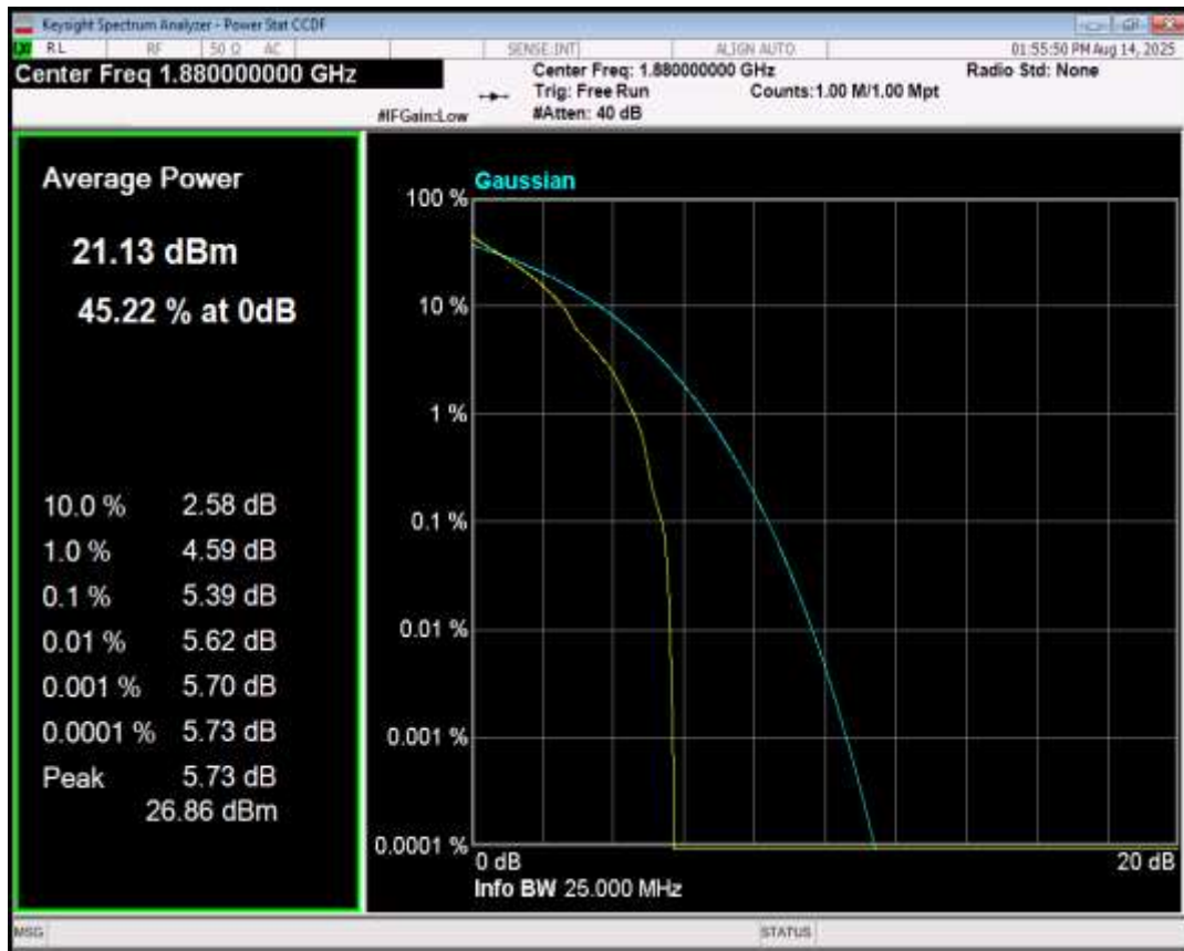
Band2 QPSK BW=20MHz Channel=19100 RB Size=1 Position=#0
