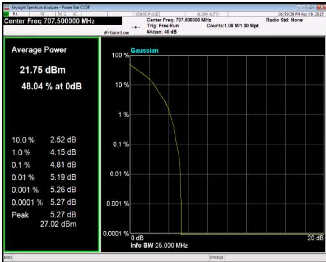
Band12 QPSK BW=3MHz Channel=23165 RB Size=1 Position=#0
