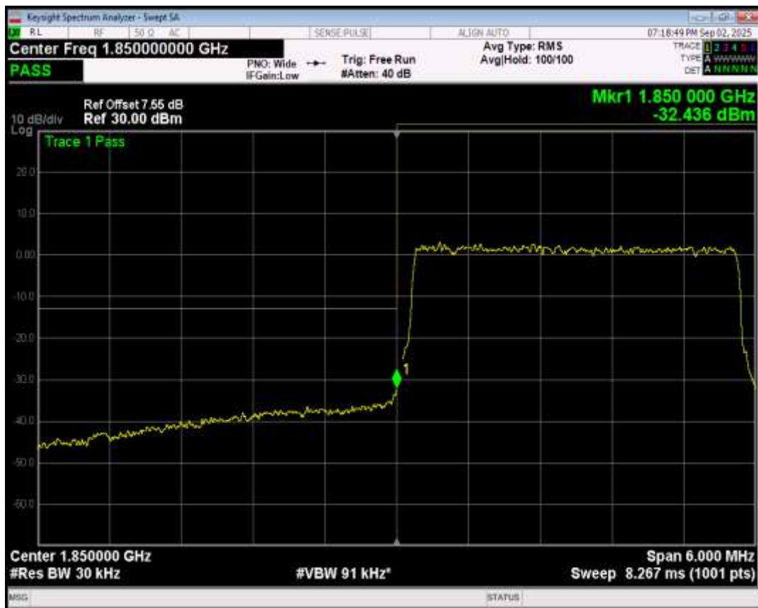
Band2 QPSK BW=3MHz Channel=19185 RB Size=15 Position=#0
