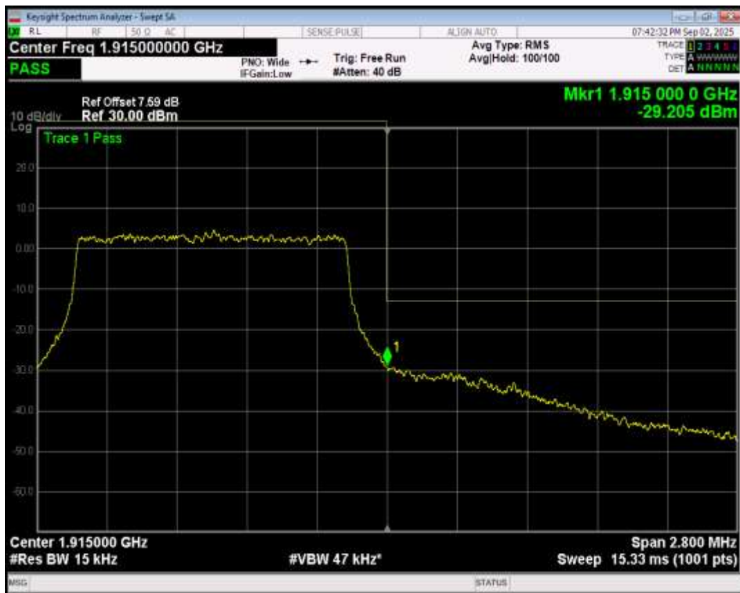
Band25 QPSK BW=3MHz Channel=26055 RB Size=15 Position=#0
