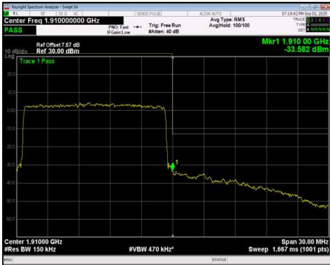
Band2 16QAM BW=15MHz Channel=19125 RB Size=75 Position=#0
