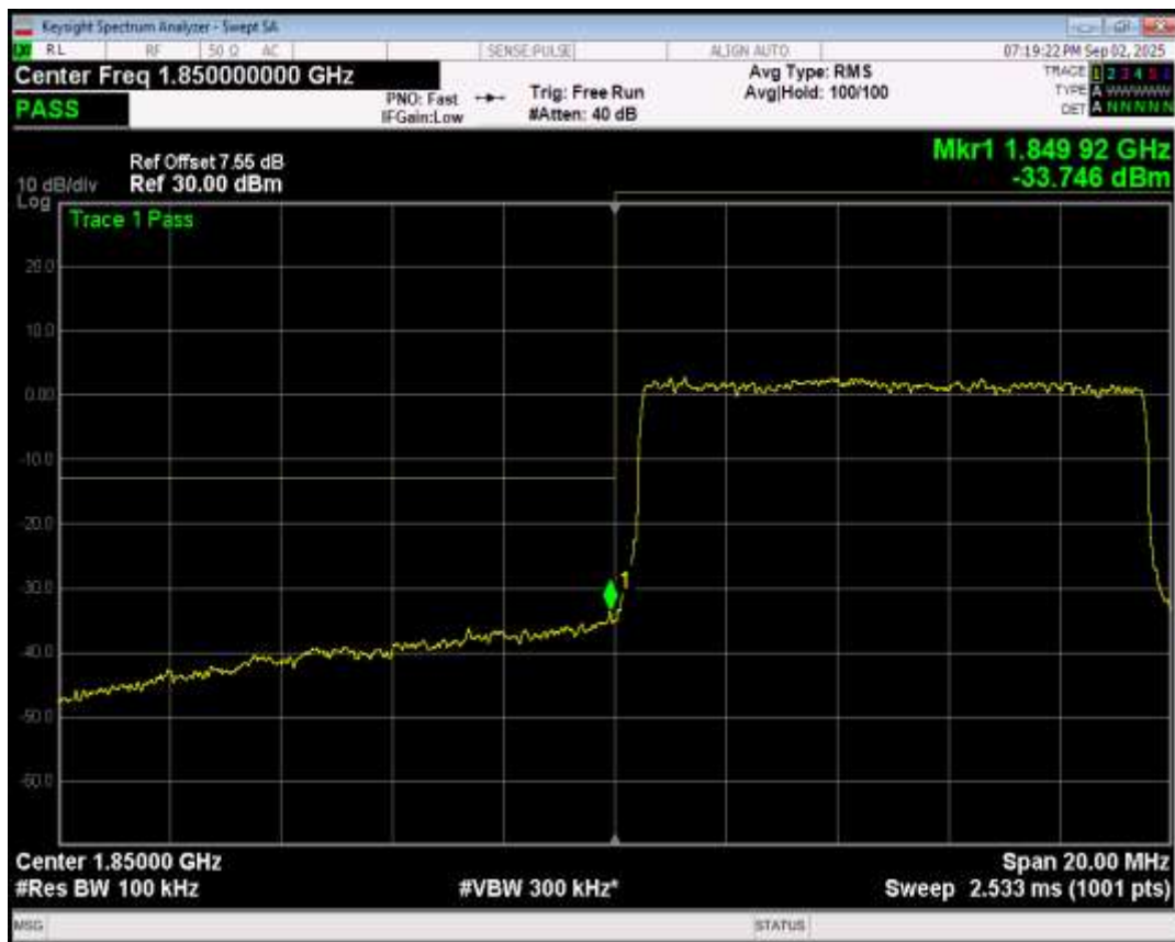
Band2 QPSK BW=10MHz Channel=19150 RB Size=50 Position=#0
