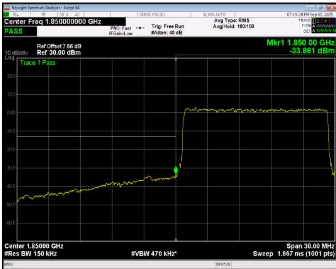
Band2 QPSK BW=15MHz Channel=19125 RB Size=75 Position=#0
