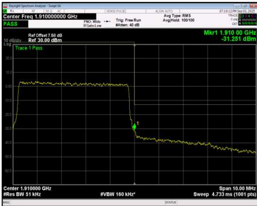
Band2 QPSK BW=10MHz Channel=18650 RB Size=50 Position=#0
