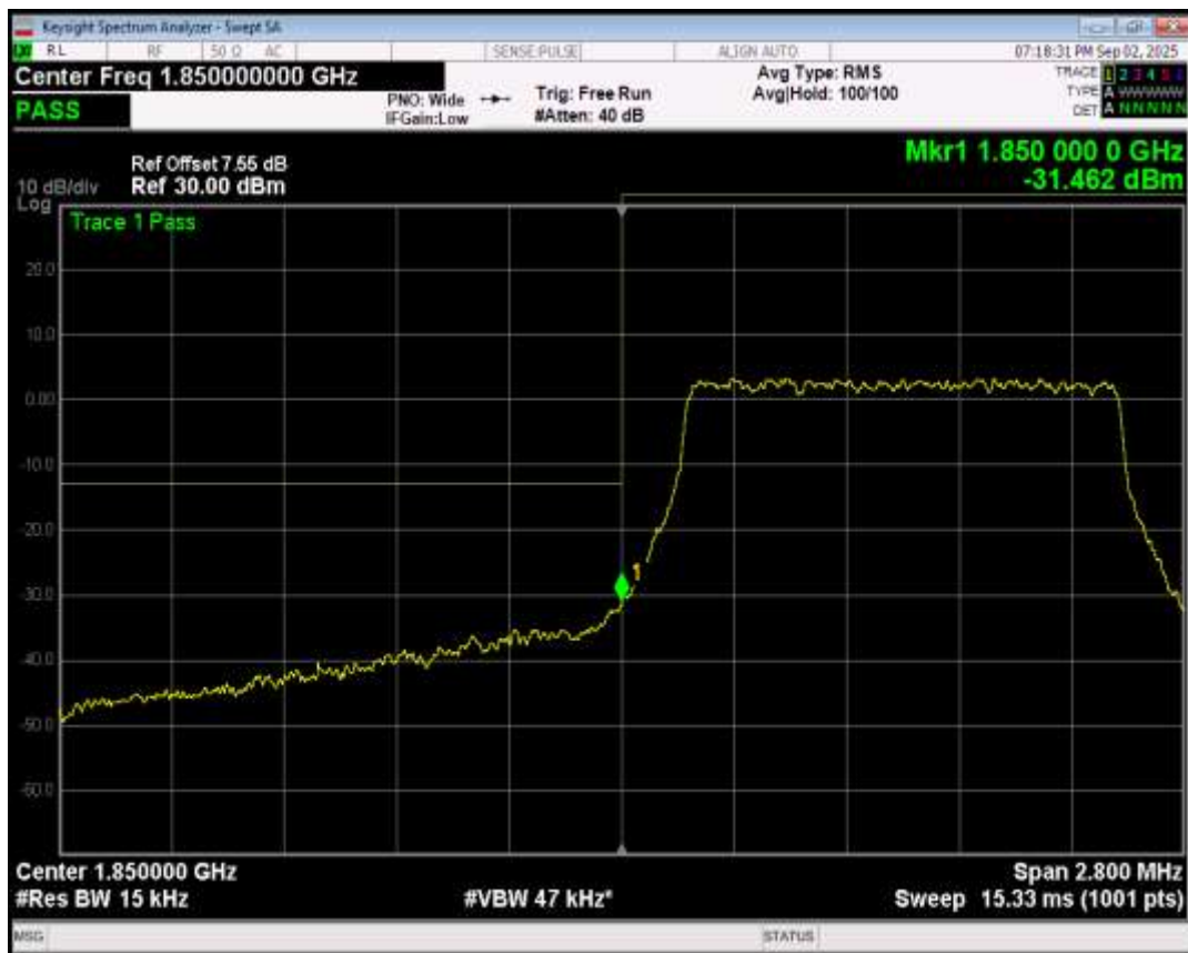
Band2 QPSK BW=1.4MHz Channel=19193 RB Size=6 Position=#0
