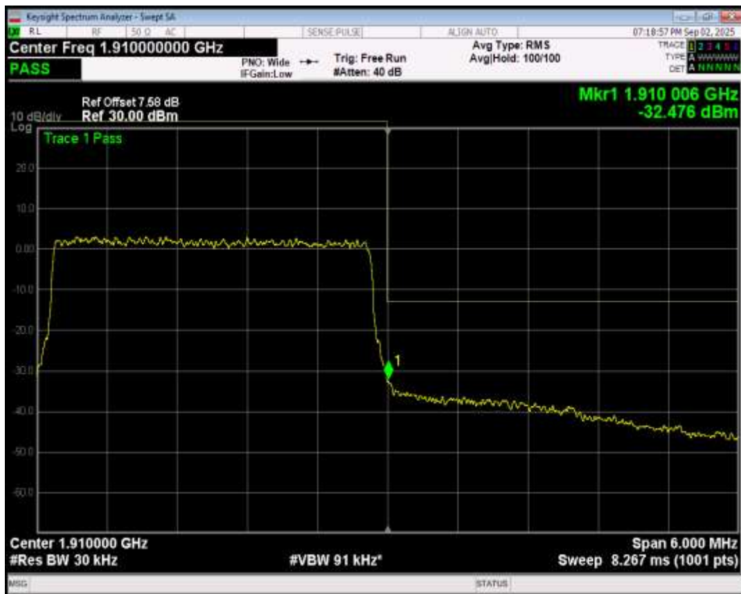
Band2 QPSK BW=5MHz Channel=18625 RB Size=25 Position=#0
