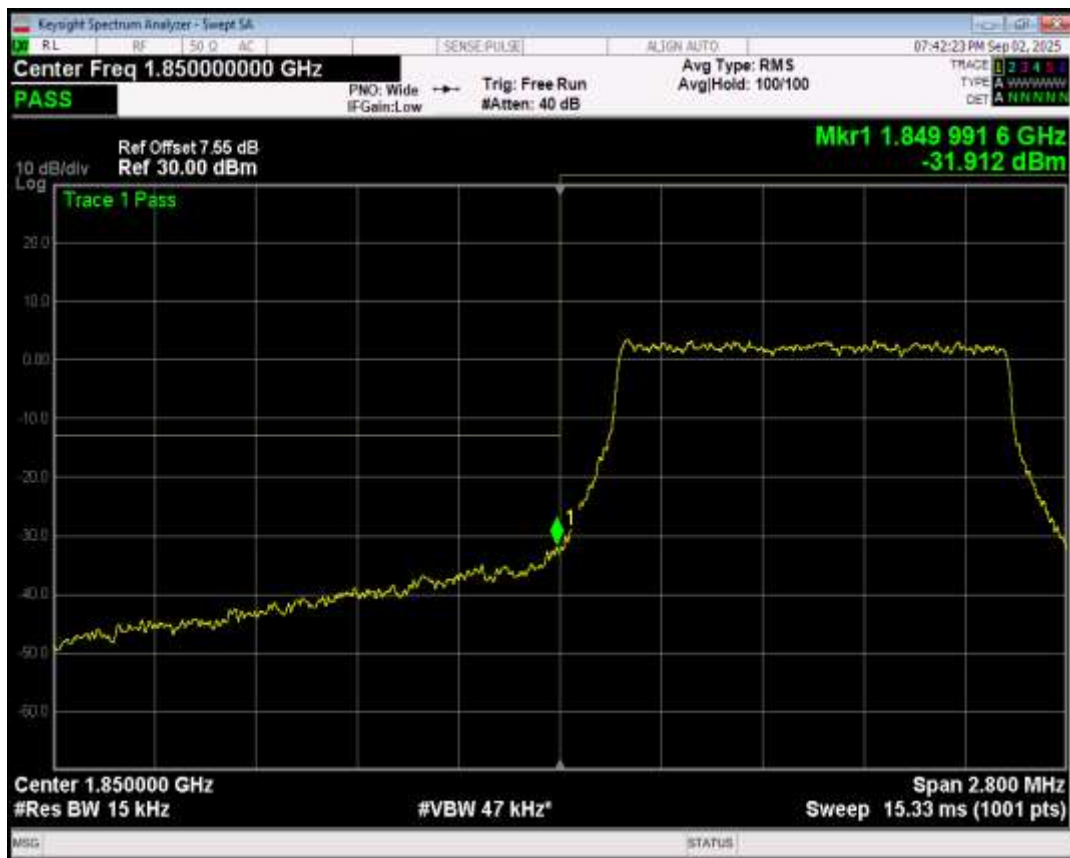
Band25 QPSK BW=1.4MHz Channel=26683 RB Size=6 Position=#0
