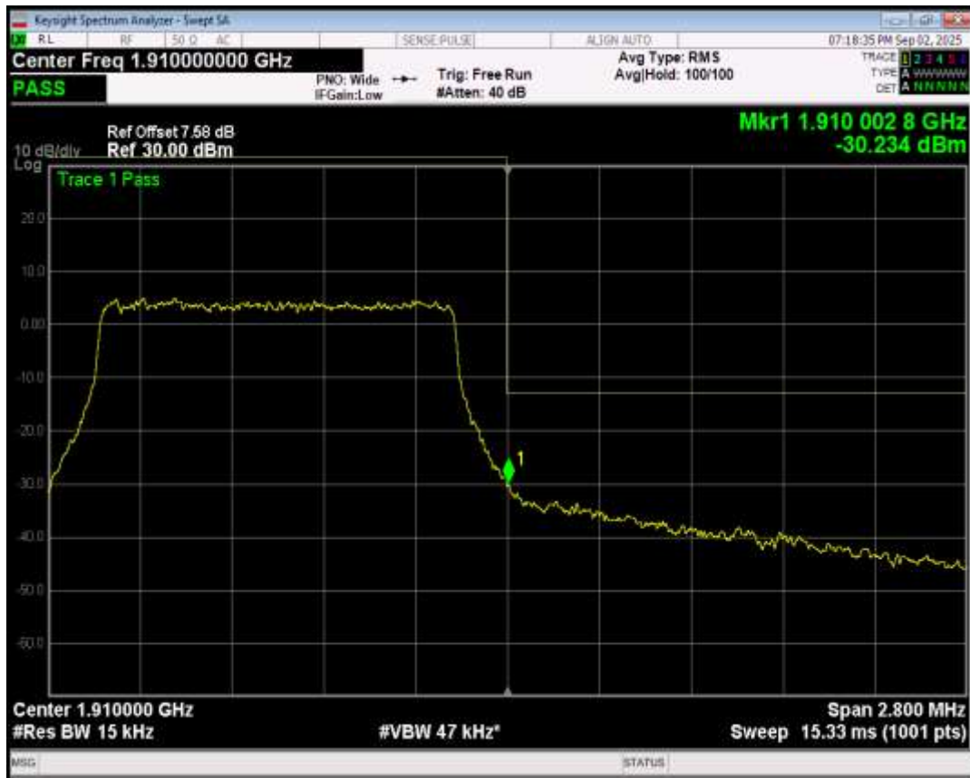
Band2 16QAM BW=1.4MHz Channel=19193 RB Size=6 Position=#0
