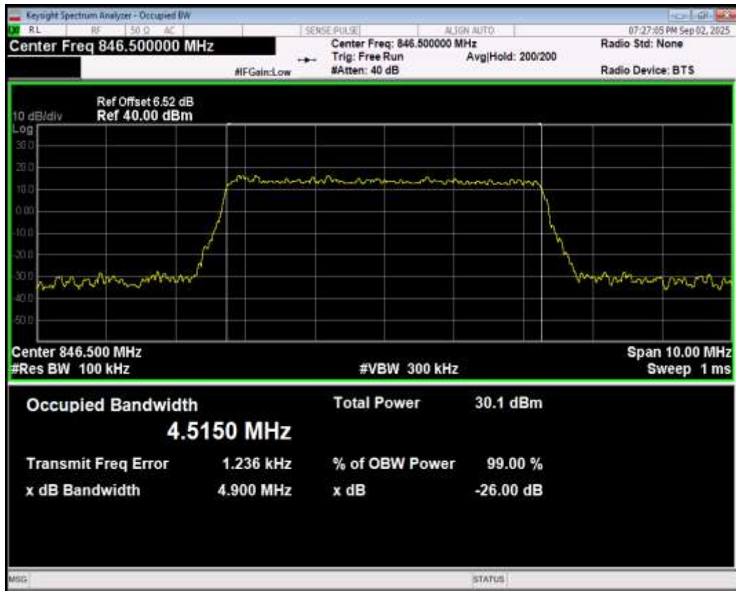
Band5 16QAM BW=5MHz Channel=20625 RB Size=25 Position=#0
