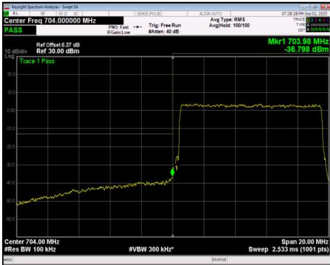
Band17 16QAM BW=10MHz Channel=23780 RB Size=50 Position=#0
