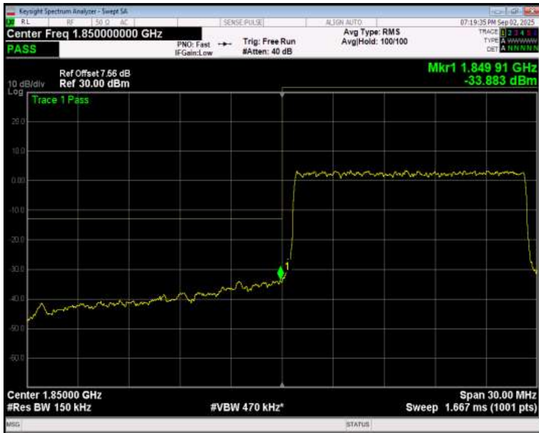
Band2 16QAM BW=15MHz Channel=18675 RB Size=75 Position=#0
