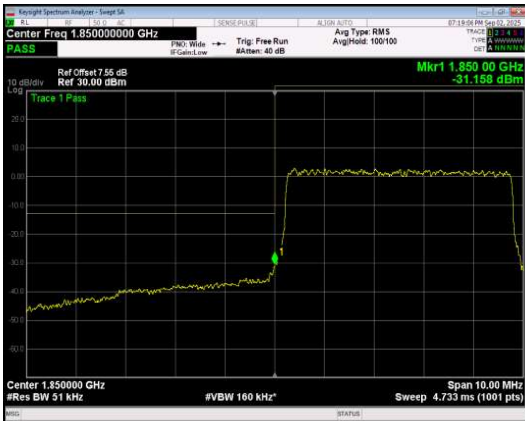
Band2 QPSK BW=5MHz Channel=19175 RB Size=25 Position=#0
