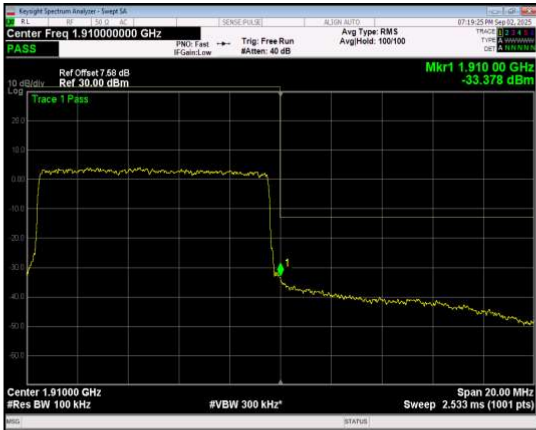
Band2 16QAM BW=10MHz Channel=19150 RB Size=50 Position=#0
