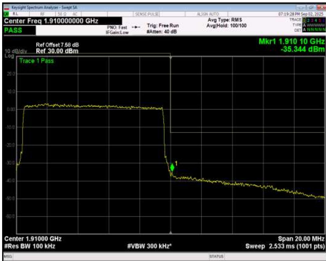
Band2 QPSK BW=15MHz Channel=18675 RB Size=75 Position=#0
