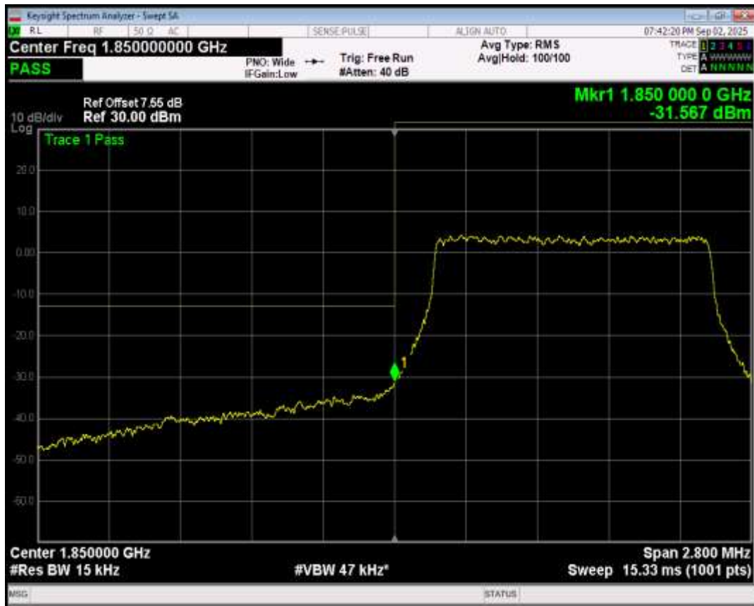
Band25 16QAM BW=1.4MHz Channel=26047 RB Size=6 Position=#0
