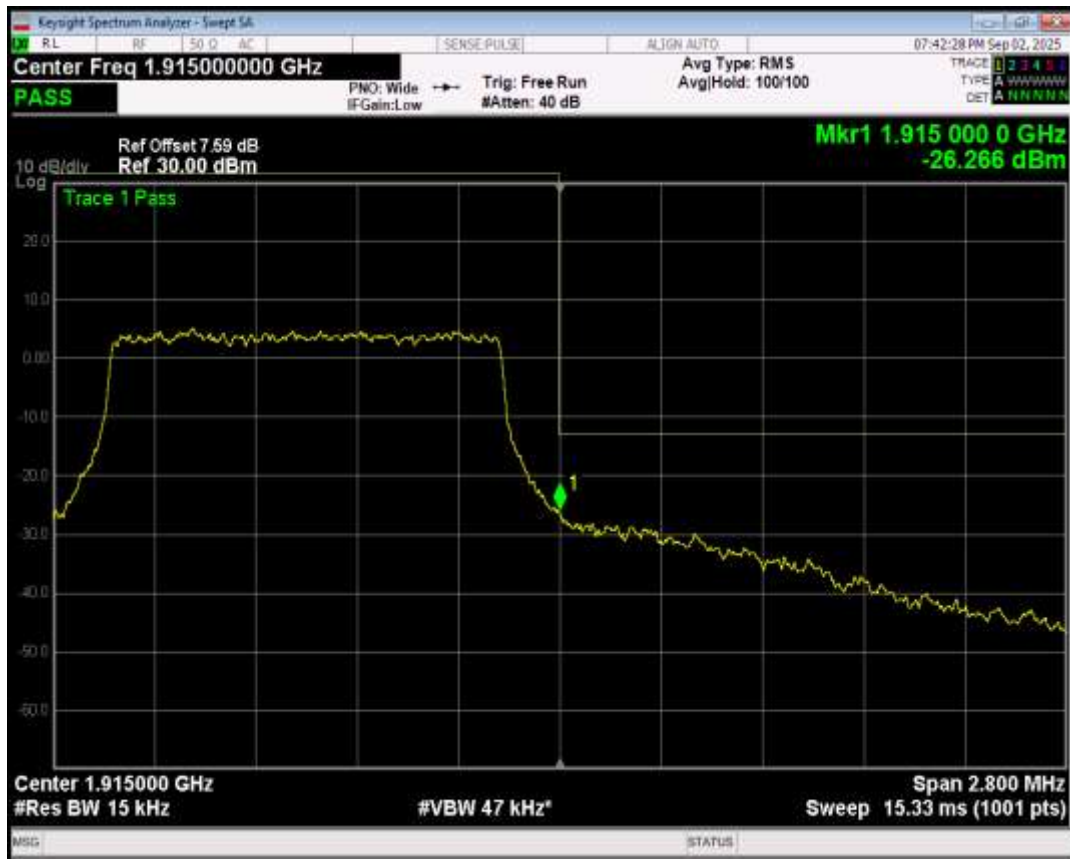
Band25 16QAM BW=1.4MHz Channel=26683 RB Size=6 Position=#0
