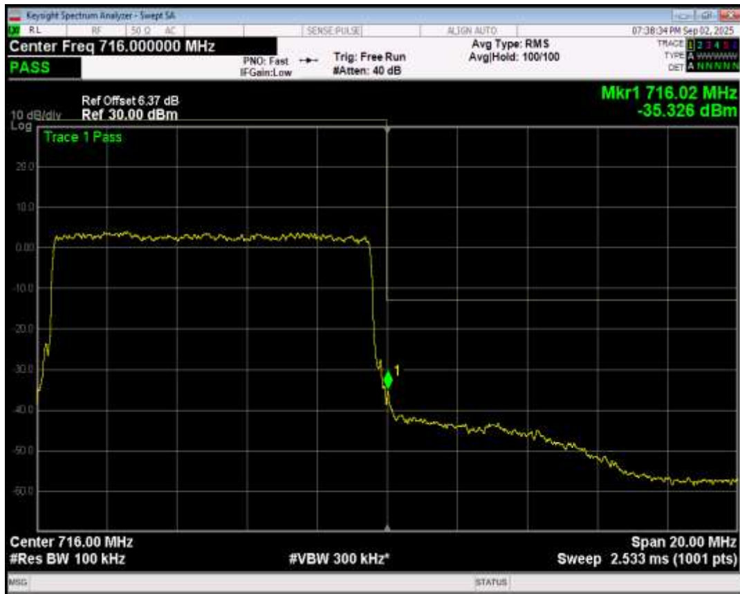
Band17 16QAM BW=10MHz Channel=23800 RB Size=50 Position=#0
