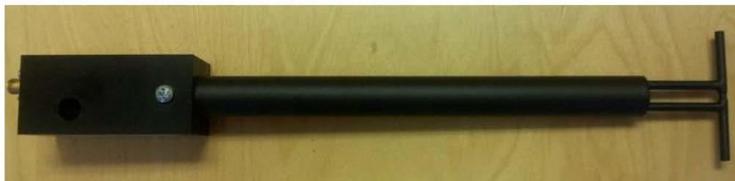
Figure 1 – MVG COMOSAR Validation Dipole
