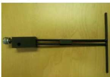
Figure 1 – MVG COMOSAR Validation Dipole
