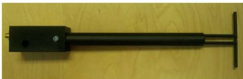
Figure 1 – MVG COMOSAR Validation Dipole
