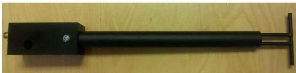
Figure 1 – MVG COMOSAR Validation Dipole
