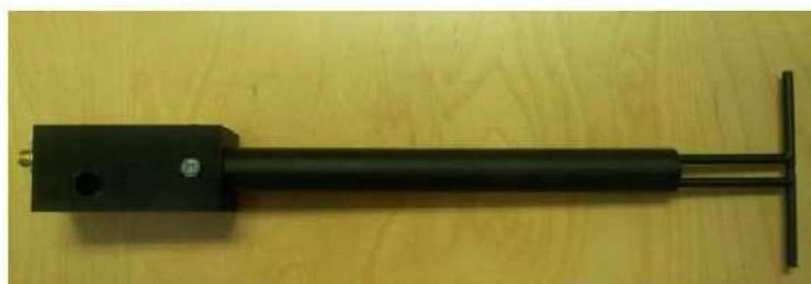
Figure 1 – MVG COMOSAR Validation Dipole
