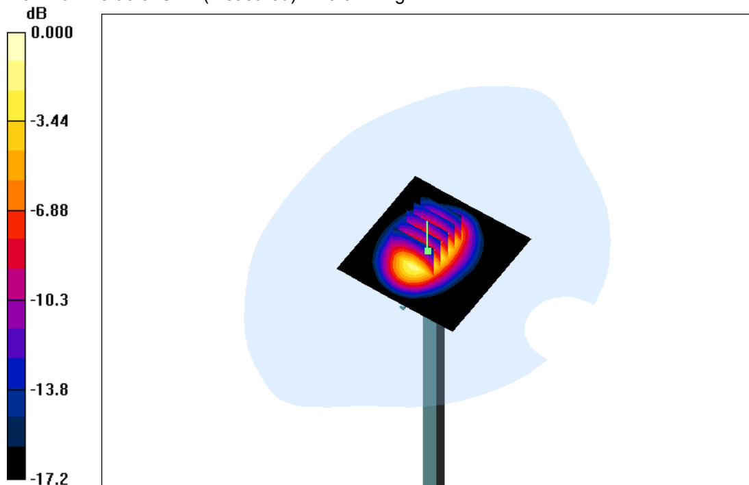
System Performance Check 1900MHz Head 250mW
