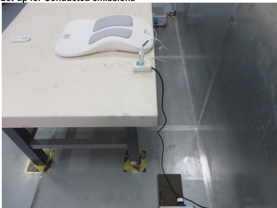
Photograph 2: Set-up for Conducted emissions
