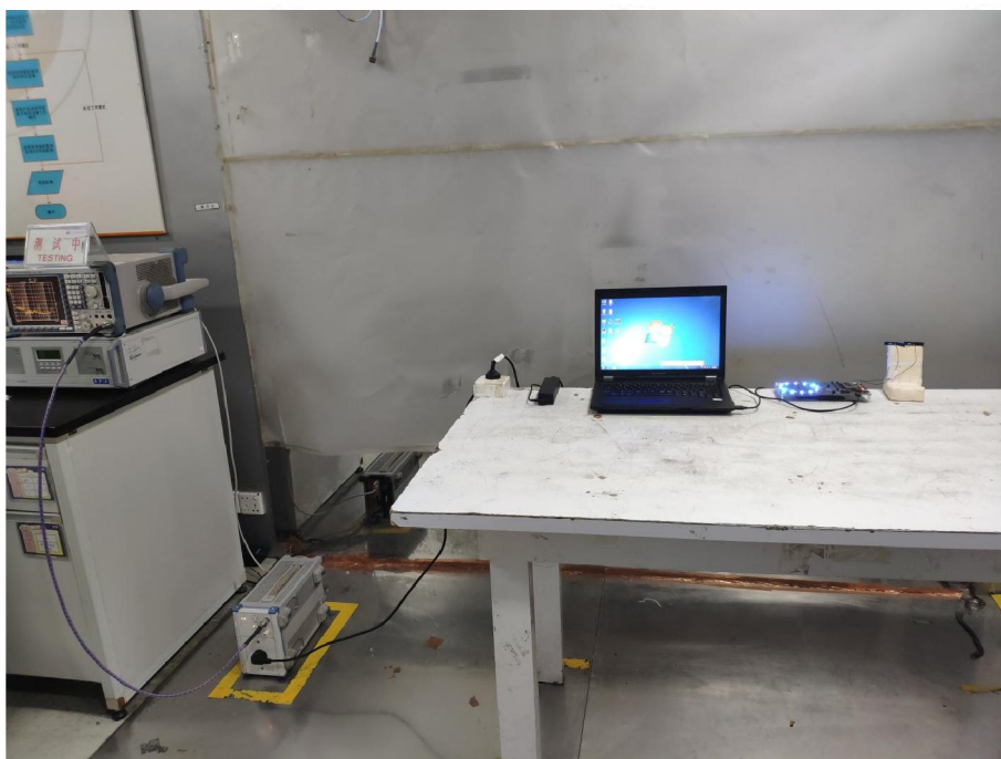
Conducted Emissions Test Setup
