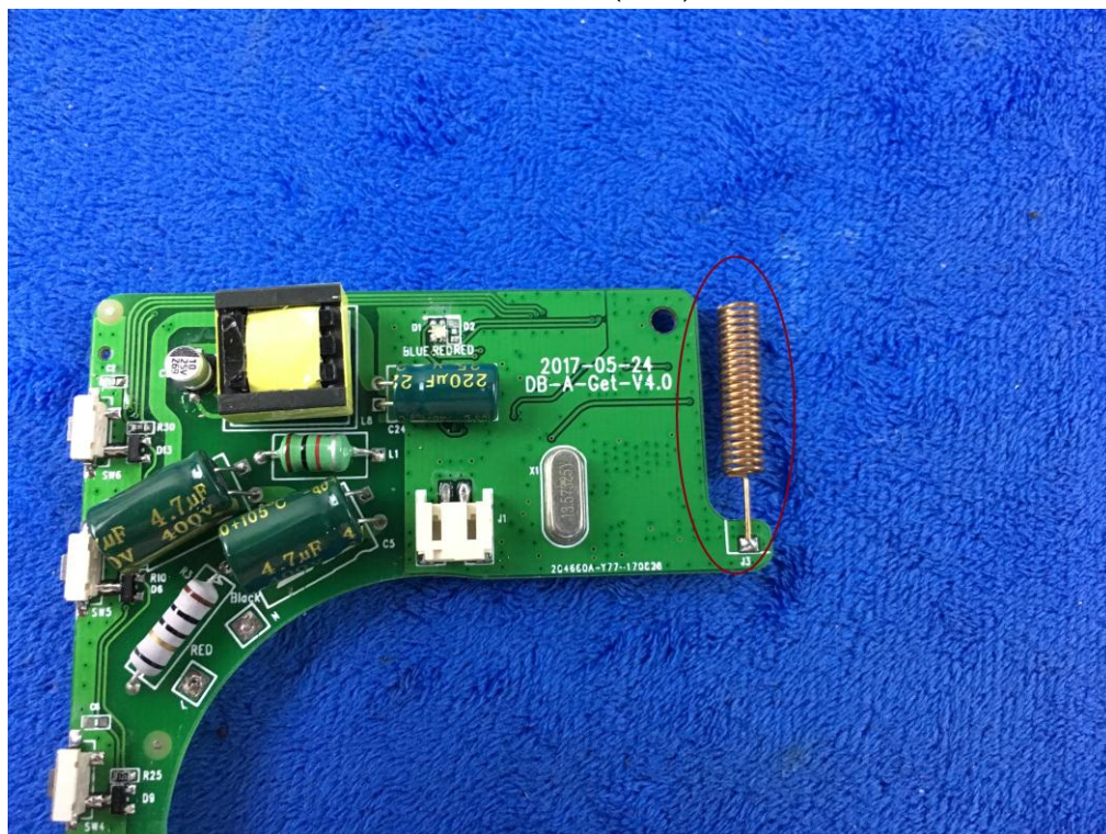
Antenna View ( RX )
