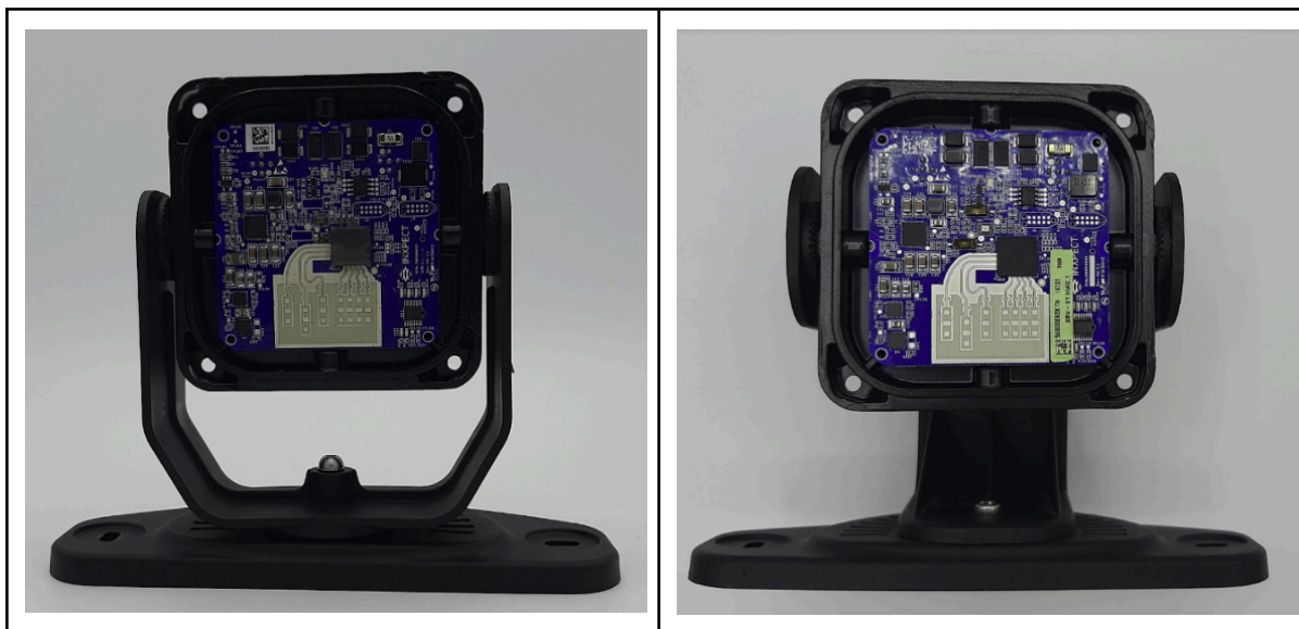
Figure 1: front view without cover with 2-axis rotating stirrup (on the left) and 3-axis rotation stirrup (on the right)
